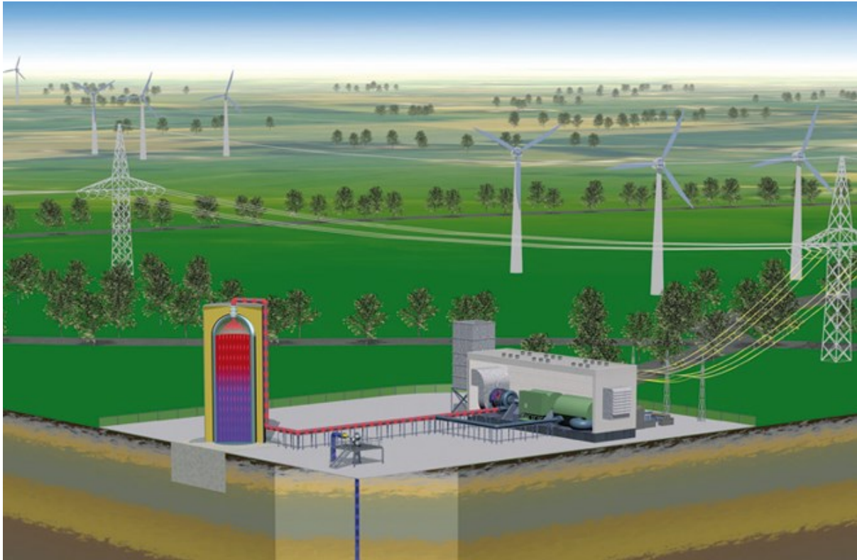
Figure 7: RWE's vision for an ACAES plant [15].
