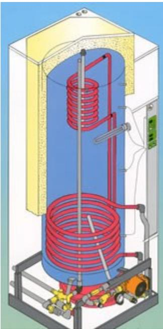
For solar domestic hot water, the heat exchanger from the solar collectors is usually placed in the bottom of the store, cf. the lower coil in figure 1. Often, an extra coil is placed in the top of the store to raise the temperature by an additional heat source, when needed.
