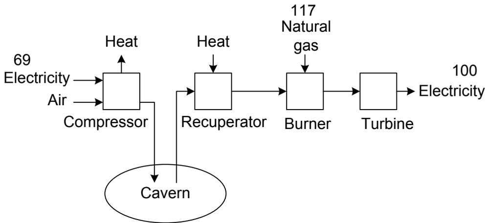
The air, which is compressed, gets warm and needs to be cooled. Similarly, the high pressure air from the cavern is cooled, when the pressure is reduced, and therefore needs to be heated before entering the burner. No external heat is needed, since heat from compression is re-used. The overall energy efficiency is  $100 / (69 + 117) = 0.54$ .
