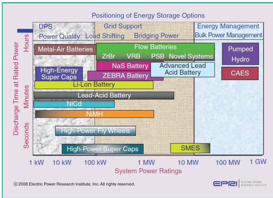
Figure: Storage technology comparison by application (power level) and storage time ([3]. UPS: Uninterruptible Power Supply (e.g. backup for data centres to support the Internet and communication centres).
