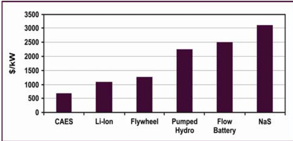
Figure: Energy storage technologies cost estimates. The CAES technology (cf. technology element 41) also requires fuel costs for discharging, which are not captured in the figure. If the system operated on compressed air alone, the costs per kilowatt (kW) would be approximately three times greater [4].
