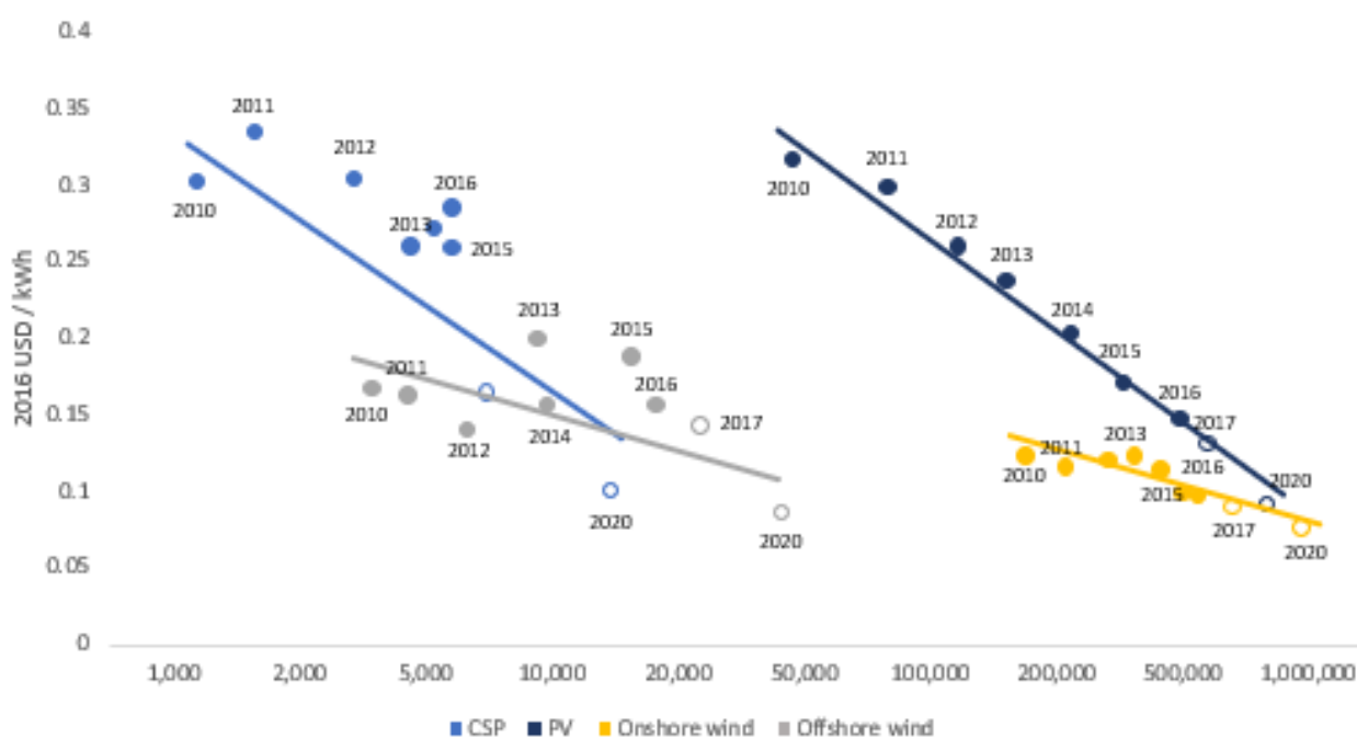
Figure 27: Learning curves for the global weighted average levelized cost of electricity from CSP, solar PV, onshore and offshore wind based on cumulative deployment, 2010-2020
