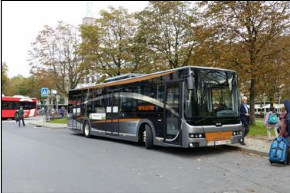
Lithium ion batteries have a current energy density of about 0.1 kWh/kg (US DOE). This would suggest that the battery pack has a weight of 3,000 kg. There will be less steel and cast iron employed as the weight of the bus is only 100 kg more than the standard bus. The default bill of material for the electric bus used in the model is shown below.
