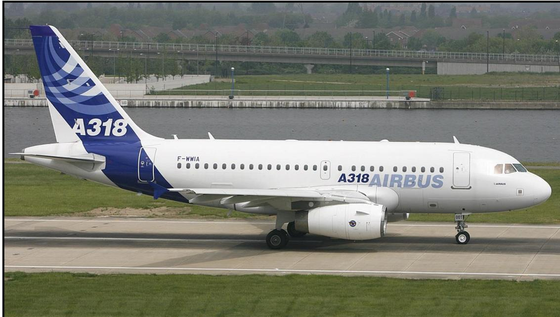
The operating empty weight of this plane is 39,500 kg (Airbus, 2009). This has been scaled to 33,776 kg for the manufacturers' empty weight and the 5,724 kg for operating items has been split to 2,862 kg for fluids and the remainder for other materials. The bill of materials for the model is shown in the following table. The steel will be assumed to be 50% high strength steel and 50% stainless steel.
