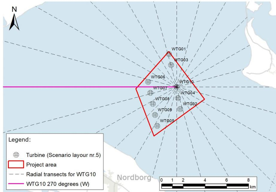
Figure 10 Radial transect used in the calculations.
