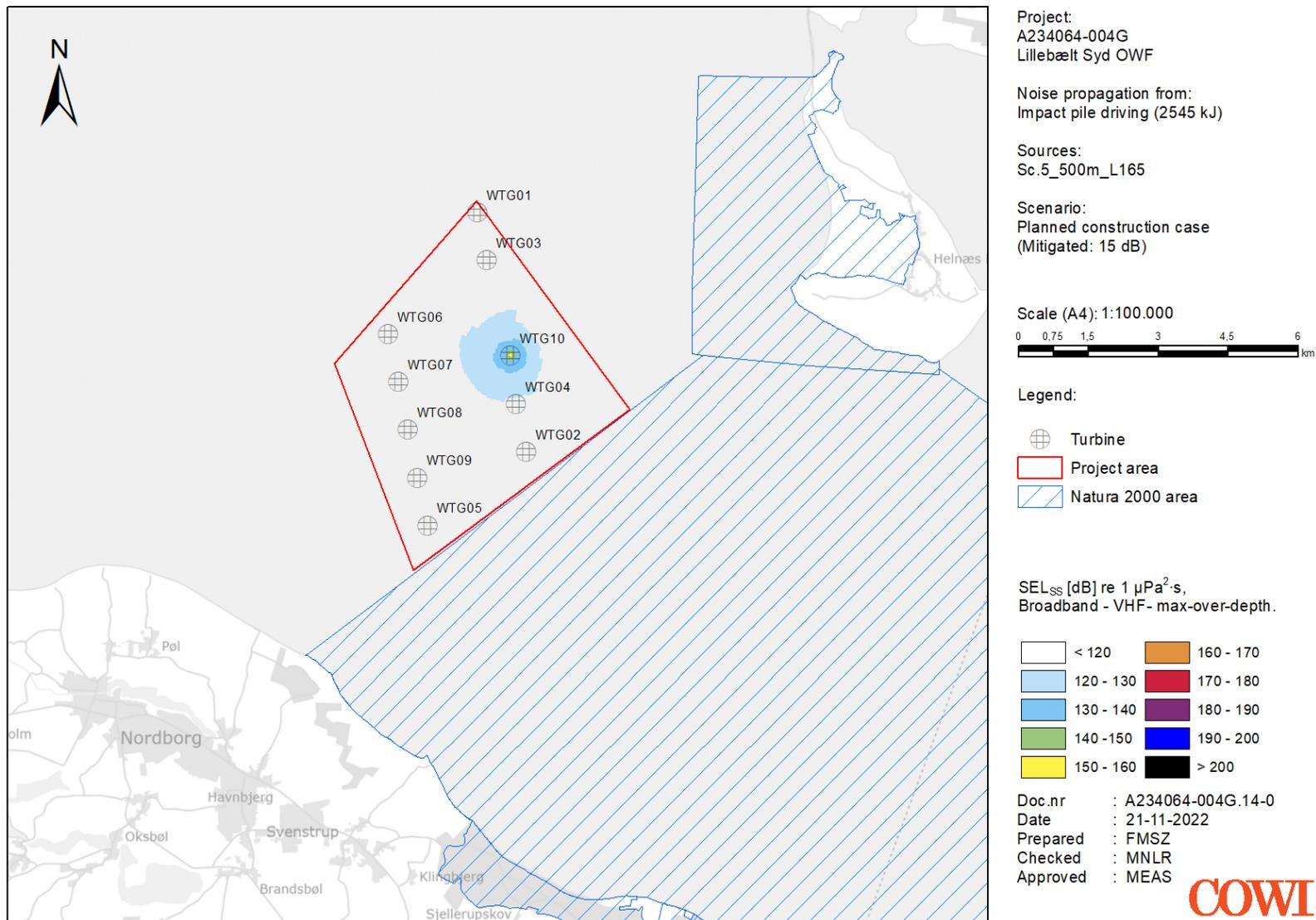
Figure 19 Construction noise map: Mitigated (15 dB) SEL<sub>SS</sub> at position WTG10
