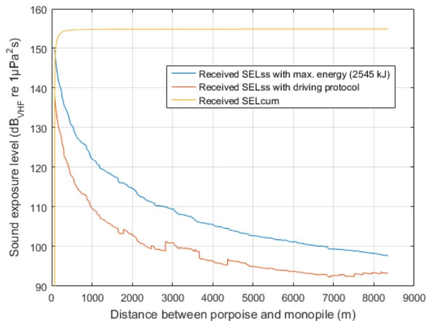
Figure 11 Calculation of  $SEL_{cum}$  under mitigated conditions (15 dB) for a porpoise with an initial distance of 75 m. Blue: Received  $SEL_{ss}$  if all hammer strikes were done at 100% energy (2945 kJ). Red: Correction of the blue plot with the actual driving protocol BH03. Yellow:  $SEL_{cum}$  calculated from the red plot as received by the animal.
