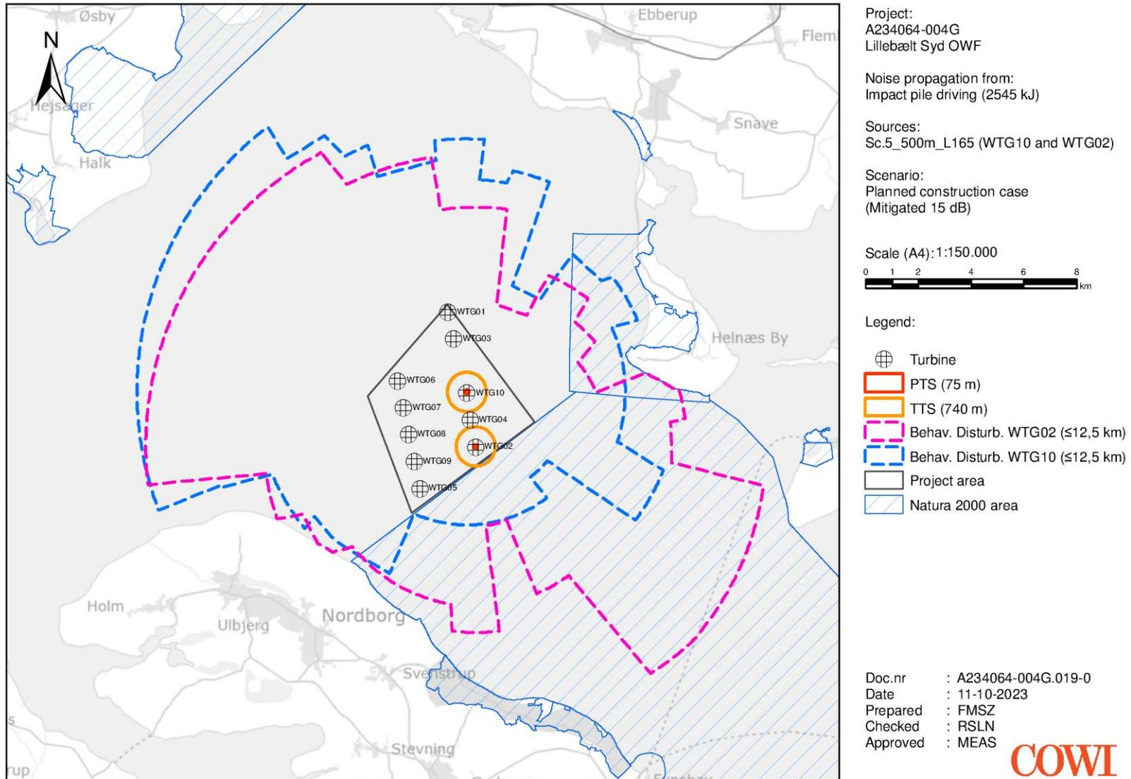
Figure 20 Construction noise map: Buffer to main thresholds depending on the porpoise's initial position. Based on  $SEL_{cum}$  and SPL calculations for a planned, mitigated (15 dB) scenario layout nr. 5. Positions WTG02 and WTG10. PTS:  $>155$  dB<sub>VHF</sub> re  $1\mu Pa^2s$ , TTS:  $>140$  dB<sub>VHF</sub> re  $1\mu Pa^2s$ , Behavioural Disturbance:  $>103$  dB<sub>VHF</sub> re  $1\mu Pa$ .
