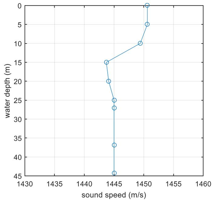
Figure 8 Derived sound speed profile (m/s) from (Lloyd’s Register, 2018).
