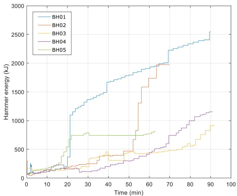
Figure 4 Driving logs showing the hammer energy as a function of time for each of the five calculated borehole positions. Extracted from (C2WIND, 2022).
