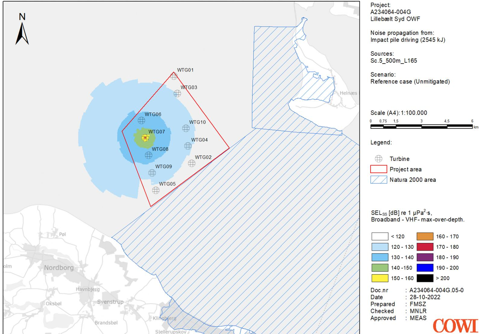
Figure 14 Construction noise map: Unmitigated SEL<sub>SS</sub> at position WTG07
