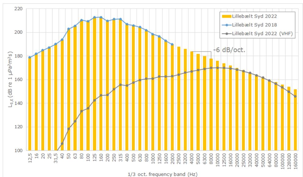
Figure 5 Source SEL<sub>SS</sub> at 1 m. Yellow: unweighted levels. Blue: unweighted levels used in the previous report (Lloyd’s Register, 2018). Gray: VHF-weighted levels. Unweighted broadband level: 220.5 dB re 1 μPa<sup>2</sup>m<sup>2</sup>s. VHF-weighted broadband level: 179.8 dB<sub>VHF</sub> re 1 μPa<sup>2</sup>m<sup>2</sup>s. Hammer energy: 2545 kJ.
