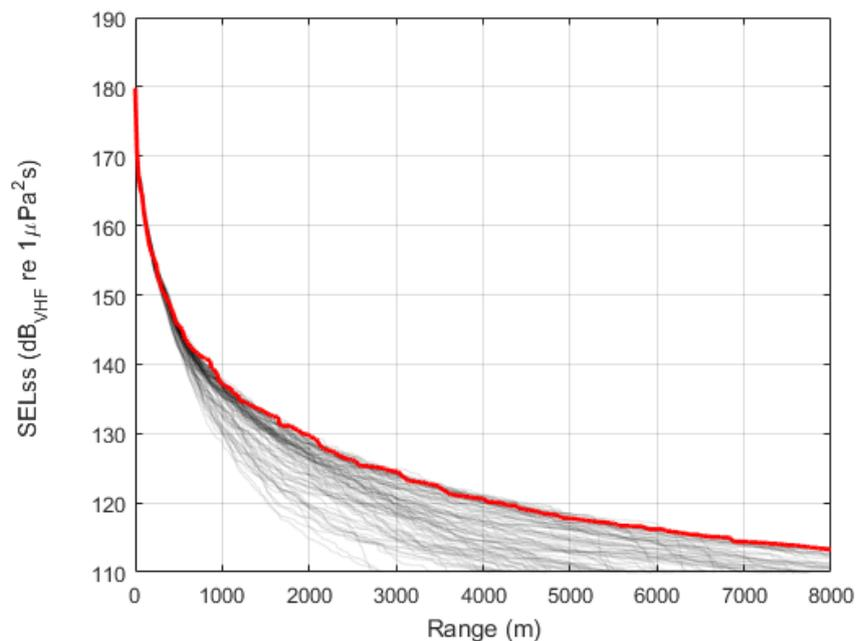
Figure 9 Ensemble of SEL<sub>ss</sub> as a function of range for the 96 calculated transects.
