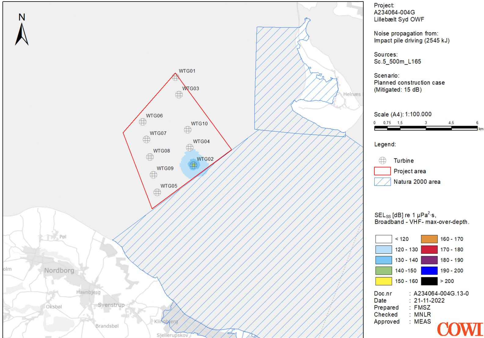
Figure 16 Construction noise map: Mitigated (15 dB) SEL<sub>ss</sub> at position WTG02
