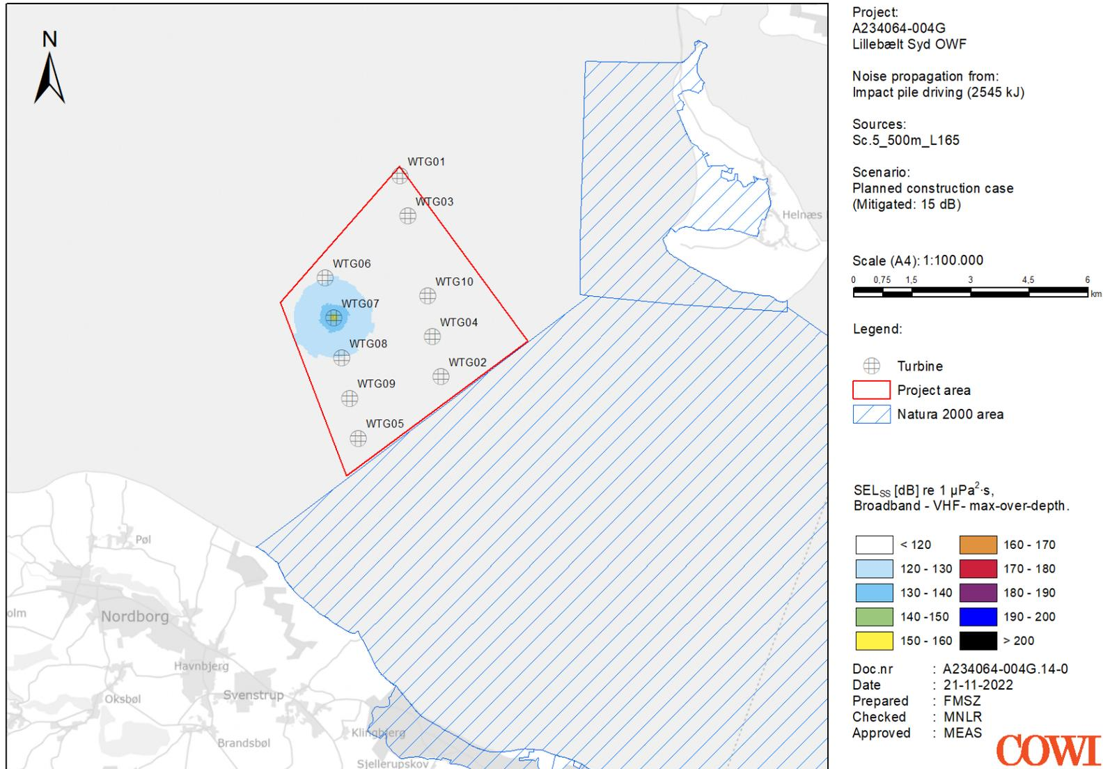
Figure 18 Construction noise map: Mitigated (15 dB) SEL<sub>ss</sub> at position WTG07
