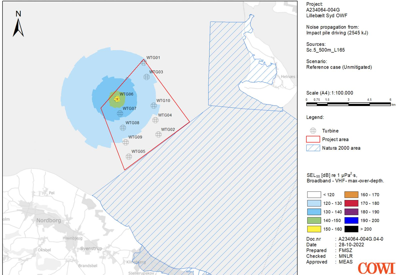
Figure 13 Construction noise map: Unmitigated SEL<sub>SS</sub> at position WTG06
