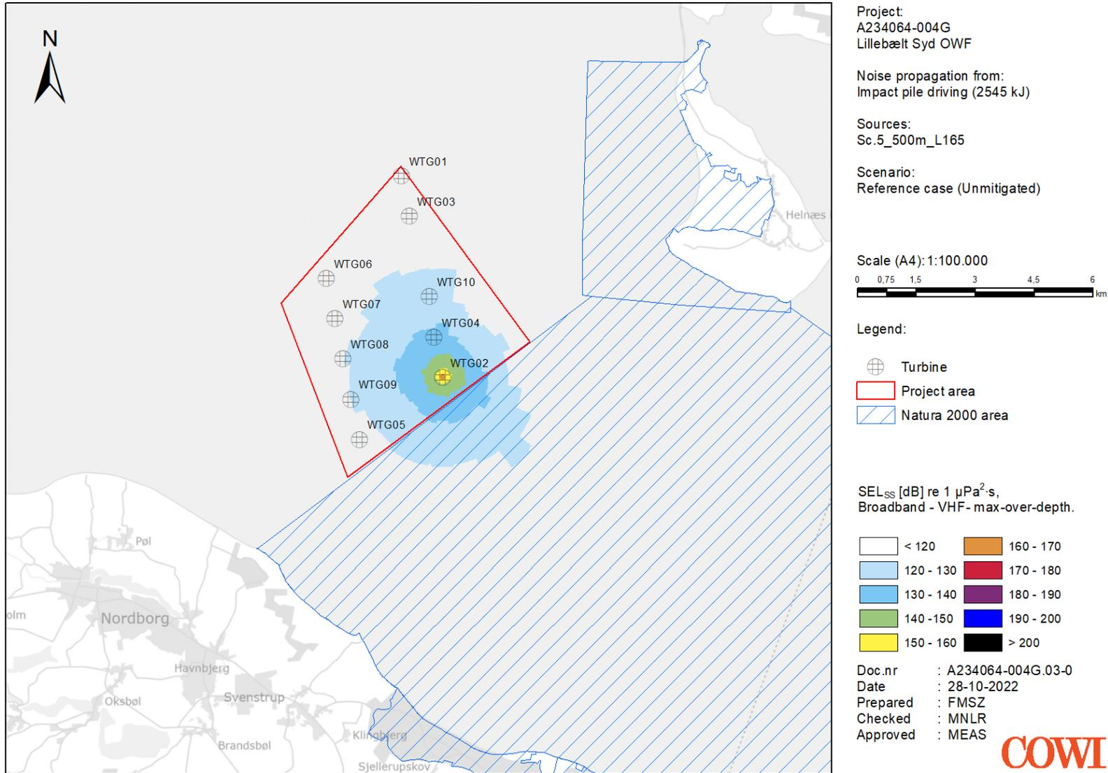
Figure 12 Construction noise map: Unmitigated SEL<sub>ss</sub> at position WTG02
