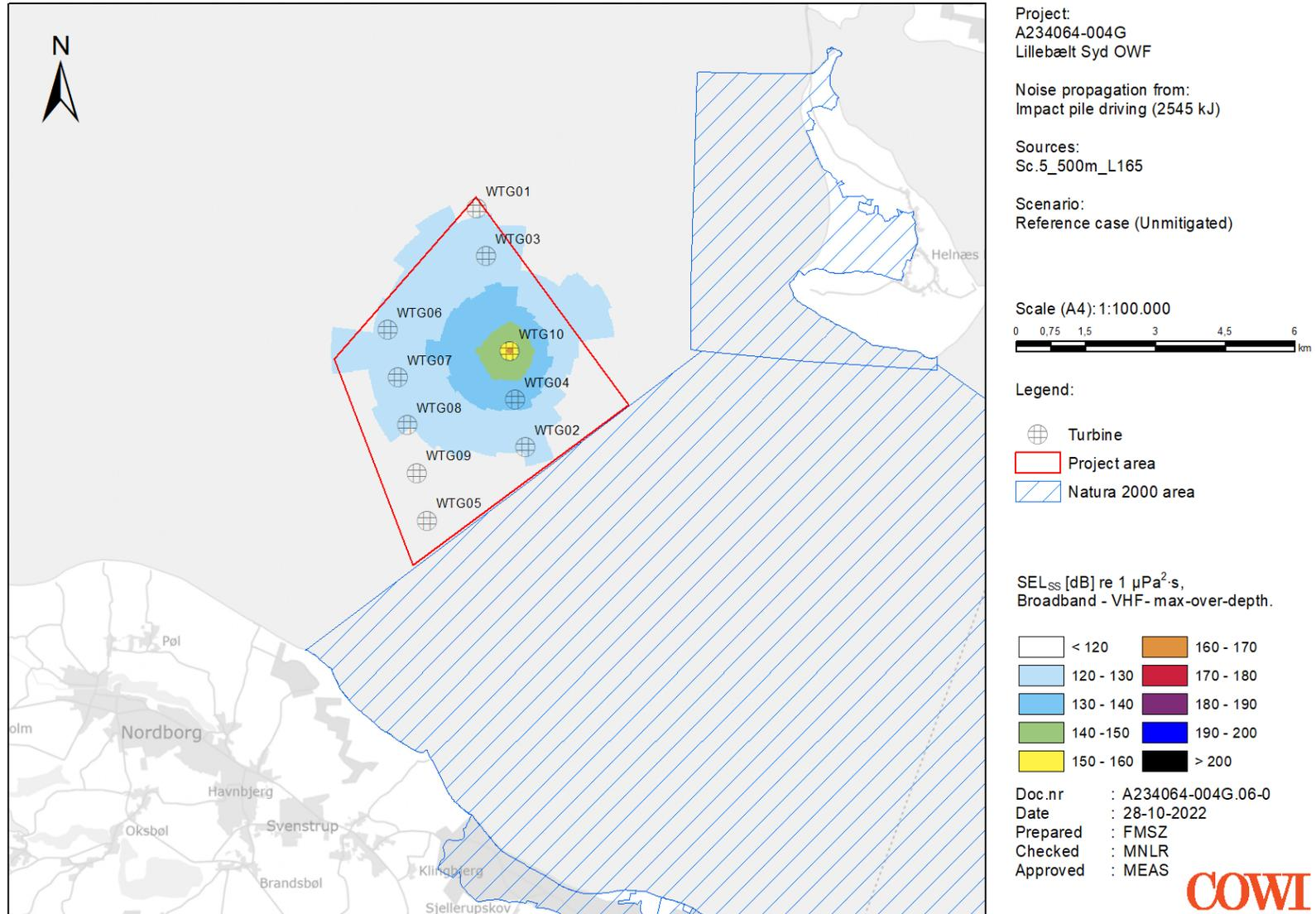
Figure 15 Construction noise map: Unmitigated SEL<sub>SS</sub> at position WTG10
