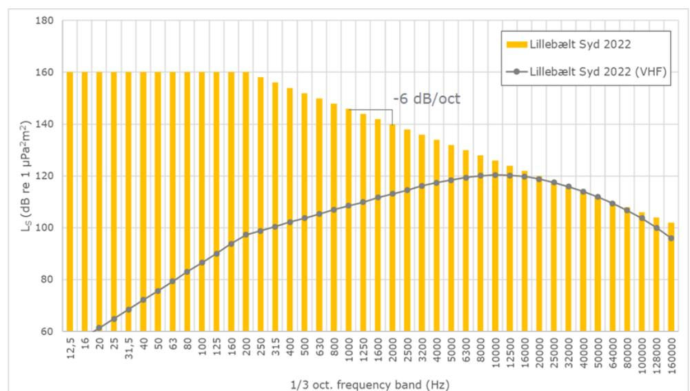
Figure 6 Source SPL at 1 m. Yellow: unweighted levels. Gray: VHF-weighted levels. Unweighted broadband level: 171.7 dB re 1  $\mu\text{Pa}^2\text{m}^{-2}$ . Turbine power: 15 MW.
