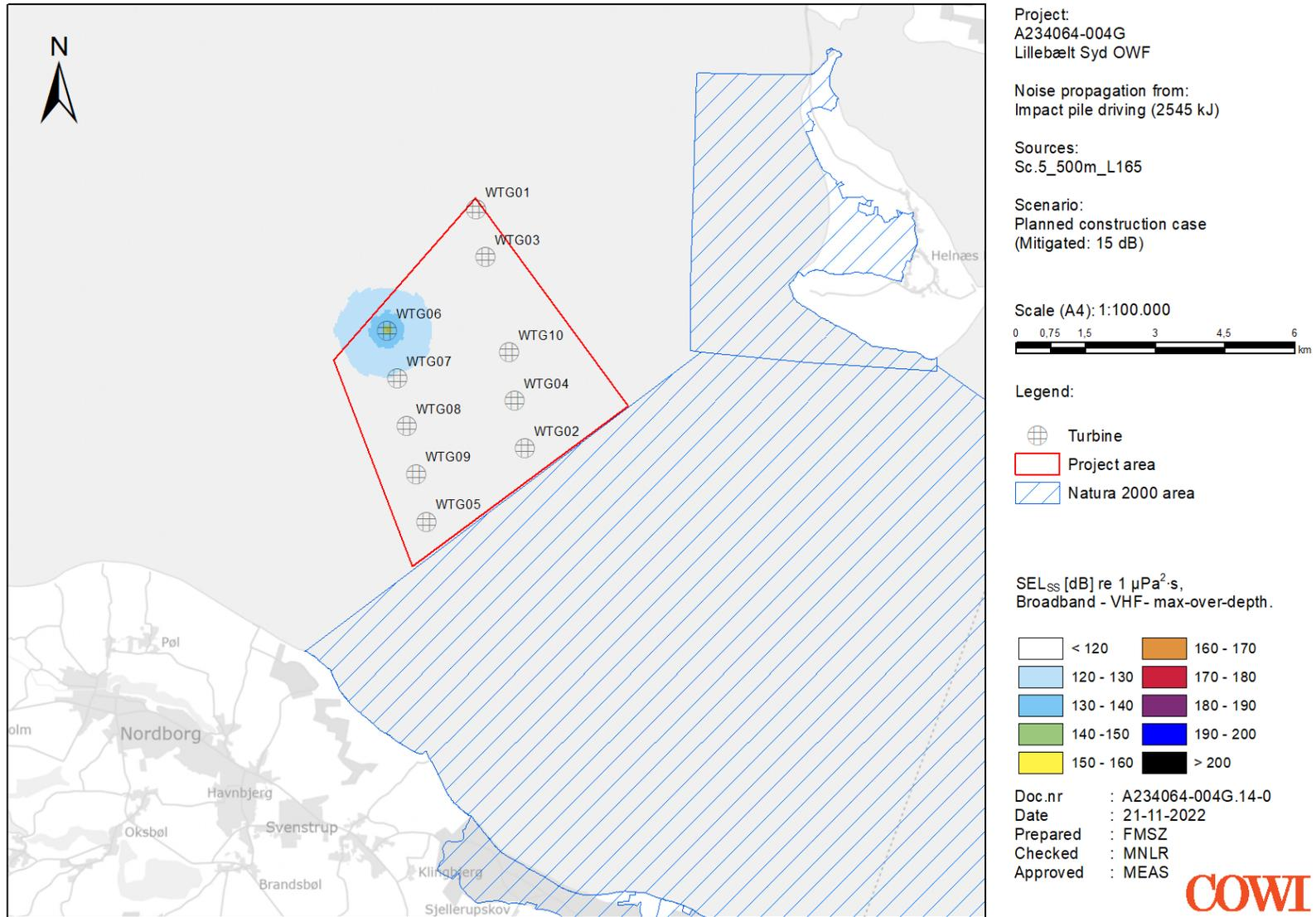
Figure 17 Construction noise map: Mitigated (15 dB) SEL<sub>SS</sub> at position WTG06
