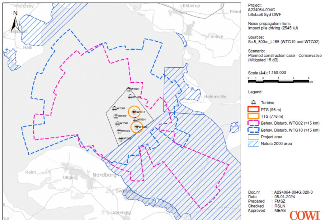
Figure 5 Resulting impact areas for porpoises (VHF) for the conservative sound speed profile and with noise mitigation (15 dB). Results shown for WTG02 and WTG10.
