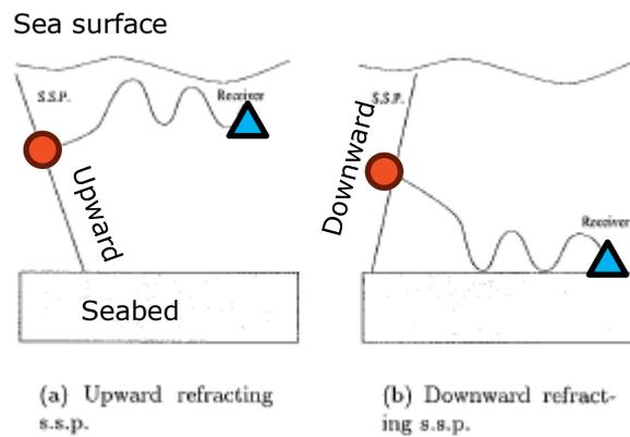
Figure 3 Generic ray traces diagrams for upward- and downward refracting sound speed profiles (s.s.p.). Reworked from (Lützen 1998). Red dot is the sound source, and blue triangle is a receiver.
