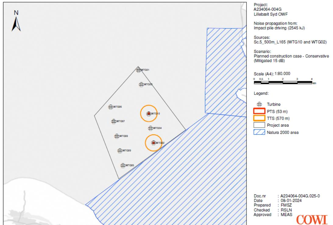
Figure 6 Resulting impact areas for harbour seals and grey seals (both PCW) for the conservative sound speed profile and with noise mitigation (15 dB). Results shown for WTG02 and WTG10.
