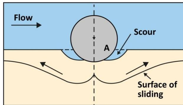
Figure 3.3 – Scour mechanism
