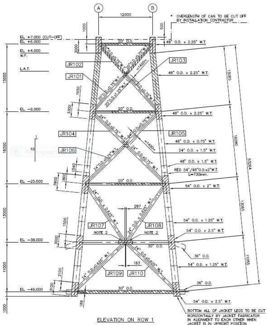
Figure 6-5 Jacket elevation.
