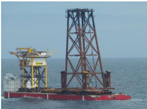
Figure 6-18 Example of transport on barge.
