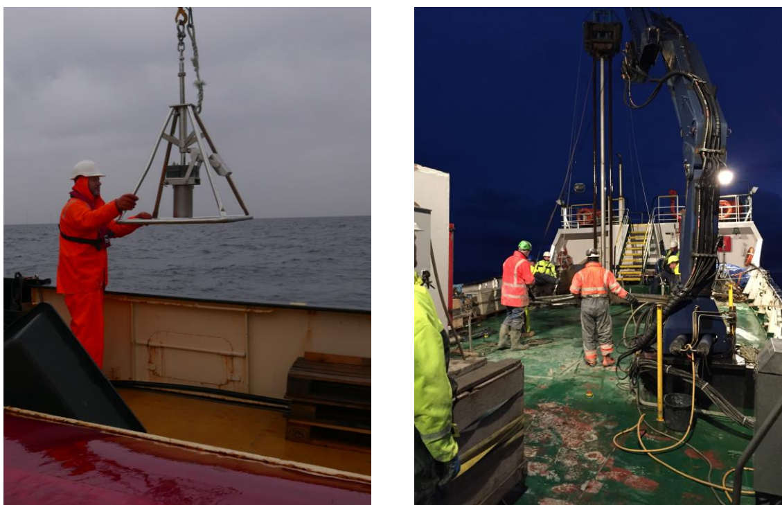
Figure 7-4 HAPS core sampler for surface sediment sampling (left) and Vibrocore sampler for deeper sediment samples (right).
