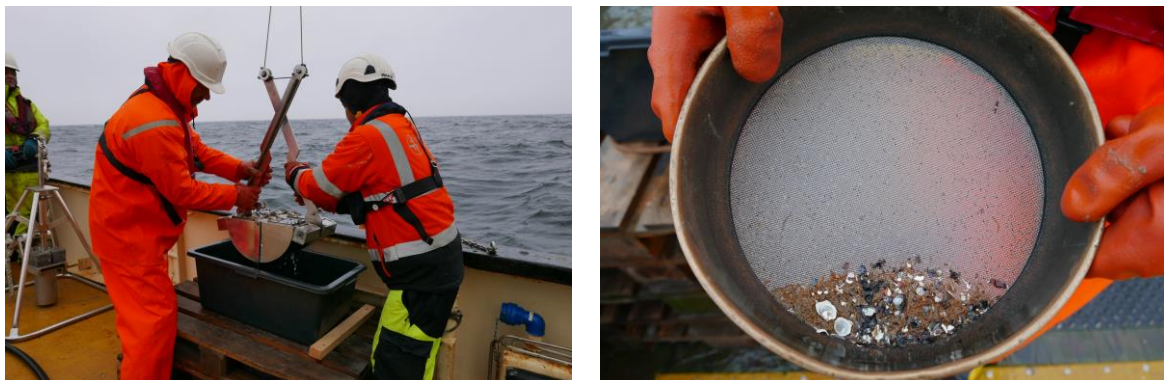
Figure 7-8 Sampling of infauna was undertaken with a Van Veen sampler (left). An example of an infauna sample (right).
