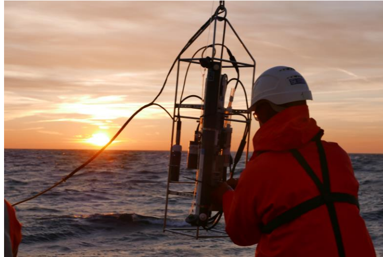
Figure 7-2 CTDO profiler and Niskin water sampler.
