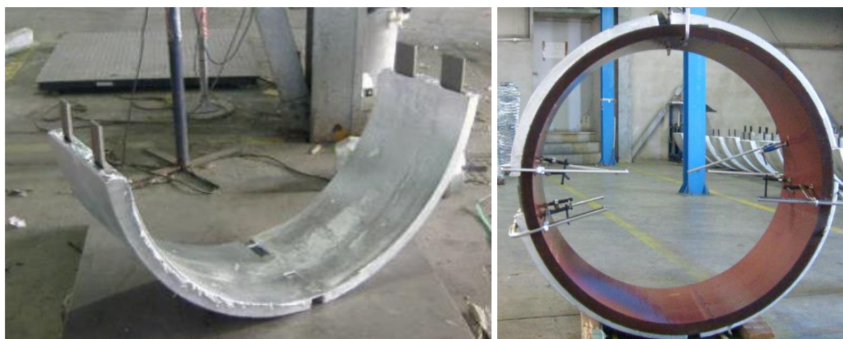
Figure 6-10 Bracelet anode. Left: a half shell; right: two half shells trial fitted to a pipe.
