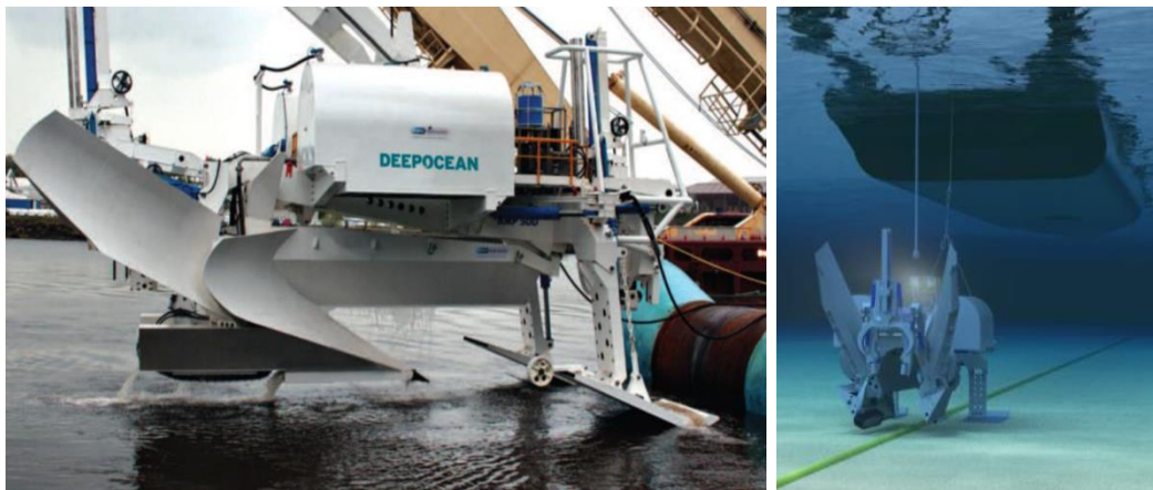
Figure 6-21 Post-lay trenching. Typical pipeline plough in operation on the seabed.
