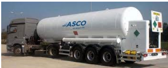
Figure 7. CO 2 semi-trailer from ASCO. Source; www.ascoco2.com
