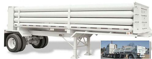
Figure 38: Trailer and storage is same vessel.
