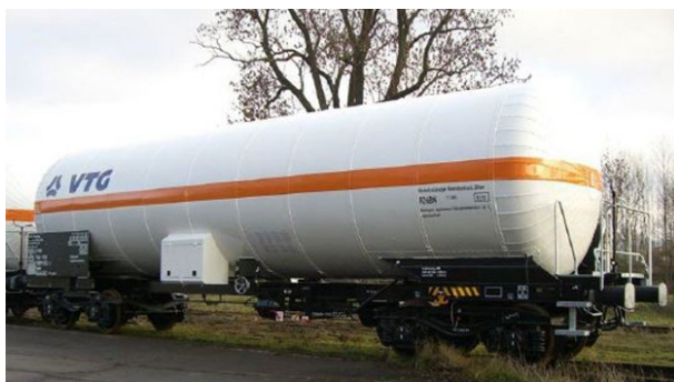
Figure 8. Railroad car for liquid CO 2 transport. Source: www.VTG.com
