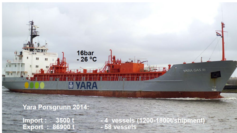
Figure 6. M/T Yara Gas III liquid CO 2 carrier. [7]
