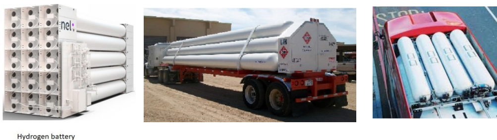
Figure 9: Hydrogen storage, transportation and fuel tank.
