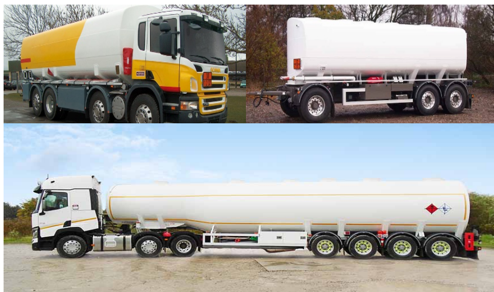
Figure 17: a) Tank, b) trailer, and c) tank trailer (semi-trailer)
