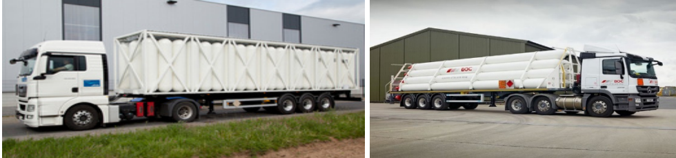
Figure 19: Hydrogen tube trailer types
