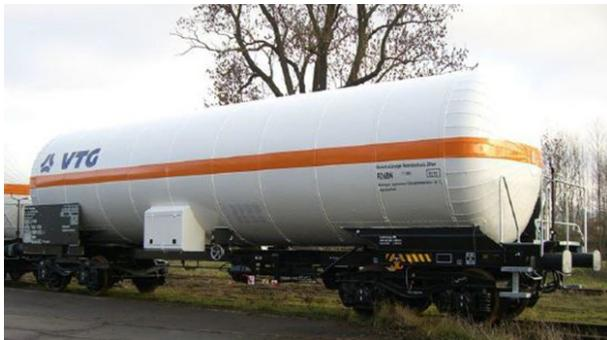
Figure 8. Railroad car for liquid CO<sub>2</sub> transport. Source: [www.VTG.com](http://www.VTG.com)
