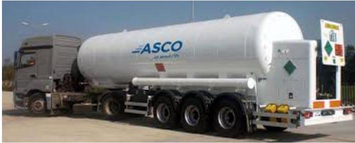
Figure 7. CO<sub>2</sub> semi-trailer from ASCO. Source; [www.ascoco2.com](http://www.ascoco2.com)
