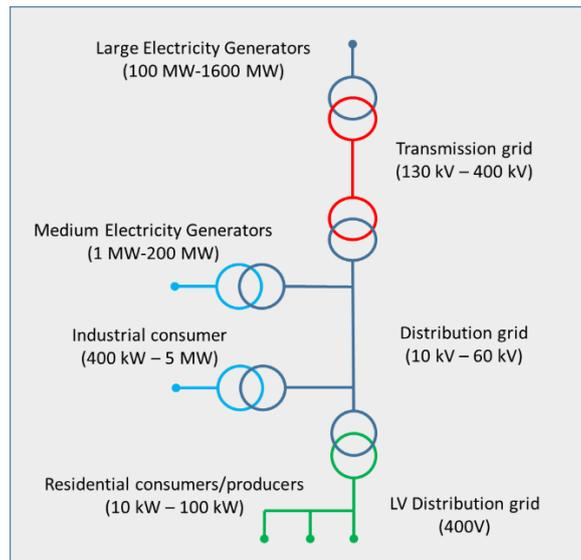
Figure 1: Major components in an electric power grid
