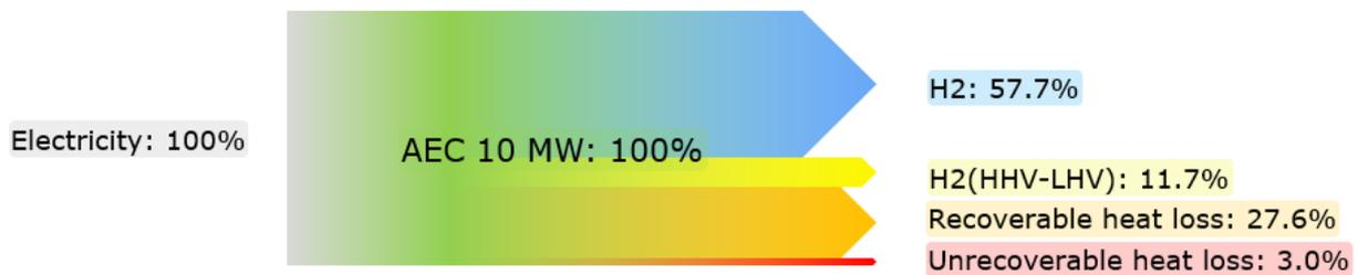
Figure 9 The energy inputs and outputs of an AEC (2020, 10 MW hydrogen plants). Data is derived from Ramboll references.
