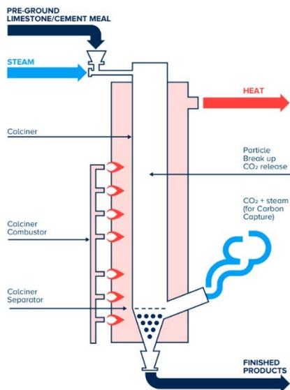
Figure 25 The heart of the process is the indirect fired LEILAC calcinatory.[8]
