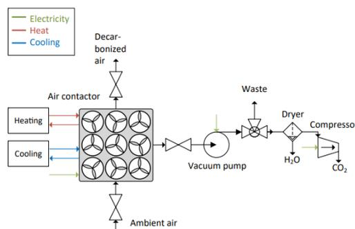
Figure 37. Solid adsorption direct air capture layout [2].
