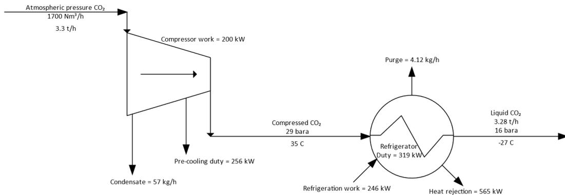
Figure 58: Example of the energy balance for a CO<sub>2</sub> compression and liquefaction plant.
