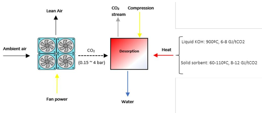
**Figure 41. DAC energy balance diagram.** Yellow arrows represent electrical energy. Black arrows stand for the air streams entering the system and the red arrow the heat requirements for CO<sub>2</sub> desorption.
