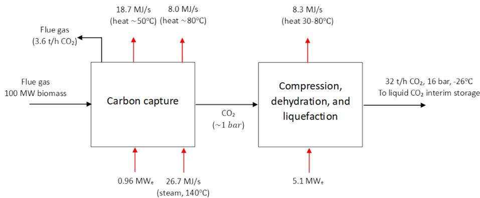
Figure 10. Illustration of energy balance for a CO<sub>2</sub> capture and liquefaction plant treating all flue gas from a 100 MW<sub>th</sub> biomass boiler that is equipped with flue gas condensation. 90% of the CO<sub>2</sub> in the flue gas is captured corresponding to 32 t CO<sub>2</sub> output per hour. Black arrows: Mass streams. Red arrows: Energy streams.
