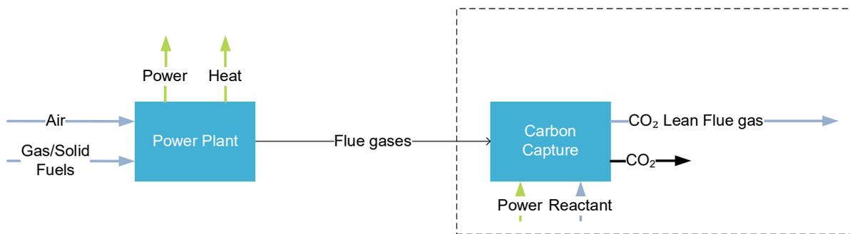
Figure 3: Post combustion
