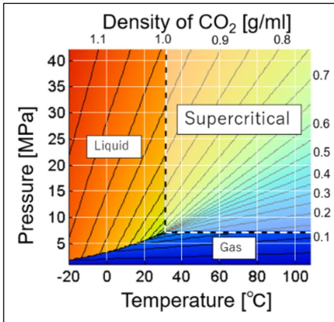
Figure 64. CO<sub>2</sub> density at varying pressure and temperature Image source: ITEC Co., Ltd. Osaka, Japan.
