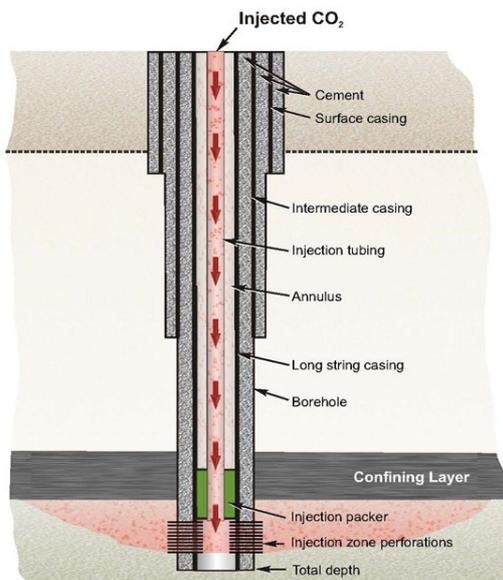
Figure 0-33: High level diagram of injection well [23]
