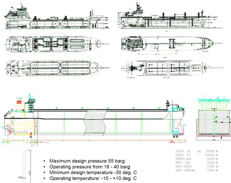
Figure 66. Top) Sketch of refrigerated CO<sub>2</sub> ship designs for Gassco Concept study [12]. Bottom) sketch of Knutsen Shipping’s design of a pressurised CO<sub>2</sub> carrier (PCO<sub>2</sub>) [13].
