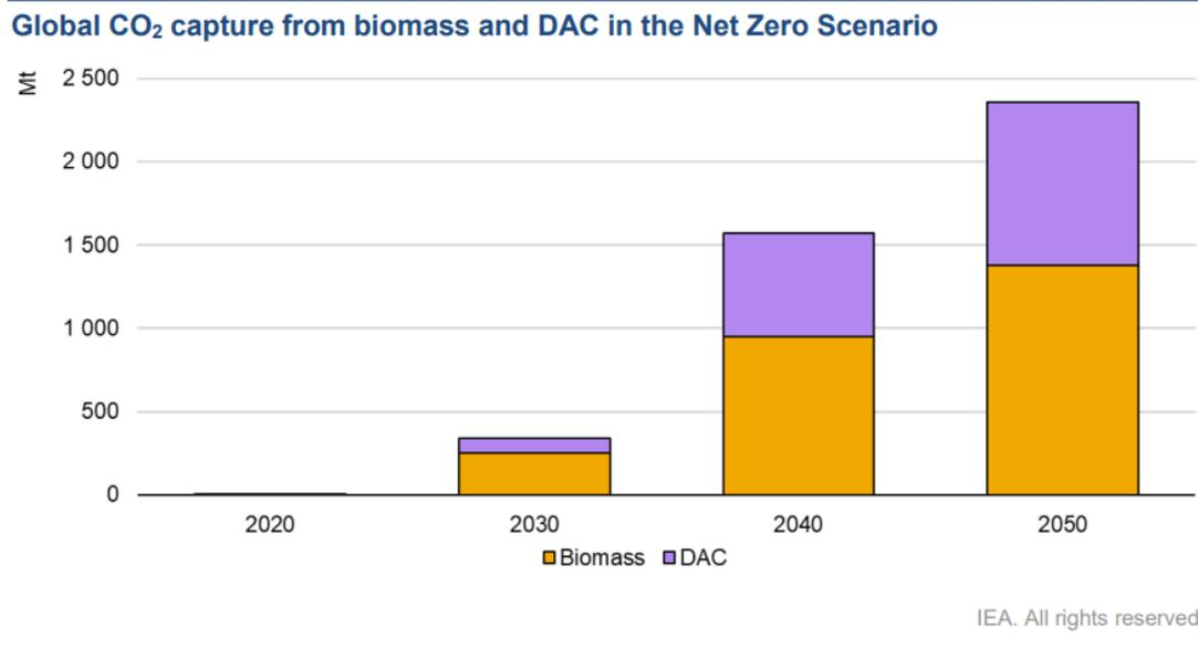
Figure 39. DAC global CO<sub>2</sub> capture demand in the Net Zero Scenario [12].
