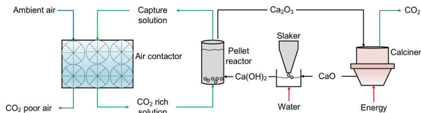
Figure 38. Liquid absorption direct air capture process flowsheet [6].
