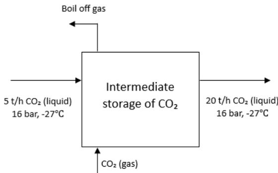
Figure 62. Overview of input and output for intermediate storage of CO<sub>2</sub>.
