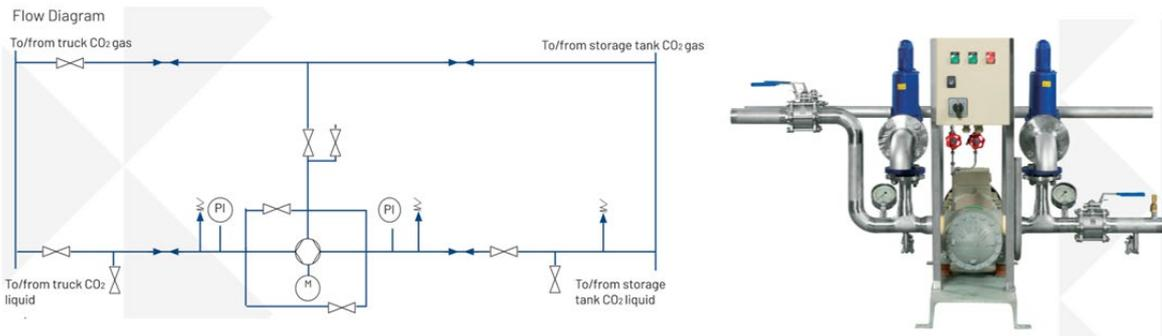
Figure 61. Truck filling unit. Source: [Pentair - CO<sub>2</sub> Truck Filling Unit - TFU - Pentair | Pentair Food & Beverage \[2\]](#)
