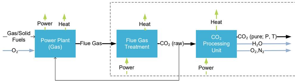
Figure 5: Oxy-fuel combustion
