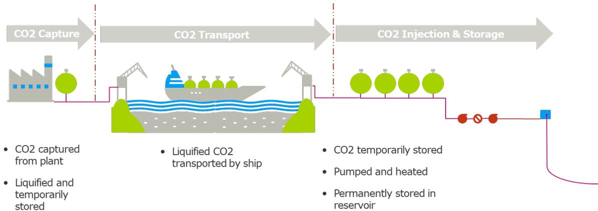
Figure 0-11: Interface between the different elements of CCS
