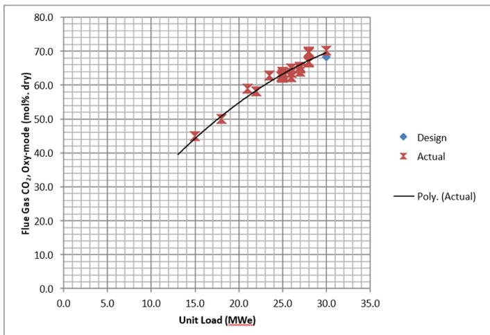
Figure 27 CO<sub>2</sub> concentration dependent on load at Callide oxy-fuel plant from [11]
