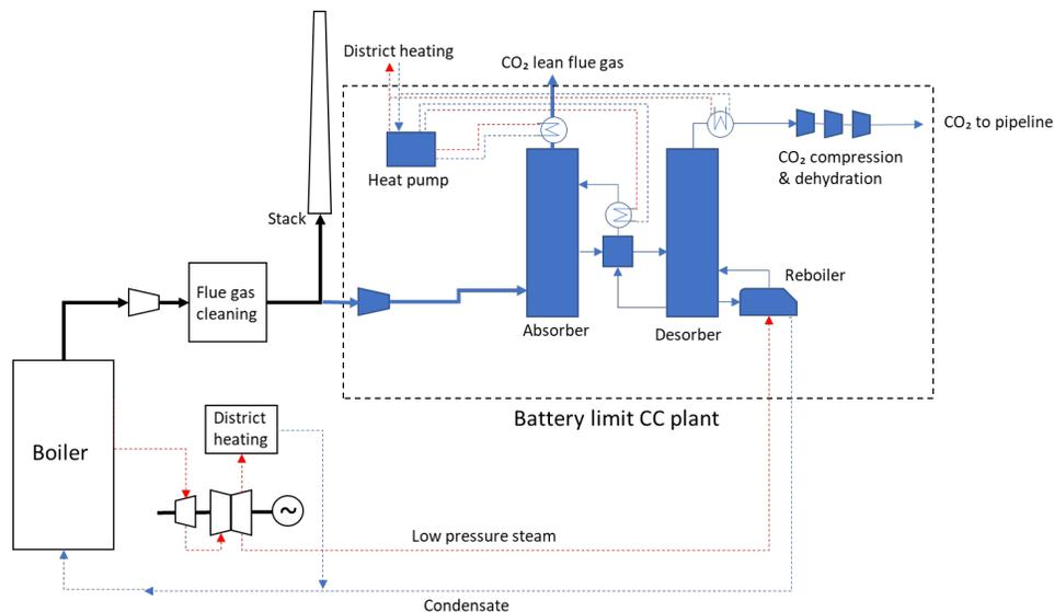
**Figure 11. Illustration of amine CC retrofit to CHP plant. The CC plant includes a booster fan and CO<sub>2</sub> compression plant. The pre-scrubber has been omitted as the CHP has flue gas condensation and excellent flue gas cleaning. As an option heat pumps may be used to upgrade low value heat from CC plant to district heating.**
