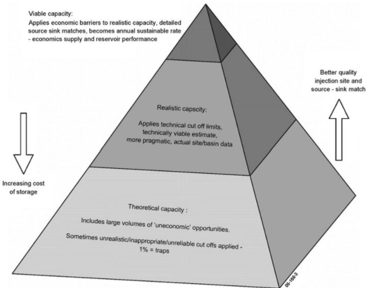
Techno-economic resource pyramid for capacity for CO<sub>2</sub> geological storage, showing the three levels of theoretical, realistic and viable estimates. Theoretical includes the entire pyramid, realistic the top two portions and viable only the top portion.
