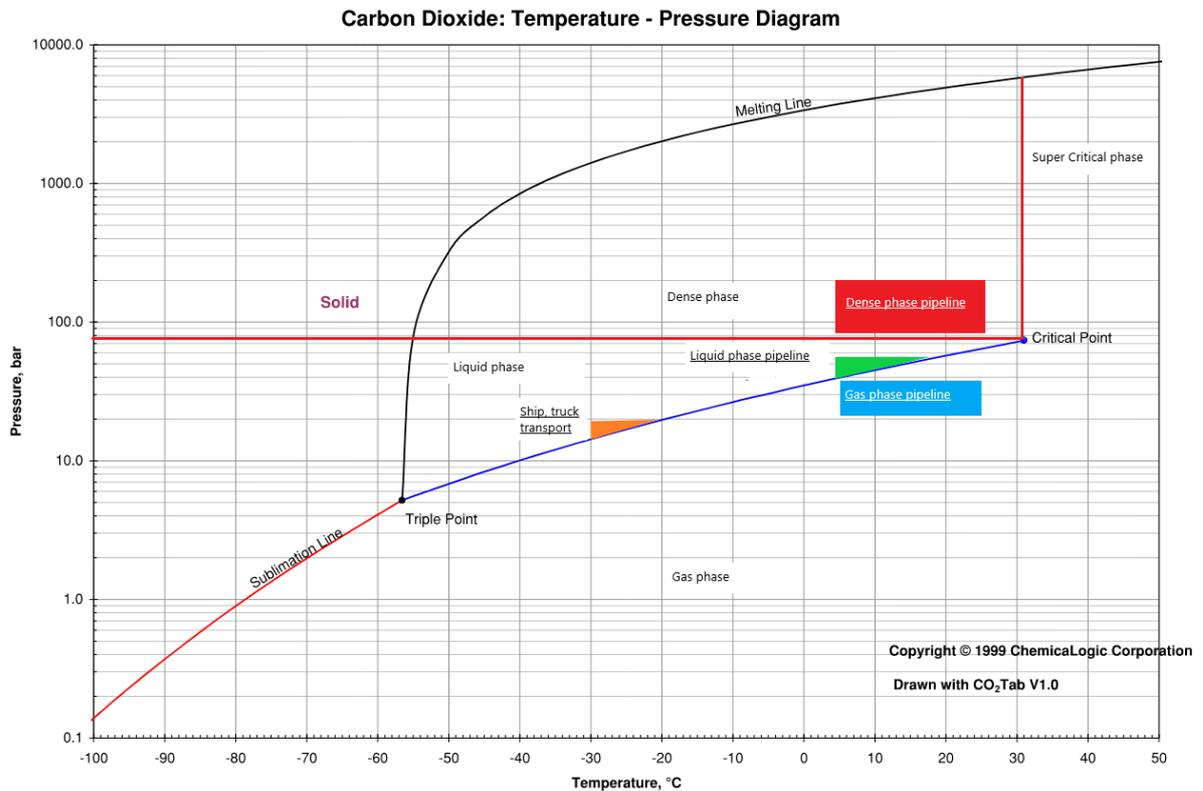
Figure 45. CO<sub>2</sub> phase diagram with the options for liquid-, gas- and dense phase transportation.
