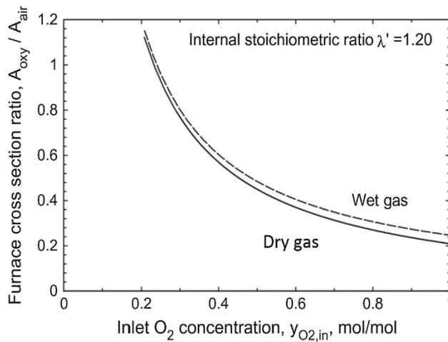
Figure 29 Potential to reduce boiler size by increasing O<sub>2</sub> concentration.[14]
