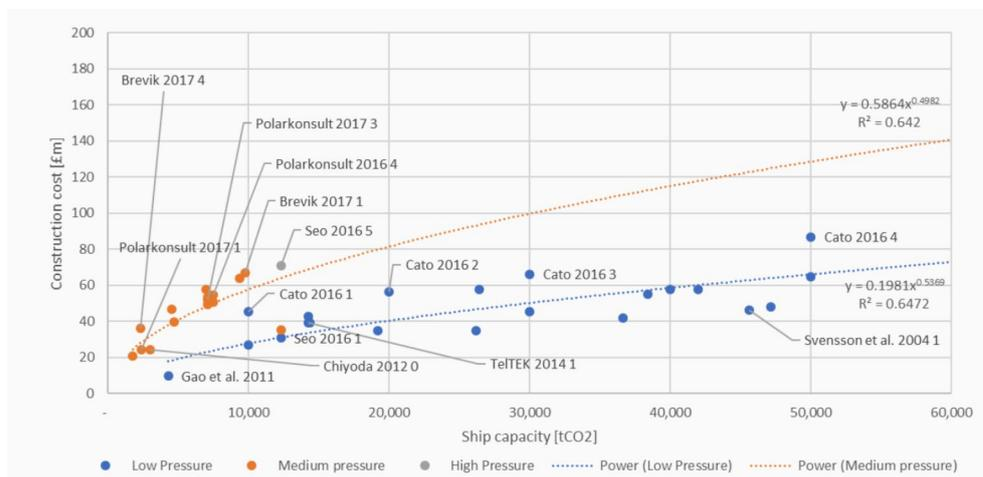
**Figure 67. Investment cost for CO<sub>2</sub> carriers as a function of capacity from [9]. Low pressure 5-8 bar, Medium pressure: 15-20 bar.**
