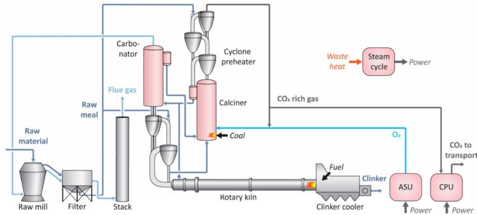
Figure 22. Partial oxy-fuel combustion with integrated Calcium looping.[3]
