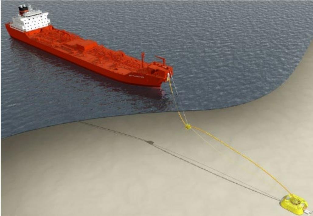
Figure 0-30: Single Anchor Loading system (NOV) [22]
