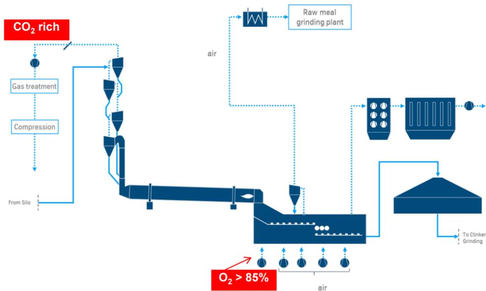
Schematic diagram of a 2<sup>nd</sup> generation oxyfuel cement plant without flue gas recirculation circuit
