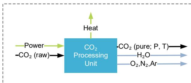
Figure 7. Illustration of CO<sub>2</sub> processing (conditioning) unit.
