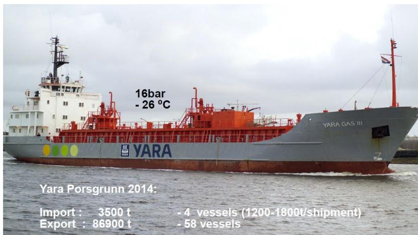
Figure 49. M/T Yara Gas III liquid CO<sub>2</sub> carrier. [7]
