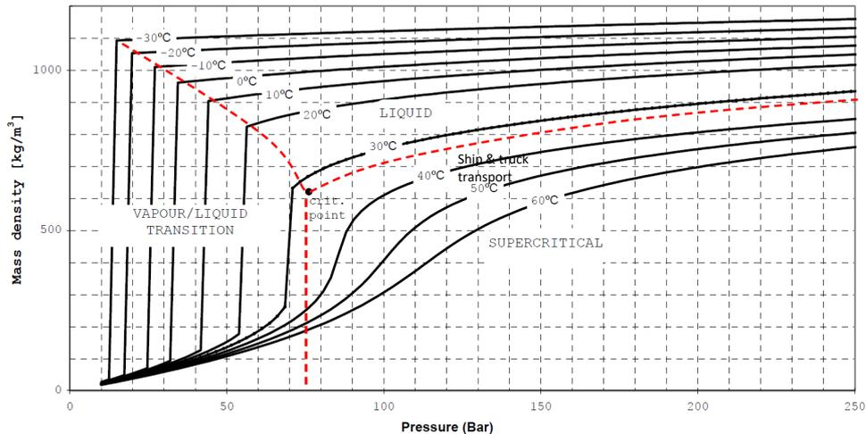
Figure 46. Mass density of pure CO<sub>2</sub> as function of pressure based on Peng-Robinson EQS. Source: DNV-GL RP-J202.
