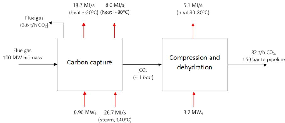
Figure 9. Illustration of energy balance for a CO<sub>2</sub> capture and compression plant treating all flue gas from a 100 MW<sub>th</sub> biomass boiler that is equipped with flue gas condensation. 90% of the CO<sub>2</sub> in the flue gas is captured corresponding to 32 t CO<sub>2</sub> output per hour. Black arrows: Mass streams. Red arrows: Energy streams.
