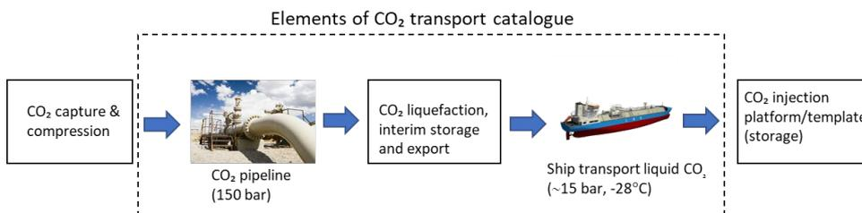
Figure 54. CO<sub>2</sub> transport by pipeline followed by liquefaction interim storage and ship transport.
