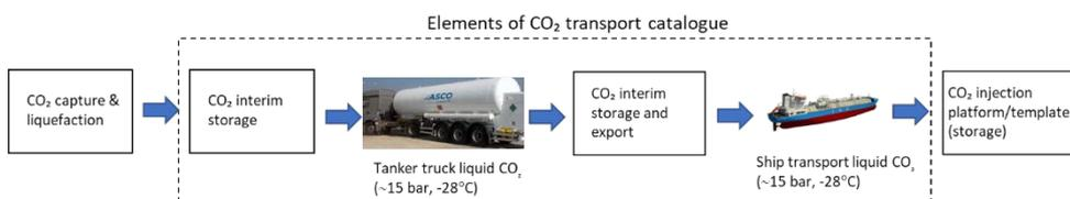
Figure 52. CO<sub>2</sub> transport by road tanker and ship to storage site/import terminal.
