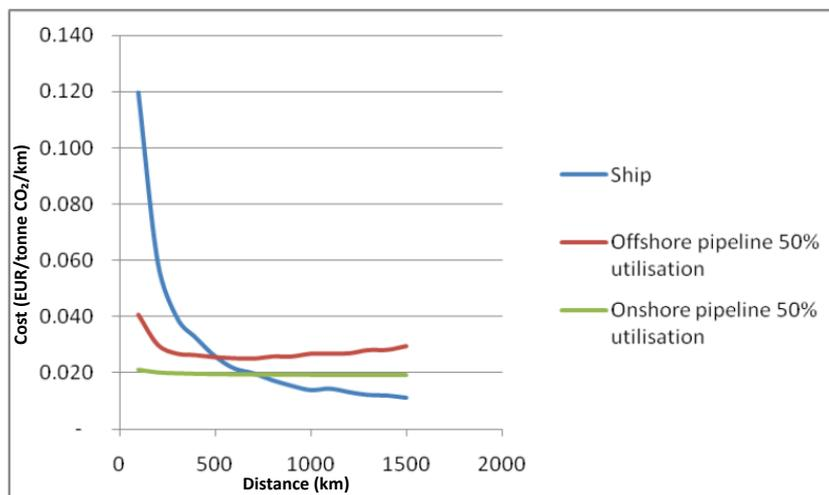
**Figure 47. Cost of CO<sub>2</sub> transport (EUR/tonne/km, 2010 cost level) by pipeline at 50% capacity and by ship at 100% capacity (including terminal) for 10 MTPA. Source: ZEP [2]**
