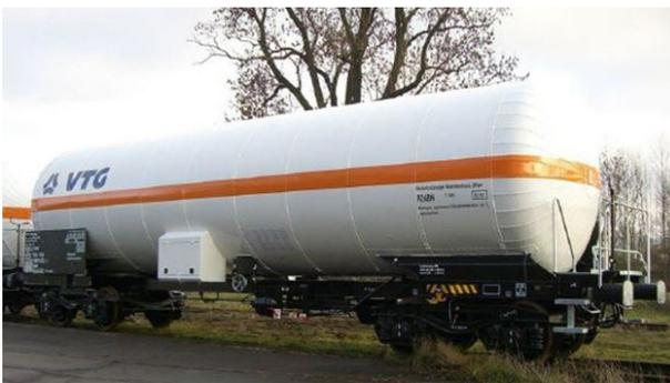
Figure 51. Railroad car for liquid CO<sub>2</sub> transport. Source: [www.VTG.com](http://www.VTG.com)
