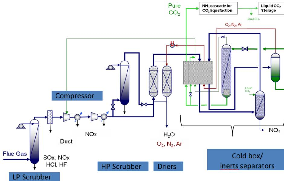
Figure 28 Upgrading of raw CO<sub>2</sub> at Callide oxy-fuel CCS. [11]
