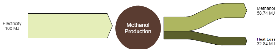
Figure 2 Methanol from Power Energy Balance
