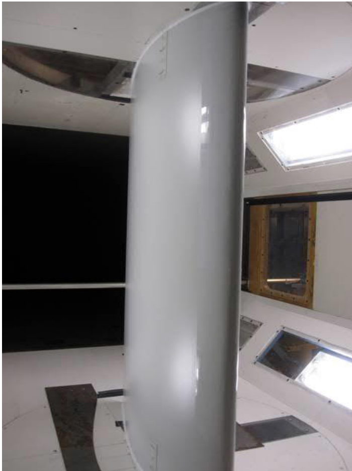
Figure 10. Wind tunnel tests on airfoil with LEP.
