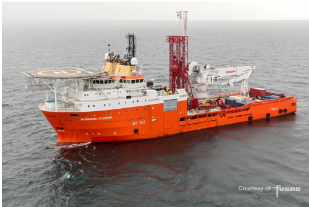
Figure 5. Typical geotechnical drillship
