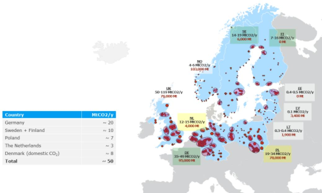
**Figure 6:** Overview of Northern European CO<sub>2</sub> point sources which could be relevant for storage in Denmark. The delineation is based on closeness to Denmark. Point sources outside of these countries could also be relevant for storage in Denmark. (Source: Study commissioned by the Danish Energy Agency, 2021)
