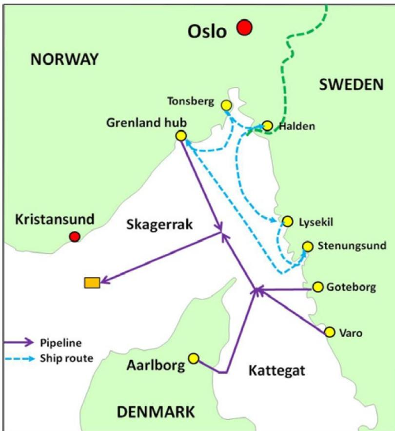
Figure 13: Possible combination of ship and pipeline transport of CO<sub>2</sub> to an offshore storage site. (Source: Haines (2015)).
