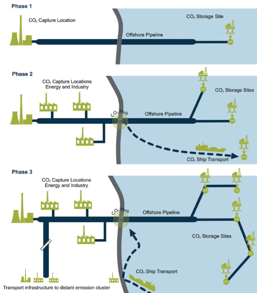
Figure 4: Schematic sketch of a stepwise CCS infrastructure development. (Source of figure: Bellona (2015), ZEP (2015)).
