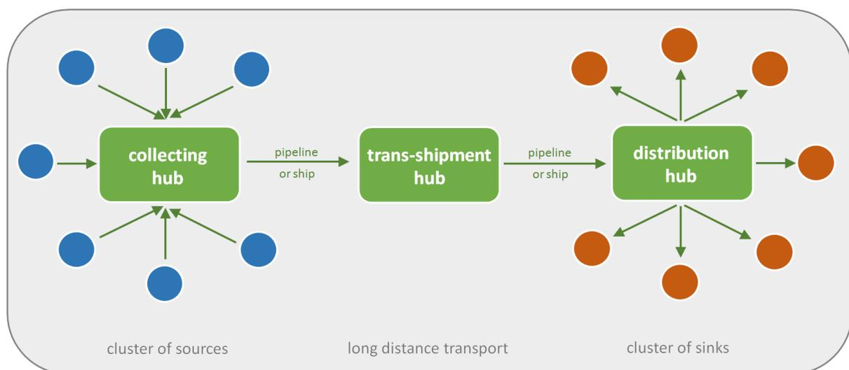
**Figure 3:** Schematic illustration of a CCS infrastructure. (Source: BGR).
