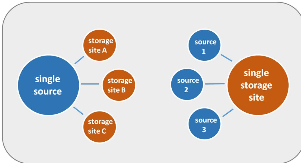
**Figure 1:** Schematic diagram illustrating CCS clusters involving a single source, e.g., large power plants in contrast to smaller industrial CO<sub>2</sub> sources. (Source: BGR).
