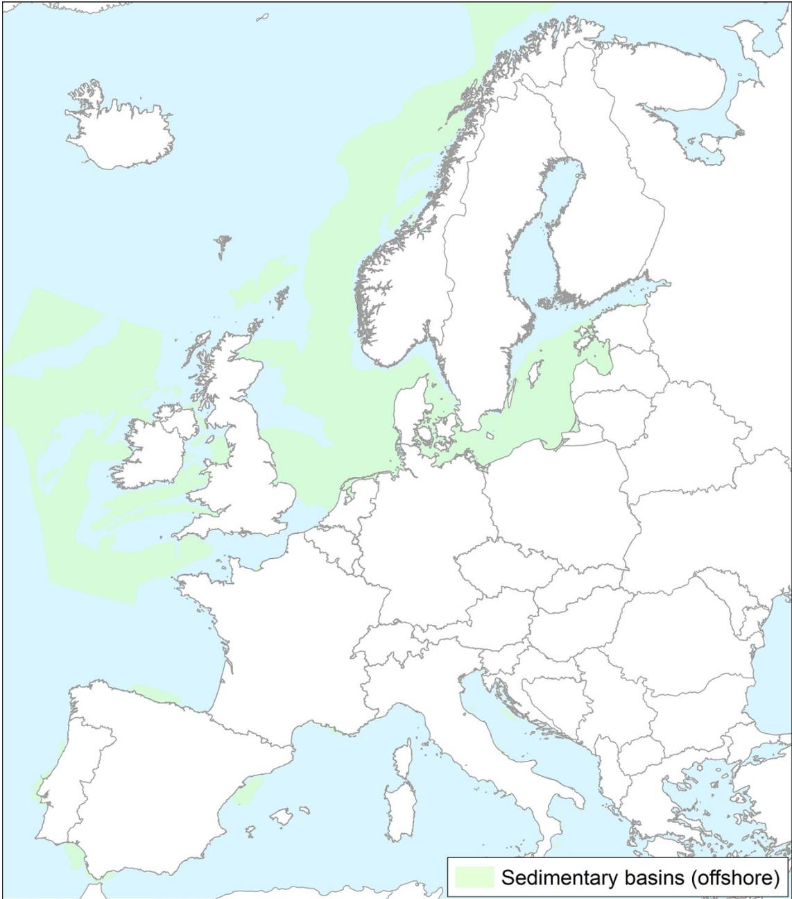
**Figure 2:** Sedimentary basins in offshore areas of Europe potentially suitable for CO<sub>2</sub> storage. Most basins are in Northern Europe. From a European infrastructure network point of view the North Sea and the Baltic Sea are of greatest interest. (Source of data: GeoCapacity, NORDICCS)
