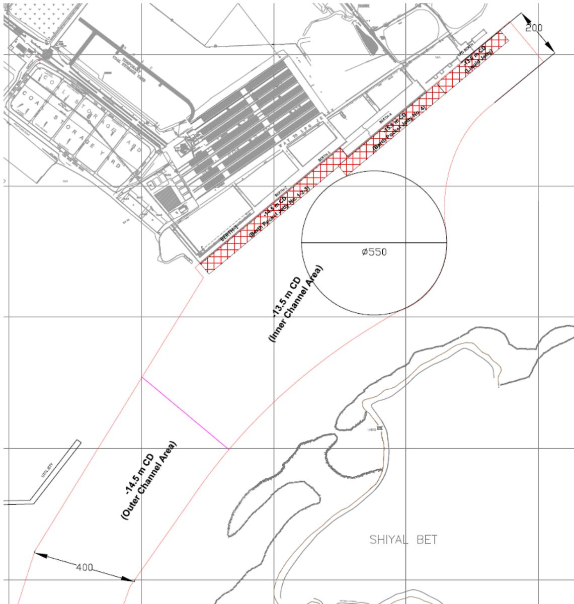
Figure 49: Pipavav Port – Approach channel and turning basin
