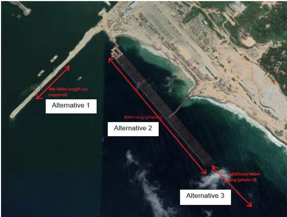
Figure 33: Vizhinjam Port – Potential alternatives for developing OW berth in Vizhinjam port.
