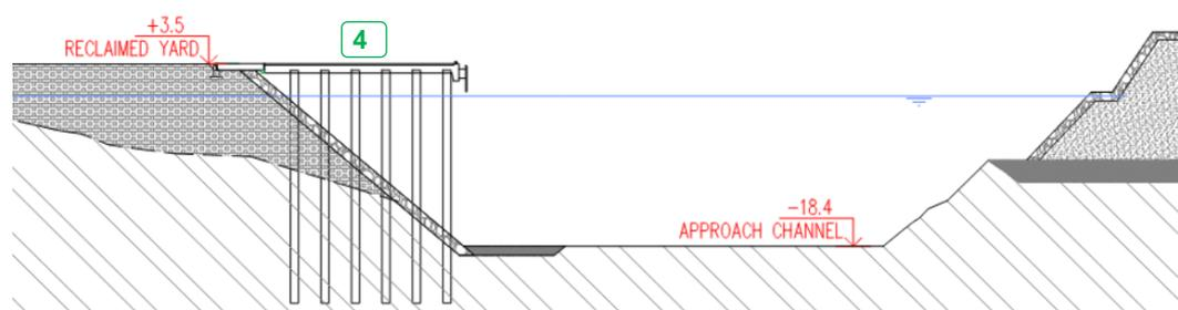
Figure 37: Vizhinjam port – Proposed sequence of works- 2
