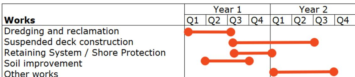
Figure 55: Pipavav Port – Indicative duration of works
