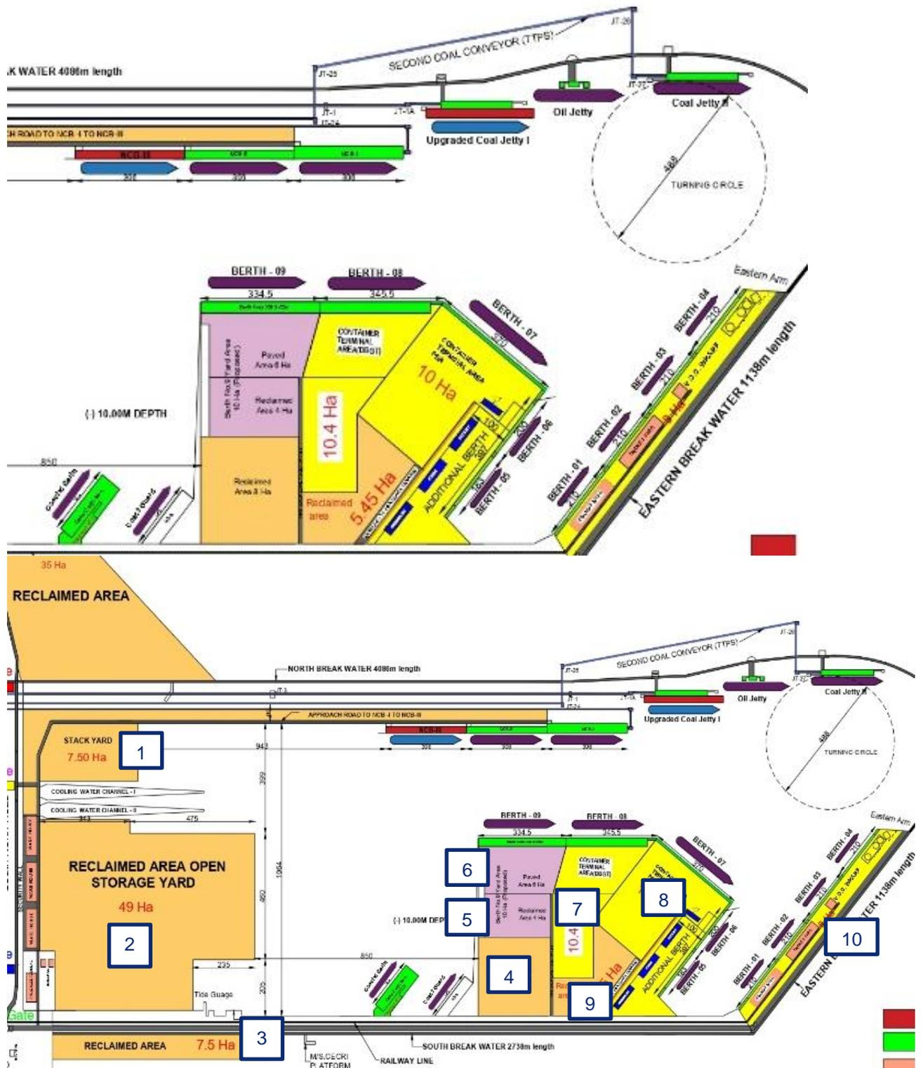
Figure 19: Tuticorin Port – Plan of existing berths and yards. Numbers given refer to yard areas as noted in Table 19.
