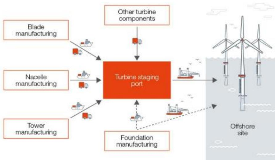
Figure 8: Typical process of sourcing and installation of components in OWF.
