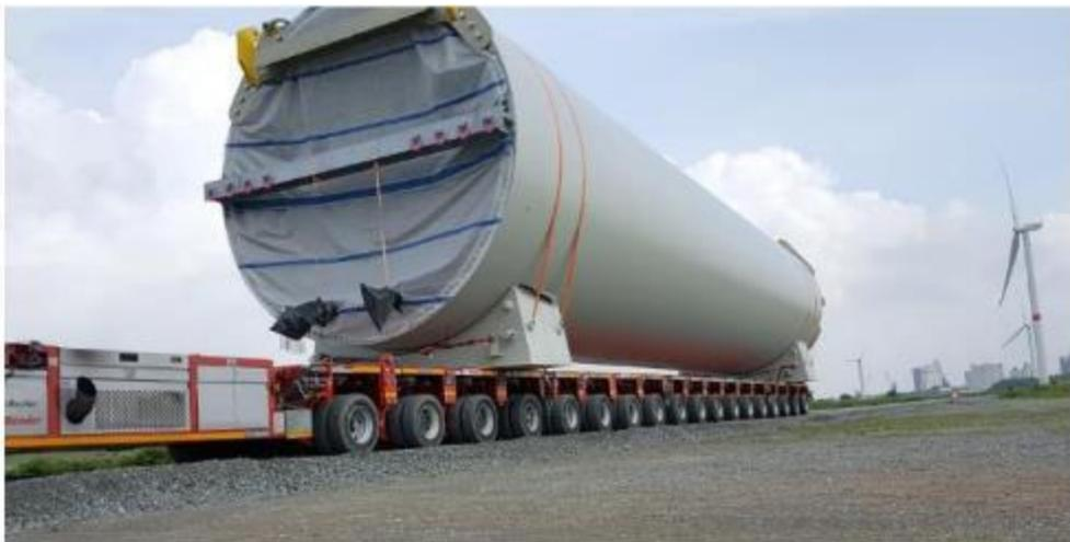
*Figure 69: SPMT for transportation of large and heavy components*
