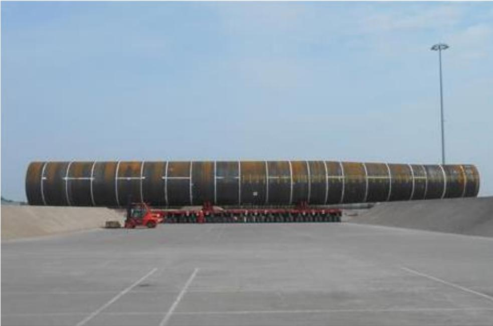
*Figure 73: Monopile stored on earth embankments*
