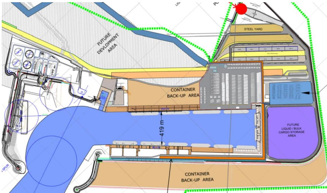
Figure 43: Hazira Port – Layout option for yards and berths to service OWF
