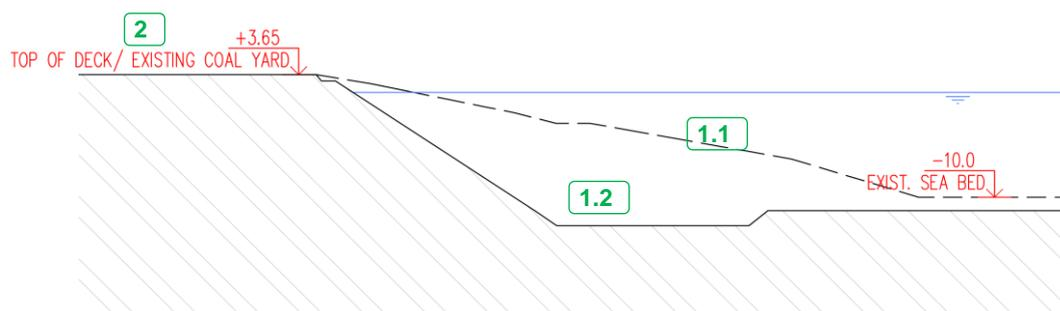
Figure 25: Tuticorin Port – Proposed sequence of works-1
