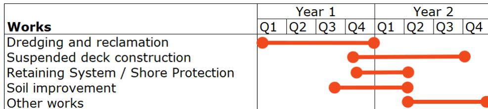
Figure 46: Hazira Port – Indicative duration of works for OW terminal development
