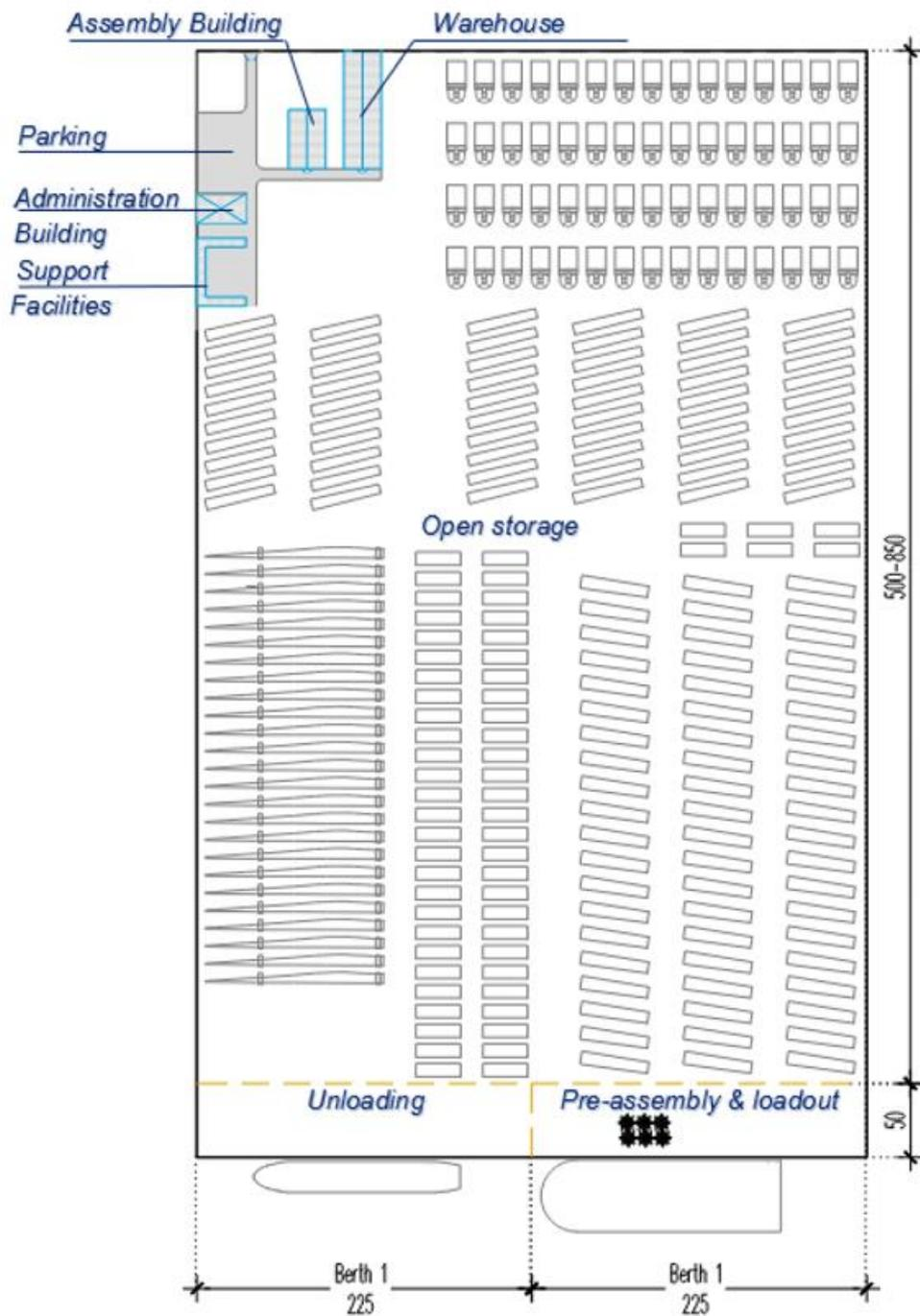
Figure 13: OW terminal – indicative masterplan. (measurements in meters)
