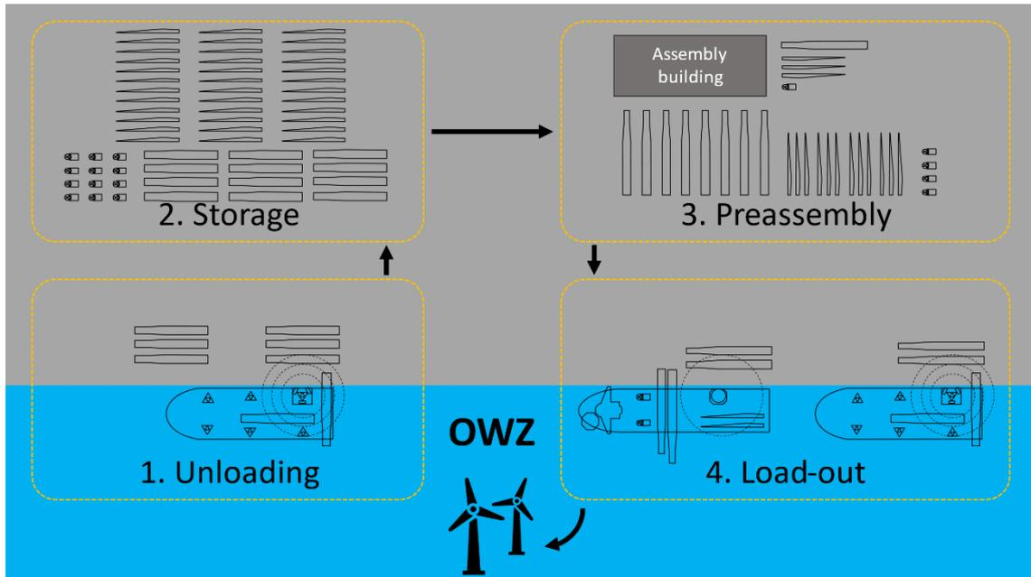
Figure 6: Diagrammatical layout for an installation port
