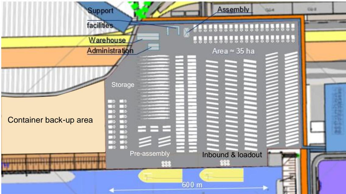
Figure 44: Hazira Port – Proposed port expansion for OWF
