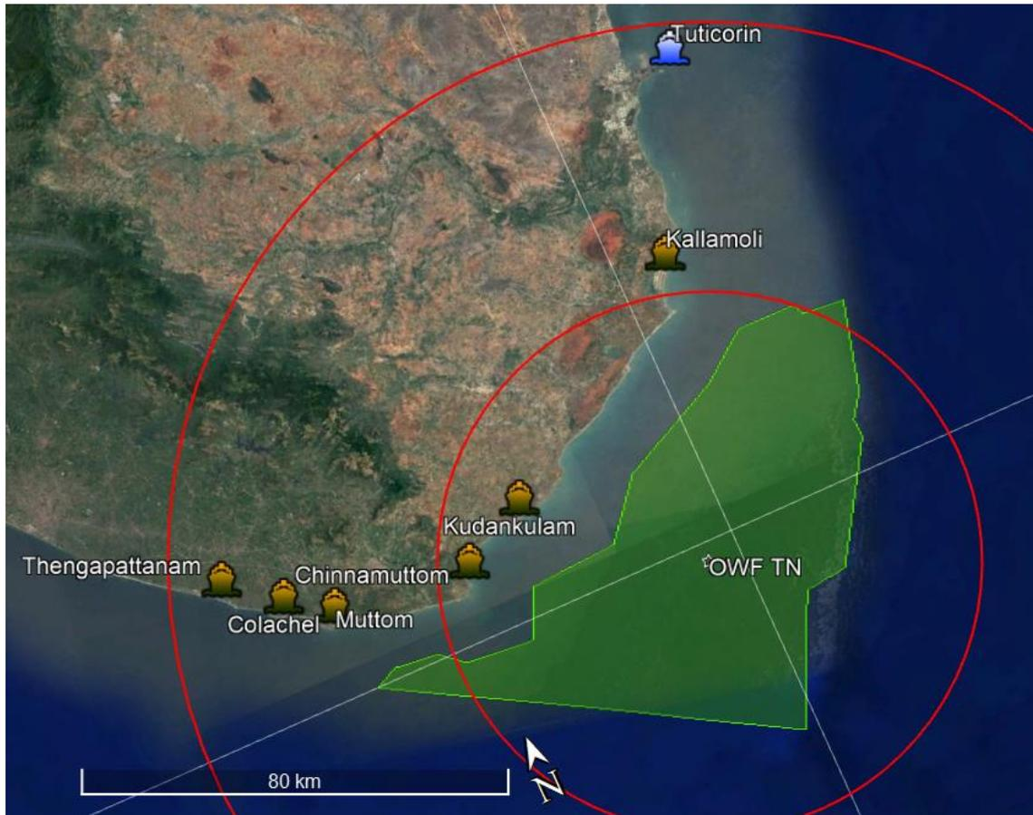
Figure 56: O&M Ports – Potential O&M bases for Tamil Nadu OWZ. Red curves denote 50km and 100km radius from OWZ central point.
