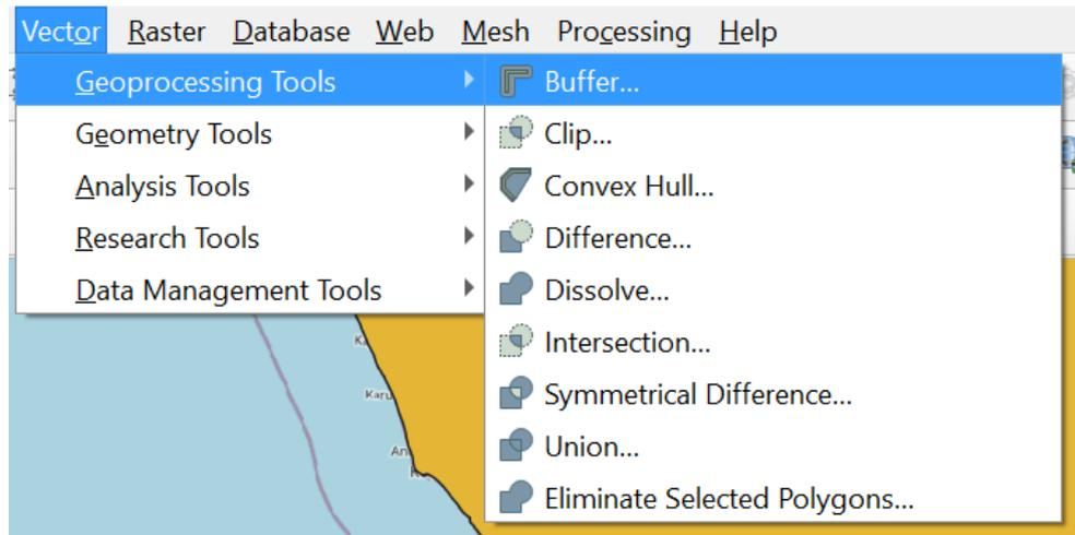
Figure 3.3: How to find the 'Buffer' geoprocessing tool
