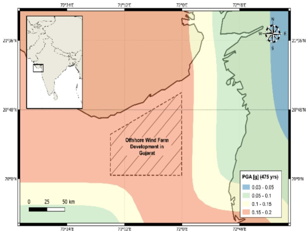
Figure 2.44 - Seismic hazard map for 475 years return period for Gujarat (Bhattacharya et al. 2021)
