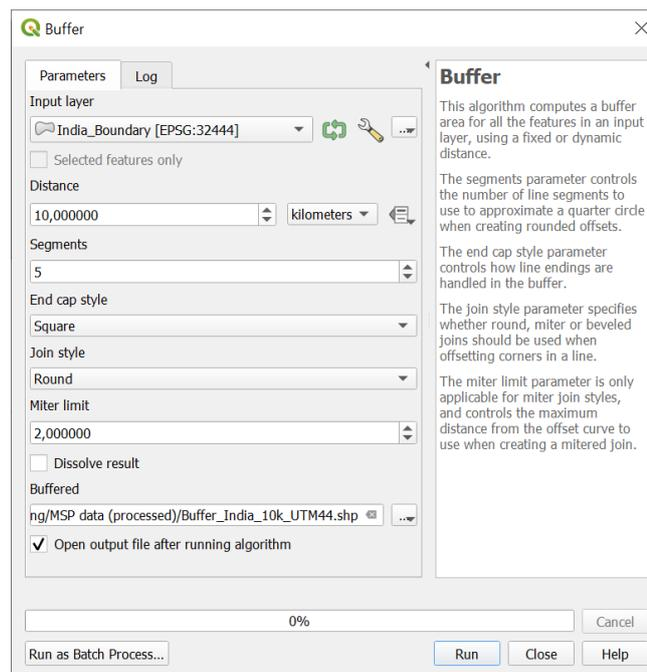
Figure 3.4: Insert parameters for the 'Buffer-tool' in QGIS
