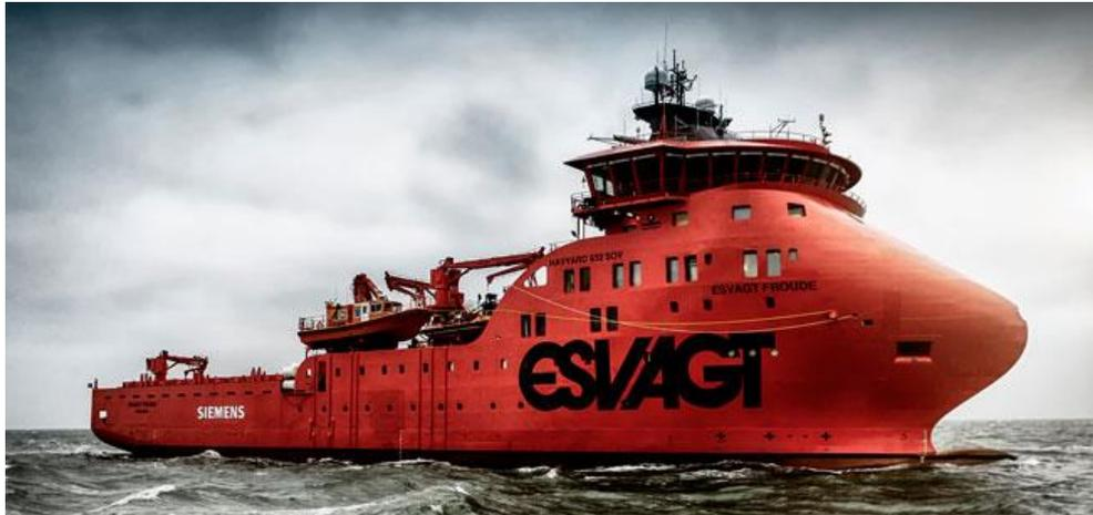
Figure 5-4 | Service Operation Vessel used by Siemens for servicing offshore wind farms
