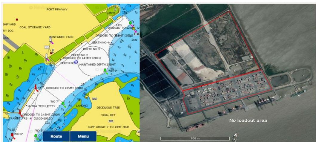
Figure 2.46 - Pipavav Port water depth and satellite photo zones (COWI, 2022)
