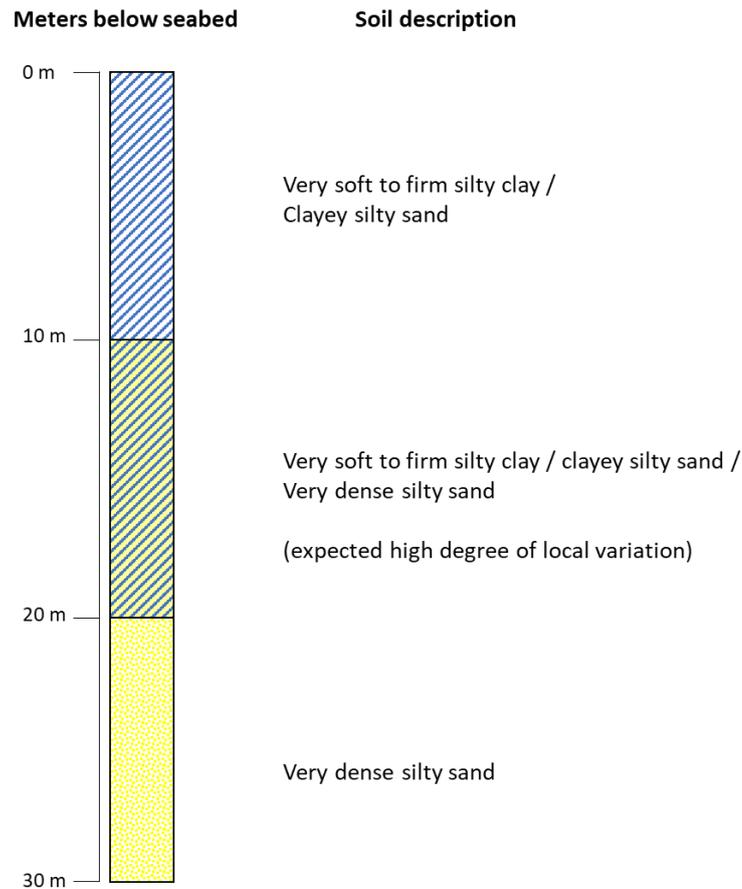
*Figure 2.41 - Illustration of stratigraphic profile of what might be expected within parts of the Zone A and C. Note this is a general illustration which cannot be used to plan for foundations, as there will be local variations that are not known at this stage.*
