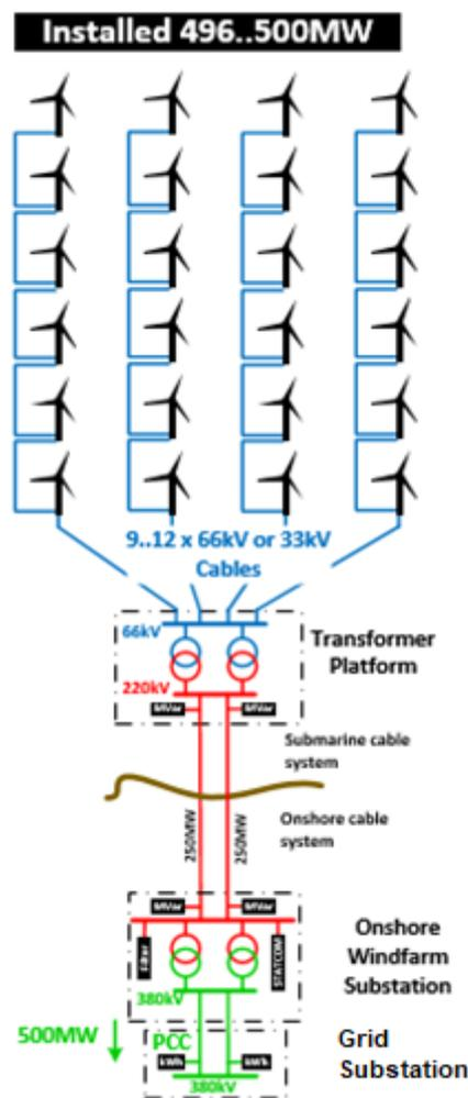
Figure 4-1 | Typical Transmission System with Offshore Substation (COWI, 2021)
