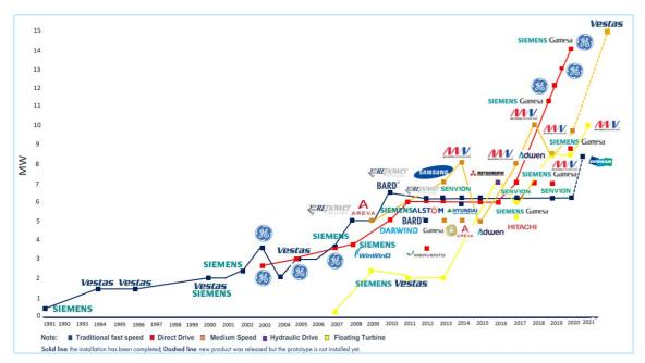
Figure 4 Offshore Wind Turbine Technology Road (excluding China) Source: (GWEC, 2021)
