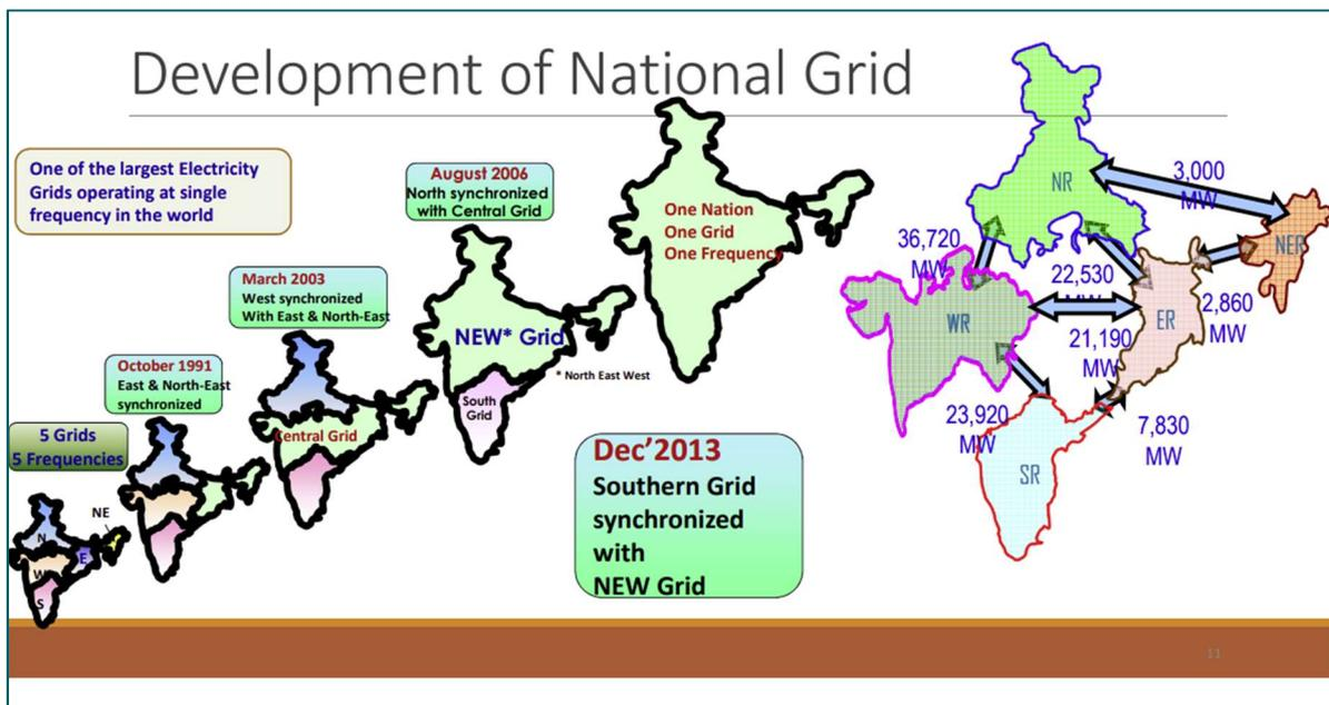
Figure 23 : Development of synchronization into one national grid. Source: [18]
