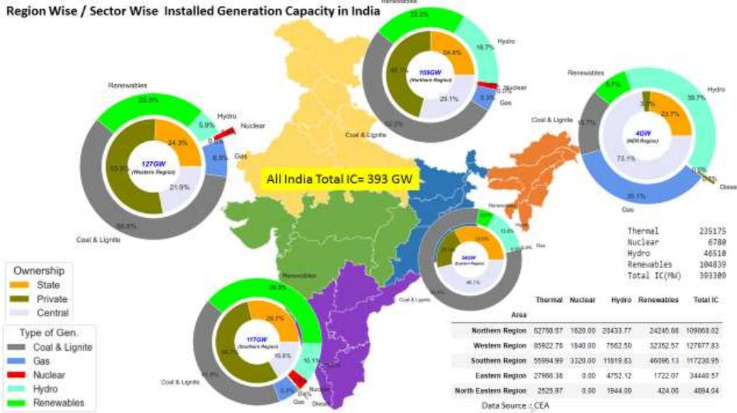
Figure 20: Regional Installed Generation Capacity 2021 - Resource wise and Sector wise [18]
