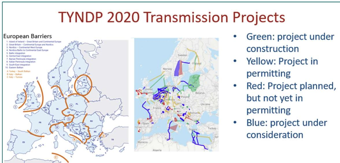
Figure 10: TYNDP 2020 transmission projects and European transmission barriers. Source [11]:
