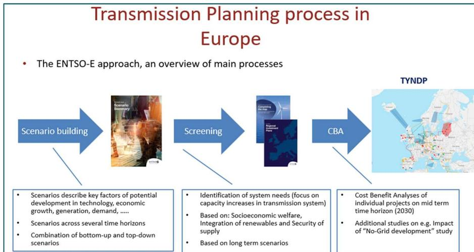
Figure 7: ENTSO-E TYNDP planning process. Source: [12]
