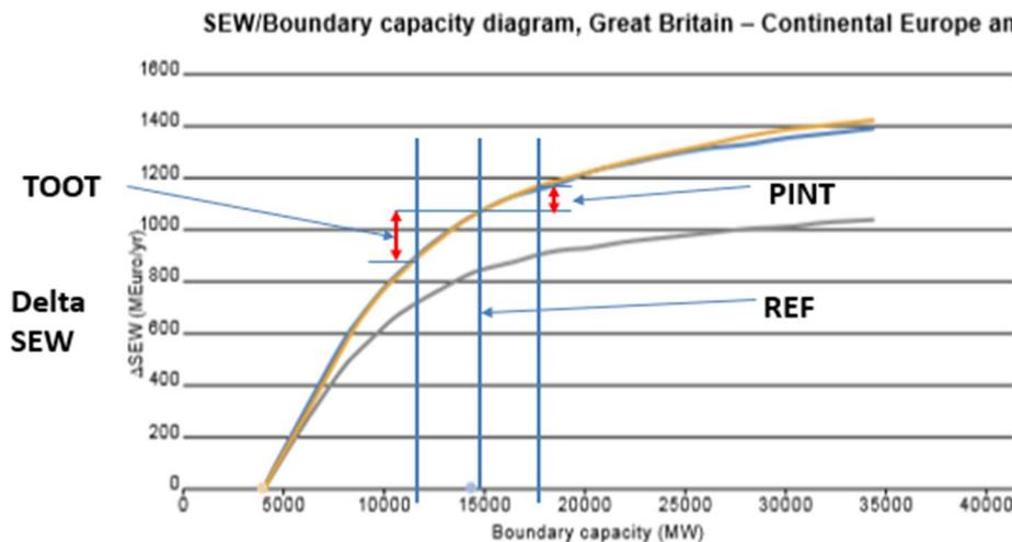
Figure 14: Illustration of economic assessment of capacity expansion according to TOOT and PINT. Source: [11]
