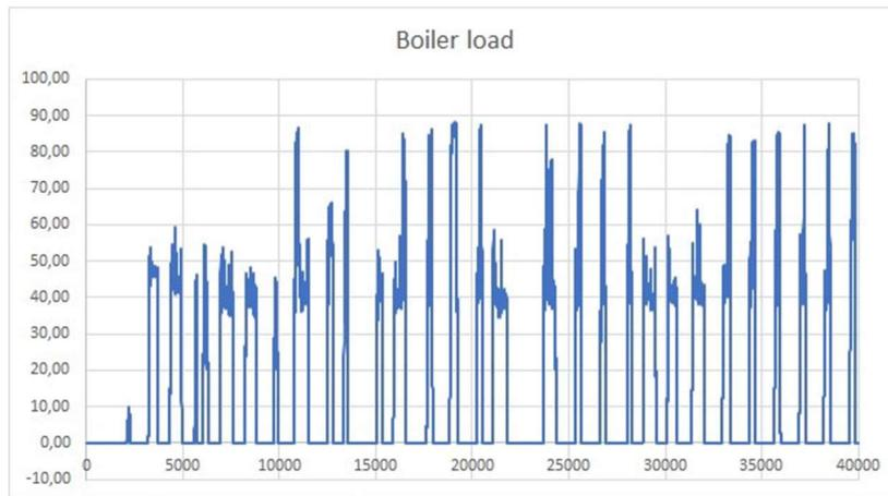
Figure 59. Boiler load one month, 7 min. values.
