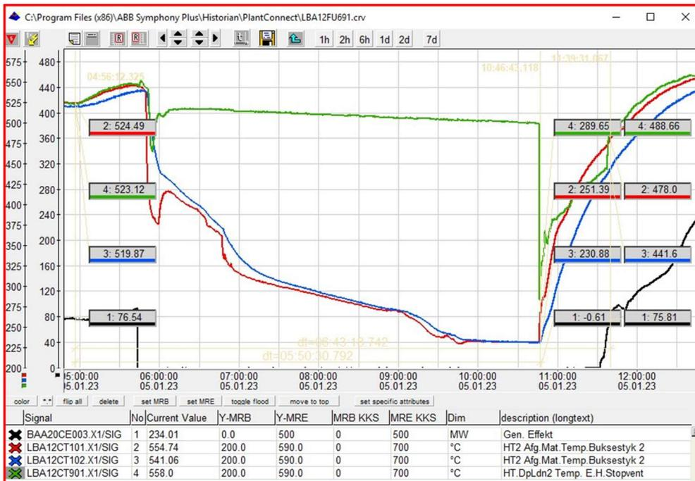
*Figure 115. Boiler and turbine trip 5/1, Material- and steam temperatures LBA12.*
