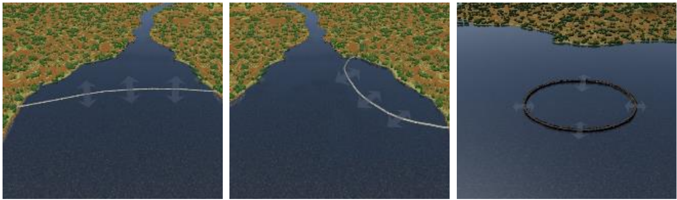
(a) (b) (c) Tidal impoundment types: (a) Tidal barrage (b) Bounded tidal lagoon (c) Offshore tidal lagoon (ref. 2)
