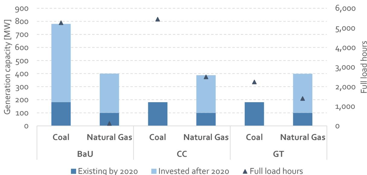
Figure 25: Installed coal and natural gas capacity in 2030, shown as existing capacity (installed before or by 2020) and additional invested capacity after 2020 as well as the corresponding full load hours.
