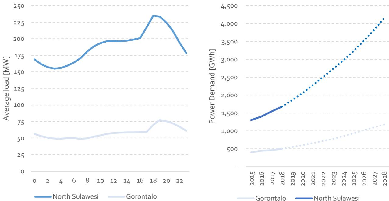
Figure 3: Load profile for 2017 and total demand including projection to 2028 [1].
