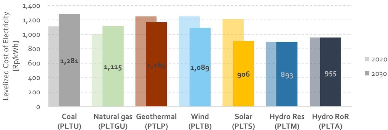
Figure: LCoE comparison for relevant power sources in Sulutgo in 2030 and comparison to 2020.
