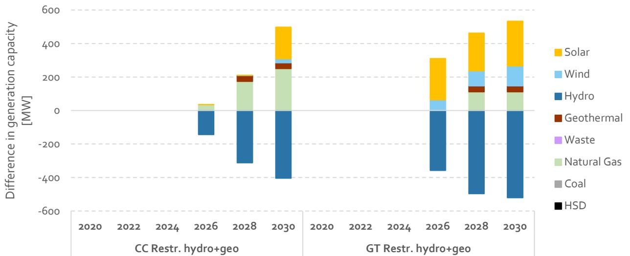
Figure 27: Differences in power capacity development between the sensitivity analyses and the respective main scenarios.
