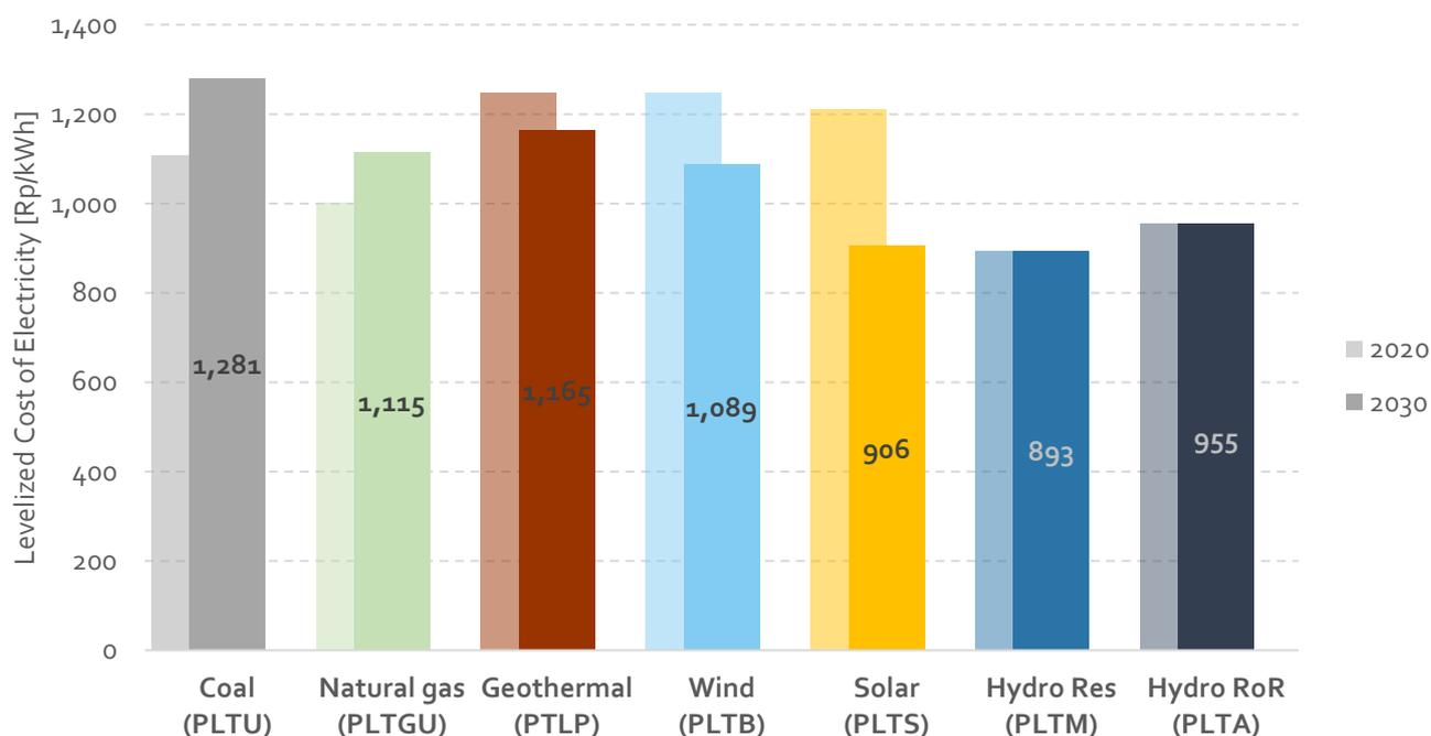
Figure 23: LCoE comparison for relevant power sources in Sulutgo in 2030 (solid) compared to 2020 (light)<sup>9</sup>. Numbers indicated represent 2030 LCoE.
