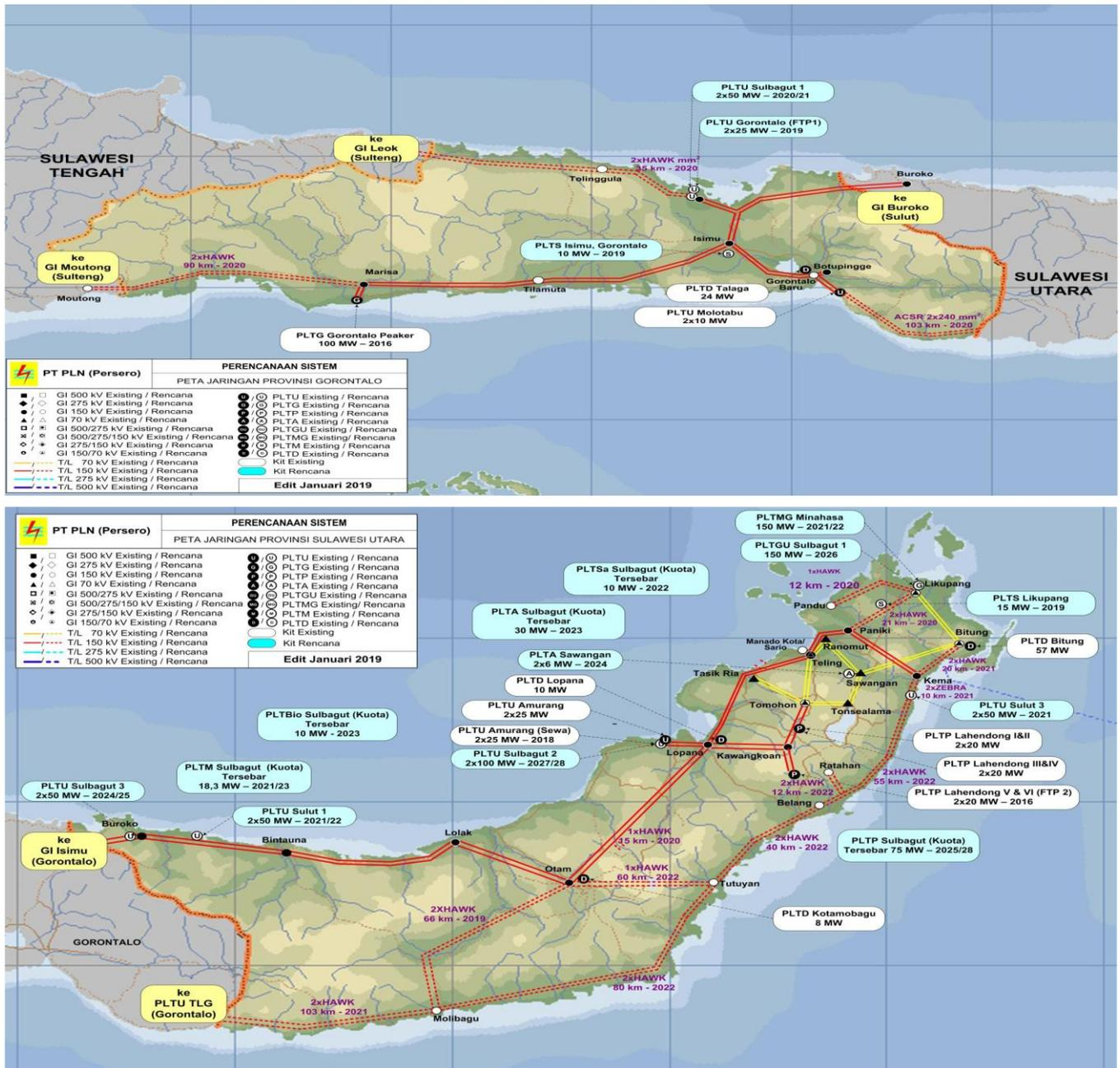
Figure 2: Overview of PLN Sulutgo system, including existing and planned generator. Source: (PT PLN Persero 2019)
