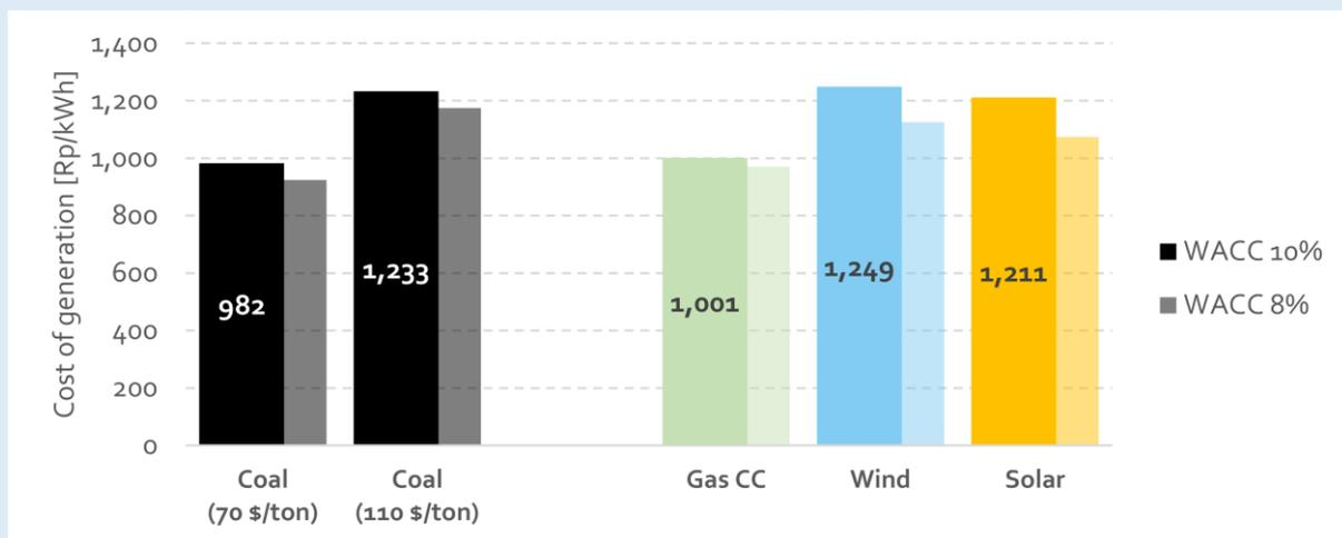
Figure 30: Generation cost of coal at 70\$/ton vs 110 \$/ton and comparison with other sources at 8 and 10% WACC.
