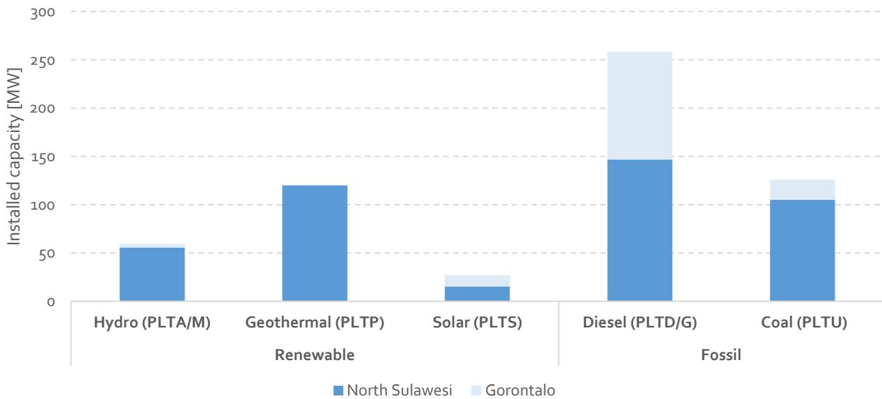
Figure 5: Installed capacity in Gorontalo and North Sulawesi, by fuel type.
