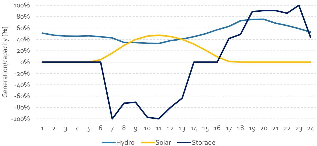
Figure 34: Generation (and charging) of hydro, solar and storage on an average day in 2030 in the GT scenario.
