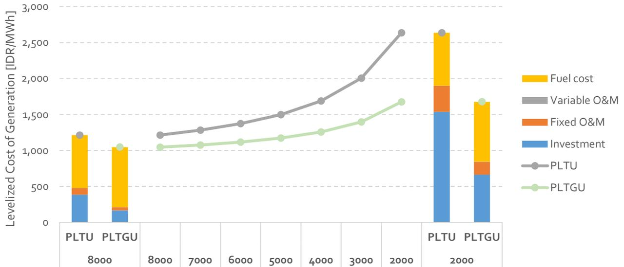
Figure 26: LCoE of coal and natural gas at different full load hours. Cost components shown at full load hours of 8,000 and 2,000.
