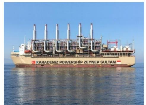
Figure 4: 120 MW mobile power plant currently stationed in Amurang.
