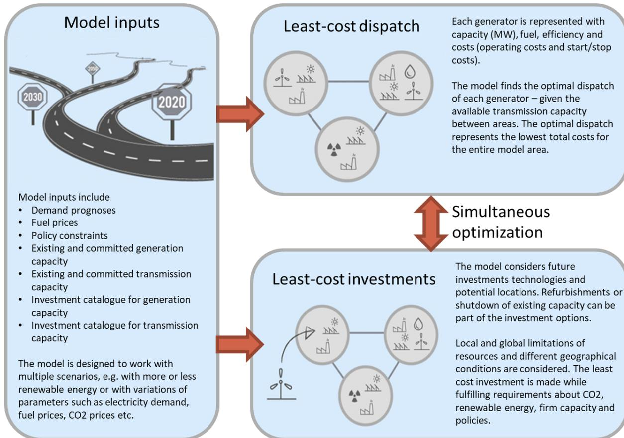
Figure 4.1: Balmore model inputs and optimization logic.
