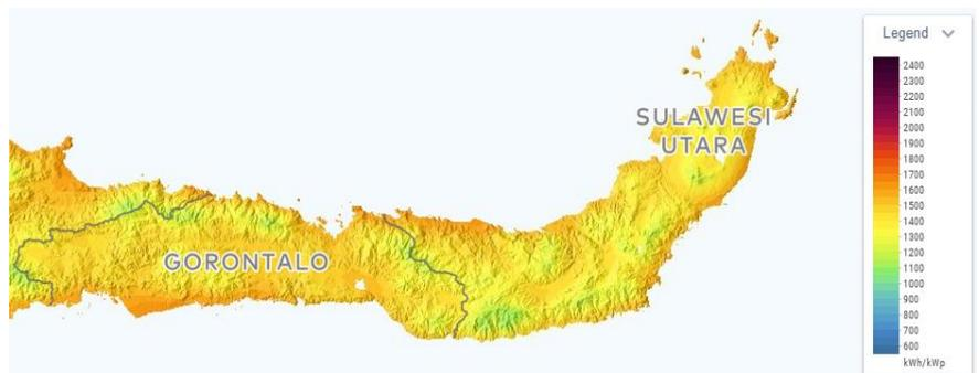
Figure 10: FLH in the area in kWh/kW based on (Global Solar Atlas 2019).
