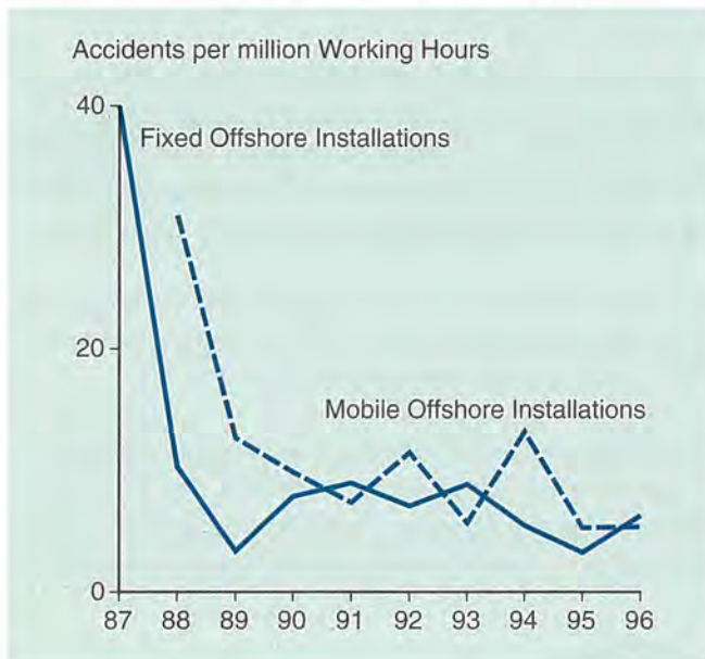
Fig. 7.1 Accident Frequency on Offshore Installations
