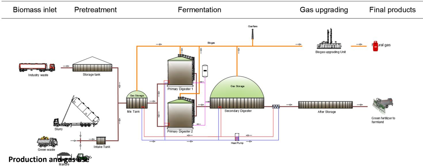
The plant uses slurry and manure from pig, cattle, mink and poultry farms. In addition it uses energy crops and agricultural and industrial residues. The majority of the slurry is pumped to the plant from farms up to 5 km away through buried pipes. In addition the plant receives trucks with biomass.
