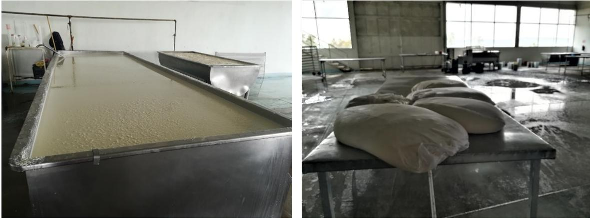
**Figure 34. “Quesera Jalpa” facilities: a) Pipe transporting mil into the factory, b) Fermentation and coagulation tank (4 000L) for cheese production, c) Dewatering of cheese curd.**
