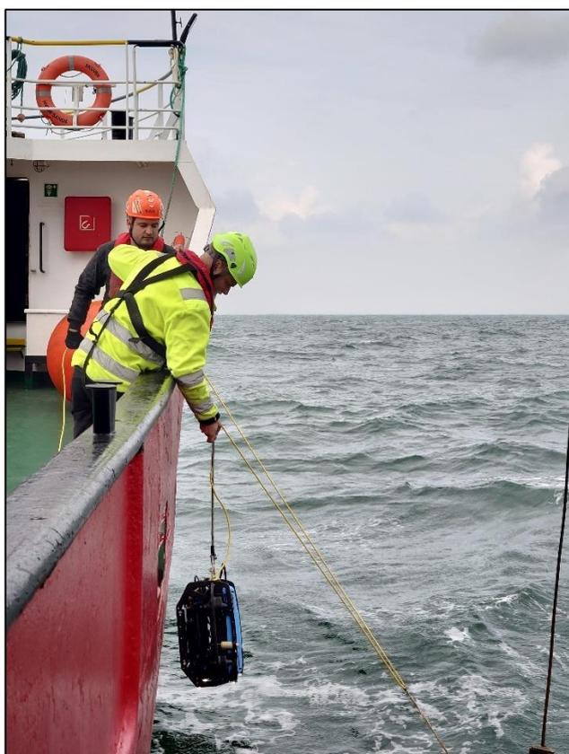
Figure 3-10. ROV (remotely operated vehicle) being pulled out of the water.
