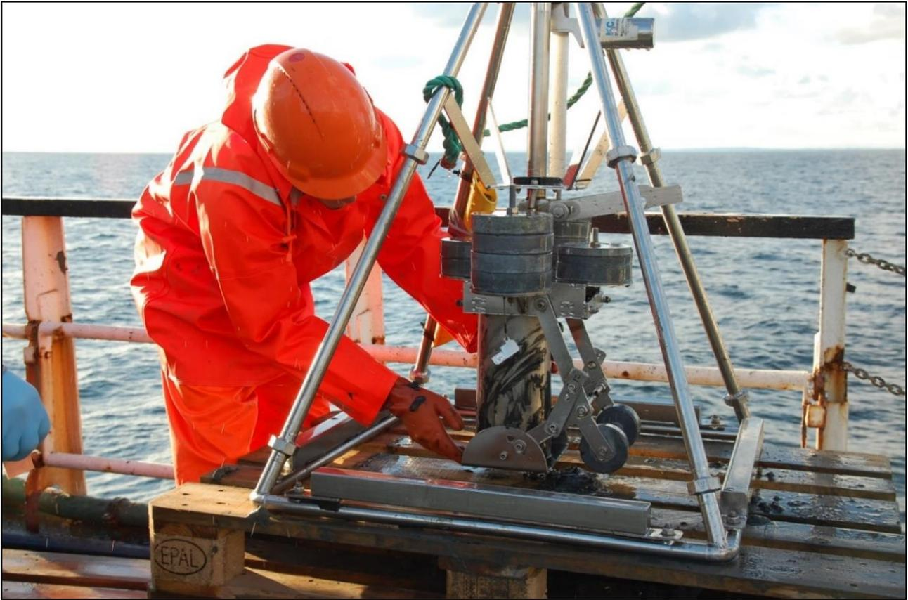
**Figure 3-11. HAPS core sampler on deck before deployment.**
