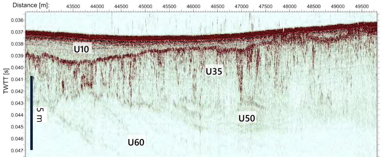
Figure 3.4: Example of SBP data quality with multiple units. Line EAAA003P1
