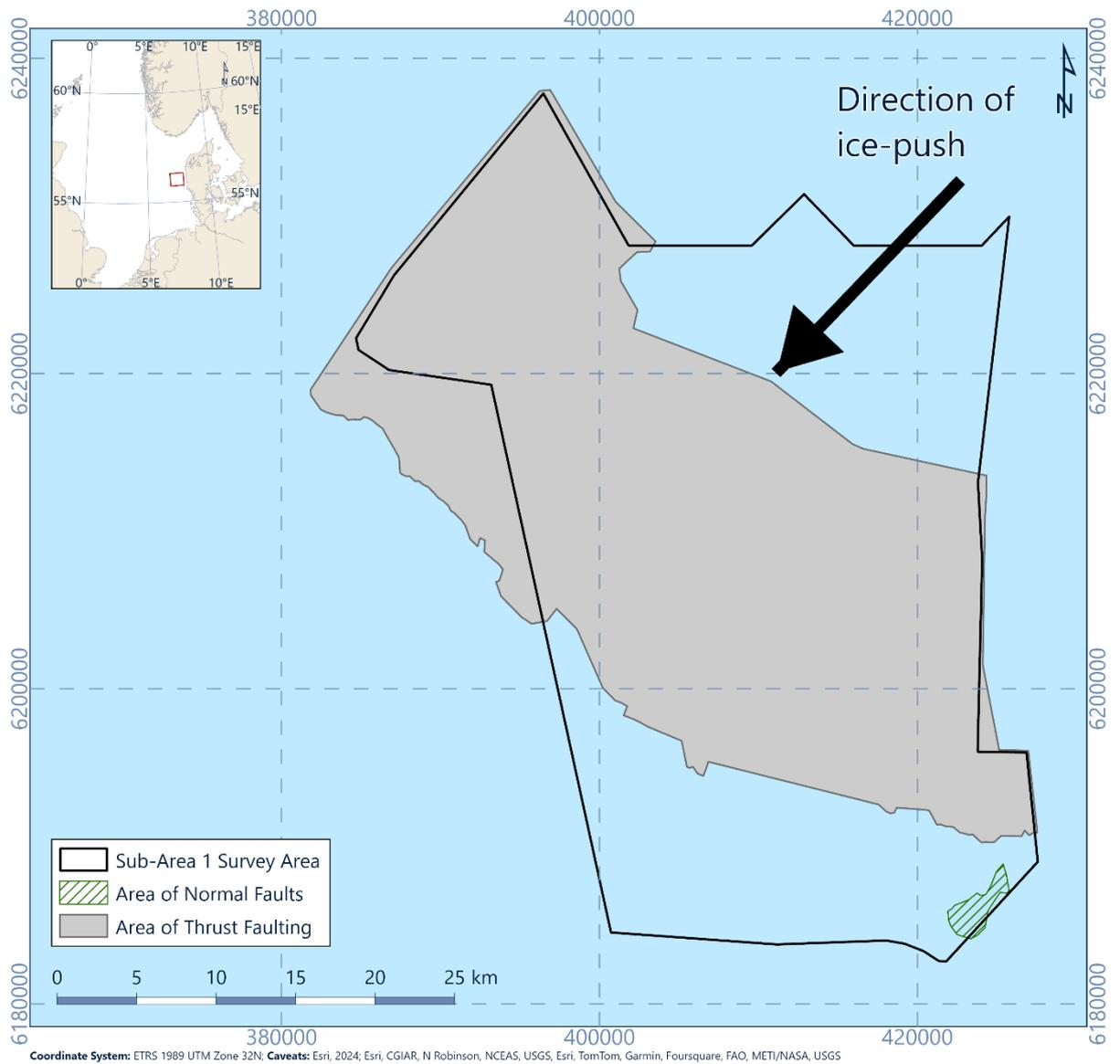
Figure 6.71: Map of the extent of glacial deformation (thrust faults) and area with normal faults in the BSU
