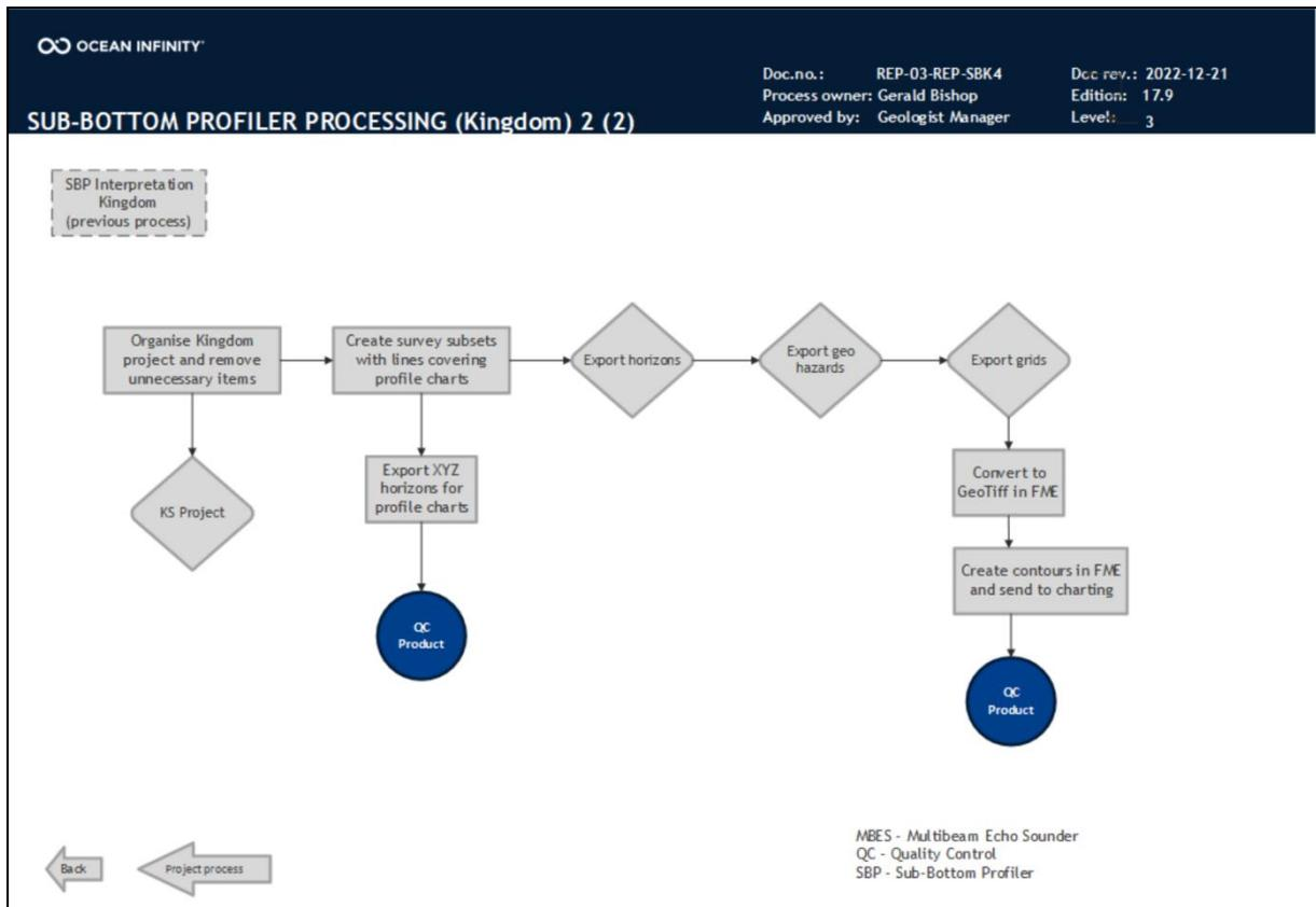
Figure 14 Workflow SBP processing (2/2).
