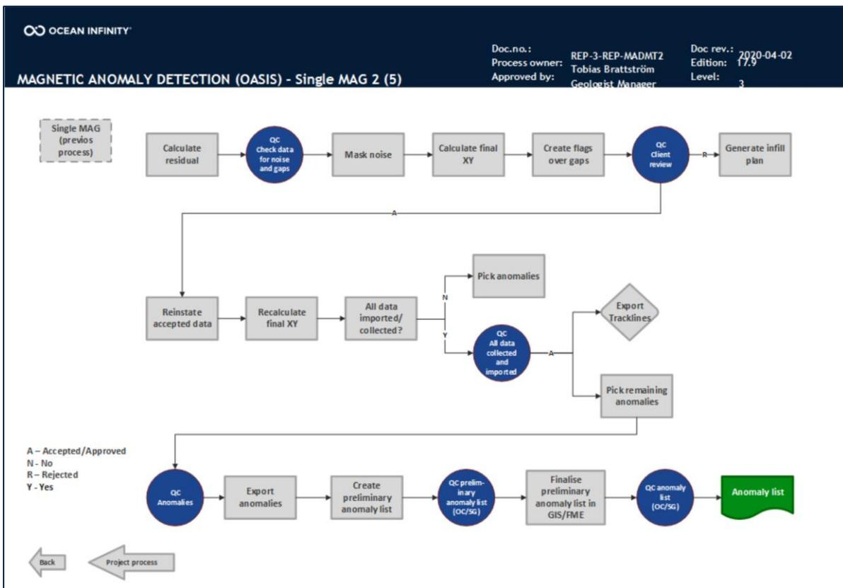
Figure 18 Workflow MAG processing.
