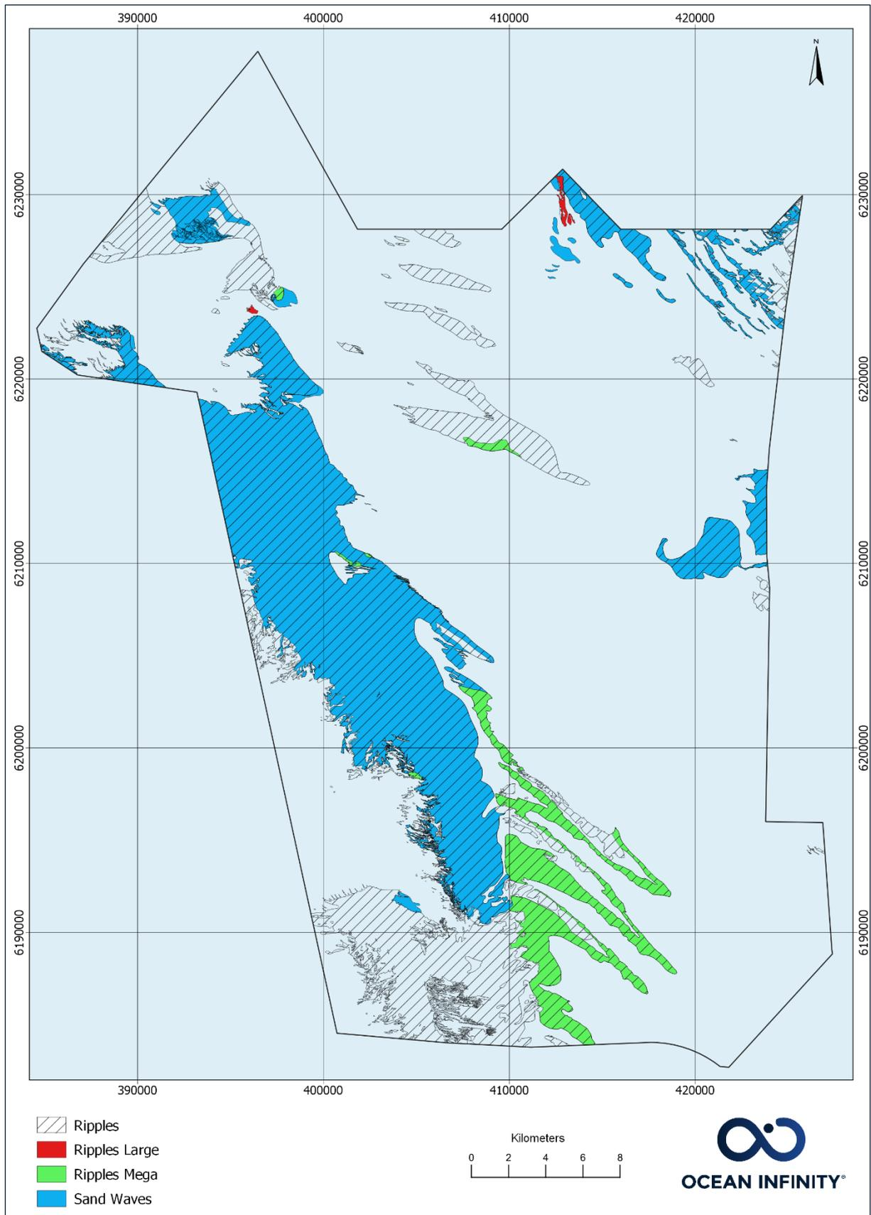
Figure 89 Distribution of Ripples, Large Ripples, Megaripples and Sand Waves in the NSA1 survey area.
