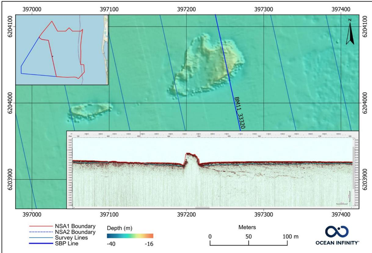
Figure 71 Till outcrop in block BM11 (MBES image above with SBP insert).
