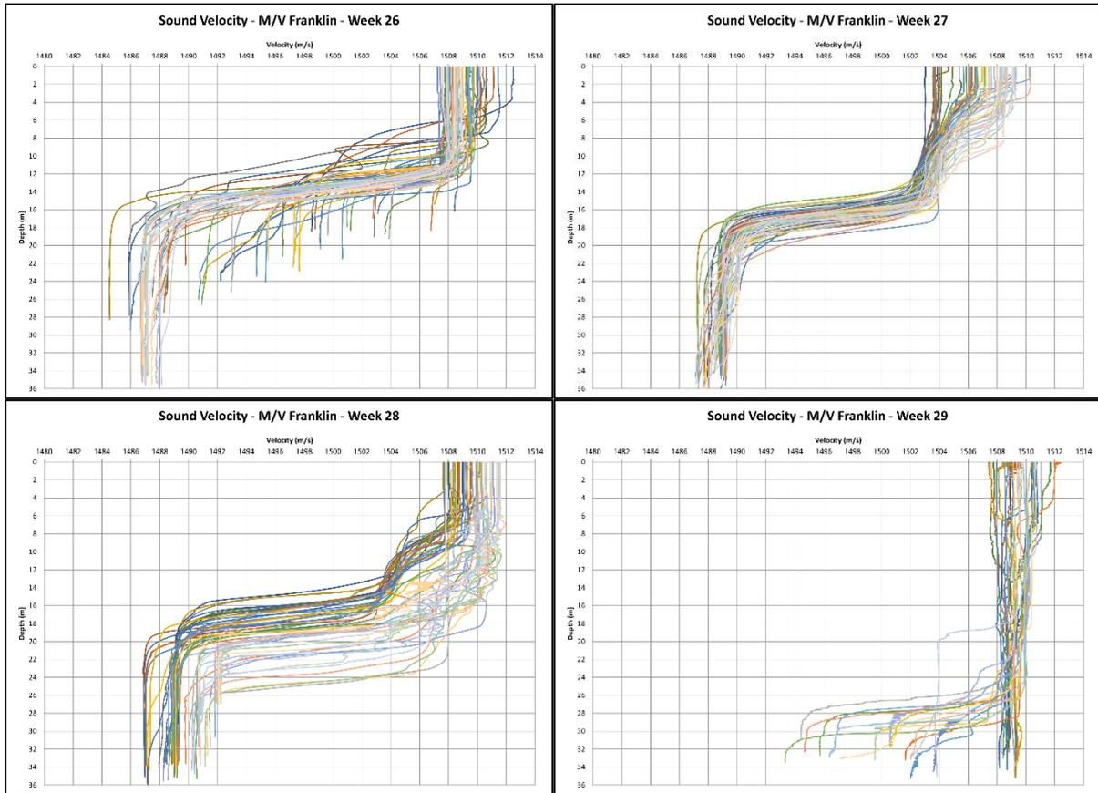
Figure 26 M/V Franklin Sound Velocity Profiles – Weeks 22 to 29.
