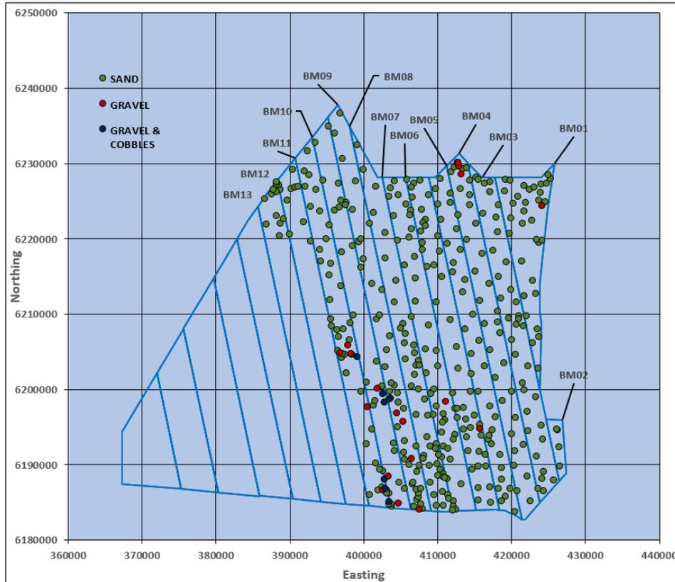
Figure 160 Distribution of SAND, GRAVEL and GRAVEL & COBBLES within NSA1.
