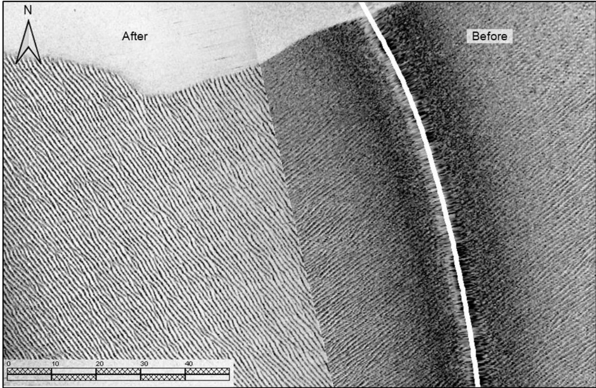
Figure 90 Example of different bedform size and direction before and after weather stand-by on BM11.
