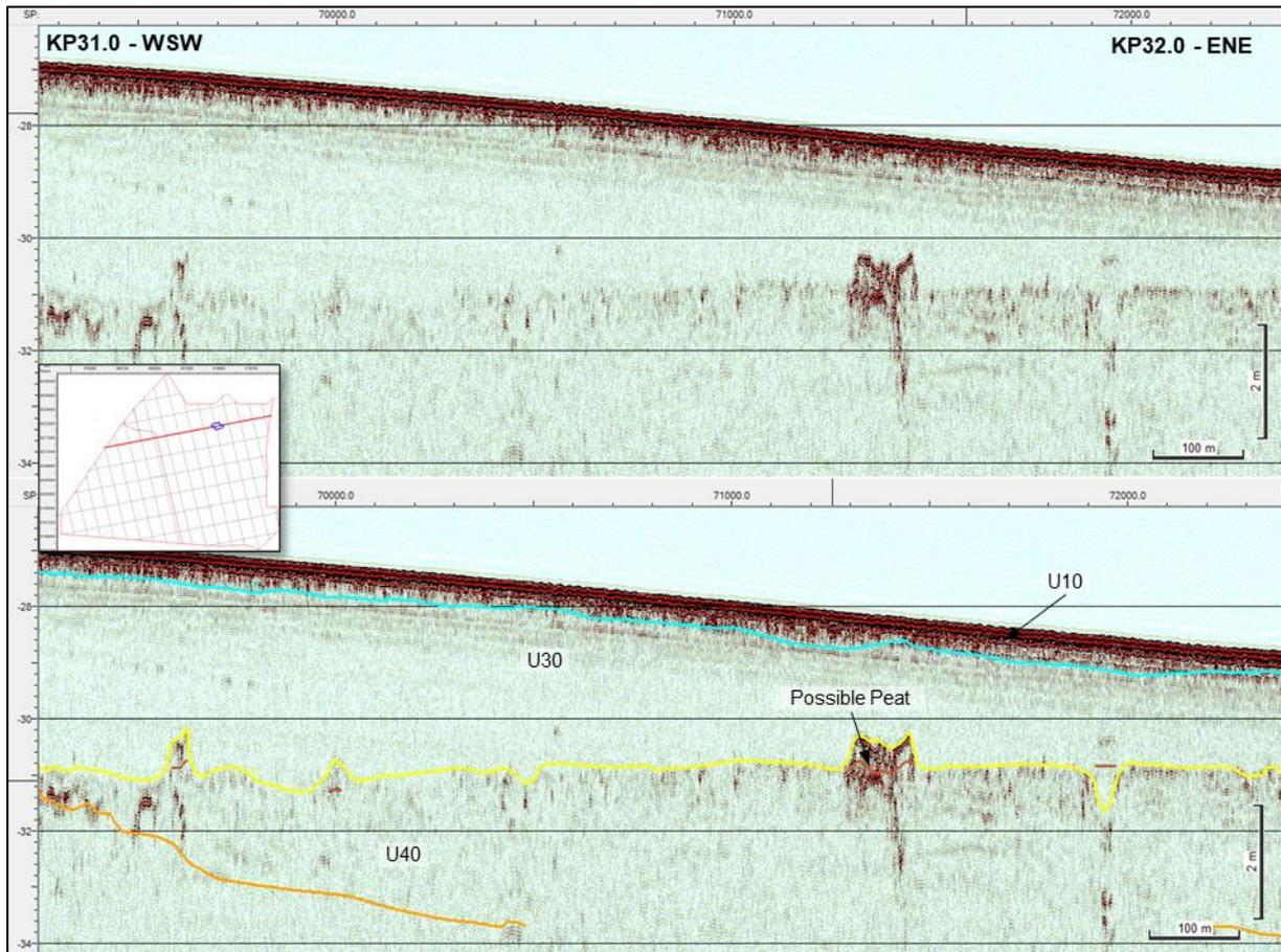
Figure 146 SBP example image of possible peat. Survey line BX01\_15000, position 410281E, 6221223N (image mid-point).
