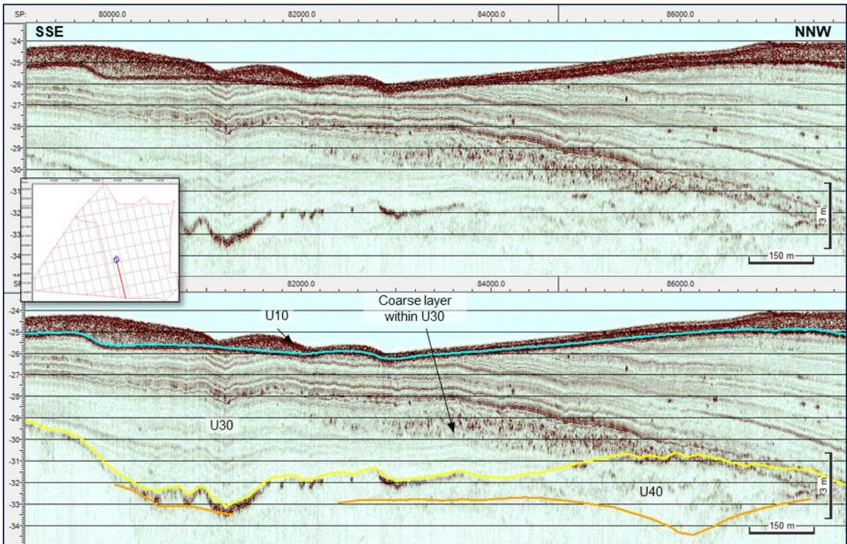
Figure 136 SBP example images of coarser layer within Unit 30. Survey line BM10\_29750, position 401354E, 6201944N (image mid-point)
