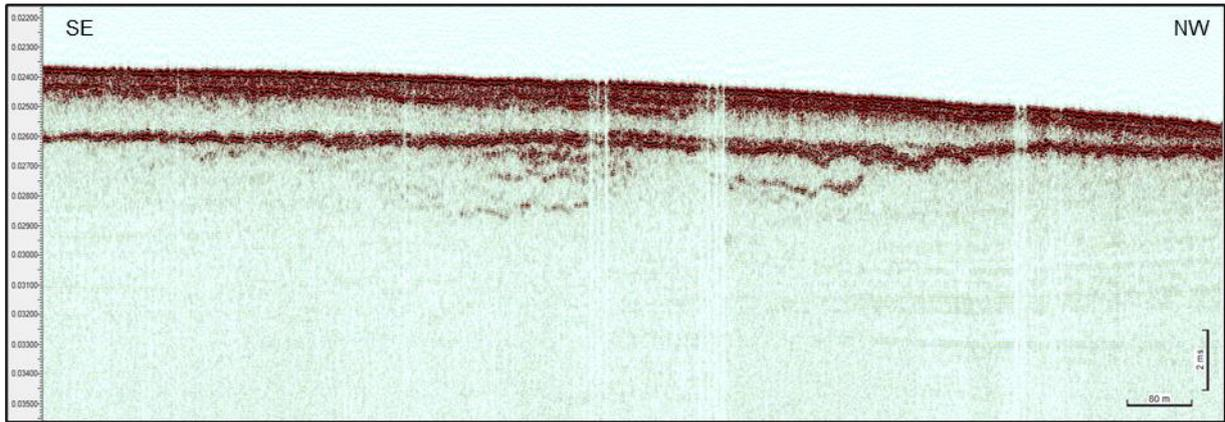
Figure 52 Processed Innomar data showing vertical striping due to weather conditions.
