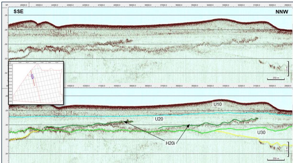
Figure 133 SBP example images of high amplitude discontinuous internal reflectors in Unit 20. Survey line BM12\_36890, position 390207E, 6219735N (image mid-point).
