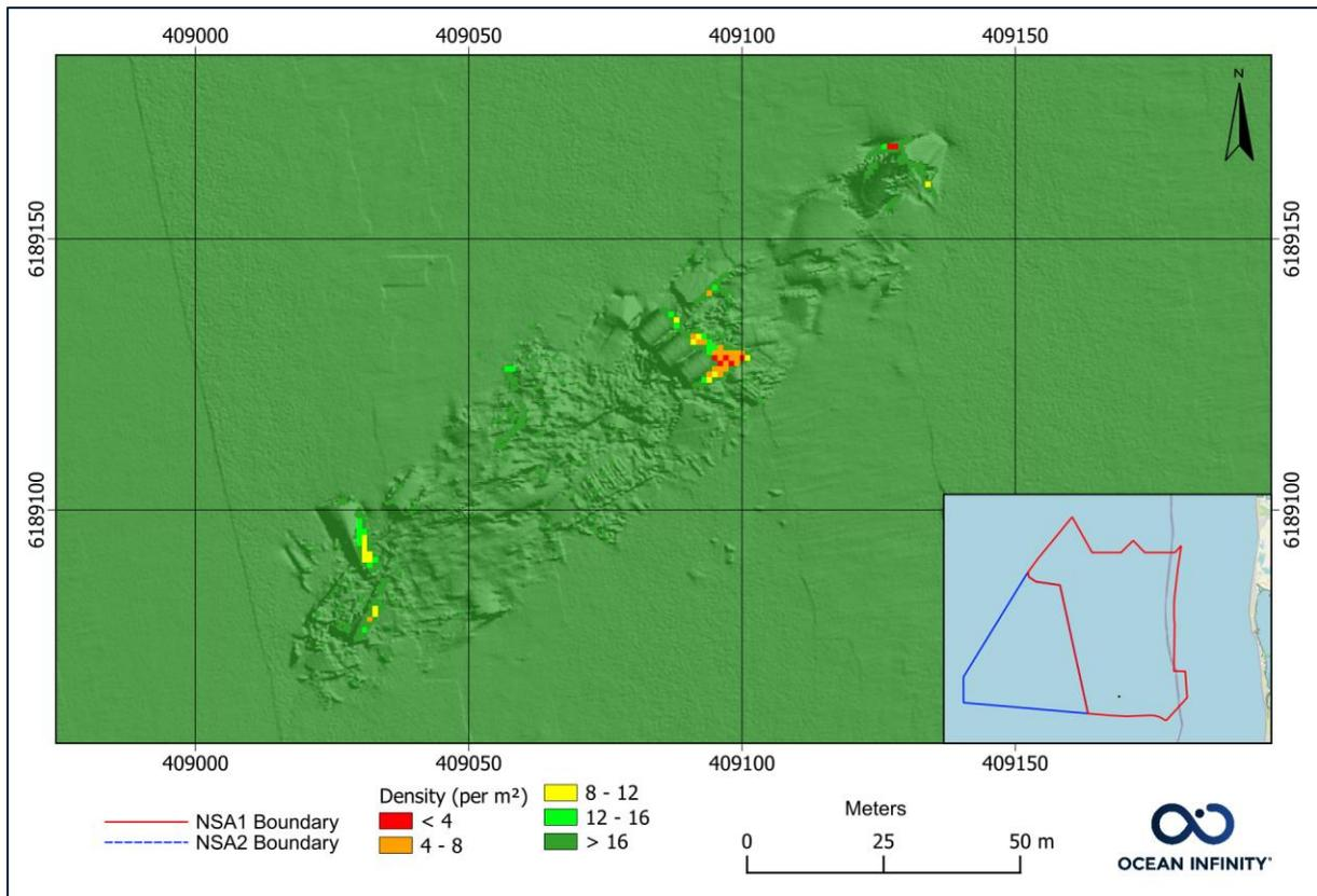
Figure 24 Low-density cells caused by feature shadowing.
