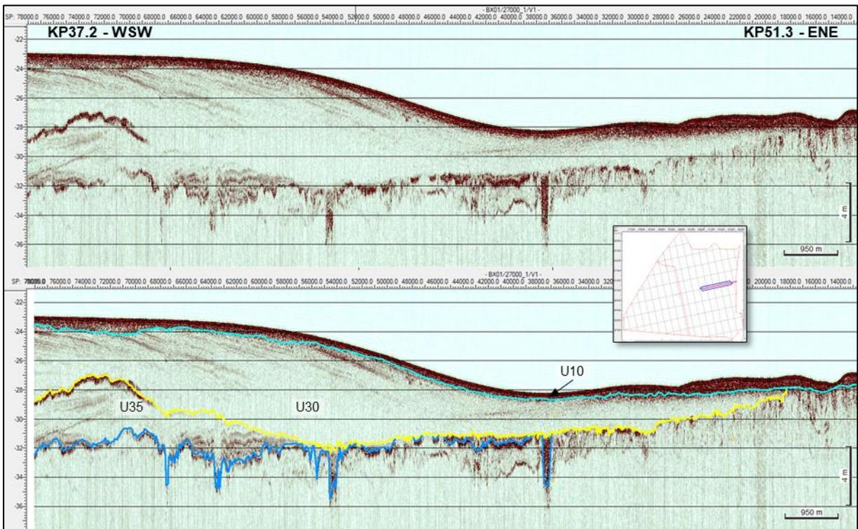
Figure 148 SBP example image of eastern part of Profile line BX01\_27000. Position 413772E, 6209693N (image mid-point).
