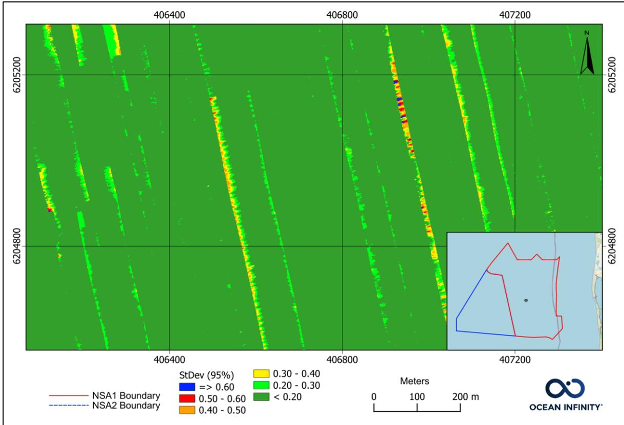
Figure 31 Example Standard Deviation plot of pycnocline affected area after initial processing.
