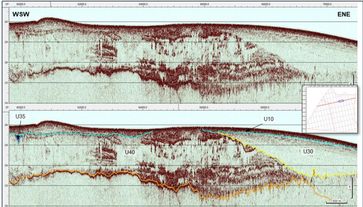
Figure 141 SBP example image of Unit40 Survey line BX01\_15000, position 409985E, 6221158N (image mid-point).
