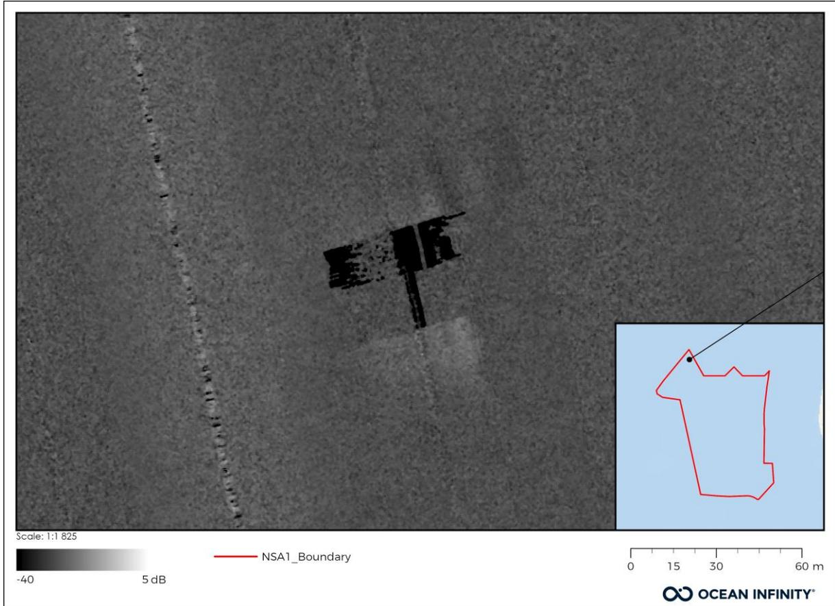
Figure 34 showing example of artefact (black) due to bubble-wash.
