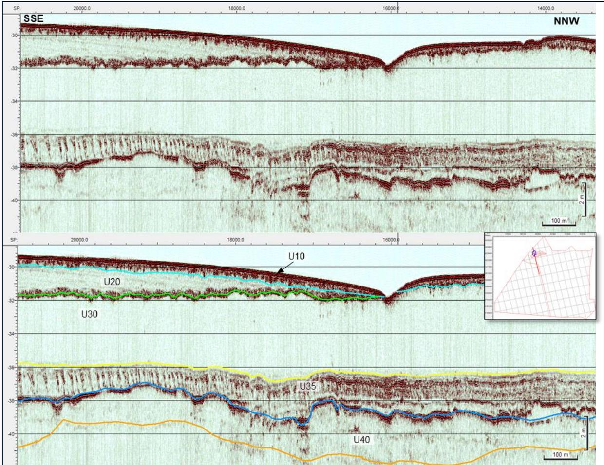
Figure 138 SBP example image of Unit 35 with (left) vertical stripes and without (right). Survey line BM12\_34930, position 39739E, 6226515N (image mid point).
