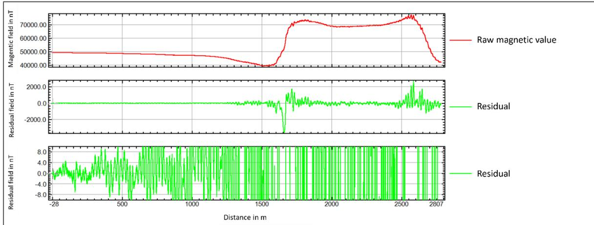
Figure 55 Magnetometer profiles showing magnetic response of cable Nordlink.
