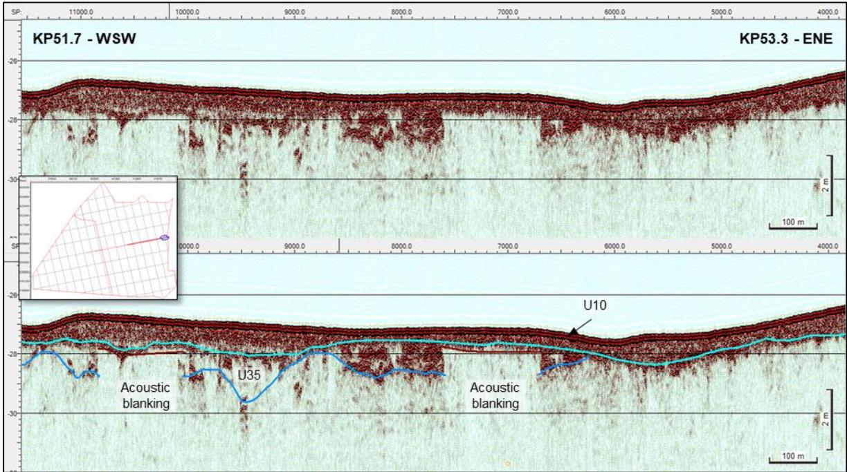
Figure 147 SBP example image of acoustic blanking. Survey line BX01\_27000, position 422328E, 6211550N (image mid-point).
