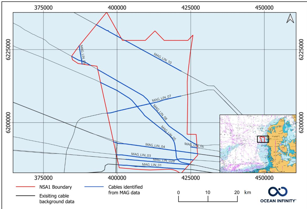
Figure 124 Magnetometer anomalies associated with existing infrastructure within the NSA1 survey area.
