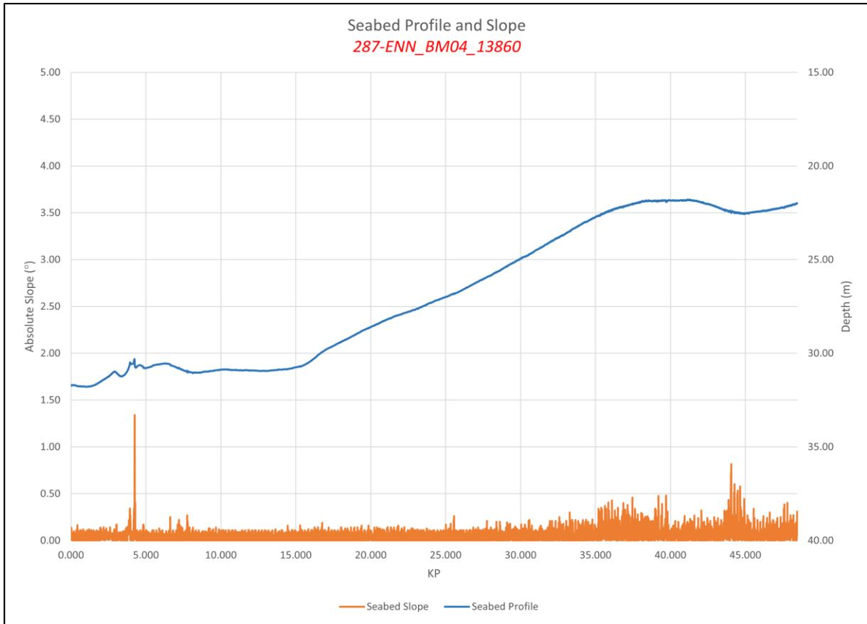
Figure 68 BM04\_13860 bathymetry longitudinal profile and slope.
