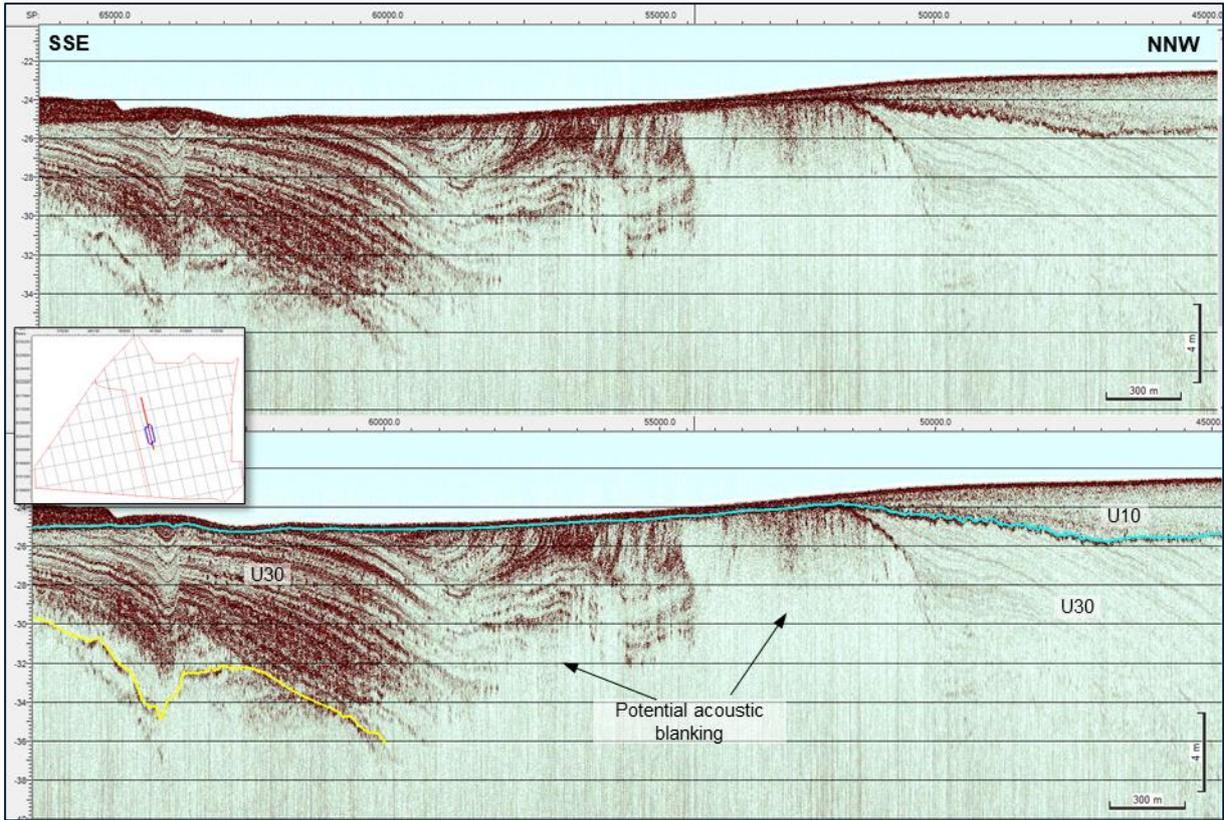
Figure 135 SBP example images of potential folding and acoustic blanking within Unit 30. Survey line BM10\_30100, position 400347E, 6204985N (image mid-point).
