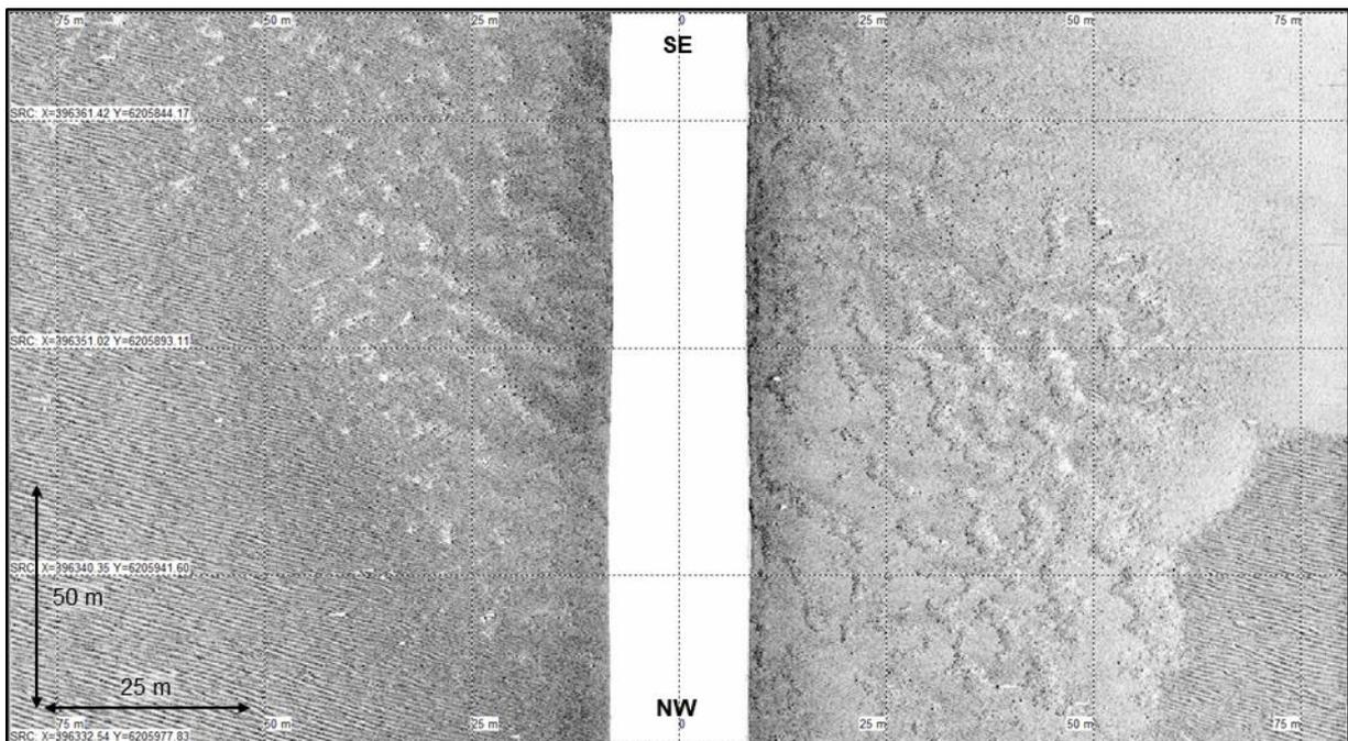
Figure 85 High frequency SSS example of TILL/DIAMICTON sediments (medium to high acoustic return).
