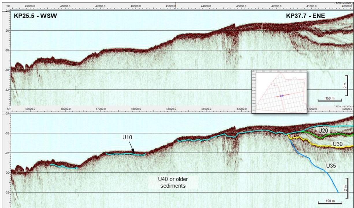
Figure 150 SBP example of outcropping U40 or older sediments in western part of Profile line BX01\_27000. Position 396961E, 6206050N (image mid-point).
