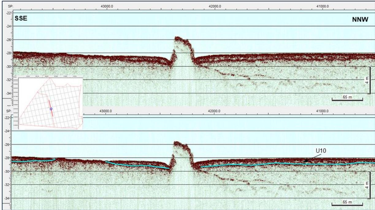
Figure 143 SBP image of outcropping Till. See also bathymetry image in Figure 76. Survey line BM11\_33320, position 397253E, 6204060N (image mid-point).
