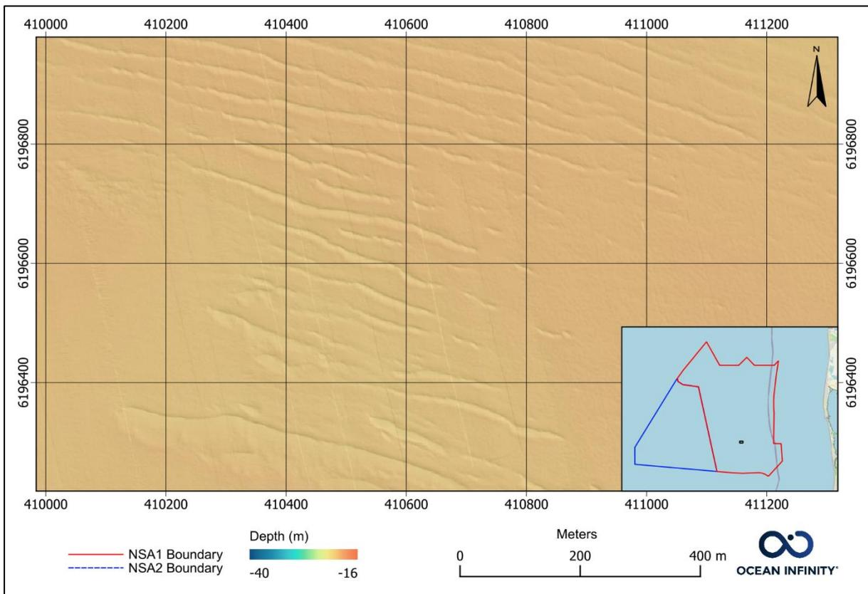
Figure 73 Sun-illuminated bathymetry – megaripples.
