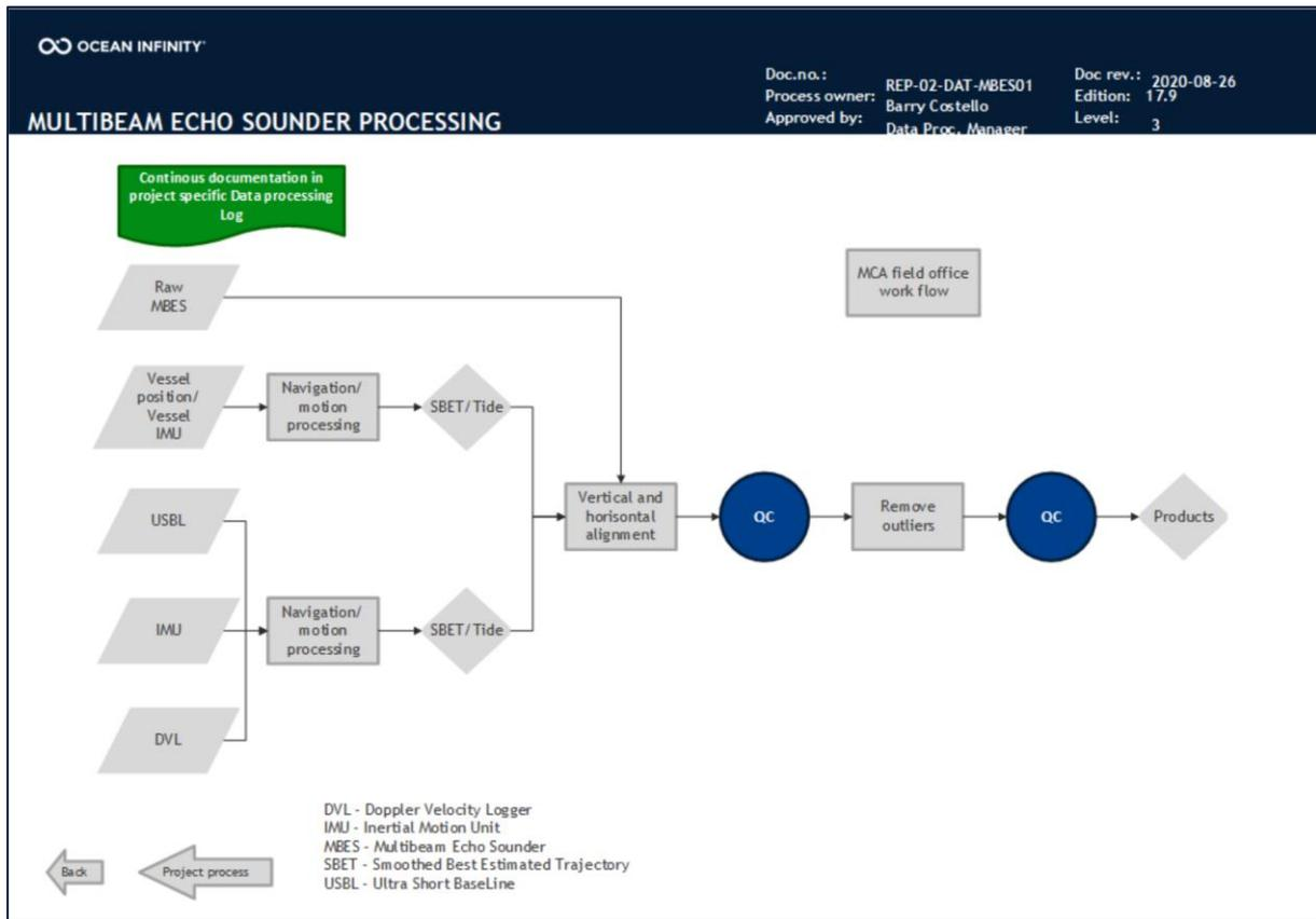
Figure 8 Workflow MBES processing.
