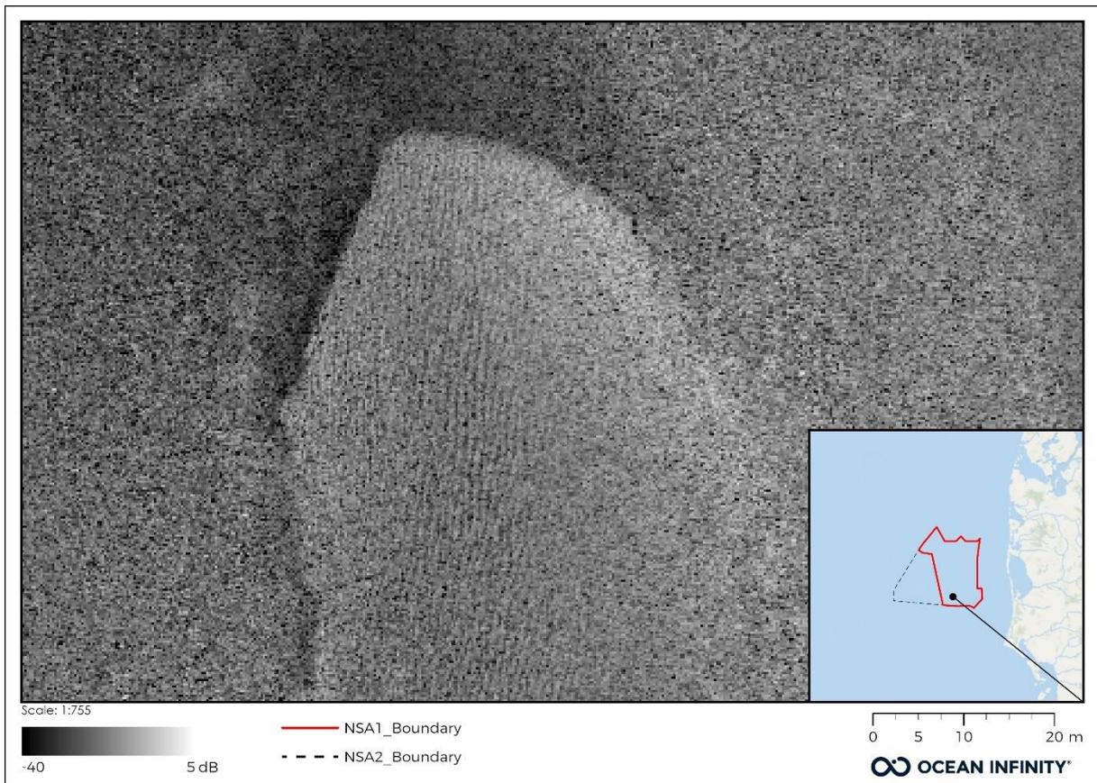
Figure 37 showing the speckled data processed in version 7.10 of FMGT.
