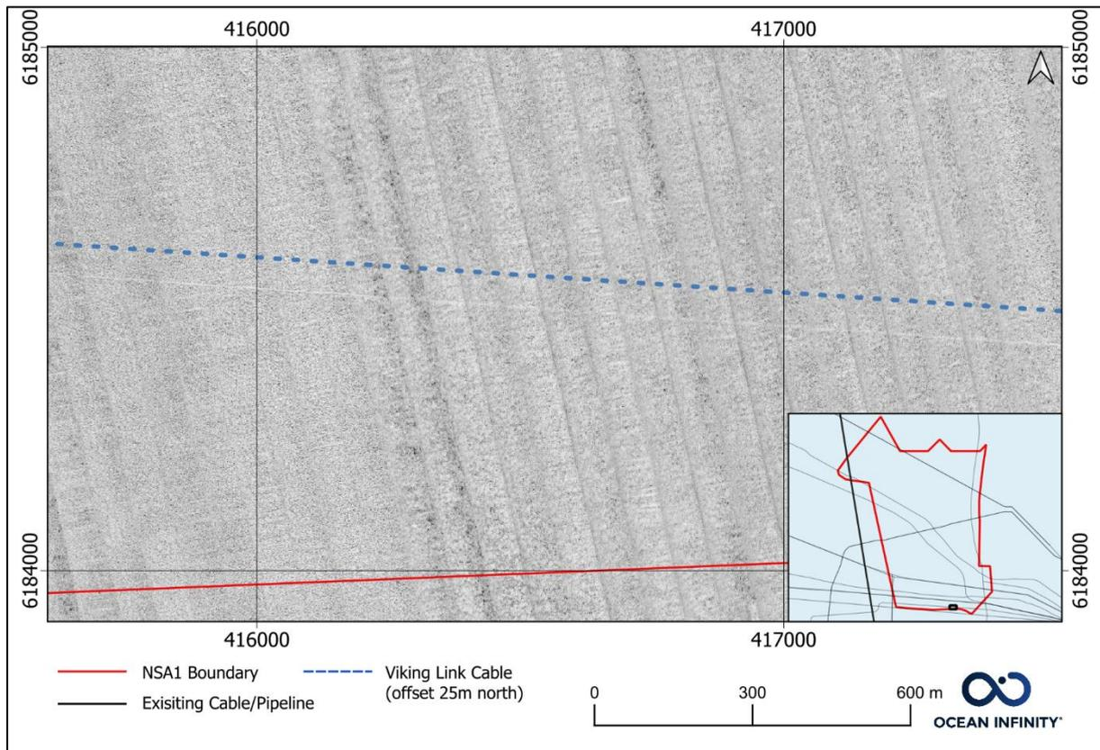
Figure 125 SSS images showing disturbed sediments related to the installation of the Viking Link cable.
