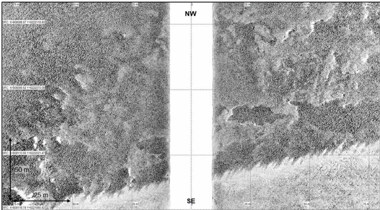
Figure 86 High frequency SSS example of Quaternary Clay and Silt sediments outcropping in block BM06.
