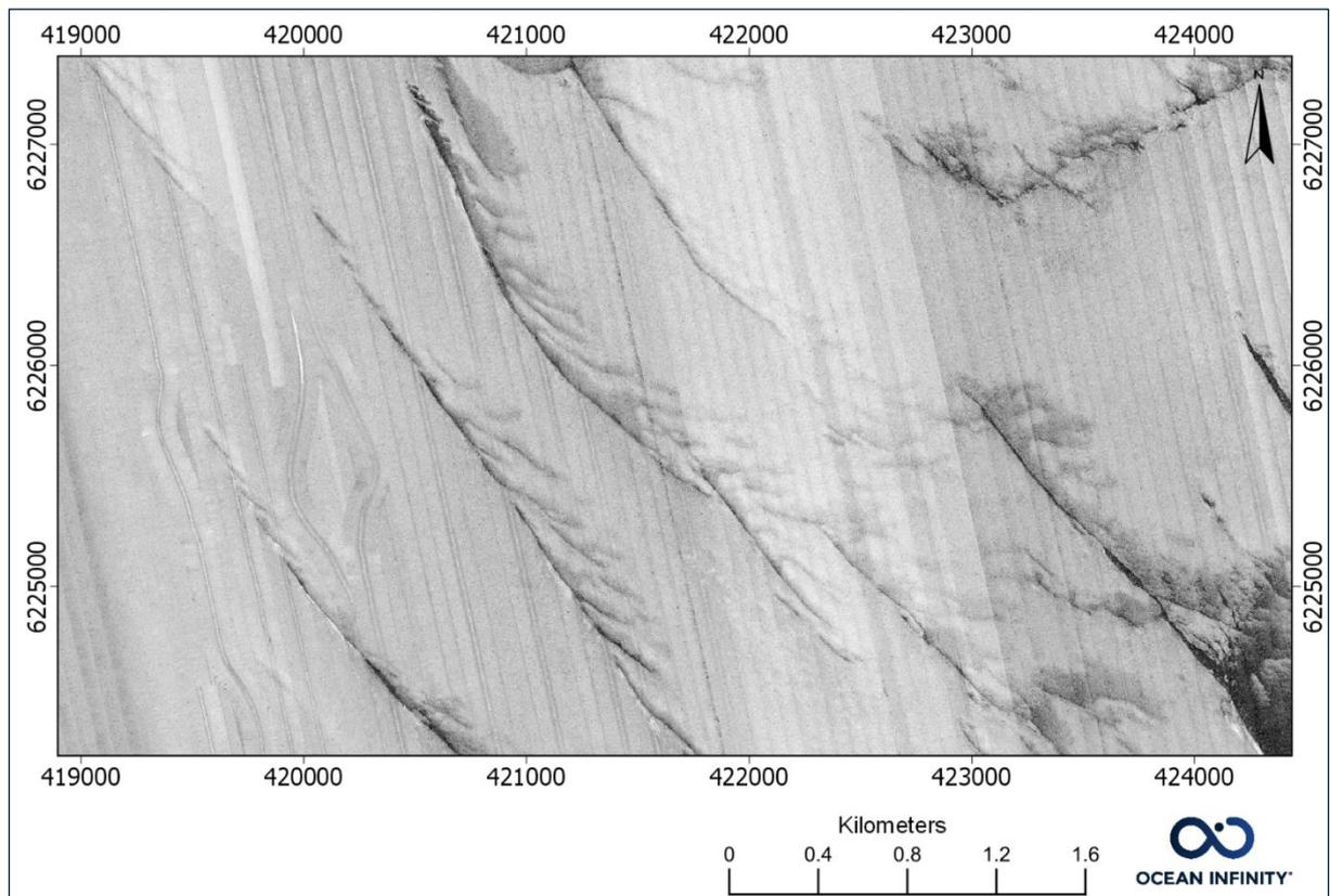
Figure 88 Example of sand waves on block BM01, orientated NW-SE.
