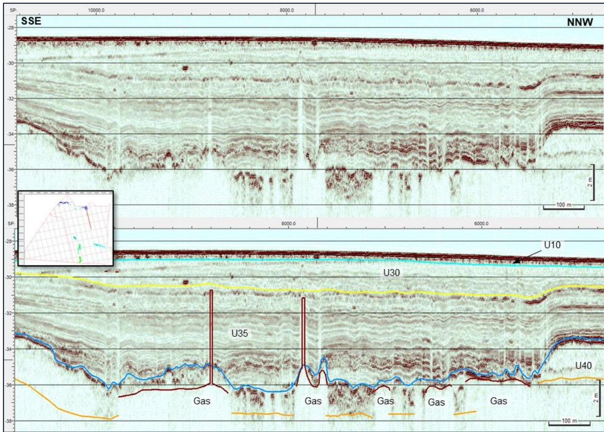
Figure 139 SBP example image of acoustic blanking (potential gas) at the base and within Unit 35. Survey line BM05\_16870, position 409798E, 6226603N (image mid point).
