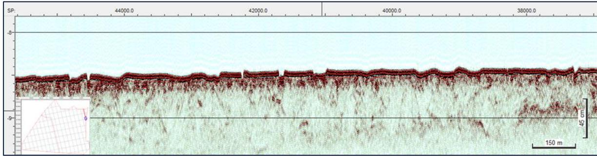
Figure 93 SBP example images of erosional depression visible in the seabed. Survey line BM01\_04340, position 423700E, 6218847N (image mid-point).
