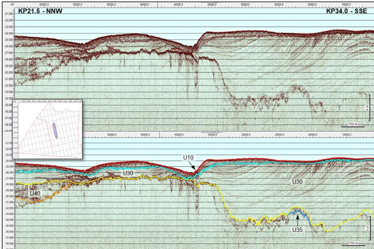
Figure 156 SBP example image of middle section of Profile line BM09\_27860. Position 401601E, 6209753N (image mid-point).
