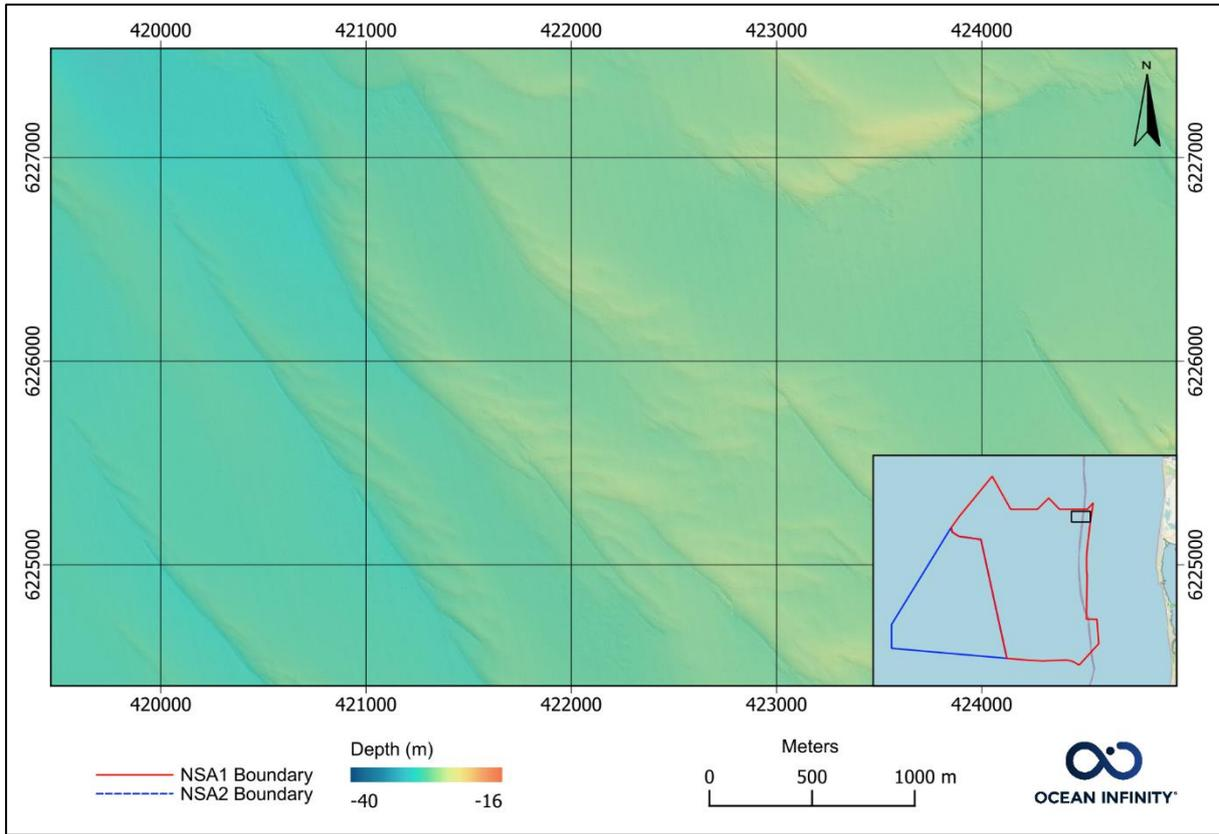
Figure 72 Sun-illuminated bathymetry – sandwaves.
