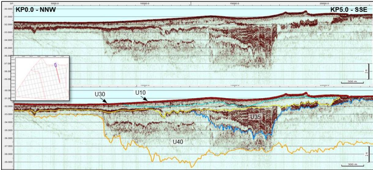
Figure 153 SBP example image of northern section of Profile line BM04\_13860. Position 411952E, 6228108N (image midpoint).
