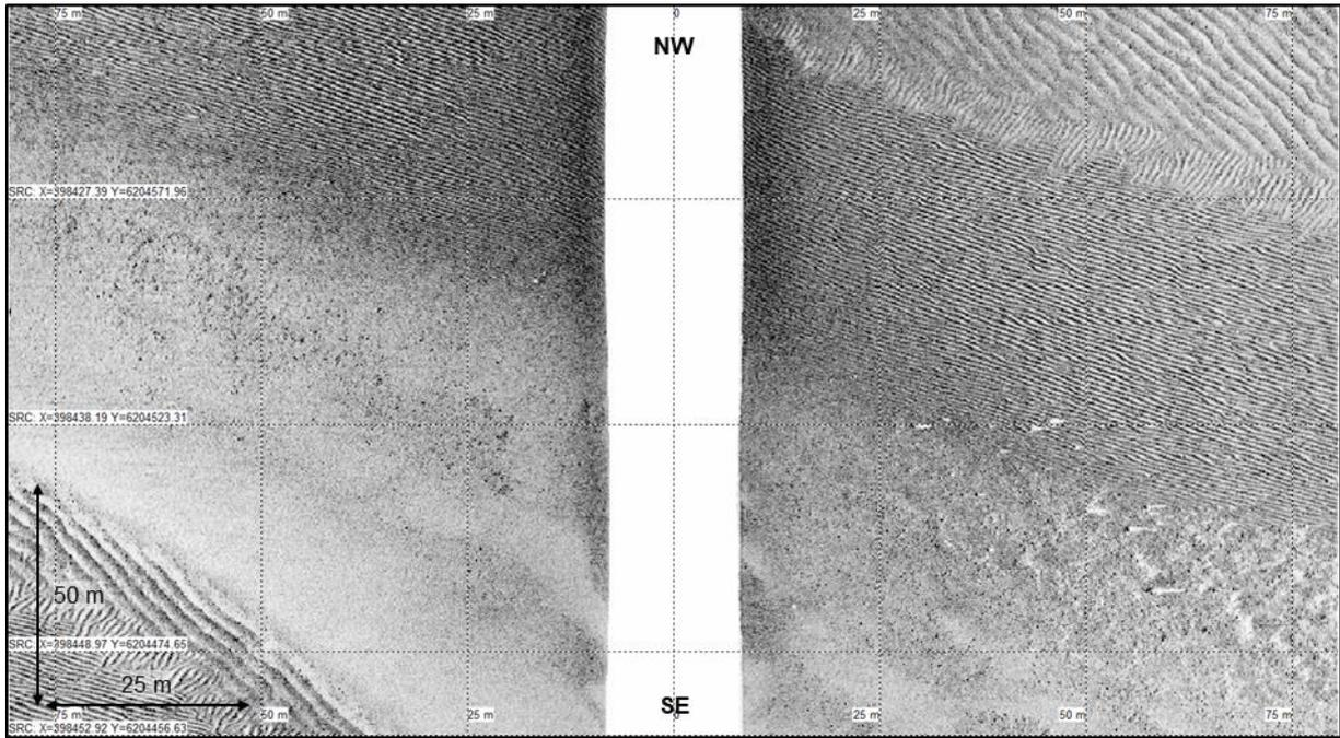
Figure 84 High frequency SSS example of SAND (medium acoustic return) and GRAVEL and coarse SAND (medium to high acoustic return) sediments.
