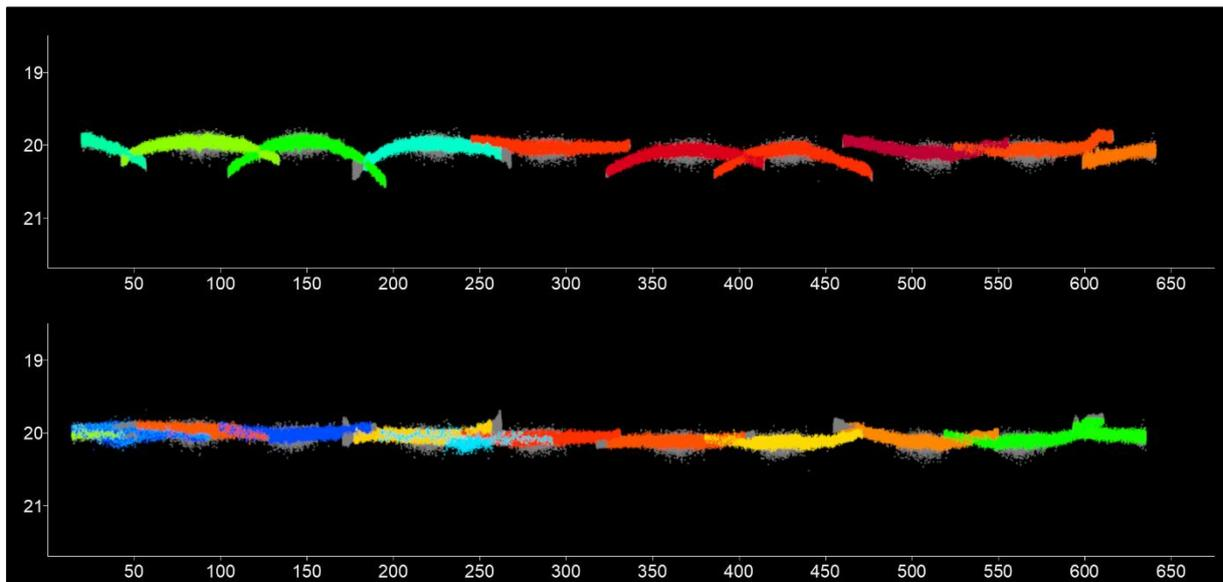
Figure 28 Cross-section of MBES data with sound velocity issues pre- and post-processing.
