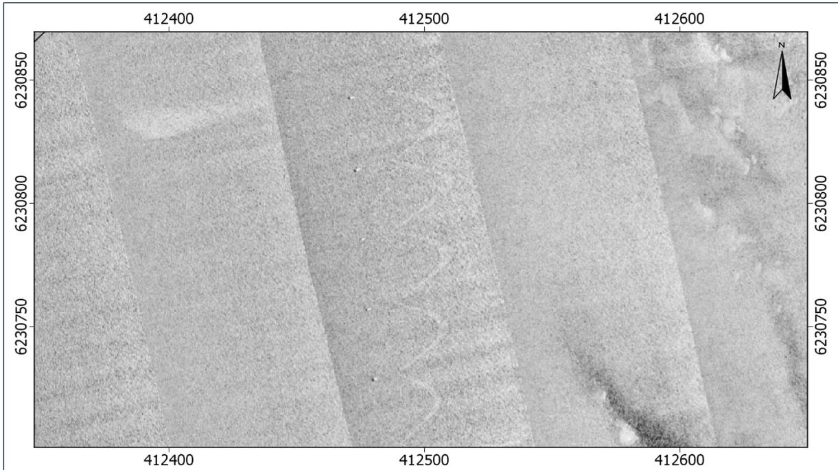
Figure 127 Example of fishing equipment with associated rope on SSS data, BM04.
