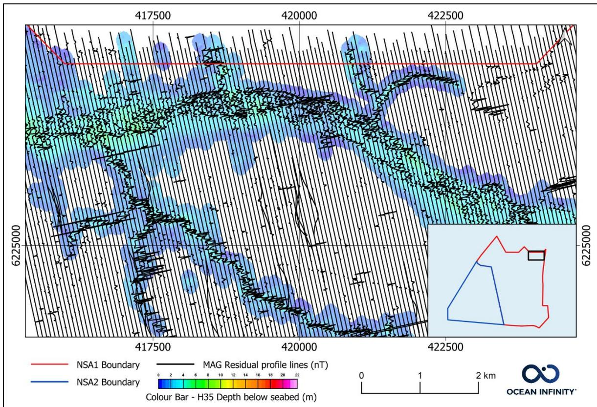
Figure 56 Close correlation between magnetic anomalies and SBP horizon H35 within NSA1 survey area.
