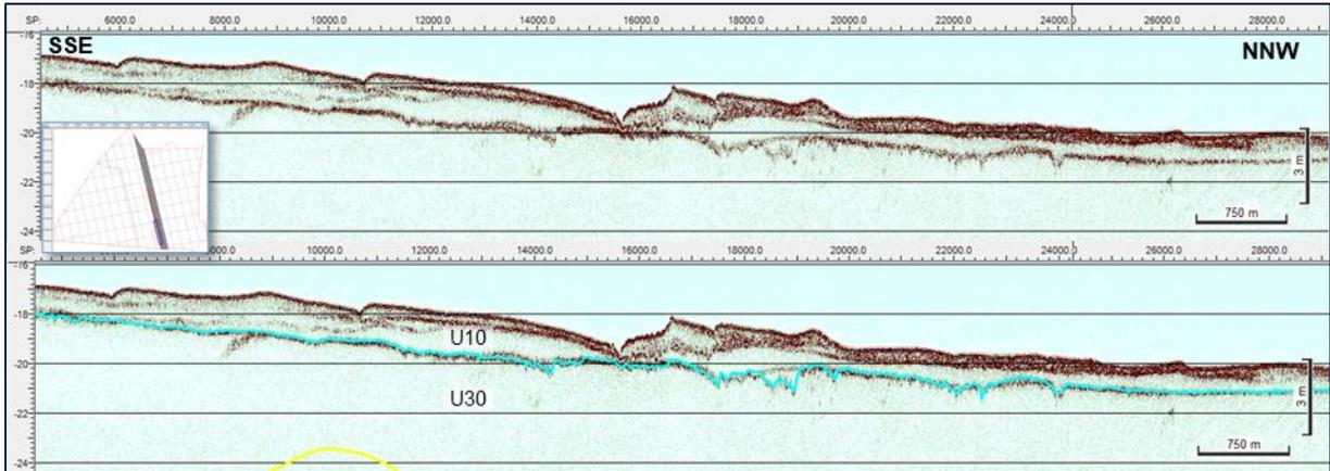
Figure 130 SBP example images of thicker Unit 10 in area of sandwaves. Survey line BM08\_25620, position 407959E, 6191046N (image mid-point).
