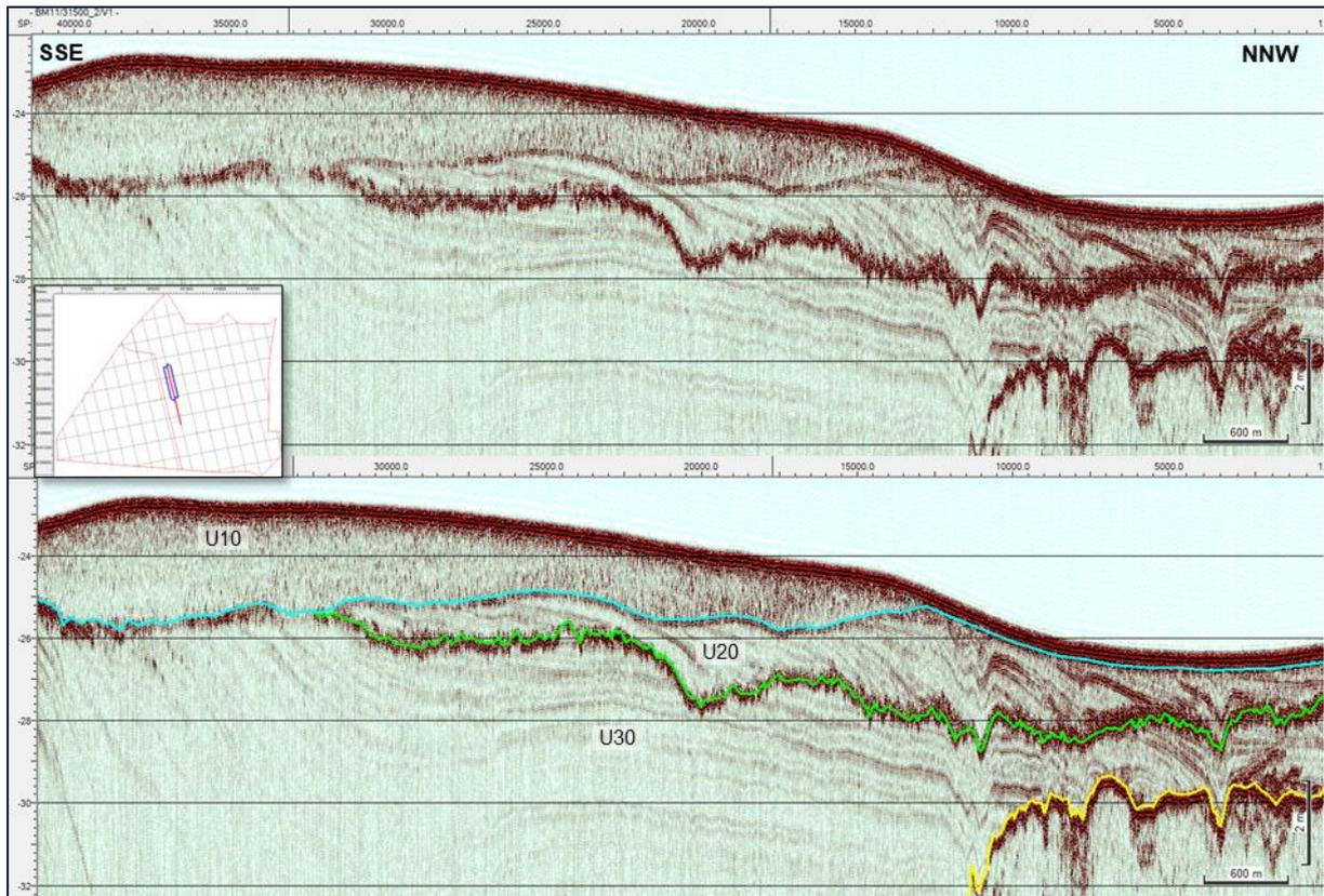
Figure 132 SBP example images of Unit 20. Survey line BM12\_31500, position 397671E, 6210726N (image mid-point).
