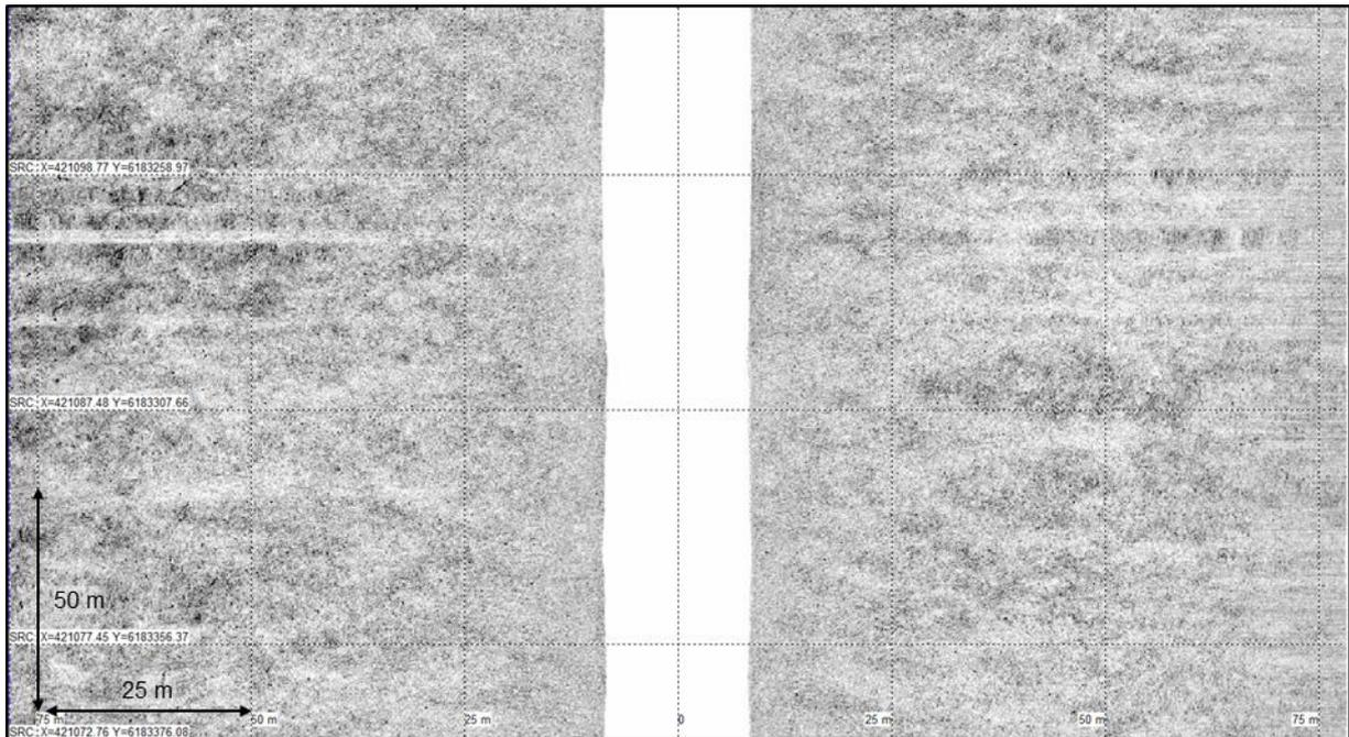
Figure 42 Example of striping in SSS data from strong pitch and roll effects in line BM05\_14420\_0005.
