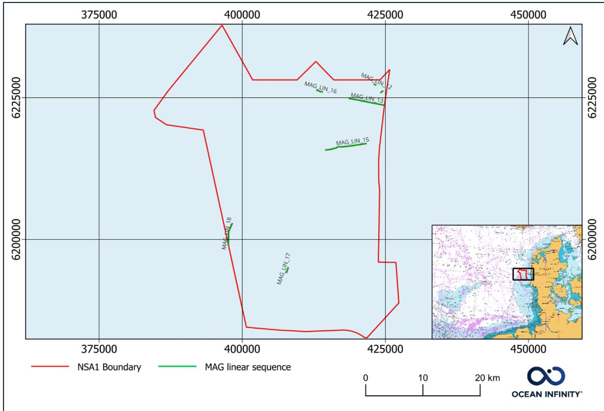
Figure 126 Digitised polylines from observed magnetic anomalies which form a linear sequence within NSA1 survey area.
