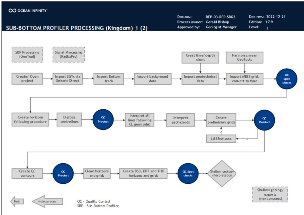
Figure 13 Workflow SBP processing (1/2).
