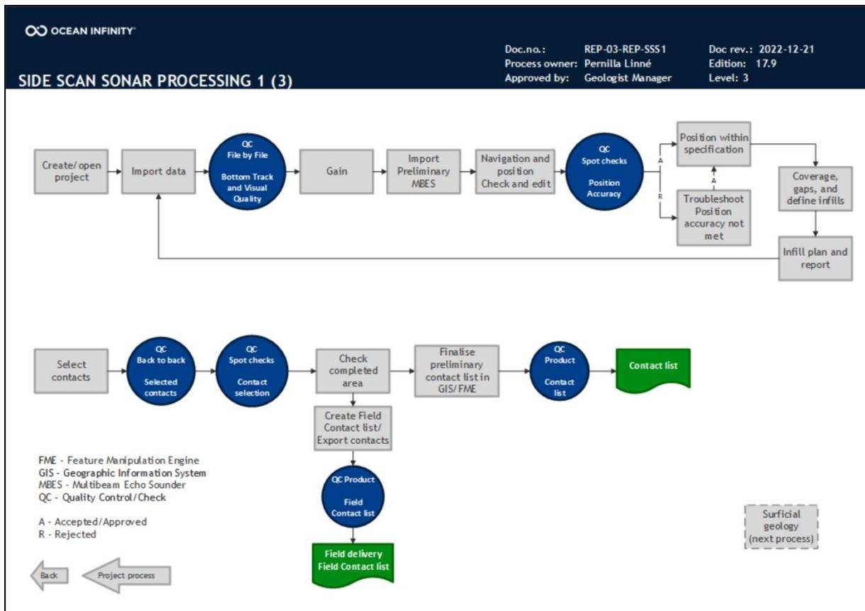
Figure 10 Workflow side scan sonar processing (1/3).
