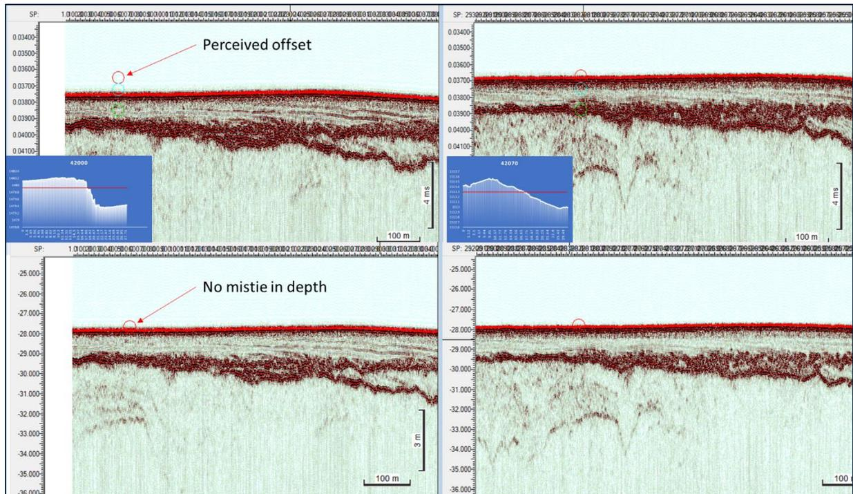
Figure 53 Demonstration of offsets in the time domain, corrected in the depth domain.
