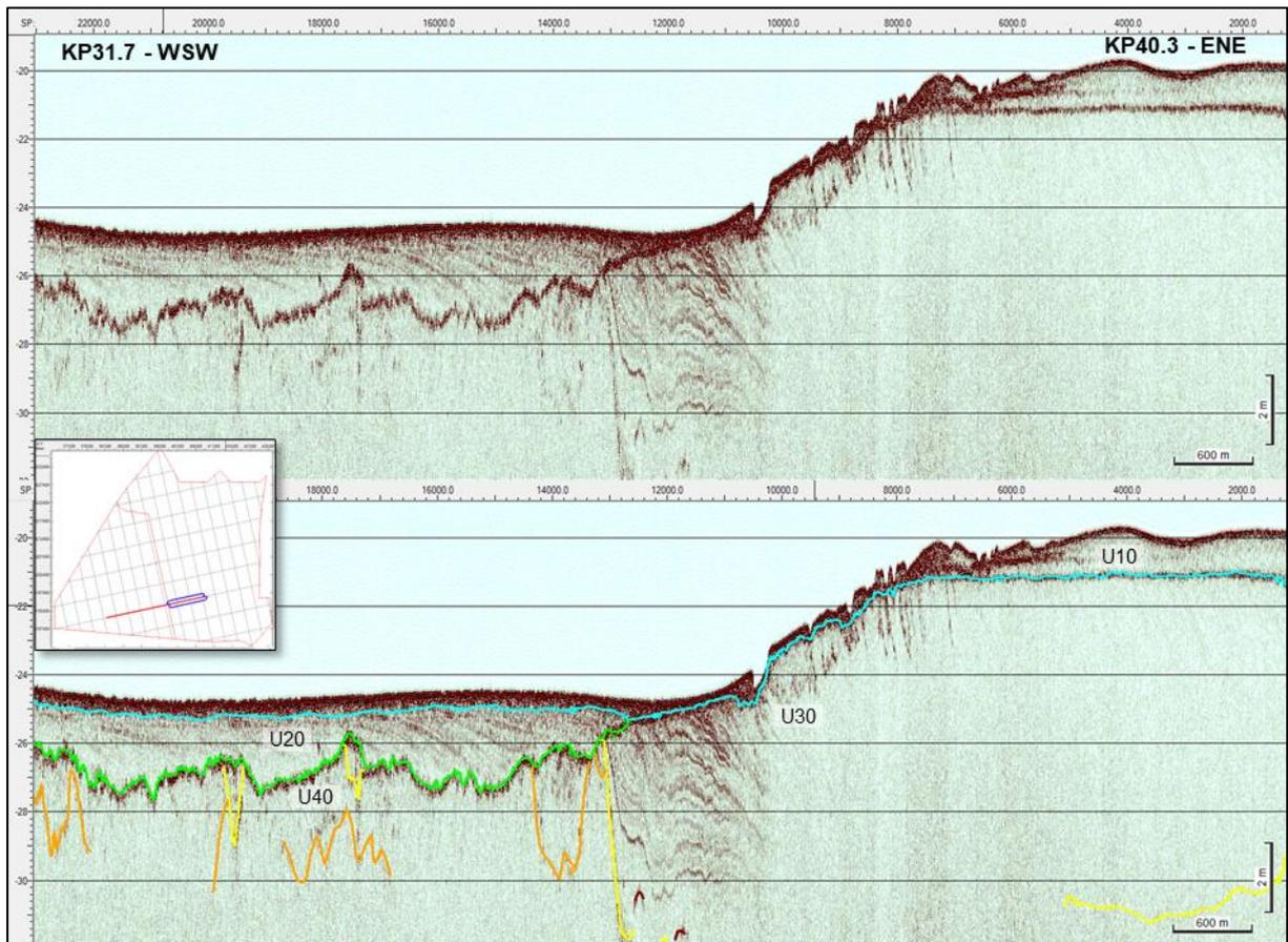
Figure 152 Profile BX01\_39000. Change in the main stratigraphy, U10 on top of U30 to U10 above U20. Position 403918E, 6195280N (image mid-point).
