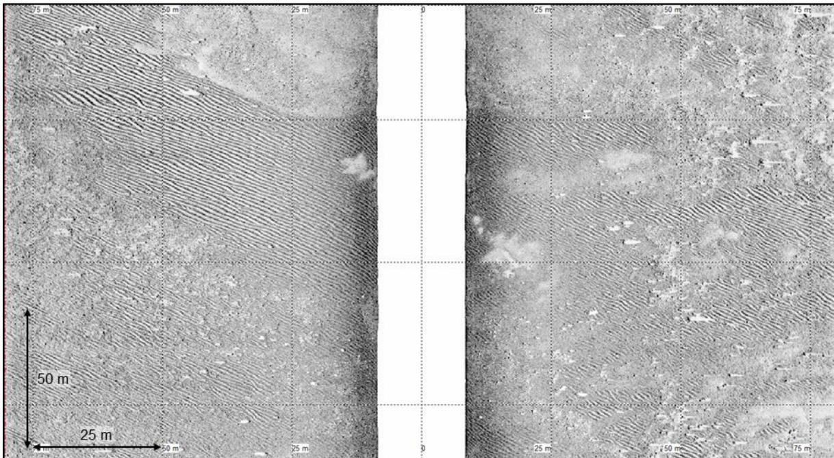
Figure 40 Example of good SSS data along line BM10\_30240\_INF001\_0707, showing boulders and ripples.
