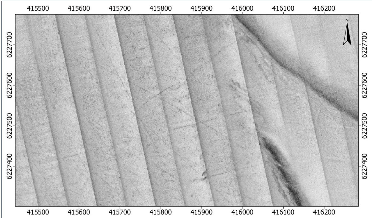
Figure 97 Example of trawl marks in SAND BM03.
