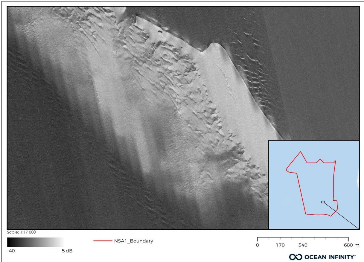
Figure 35 showing smearing artefacts showing smearing caused when passing sediment boundaries.
