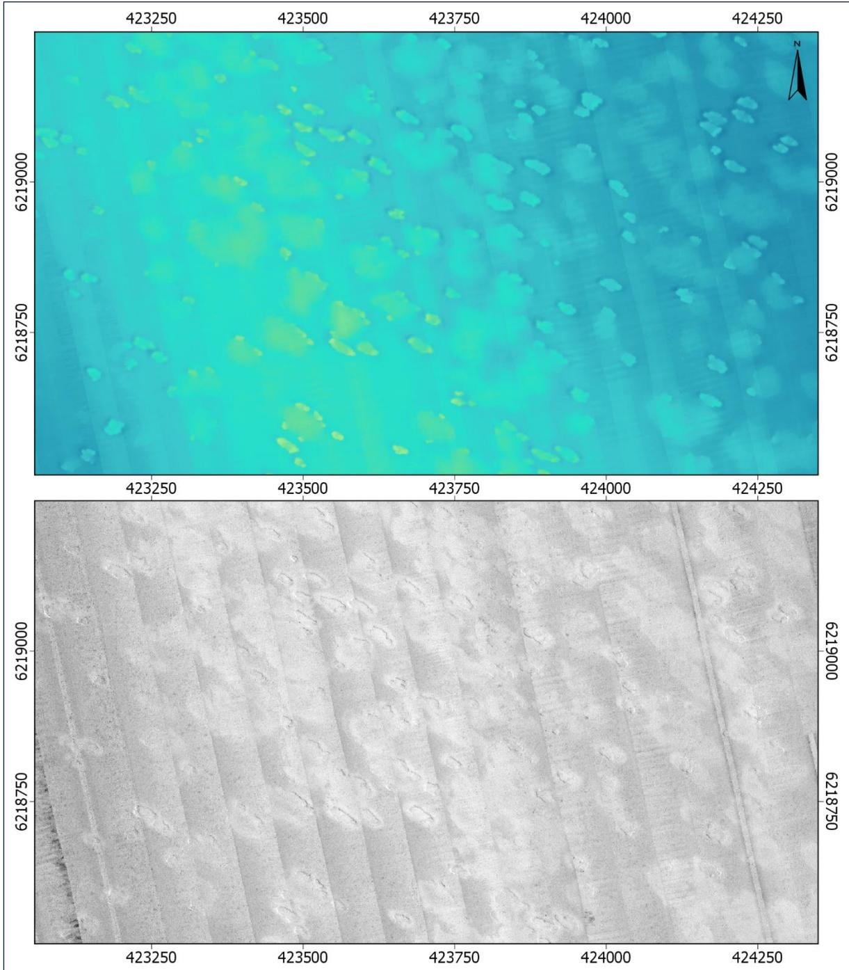
Figure 92 Erosional depressions on MBES (above) and SSS data (below). BM01.
