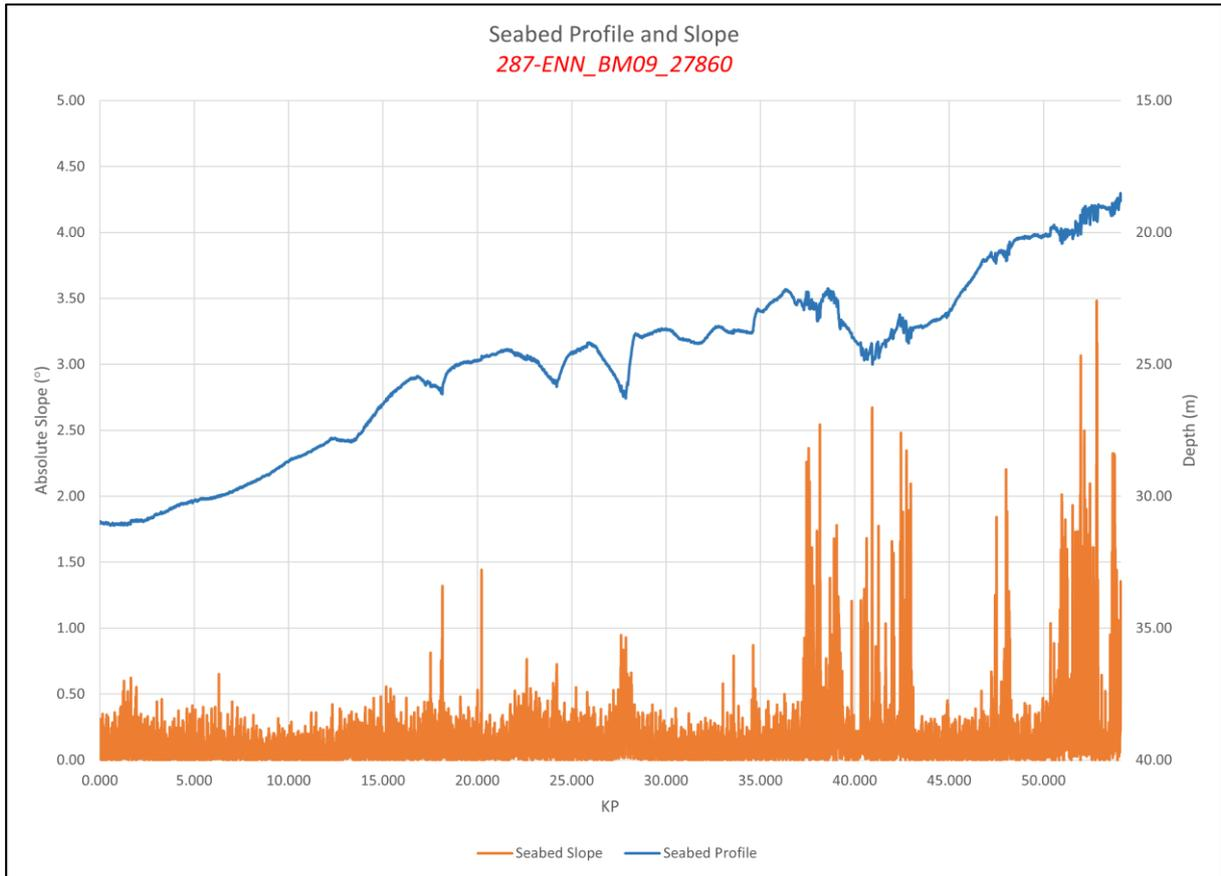
Figure 69 BM09\_27860 bathymetry longitudinal profile and slope.
