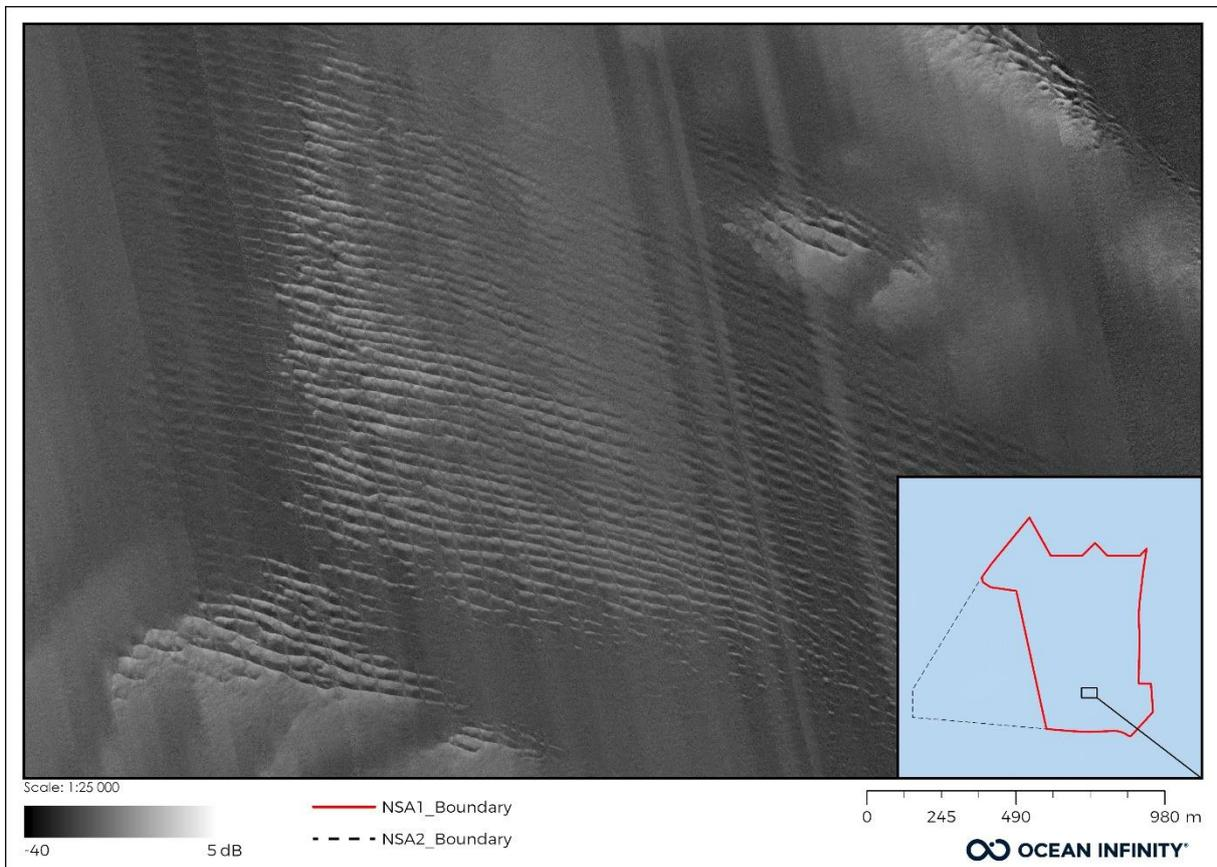
Figure 82 backscatter showing ripples in sand.
