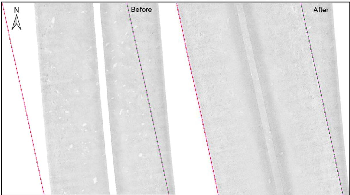
Figure 91 Example of exposed CLAY patches due to erosion of mobile top sediments before and after weather stand-by on BM10.
