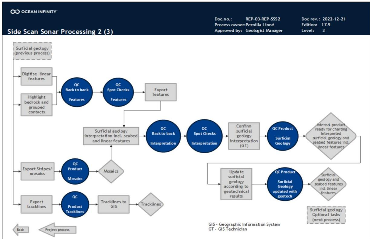
Figure 11 Workflow side scan sonar processing (2/3).
