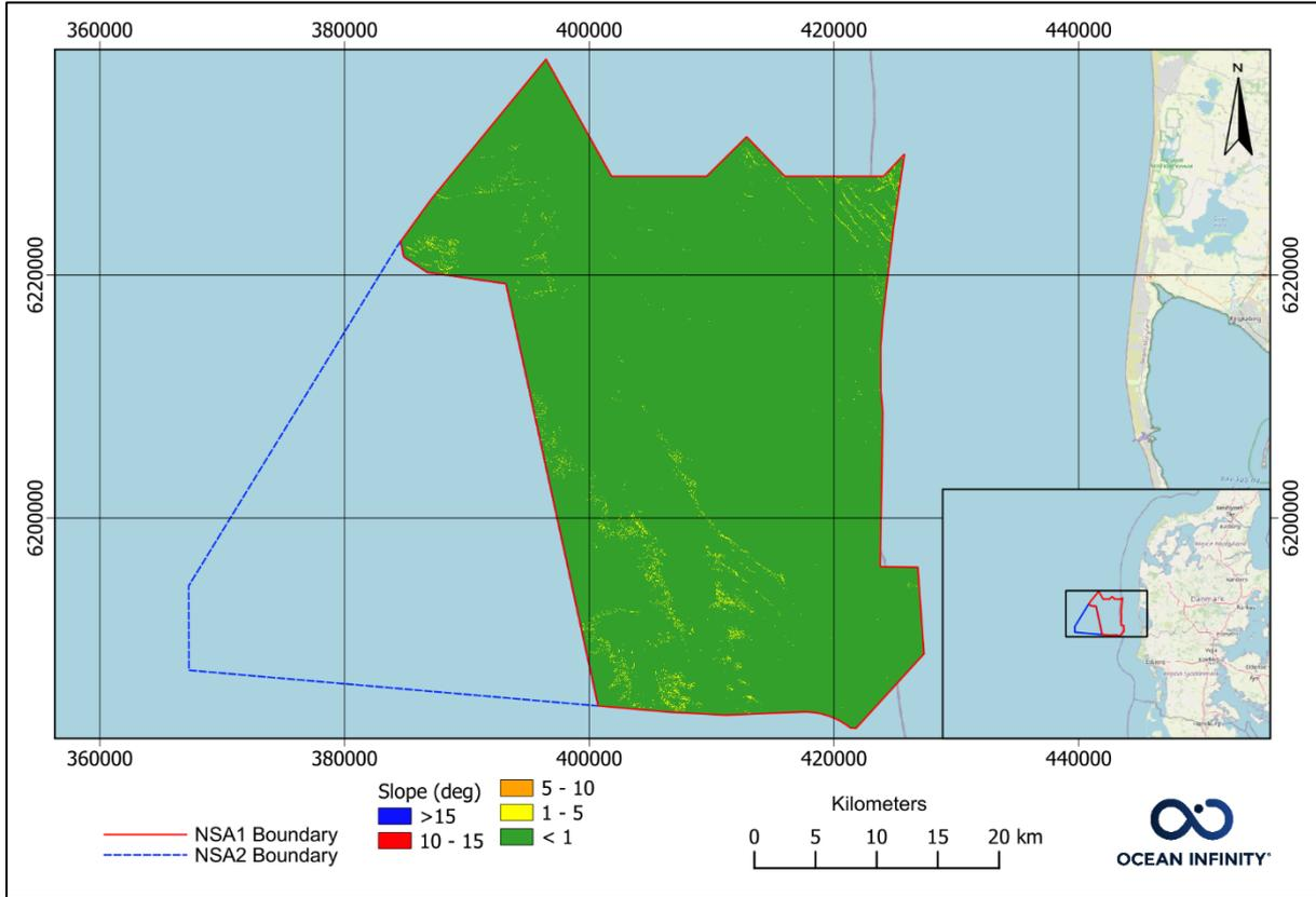
Figure 70 NSA1 bathymetry slope angle plot.
