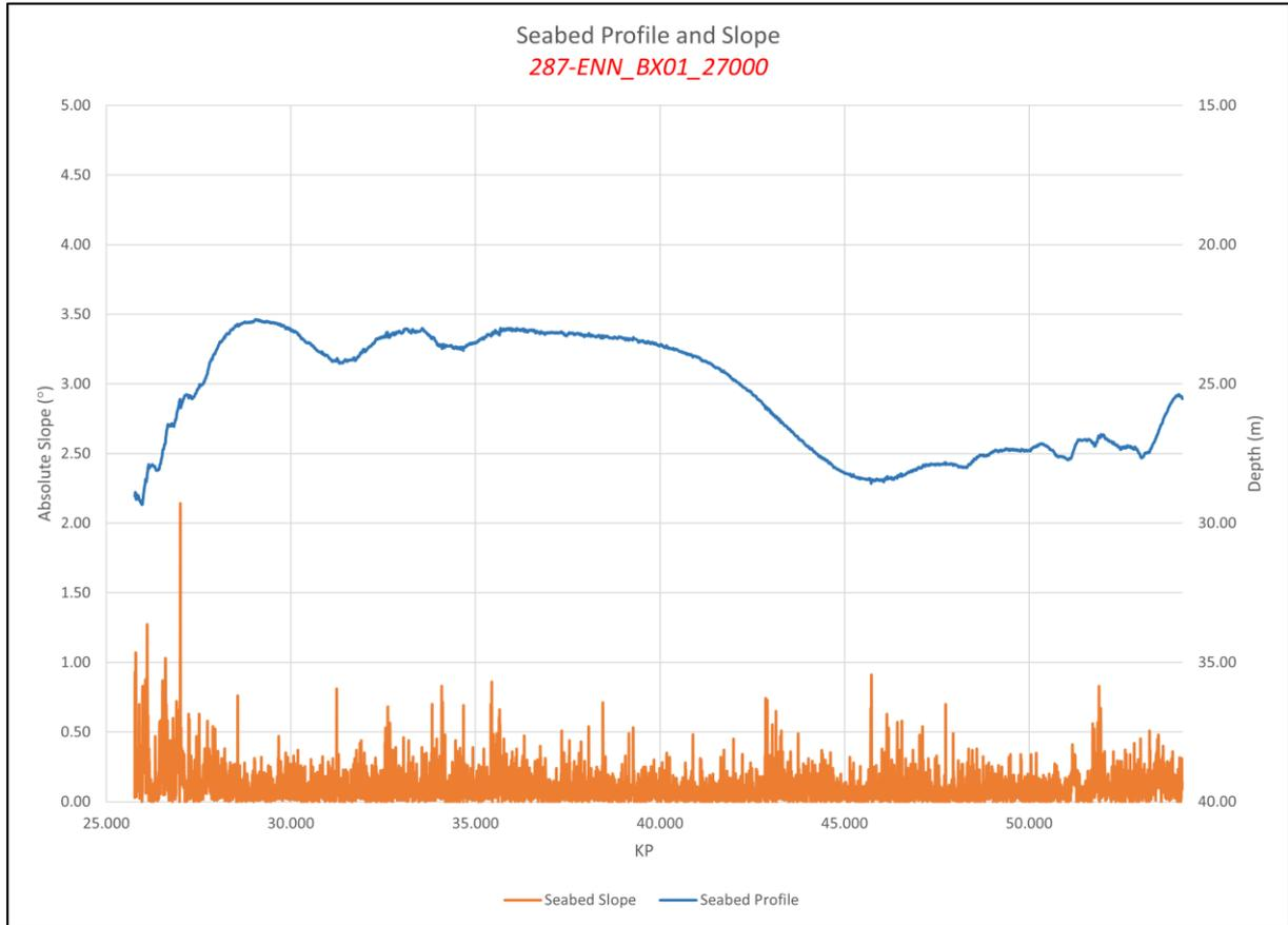
Figure 66 BX01\_27000 bathymetry longitudinal profile and slope.
