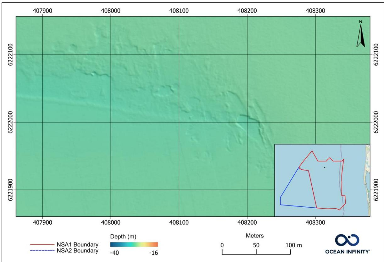
Figure 77 Sun-illuminated bathymetry - outcropping clay.
