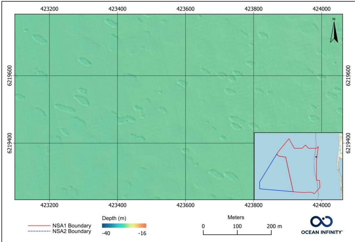
Figure 74 Sun-illuminated bathymetry - erosional depressions.
