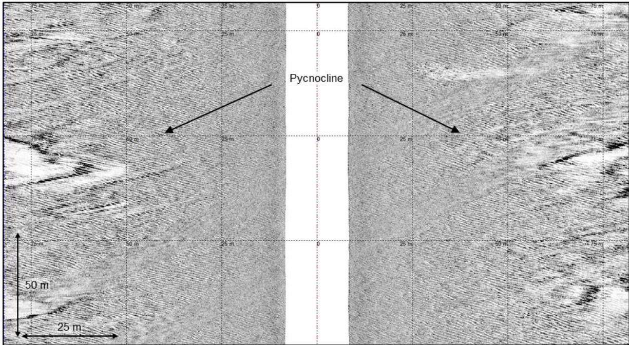
Figure 41 Pycnocline as observed on line BM14\_43540\_0659.009.
