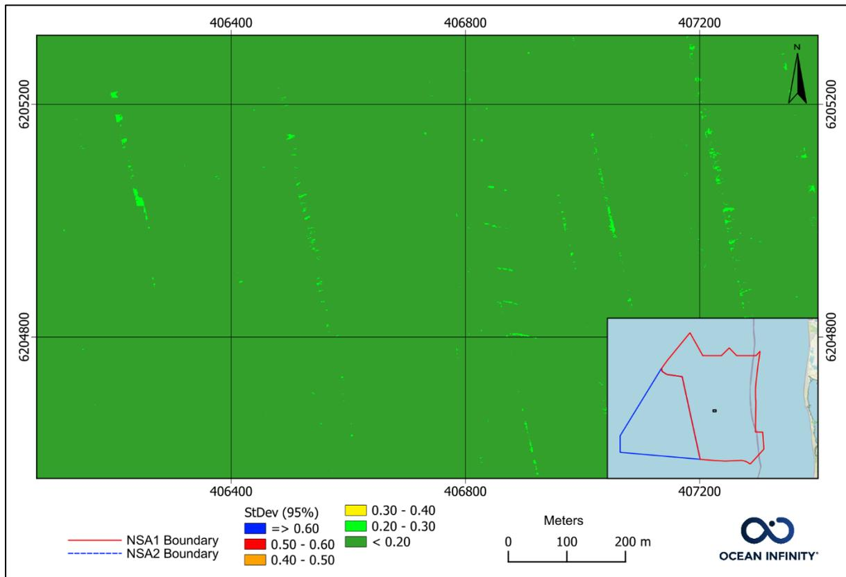
Figure 32 Example Standard Deviation plot of pycnocline affected area after further post-processing.
