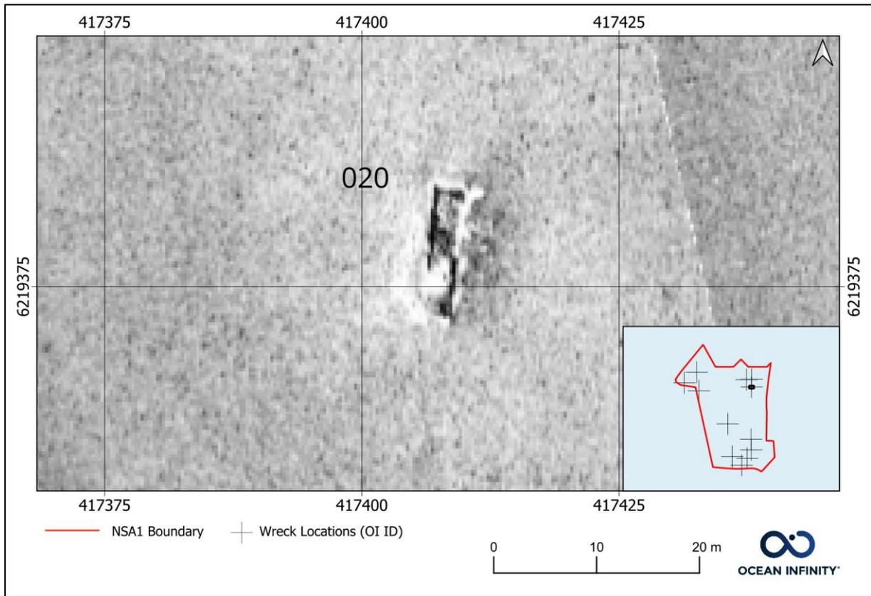
Figure 122 SSS image of possible shipping container (OI-020).
