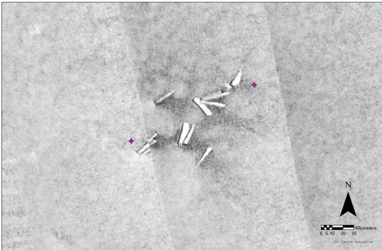
Figure 128 MAG anomalies correlated to discarded debris (likely pipes). The anomalies are manually correlated as they are 6 m and 10 m from the nearest debris item.
