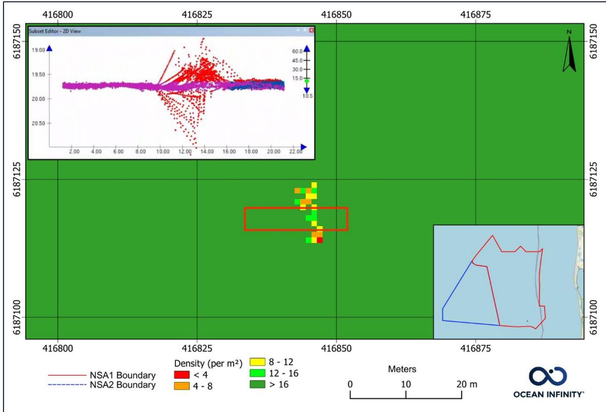
Figure 25 Low-density cells caused by data rejection during post-processing.
