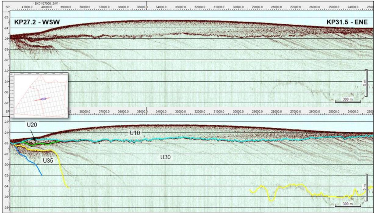
Figure 149 SBP example image of western part of Profile line BX01\_27000. Position 399599E, 6206622N (image mid-point).
