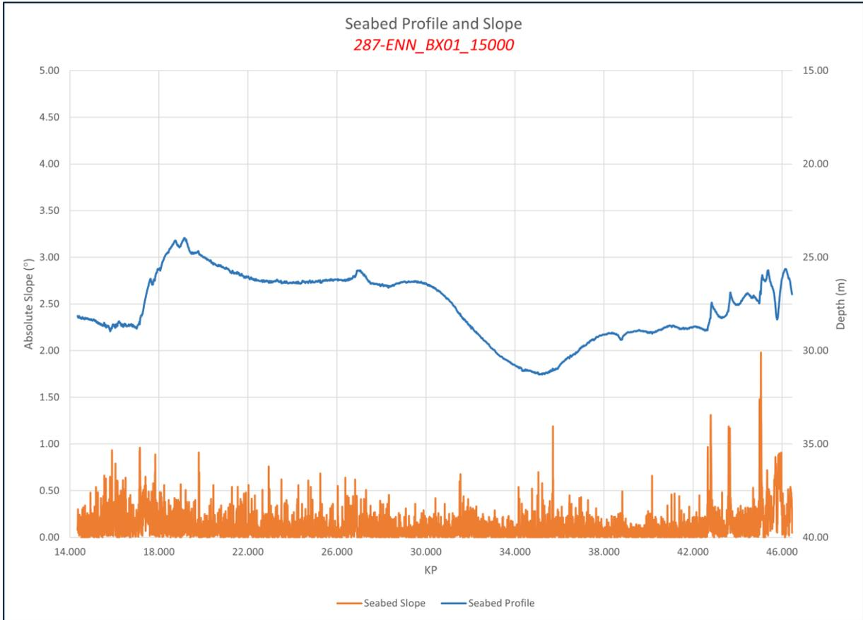
Figure 65 BX01\_15000 bathymetry longitudinal profile and slope.
