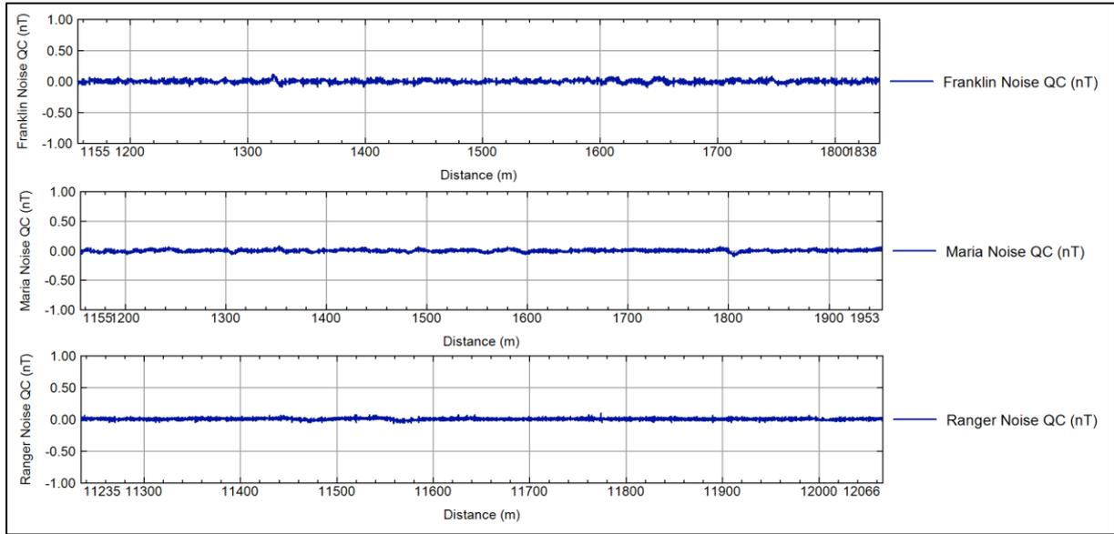
Figure 54 Noise QC of the raw nT data from the three vessels that acquired magnetometer data.
