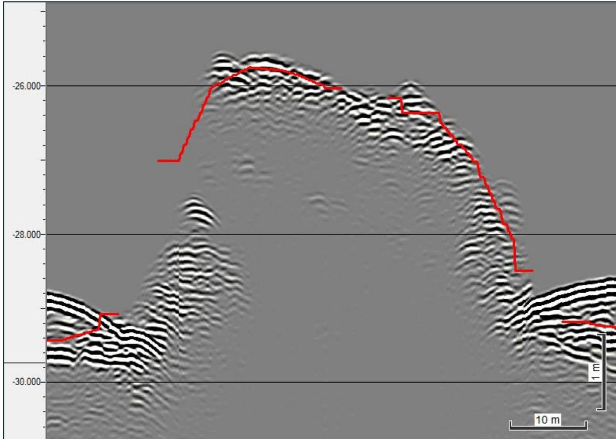
Figure 159 Example of stiff sediment grid error.
