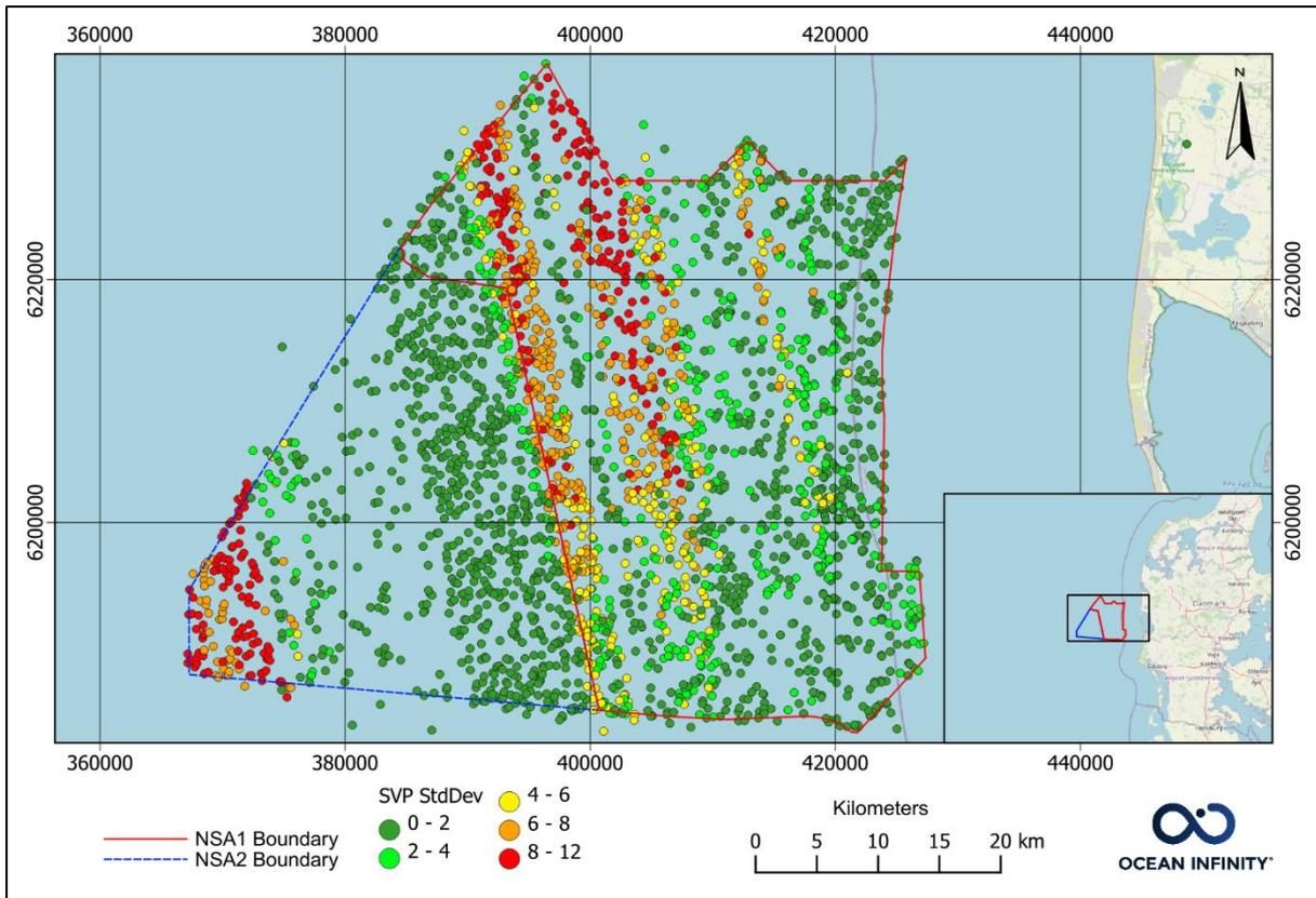
Figure 27 Sound Velocity Profile locations and Standard Deviation.
