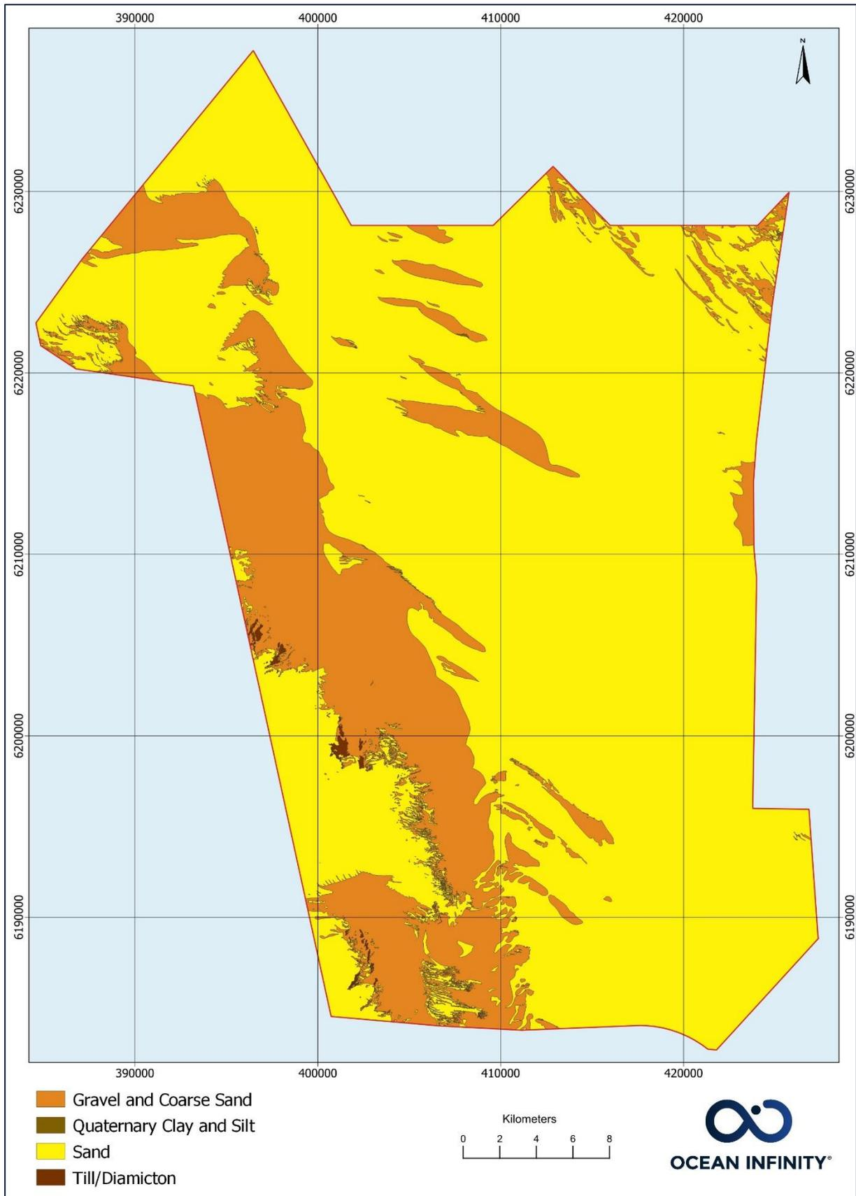
Figure 83 Overview of seabed sediments in the NSA1 survey area.
