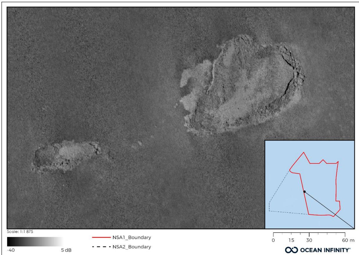
Figure 80 Outcropping till. Can also be seen in the bathy data in Figure 76 and in the SBP in Figure 143.
