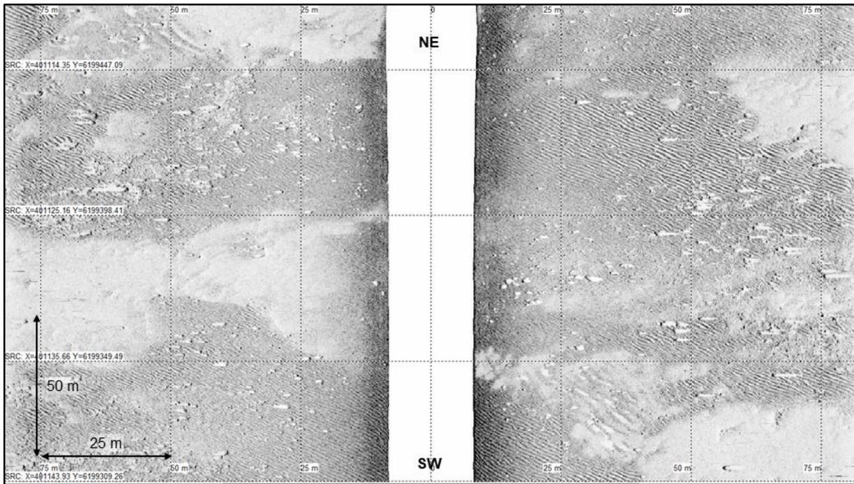
Figure 95 Example of boulder field area, Block BM10.
