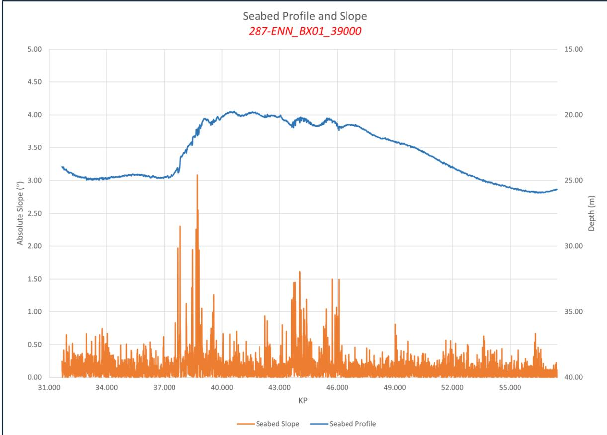
Figure 67 BX01\_39000 bathymetry longitudinal profile and slope.
