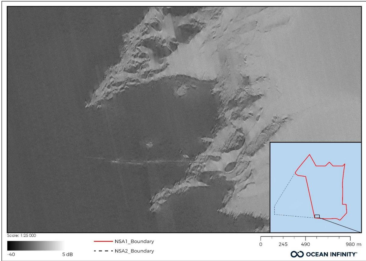
Figure 81 Sediment boundaries from the backscatter. Dark grey area is sand and lighter area is gravel and coarse sand.
