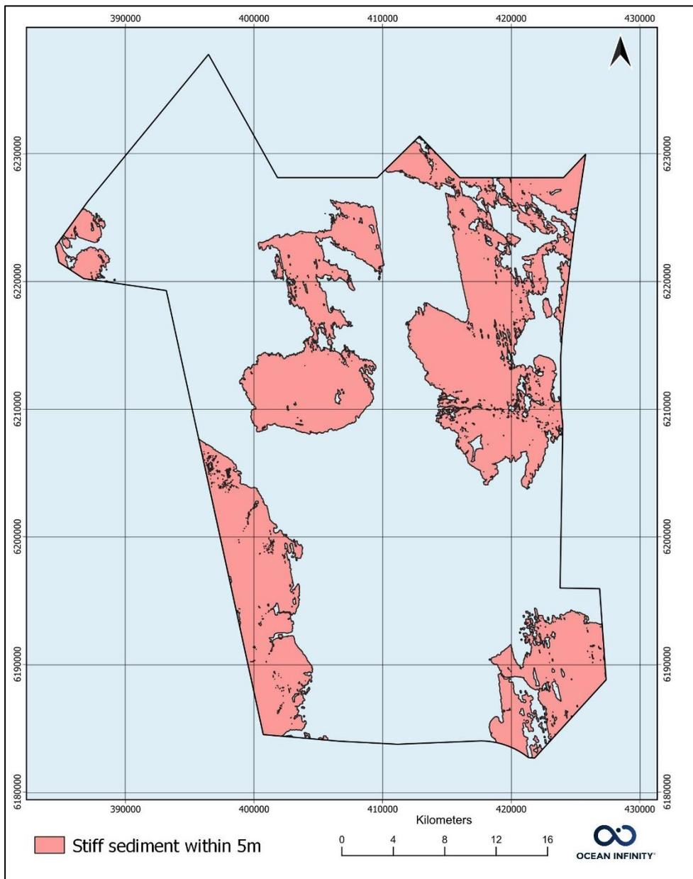
Figure 158 Areas where stiff sediments may be within 5 m of the seabed.
