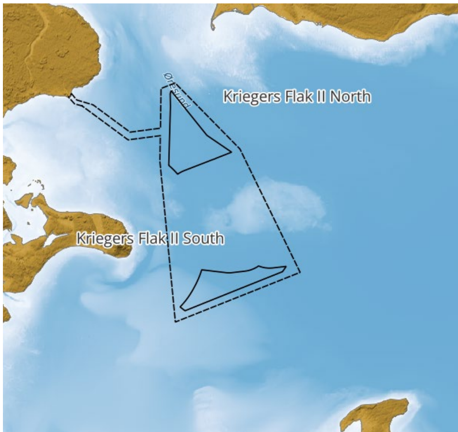
Figure 2-1 Overview of the windfarm area Kriegers Flak II. The dashed line indicates the full data delivery area, and the hatched areas indicate the OWFs.
