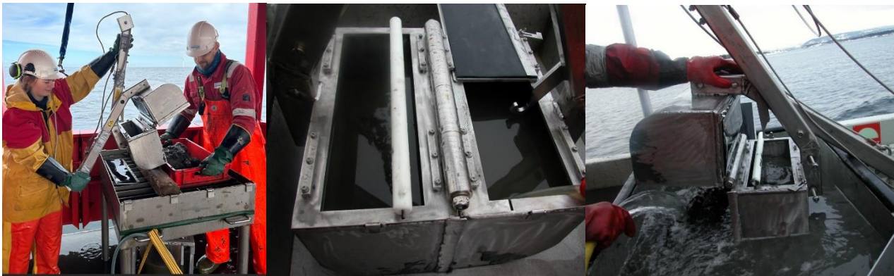
Figure 3-6. Grab sampling. Grab type used, a Van Veen type grab (collects sediments for 0.1 m 2 samples of macrofauna and 0.05 m 2 for sediment chemistry and grain size analyses).
