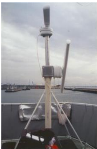
Figure 4-4 Horizontal and vertical radar mounted on a research vessel.
