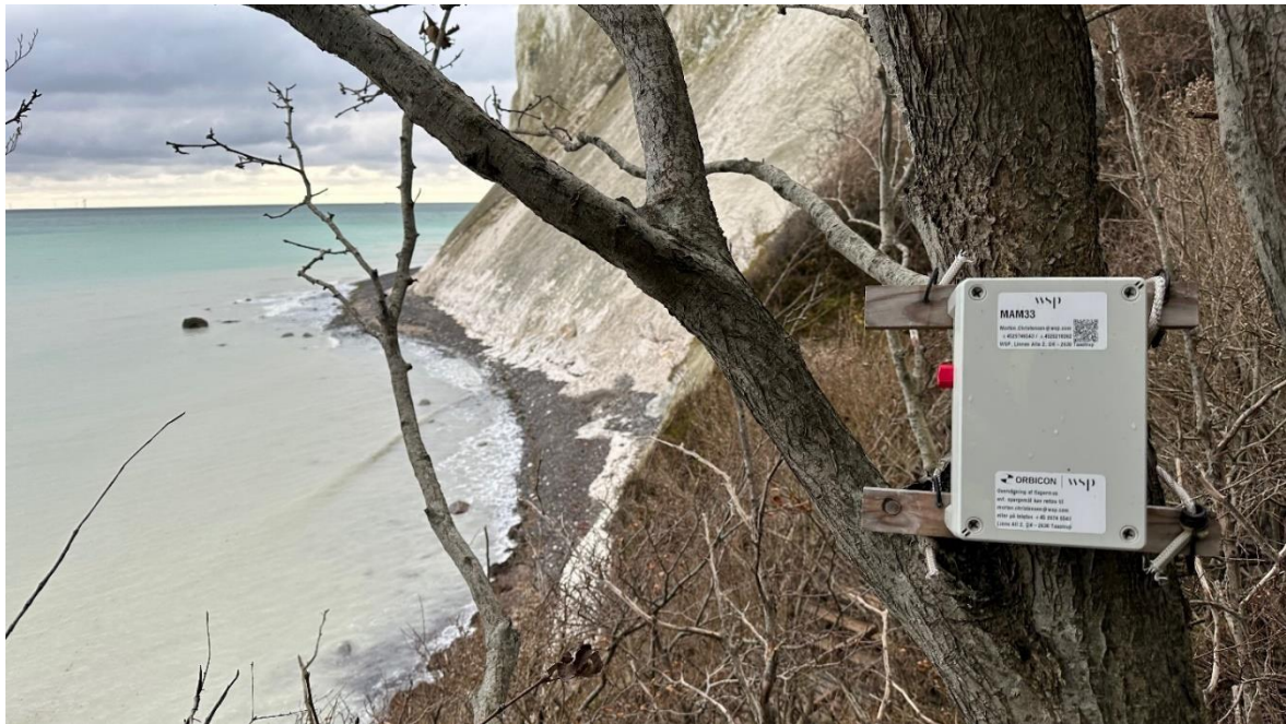
Figure 12 – Bat detector mounted on a tree at the coast of Møn
