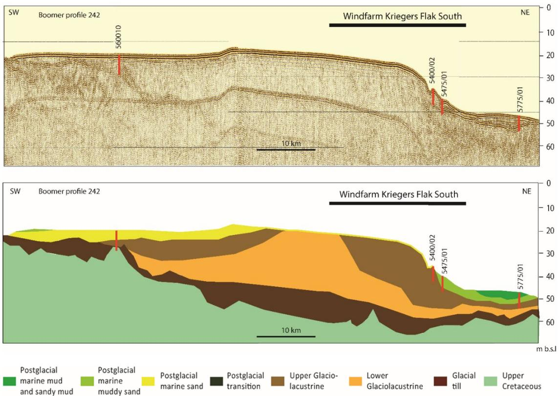
Figure 8.9 Boomer profile 242 and geological interpretation. For location, see Figure 8.4.
