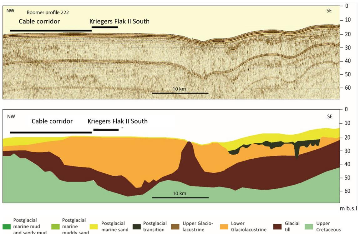
Figure 8.14 Boomer profile 222 and geological interpretation. For location, see Figure 8.4.
