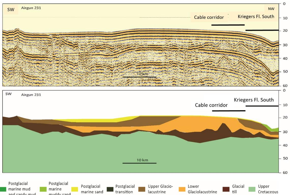
Figure 8.8 Airgun profile 231 and geological interpretation. For location, see Figure 8.4.
