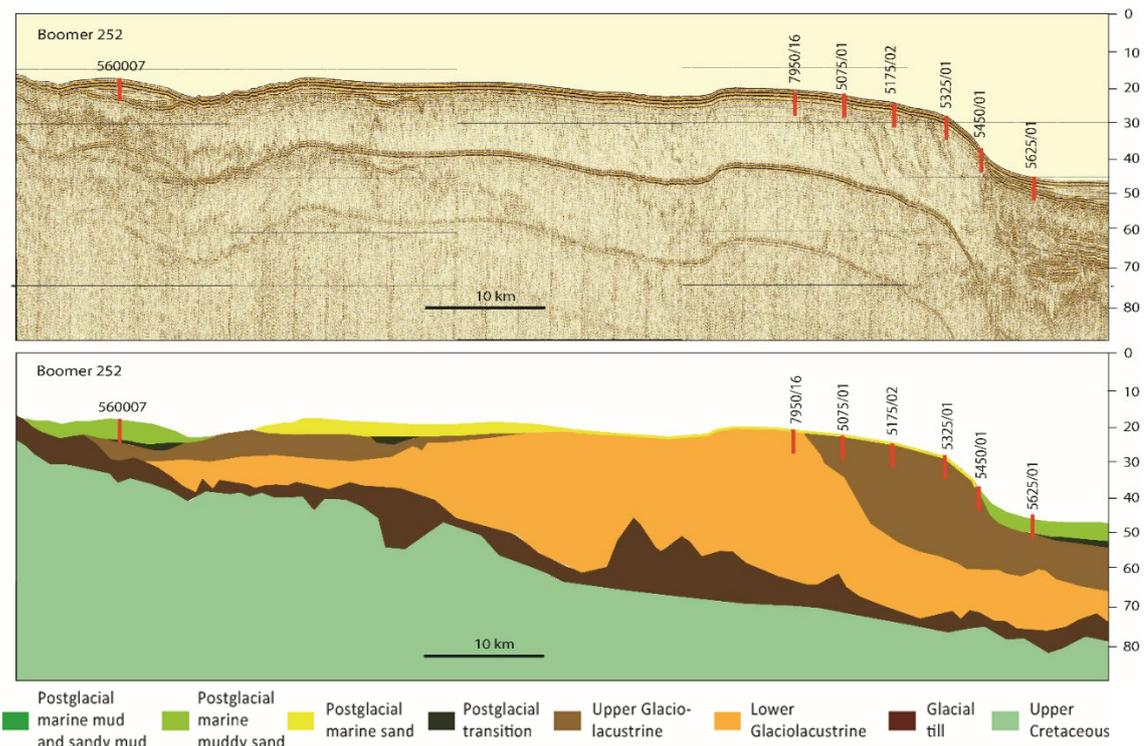
Figure 8.12 Boomer profile 252 and geological interpretation. For location, see Figure 8.4.
