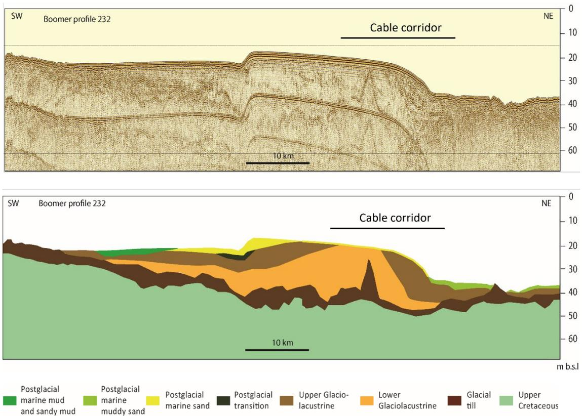
Figure 8.7 Boomer profile 232 and geological interpretation. For location, see Figure 8.4.
