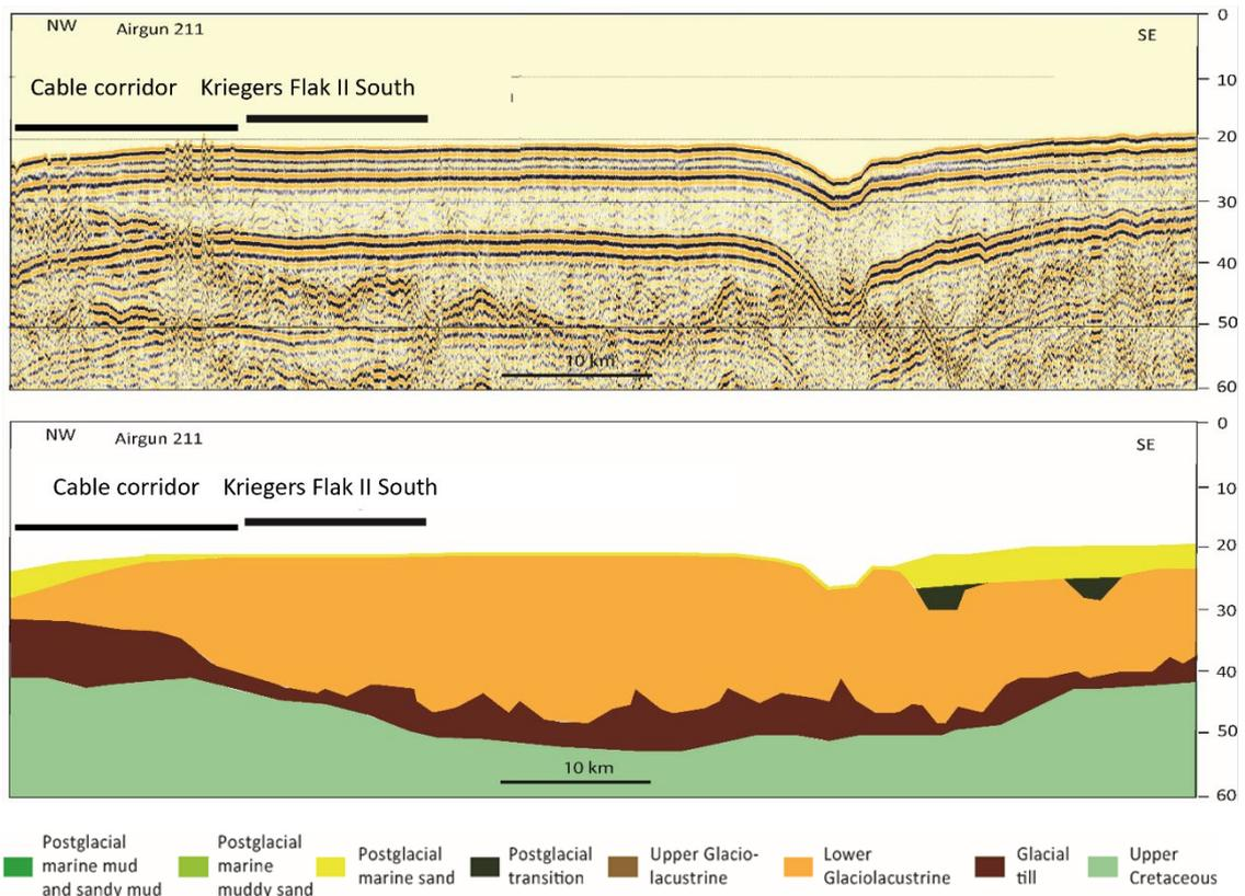
Figure 8.13 Airgun profile 211 and geological interpretation. For location, see Figure 8.4.
