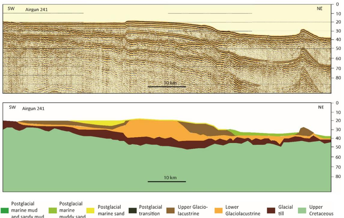
Figure 8.11 Airgun profile 241 and geological interpretation. For location, see Figure 8.4.
