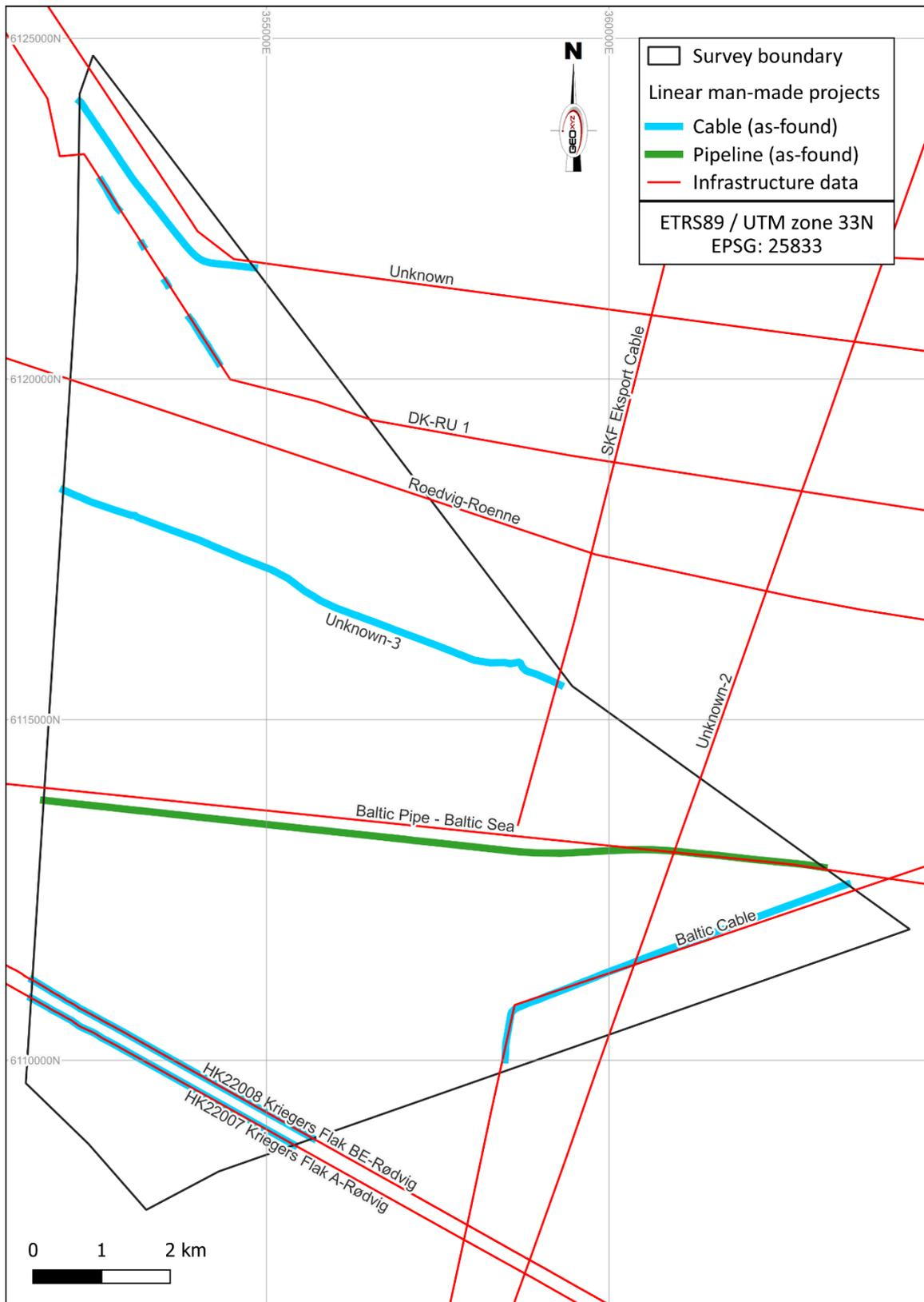
**Figure 60: A comparison of as-found cables and pipelines with existing data on their locations for the Kriegers Flak II North site**
