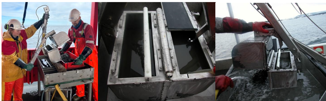
Figure 3-5. Grab sampling. Grab type used, a Van Veen type grab (collects sediments for 0.1 m 2 samples of macrofauna and 0.05 m 2 for sediment chemistry and grain size analyses).
