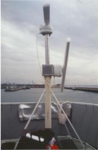
Figure 5-4 Horizontal and vertical radar mounted on a research vessel.
