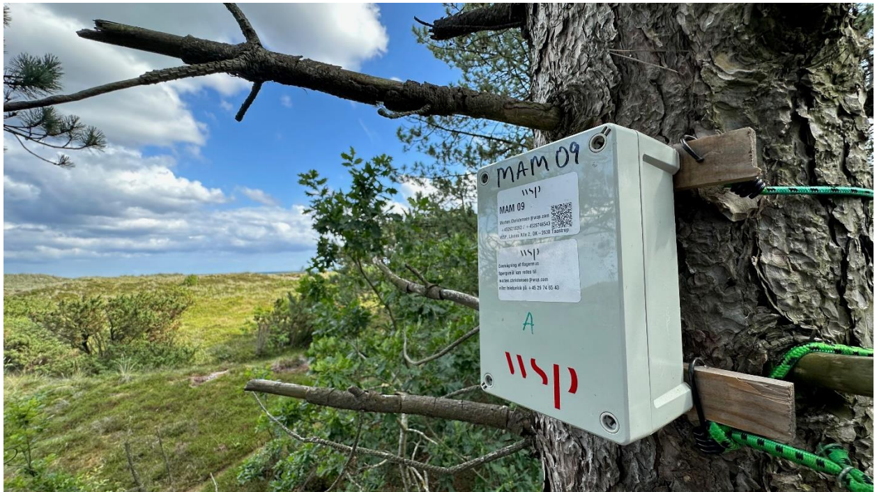
Figure 10 – Bat detector mounted on a pine tree near the coast south of Grenå (Djursland)
