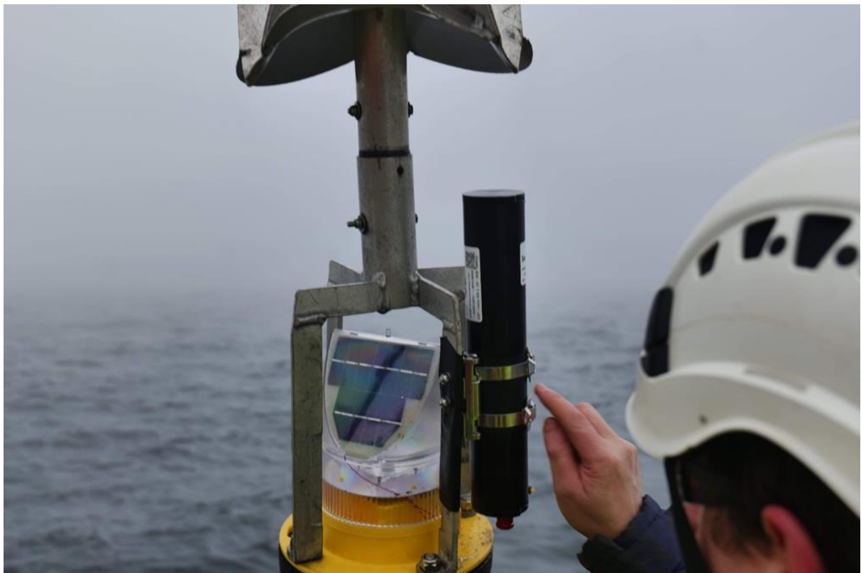
Figure 6 - Automatic bat detector mounted on a buoy used for the C-POD station in the marine mammal survey.
