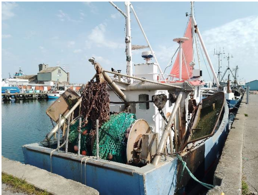
Figure 4-8. A lobster trawl in Grenå harbour. Note two trawl drums, trawl bucket, and chain block to which the two trawls are connected. Source: Krog Consult, 2024.
