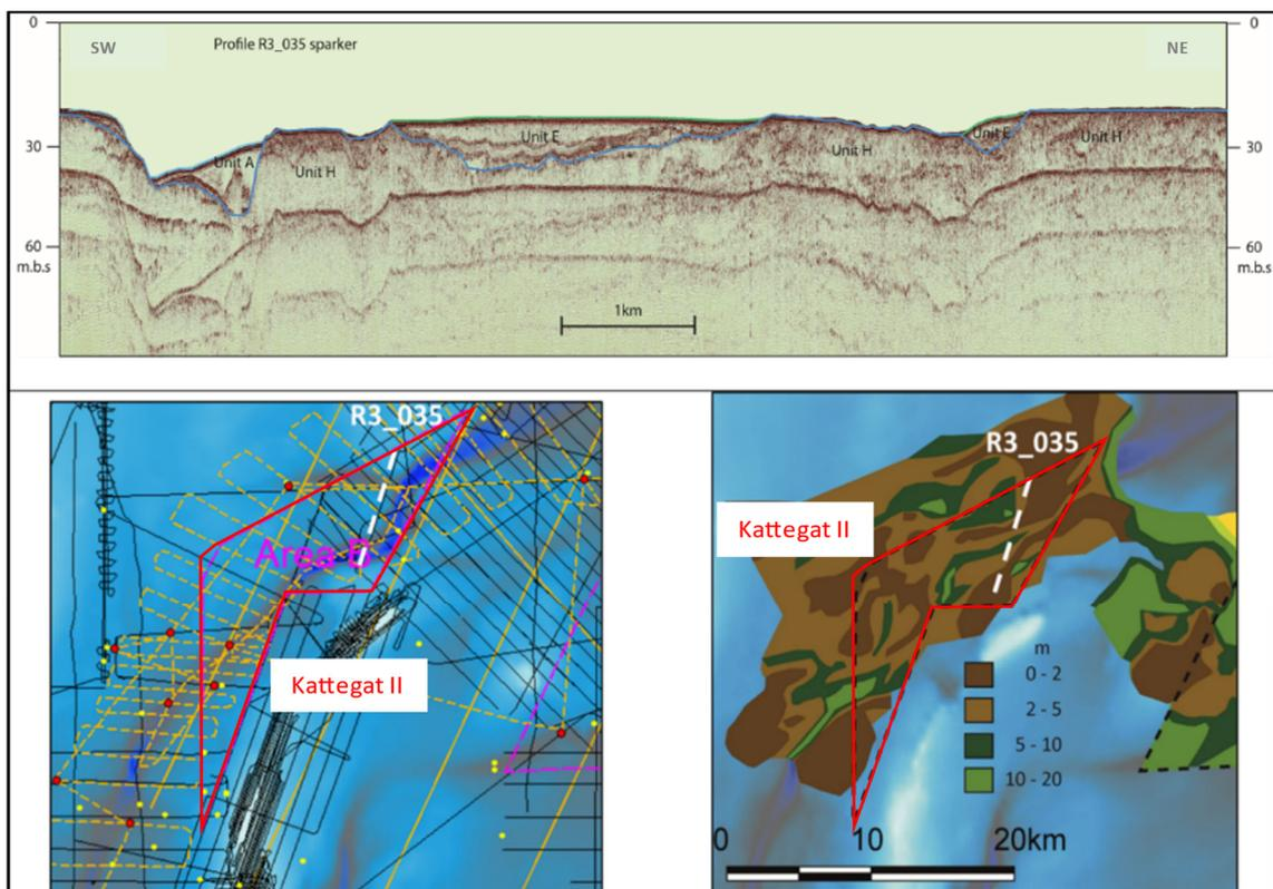
Figure 9.1 Southwest to northeast Sparker profile R3\_035 with location in relation to the seismic archive data grid (black lines are Sparker data) and the geotechnical soft sediment thickness map.
