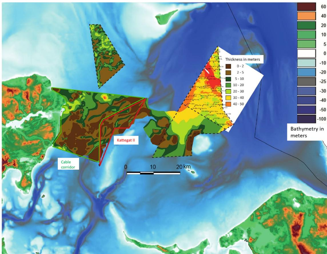
Figure 12.1 Thickness of geotechnical soft sediments in the southern Kattegat. The Kattegat II OWF area and cable corridor is shown in red and green together with the existing Anholt OWF and OWF areas covered in previous screening reports (black hatched lines).
