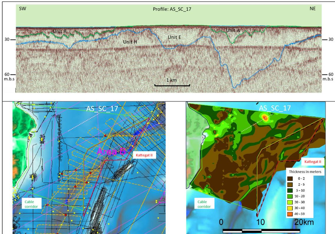
Figure 9.7 Southwest to northeast Sparker profile AS\_SC\_17 with location in relation to the Sparker seismic archive data (black lines are archive Sparker data, yellow lines Parasound data and purple lines are new Sparker data) and the geotechnical soft sediment thickness map.
