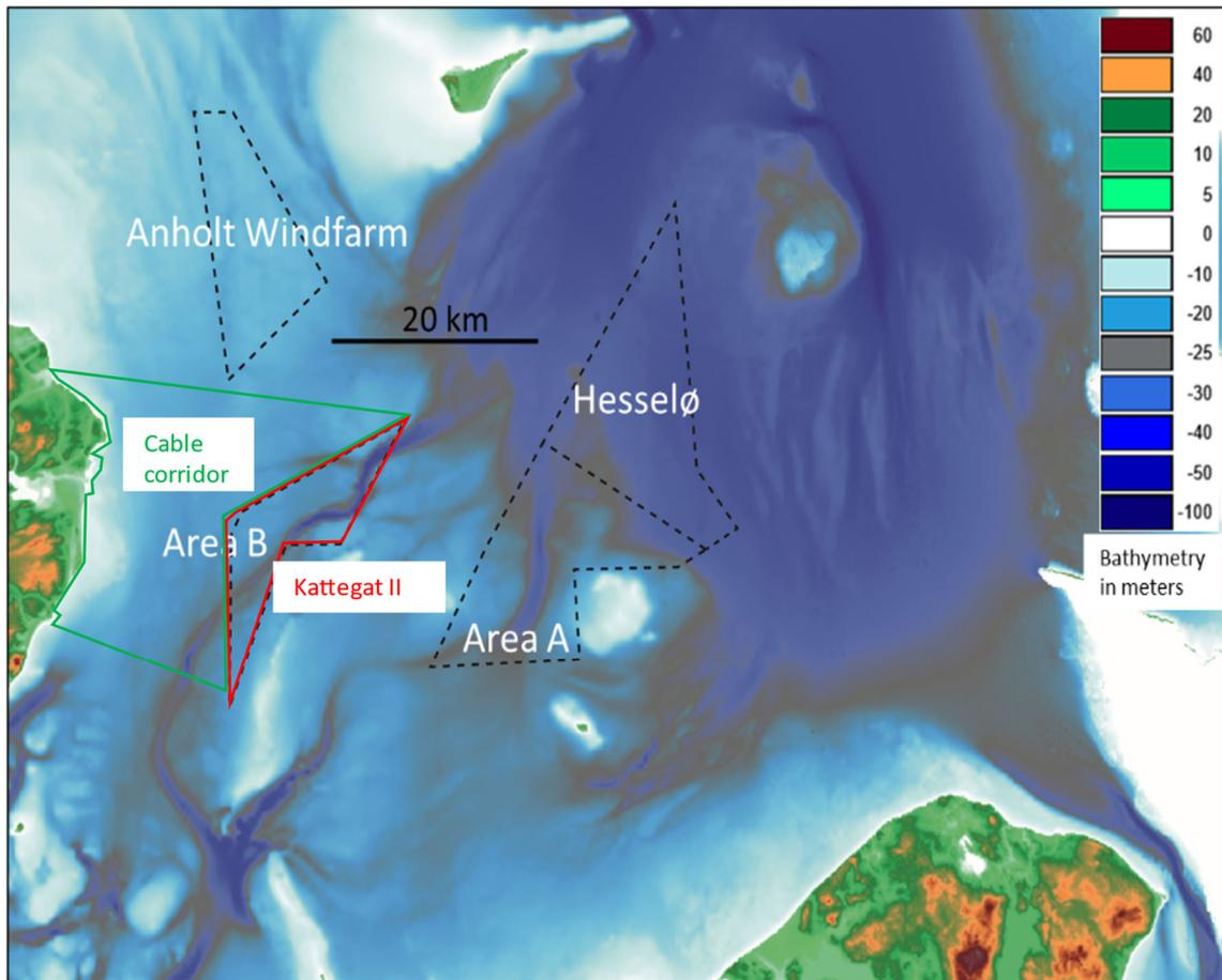
Figure 5.9 Southern Kattegat bathymetry. The Kattegat II OWF area and cable corridor is shown in red and green together with the existing Anholt OWF and OWF areas covered in previous screening reports (black hatched lines). Bathymetry from [www.emodnet-bathymetry.eu](http://www.emodnet-bathymetry.eu).
