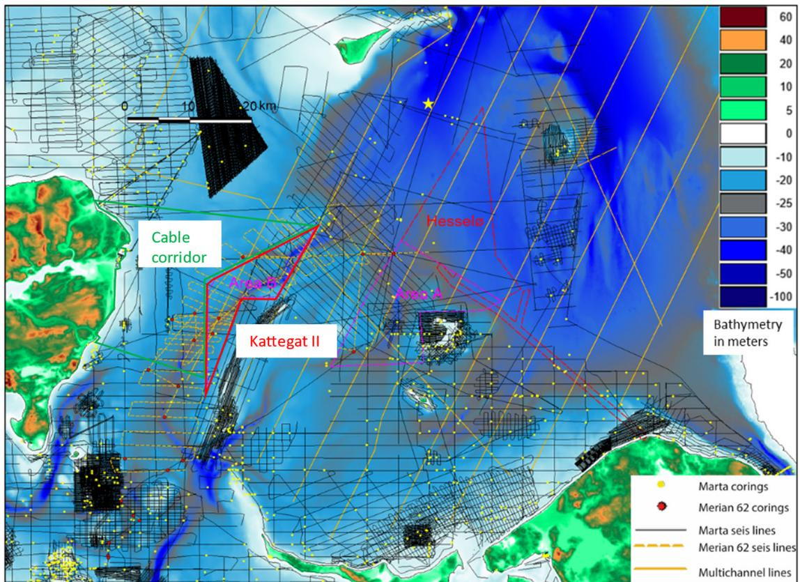
Figure 4.1. Distribution of Marta database seismic grid and core data in the southern and central Kattegat region. The Kattegat II OWF area and cable corridor is shown in red and green together with the existing Anholt OWF and OWF areas covered in previous screening reports (purple and red hatched lines). Bathymetry from [www.emodnet-bathymetry.eu](http://www.emodnet-bathymetry.eu).
