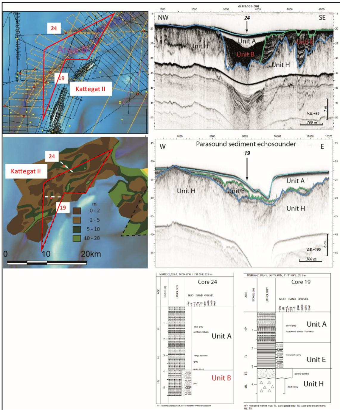
Figure 9.3 Parasound echosounder profiles from the northern and central parts of the Kattegat II OWF area with location in relation to the seismic archive data grid (yellow lines are Parasound data). The position of the seismic examples and vibrocores 24 and 19 are indicated on the geotechnical soft sediment thickness map. Core descriptions with indication of seismic units are seen in the lower right of the figure.
