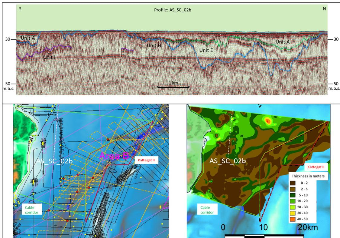
Figure 9.6 South to north Sparker profile AS\_SC\_02b with location in relation to the Sparker seismic archive data (black lines are archive Sparker data, yellow lines Parasound data and purple lines are new Sparker data) and the geotechnical soft sediment thickness map.
