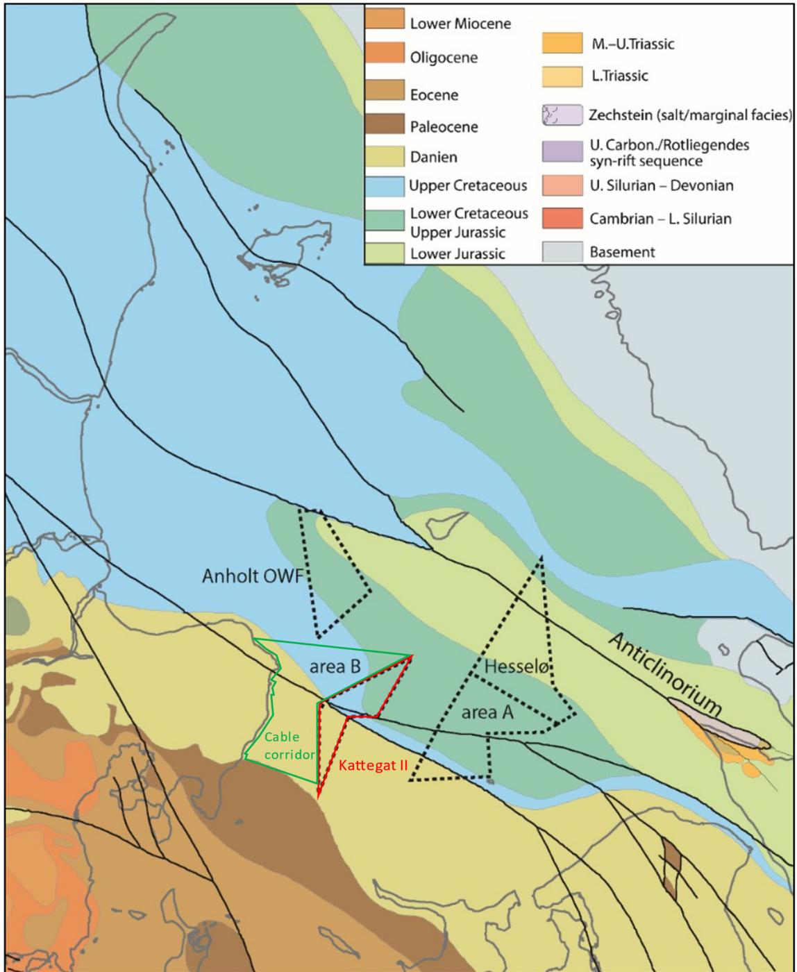
Figure 5.2. Pre-Quaternary surface geology and major faults in the Kattegat. The location of the Kattegat II OWF area and cable corridor is shown in red and green together with the existing Anholt OWF and OWF areas covered in previous screening reports (black hatched lines).
