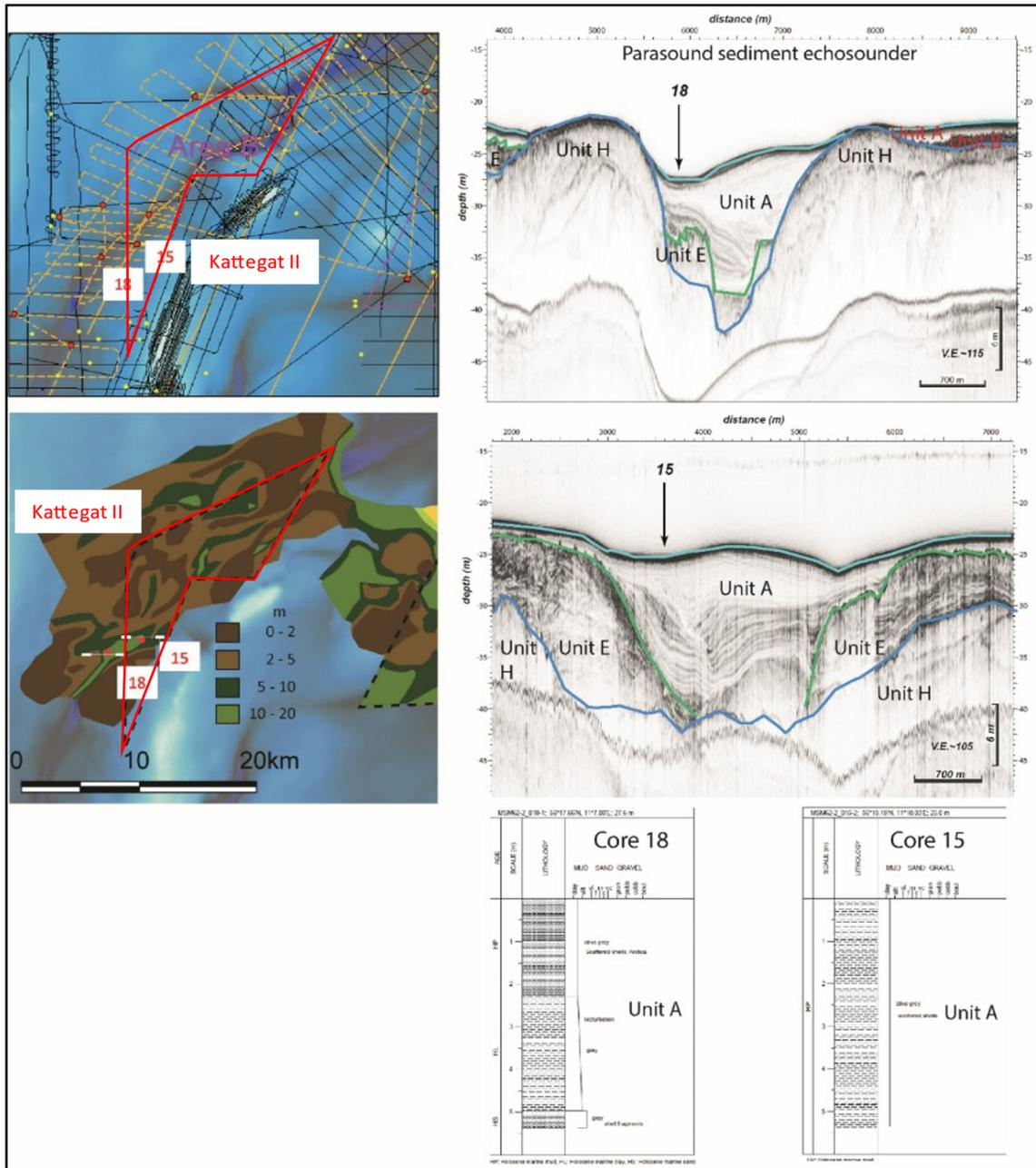
Figure 9.5 Parasound echosounder profiles from the southern part of the Kattegat II OWF area, with location in relation to the seismic archive data grid (yellow lines are Parasound data). The positions of the seismic profiles and vibrocores 18 and 15 are indicated on the geotechnical soft sediment thickness map. Core descriptions with indication of seismic units are shown below the seismic profiles.
