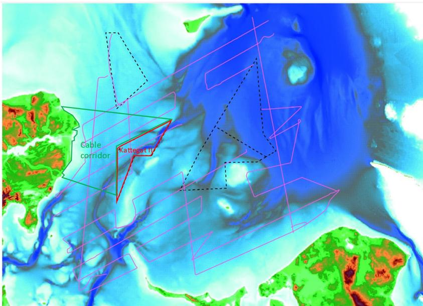
Figure 4.2 New and unpublished seismic data (in purple) used in the present study. The data are from investigations for the Danish Energy Agency as part of a geological screening for offshore wind of the Danish Sea area. The location of the Kattegat II OWF area and cable corridor is shown in red and green together with the existing Anholt OWF and OWF areas covered in previous screening reports (black hatched lines).
