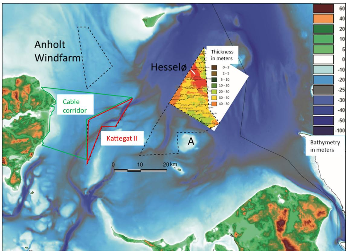
Figure 8.1 Detailed mapping of geotechnical soft sediments in the previous Hesselø OWF area. The Kattegat II OWF area and cable corridor is shown in red and green together with the existing Anholt OWF and OWF areas covered in previous screening reports (black hatched lines).
