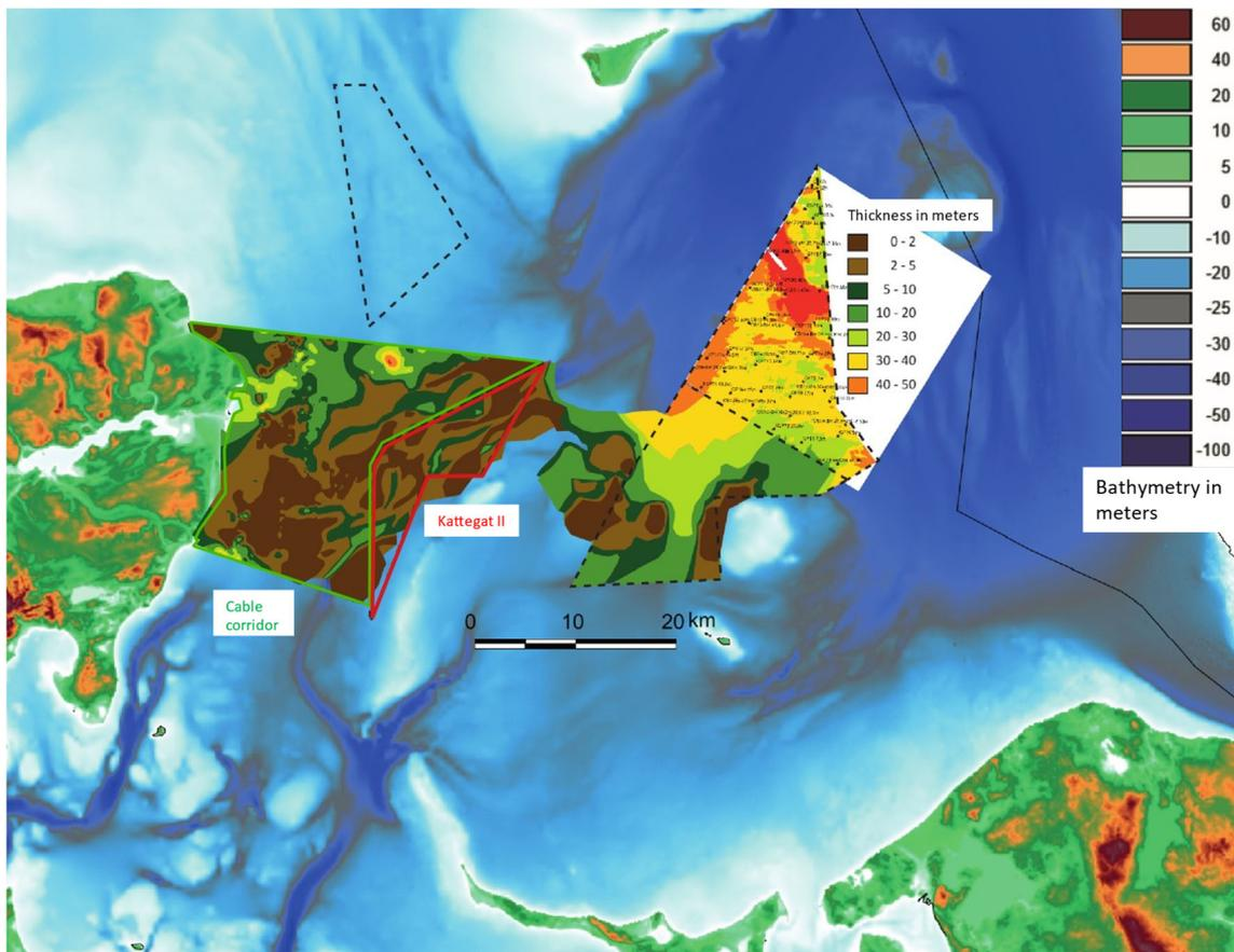
Figure 9.9 General thickness of geotechnical soft sediments (combined thickness of seismic Units A–E/F) in the current Kattegat II OWF area compared with the detailed mapping of the previous Hesselø OWF area. The Kattegat II OWF area and cable route is shown in red and green together with the existing Anholt OWF and OWF areas covered in previous screening reports (black hatched lines).
