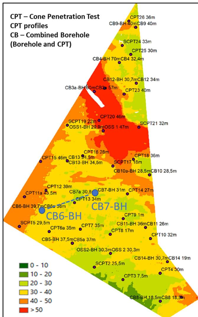
Figure 7.3 Thickness of geotechnical soft sediments (thickness of Unit A–E/F Seismic data) in the previous Hesselø OWF area. Point data show thickness of soft sediments (CPT and boreholes). There is generally a good correlation between the data sets. Local areas without correlation could be related to glacial disturbance of Unit E/(F). Figure from Energinet (2021).
