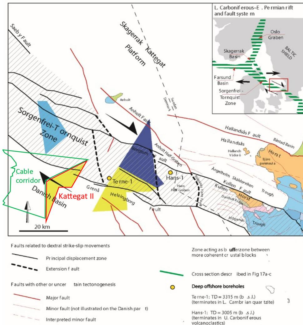
Figure 5.1. Regional structures in the southern part of the Kattegat (Erlström & Sivhed 2001). The location of the Kattegat II OWF area and cable corridor is shown in red and green together with the existing Anholt OWF (light blue) and OWF areas covered in previous screening reports (yellow and dark blue).
