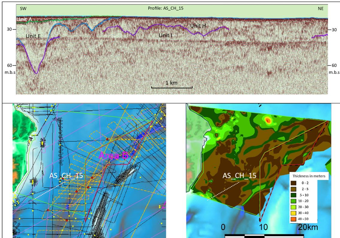
Figure 9.8 Southwest to northeast Sparker profile AS\_SC\_15 with location in relation to the Sparker seismic archive data (black lines are archive Sparker data, yellow lines Parasound data and purple lines are new Sparker data) and the geotechnical soft sediment thickness map.
