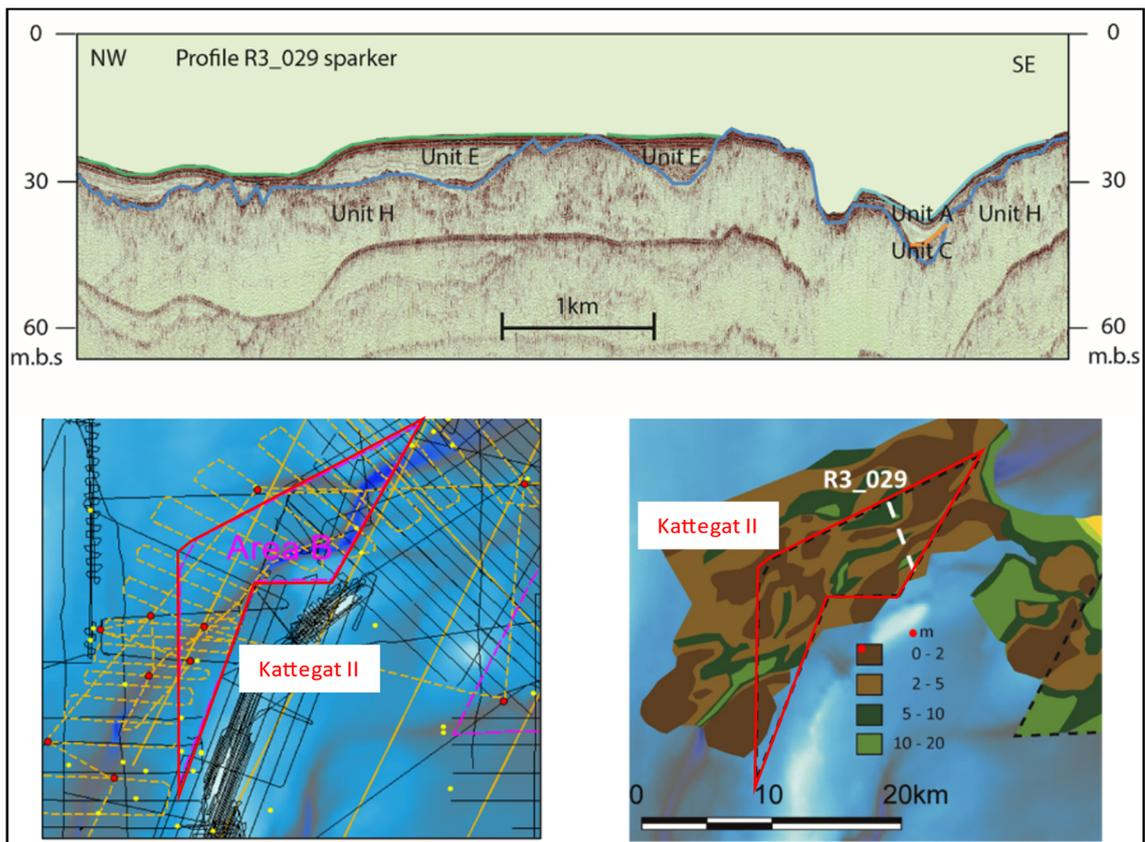
Figure 9.2 Northwest to southeast Sparker line R3\_029 with location in relation to the seismic archive data grid (black lines are Sparker data) and the geotechnical soft sediment thickness map.
