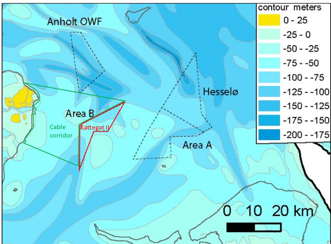
Figure 5.3. General pre-Quaternary morphology (Binzer & Stockmarr 1994). The location of the Kattegat II OWF area and cable corridor is shown in red and green together with the existing Anholt OWF and OWF areas covered in previous screening reports (black hatched lines).
