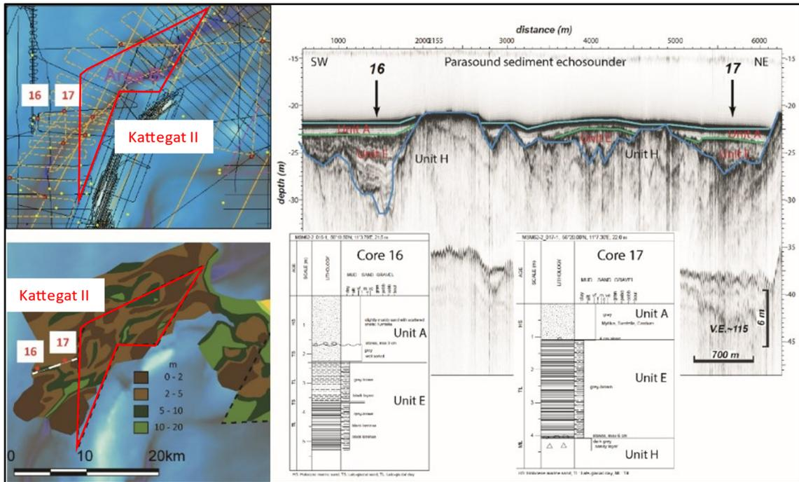
Figure 9.4 Parasound echosounder profile west of the Kattegat II OWF area, with location in relation to the seismic archive data grid (yellow lines are Parasound data). The position of the seismic example and vibrocores 16 and 17 are indicated on the geotechnical soft sediment thickness map and core descriptions with indication of seismic units are shown on the seismic profile.
