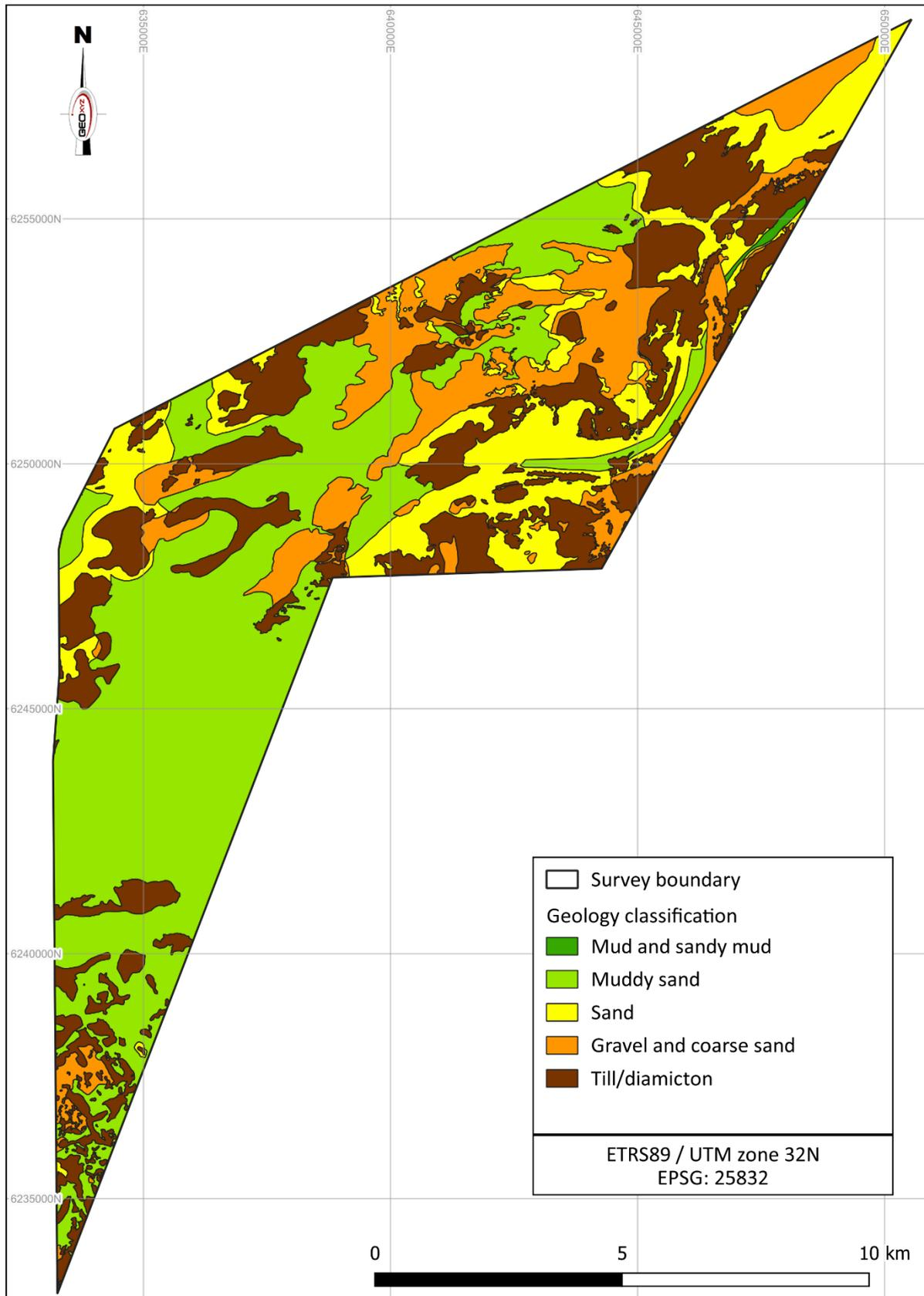
**Figure 39: Seabed surface geology classification**
