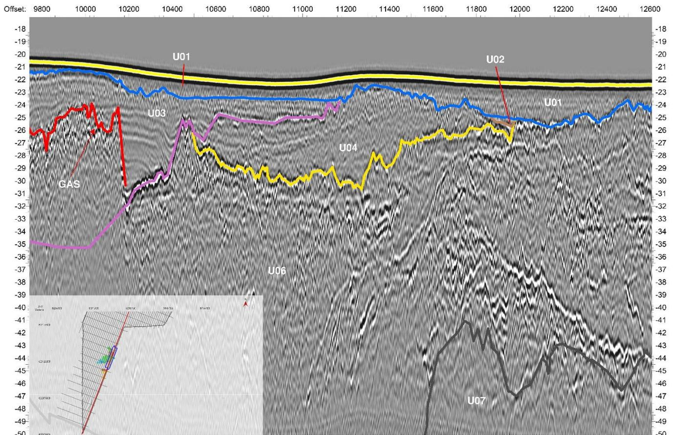
**Figure 9-11** Seismic line A\_KG\_L022\_UHR\_T\_MIG\_STK. Example of U04, in this example bounded at the top by B01 (Blue) and B03 (Purple), and at the base by B04 (Yellow). The seismic facies is seen as mostly acoustically transparent with some subparallel reflectors at the left side of the figure. The overview map in the lower left corner shows the position of the profile (red line), the displayed section (blue area), and elevation of top of U04 (see also enclosure 3.04).
