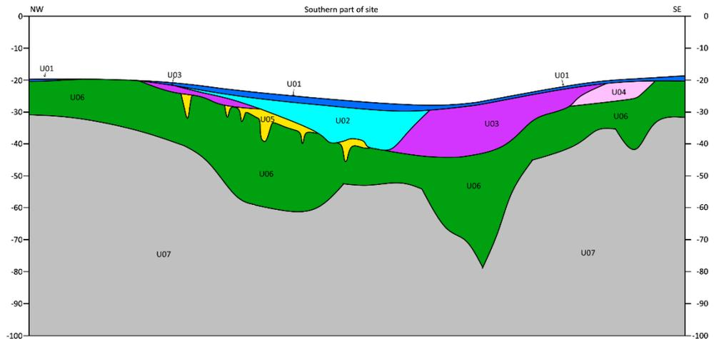
*Figure 5-2 Conceptual Geological Model cross section oriented from north-west to south-east through the southern part of the OWF project site. List of units constituting the model with assigned age and depositional environment can be found in Table 5-1.*
