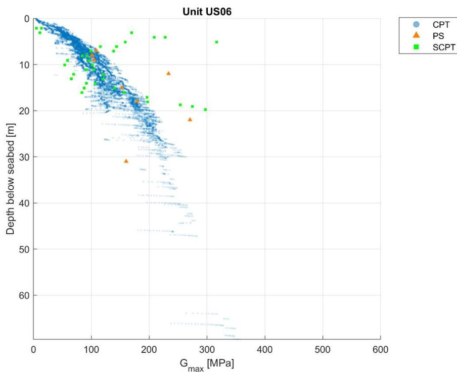
Figure 8-6 Range of  $G_{max}$  for the geotechnical unit US06.
