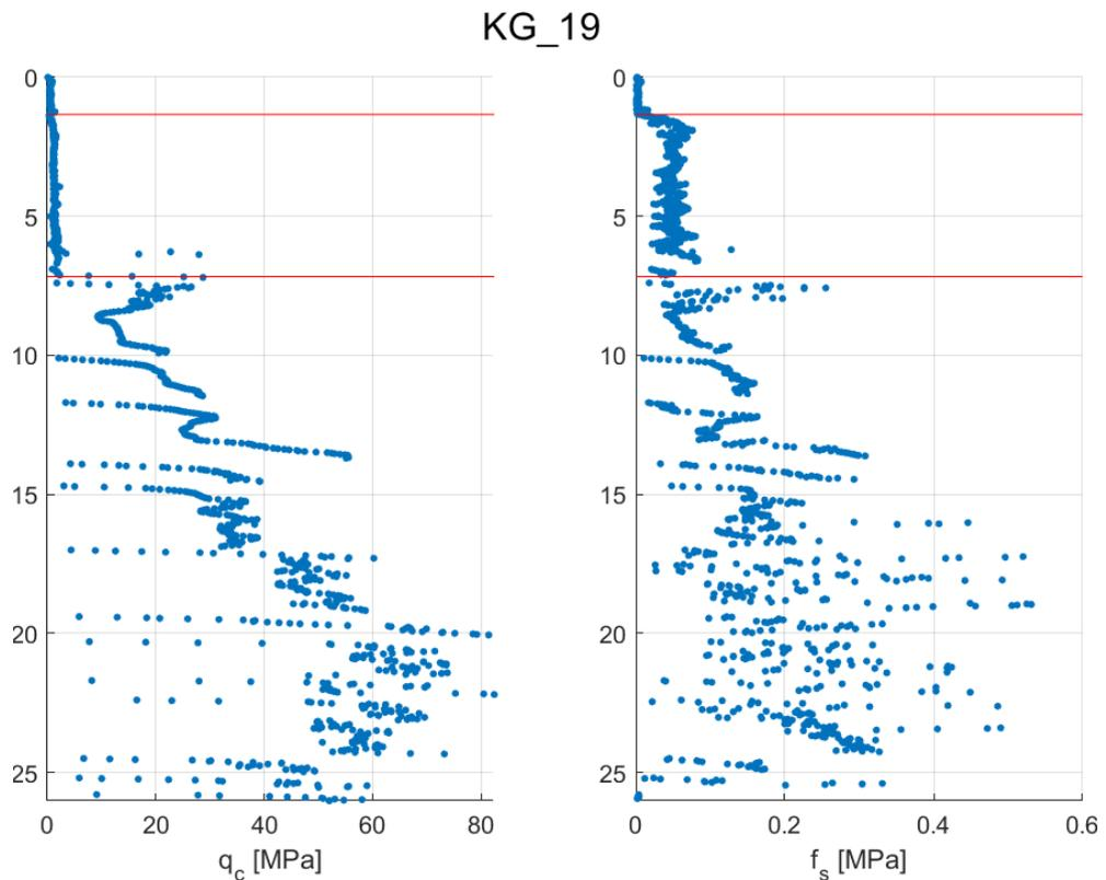
Figure 10-11  $q_c$  and  $f_s$  from CPT measurements for KG\_19 found as representative for zone VII. More information about the location can be found in Appendix A.
