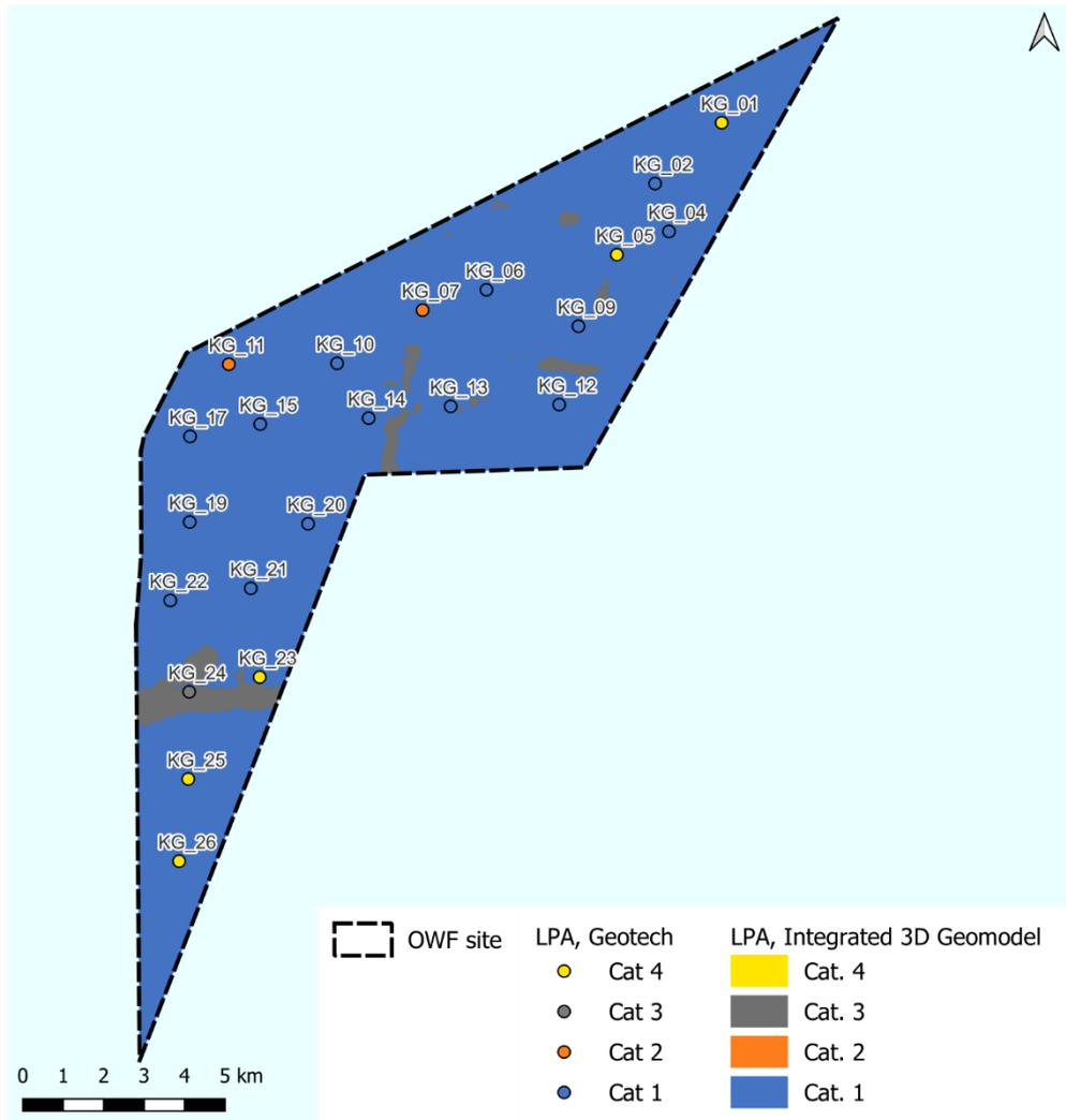
Figure 11-3 Results from leg penetration analysis for Generic O&M Vessel.
