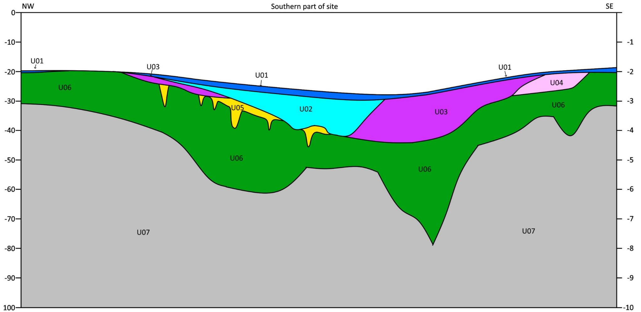
Figure G-2 Conceptual model cross section oriented from north-west to south-east through the southern part of the OWF project site.
