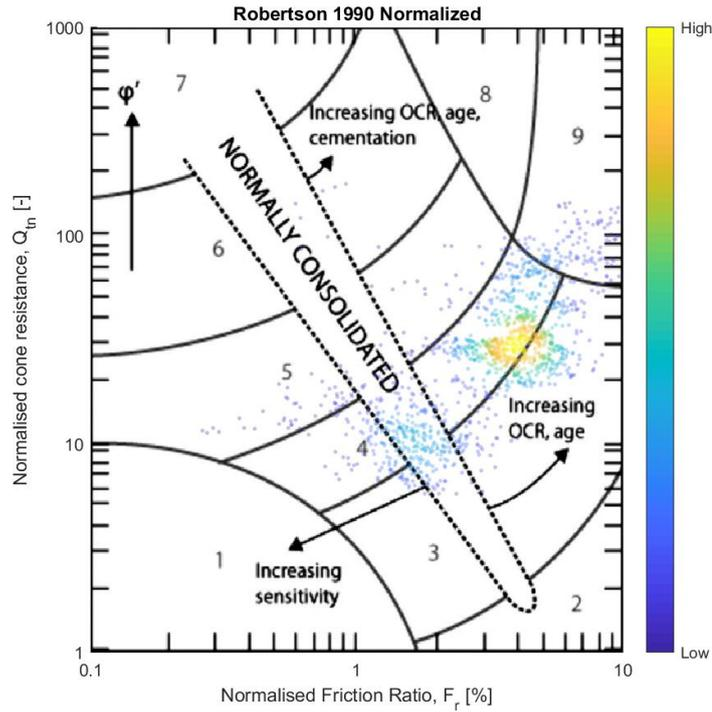
Figure 7-3 Robertson  $Q_{tn} - F_r$  classification chart for soil behaviour type plotted for all CPT survey locations for the geotechnical unit UC03.
