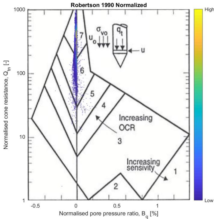
Figure 7-6 Robertson  $Q_{tn} - B_q$  classification chart for soil behaviour type plotted for all CPT survey locations for the geotechnical unit US06.
