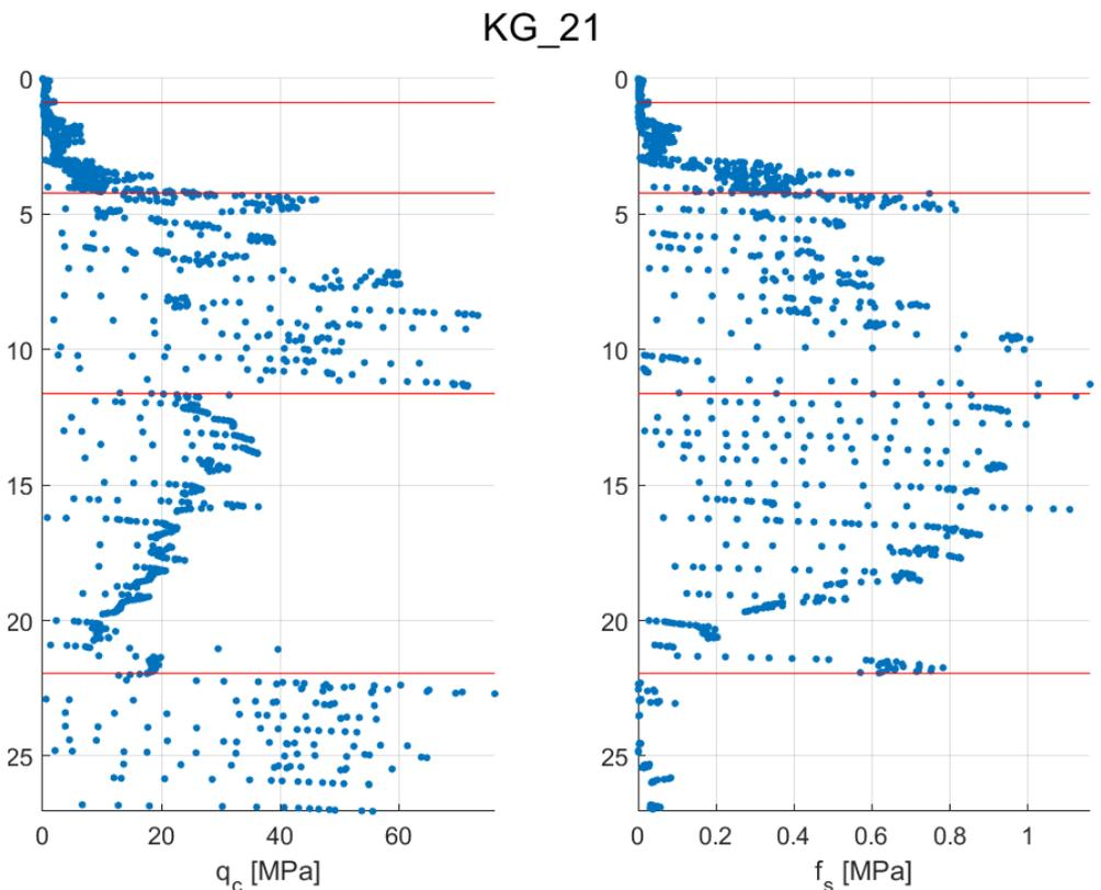
Figure 10-10  $q_c$  and  $f_s$  from CPT measurements for KG\_21 found as representative for zone V. More information about the location can be found in Appendix A.
