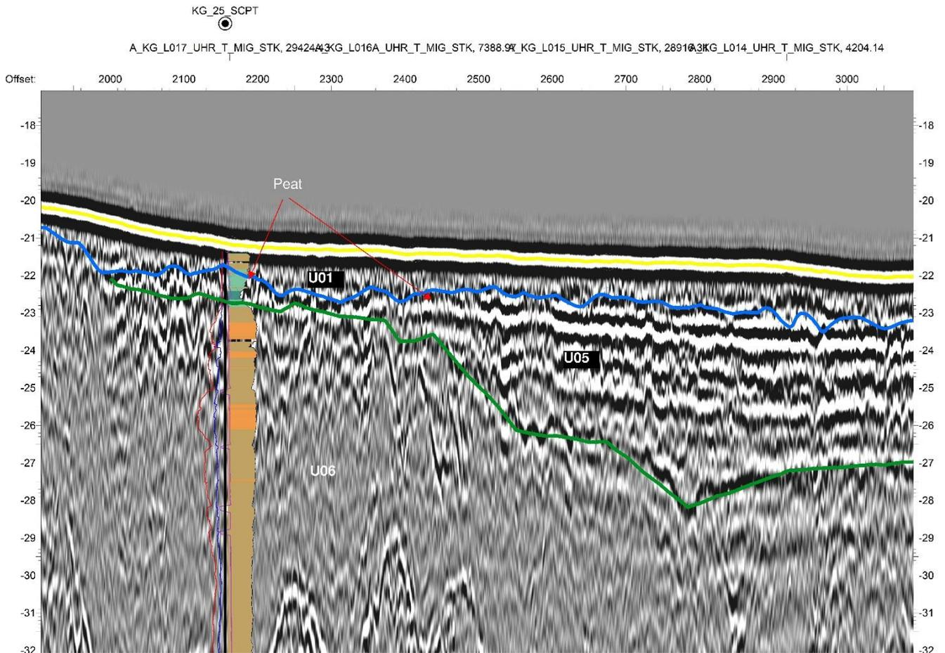
Figure 9-4 Seismic line A\_KG\_X007\_UHR\_T\_MIG\_STK. Example of KG\_25\_SCPT where peat was found in layers in the upper 1.5 m. In the seismic profile the peat is seen as a layer of high amplitude reflections and is interpreted as marking the Holocene transgression into a marine environment.
