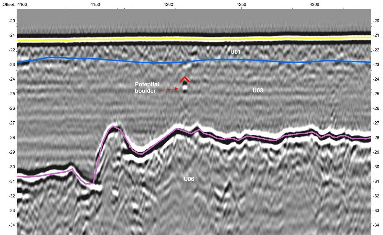
Figure 9-6 Seismic line A\_KG\_X010\_UHR\_T\_MIG\_STK. Example of a hard kick in U03 interpreted as a potential boulder.
