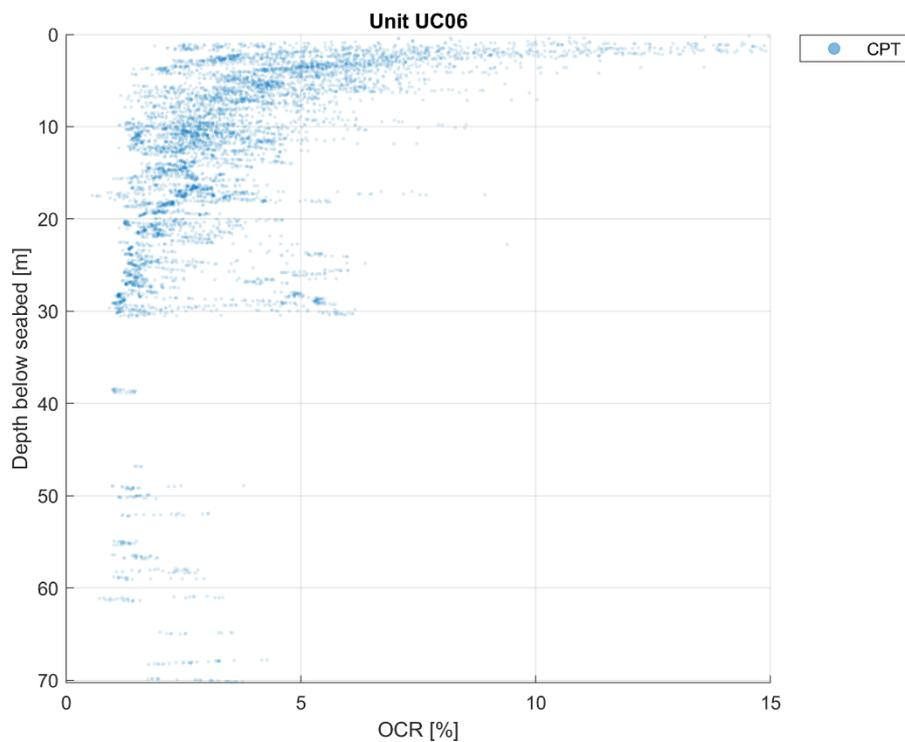
Figure 8-2 Range of OCR for geotechnical unit UC06.
