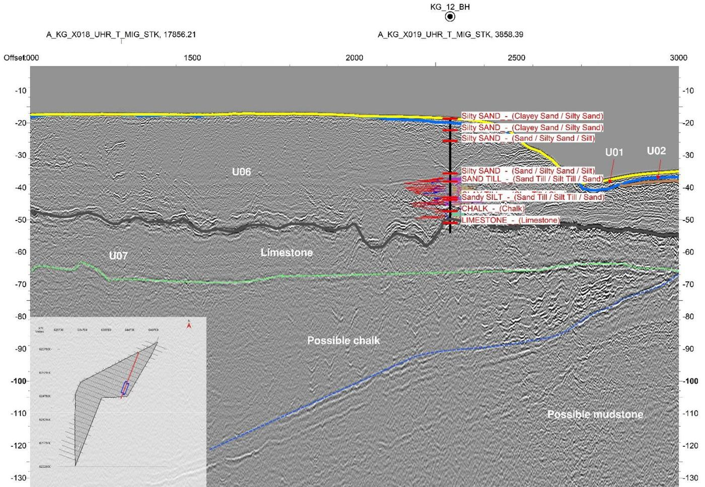
Figure 9-17 Seismic line A\_KG\_L038\_UHR\_T\_MIG\_STK. Example of an angular unconformity seen in the bedrock due to tectonic uplift and erosion. Proposed boundaries between limestone, chalk and mudstone are drawn. These boundaries are not verified by geotechnical data (KG\_12) and are not mapped in the Kattegat OWF IGM, but are all included in U07. The overview map in the lower left corner shows the position of the profile (red line) and the displayed section (blue area).
