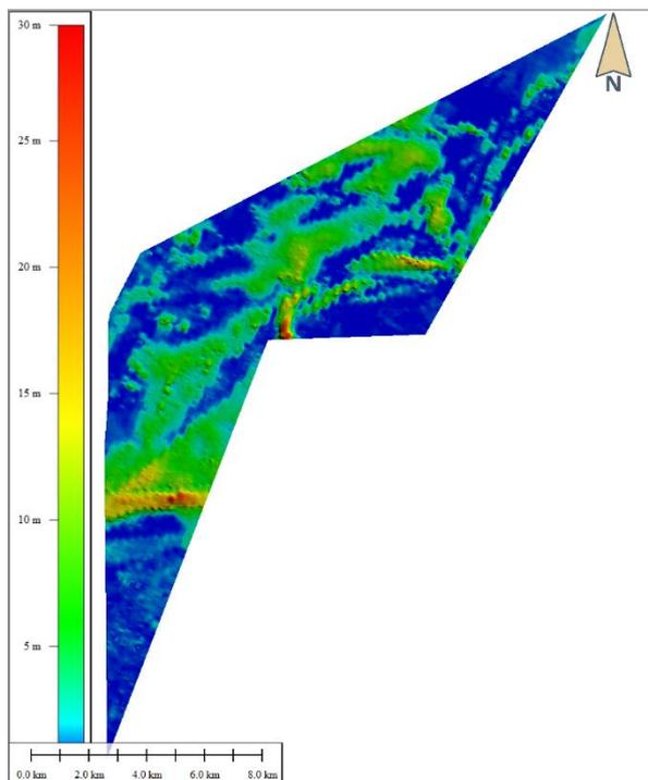
Figure 10-2 Combined thickness of soft sediments derived from units U01, U02, U03 and U04.
