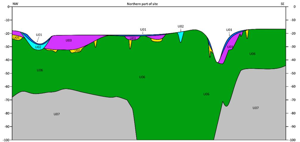
*Figure 5-1 Conceptual Geological Model cross section oriented from north-west to south-east through the northern part of the OWF project site. List of units constituting the model with assigned age and depositional environment can be found in Table 5-1.*
