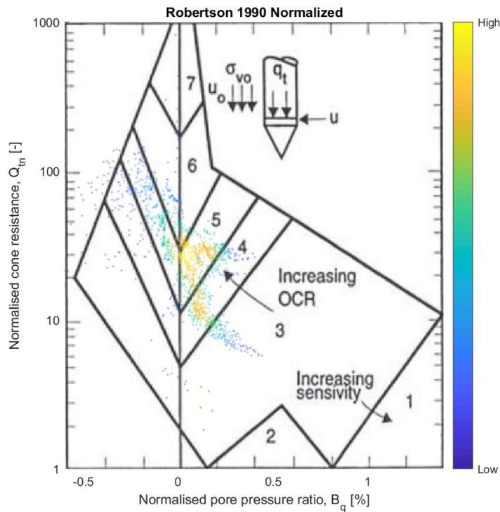
Figure 7-4 Robertson  $Q_{tn} - B_q$  classification chart for soil behaviour type plotted for all CPT survey locations for the geotechnical unit UC03.
