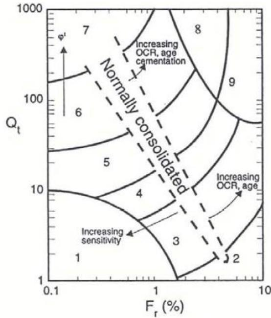
Figure 7-1 Robertson  $Q_t - F_r$  classification chart for soil behaviour type, cf. Ref. /2/. As recommended in Ref. /2/ the normalised cone resistance ( $Q_{tn}$ ) is considered instead of  $Q_t$  when evaluating the soil behaviour type.
