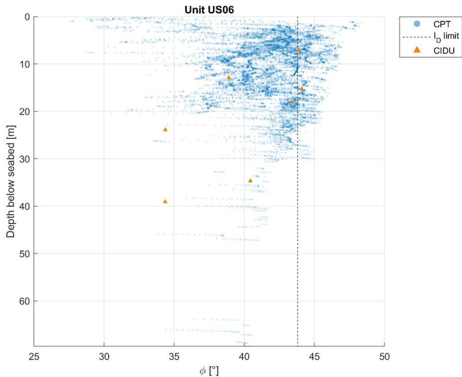
Figure 8-4 Range of  $\varphi'$  for geotechnical unit US06.
