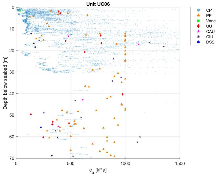
Figure 8-5 Range of  $c_u$  for the geotechnical clay unit UC06 using CPT correlation (blue dots) and laboratory test results.
