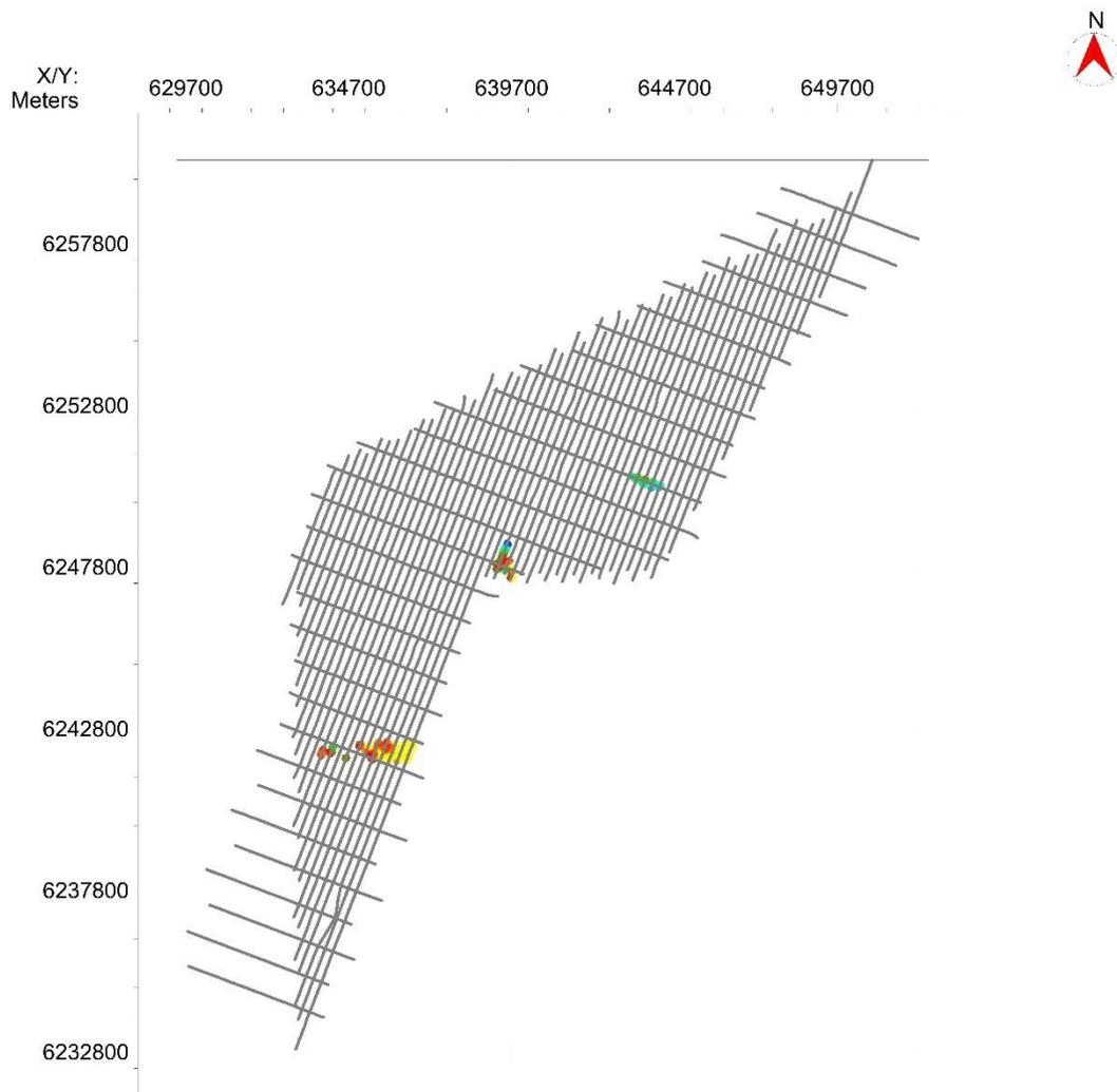
Figure 9-2 Extend of shallow gas found in Kattegat OWF area.
