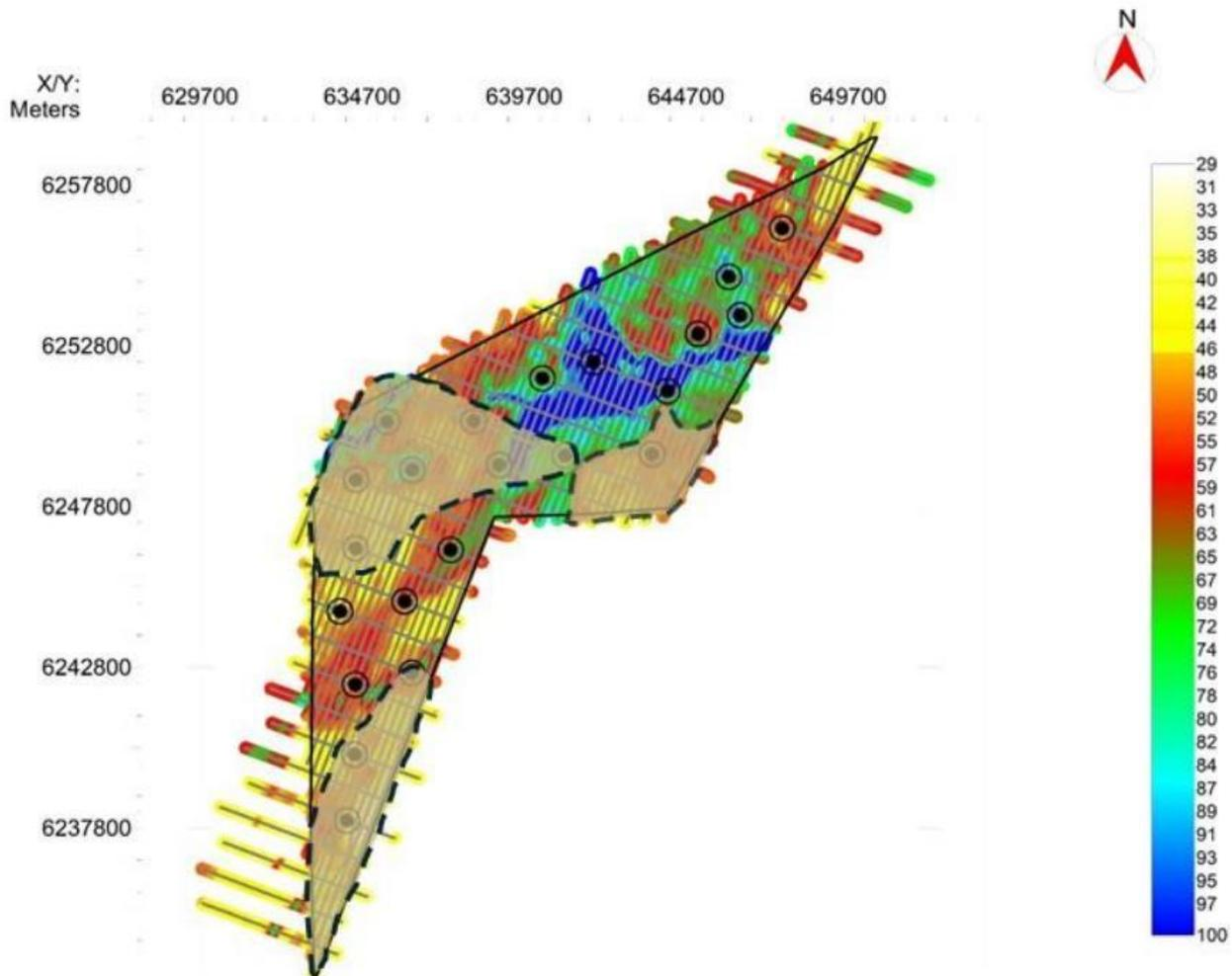
Figure 9-14 Map showing areas of U06 where a sandy top is found in the geotechnical data for the unit generally described as TILL. The beige areas marked by a stippled line are the areas where sand is found in the top of the unit. The thickness of the sand varies from a few meters up to approximately 20 m. The base of the unit is shown in elevation to MSL.
