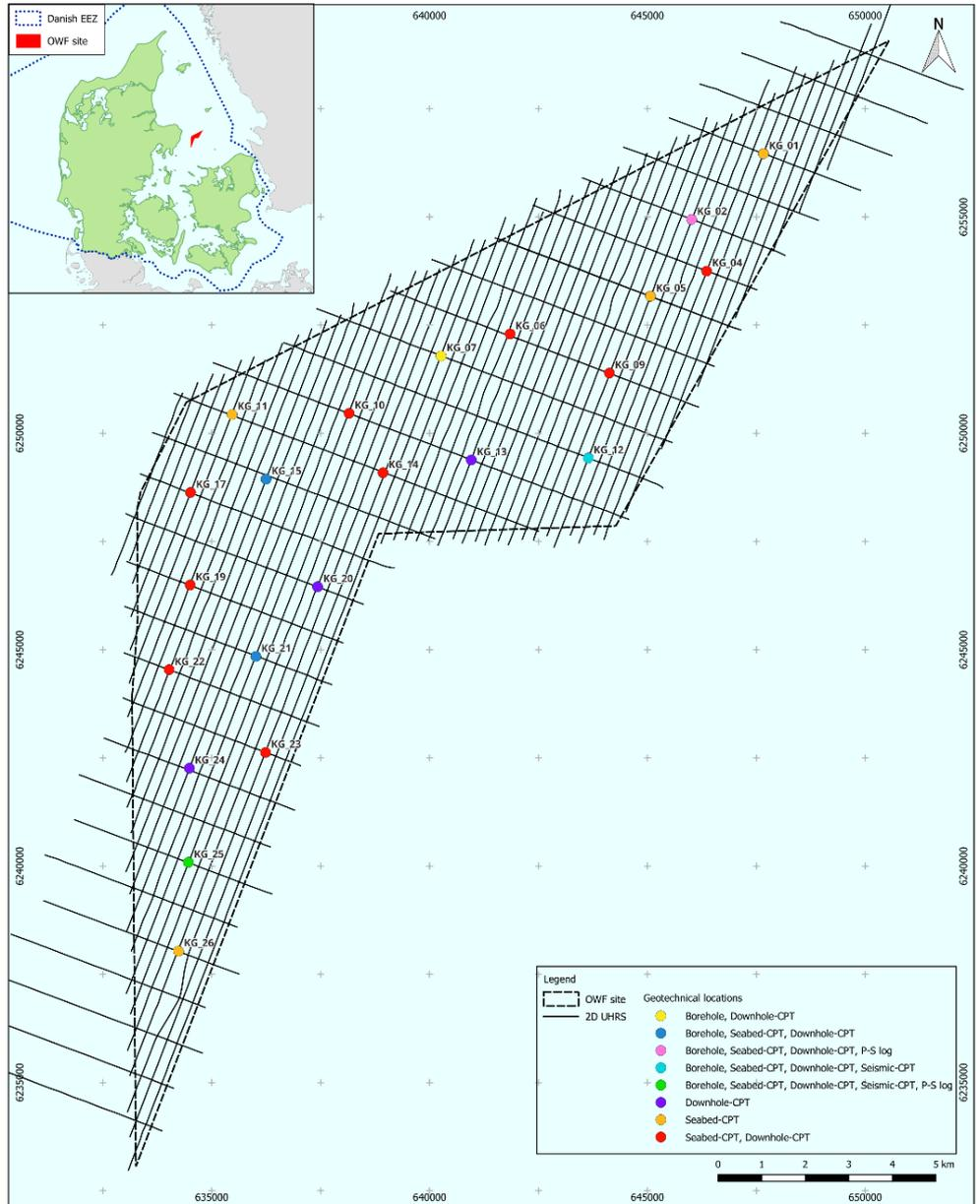
Figure 3-1 Overview map of the Kattegat OWF project site with locations for the 2D UHRS seismic lines and geotechnical data (borehole, CPT and P-S log).
