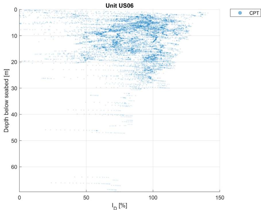
Figure 8-3 Range of estimated  $I_D$  using CPT correlations for geotechnical unit US06.
