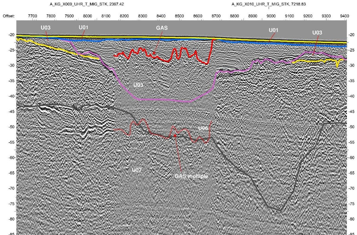
Figure 9-3 Seismic line A\_KG\_L020\_UHR\_T\_MIG\_STK: Example of shallow gas (red) in U03, which is both seen to create a zone of seismic masking below as well as a gas multiple.
