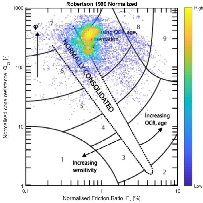
Figure 7-5 Robertson  $Q_{tn} - F_r$  classification chart for soil behaviour type plotted for all CPT survey locations for the geotechnical unit US06.
