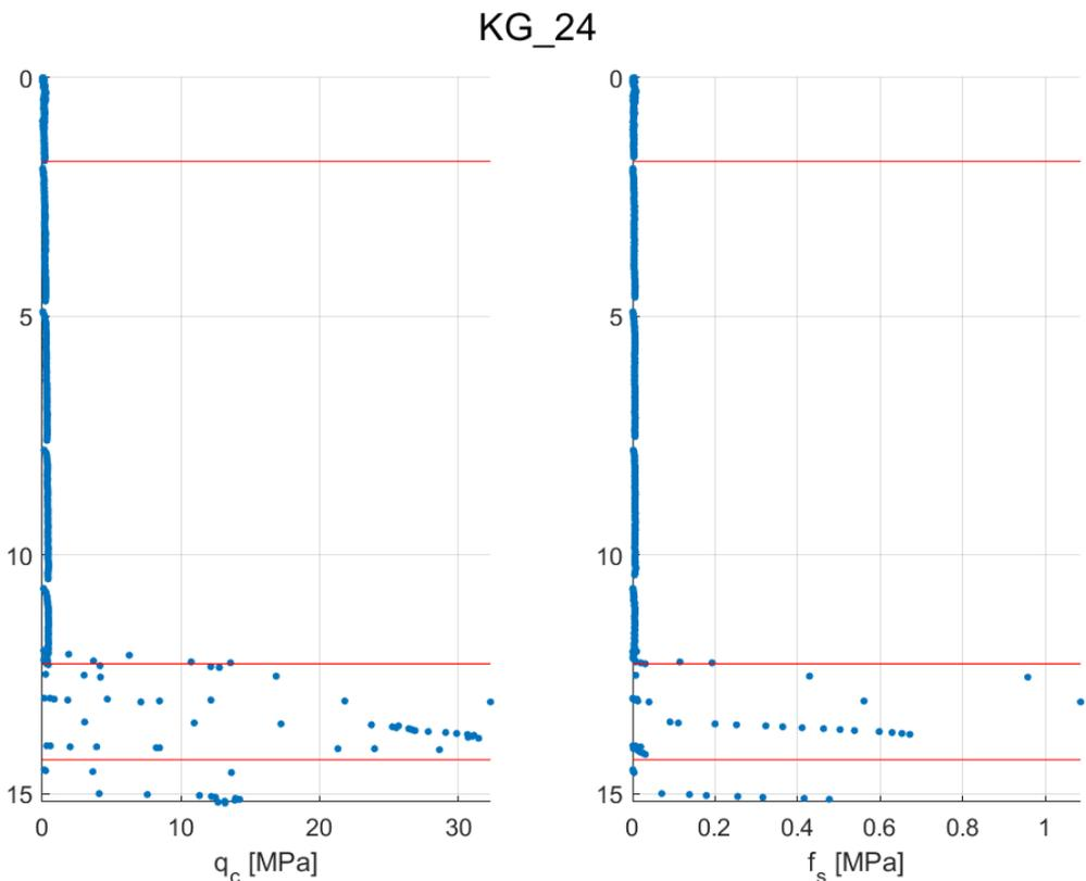
Figure 10-12  $q_c$  and  $f_s$  from CPT measurements for KG\_24 found as representative for zone VIII. More information about the location can be found in Appendix A.
