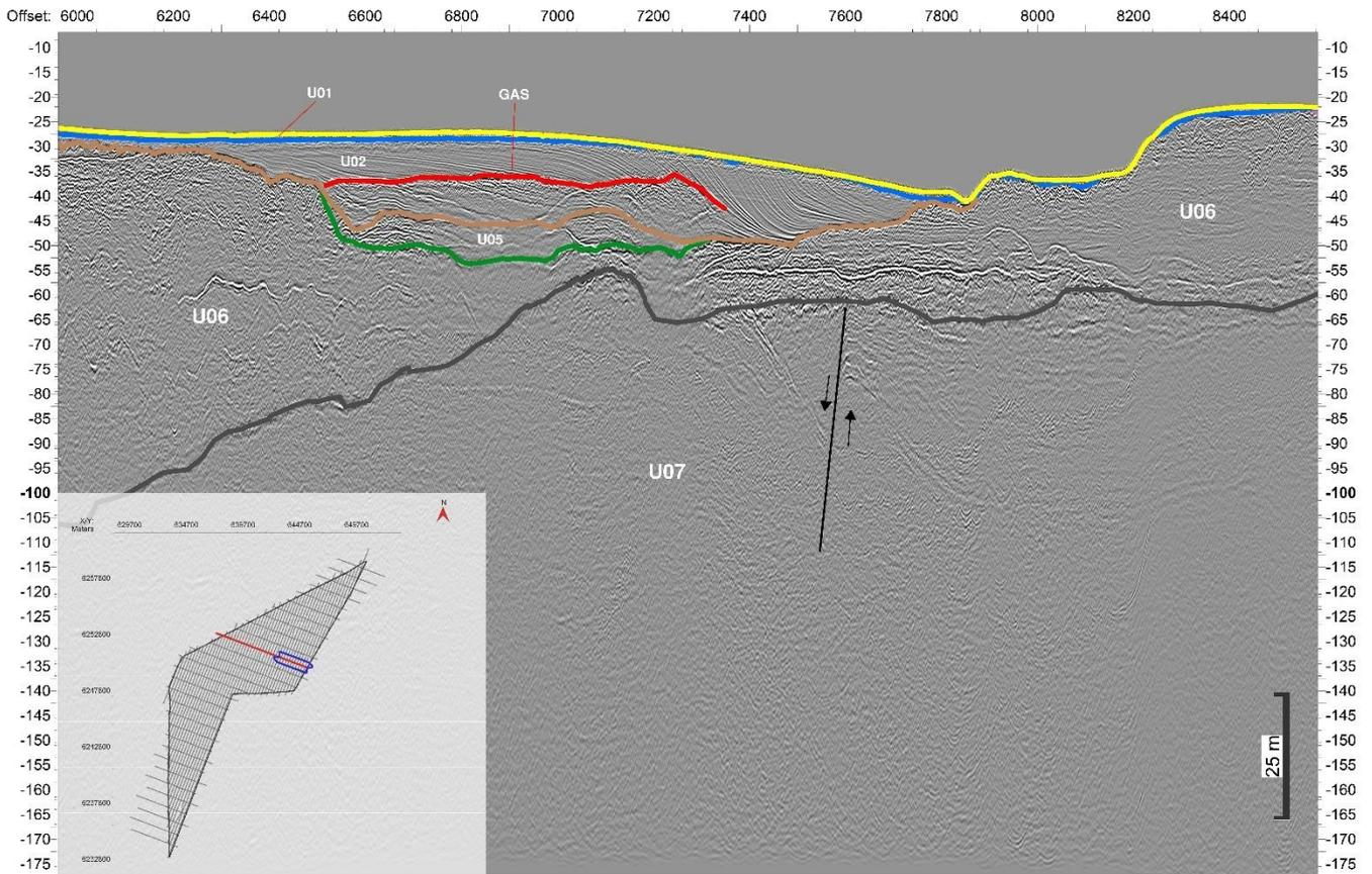
Figure 9-5 Seismic line A\_KG\_X020\_UHR\_T\_MIG\_STK. Example of a fault identified in U07.
