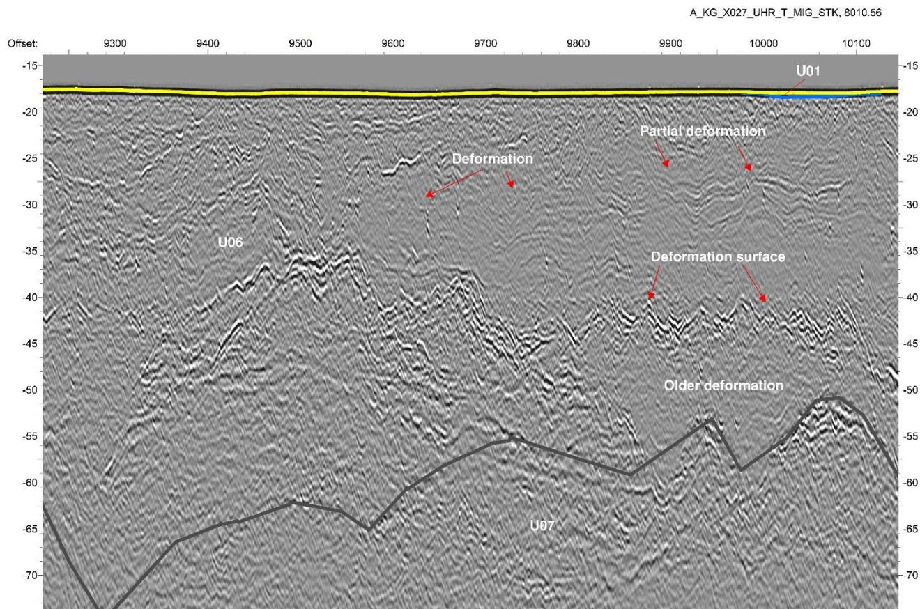
Figure 9-7 Seismic line A\_KG\_L037\_UHR\_T\_MIG\_STK. Example of a profile showing U06 where different grades and generations of glacial deformation are seen.
