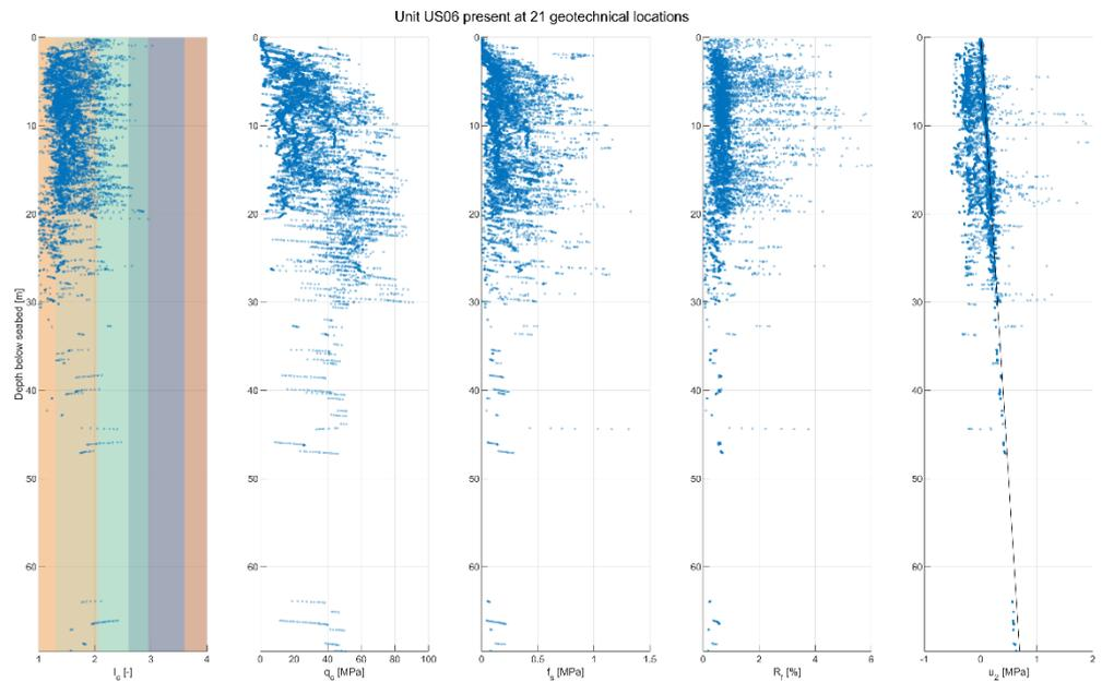
Figure 8-1 Range of CPT parameters for geotechnical unit US06.
