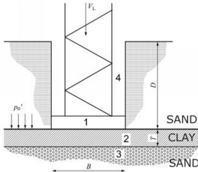
Figure 11-1 Sketch illustrating relevant parameters regarding squeezing, Ref. /12/.
