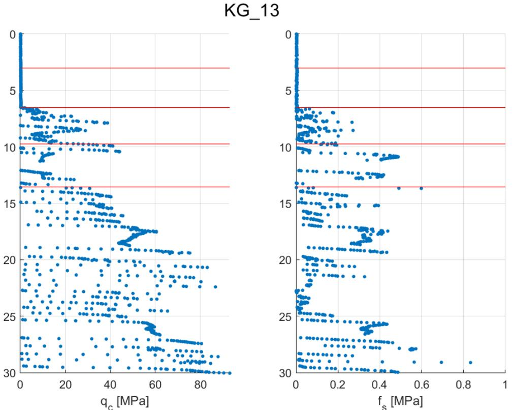
Figure 10-8  $q_c$  and  $f_s$  from CPT measurements for KG\_13 found as representative for zone II. More information about the location can be found in Appendix A.
