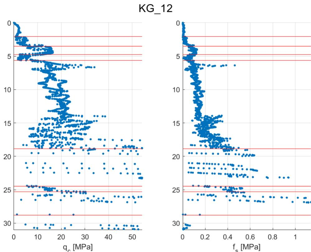
Figure 10-9  $q_c$  and  $f_s$  from CPT measurements for KG\_12 found as representative for zone IV. More information about the location can be found in Appendix A.
