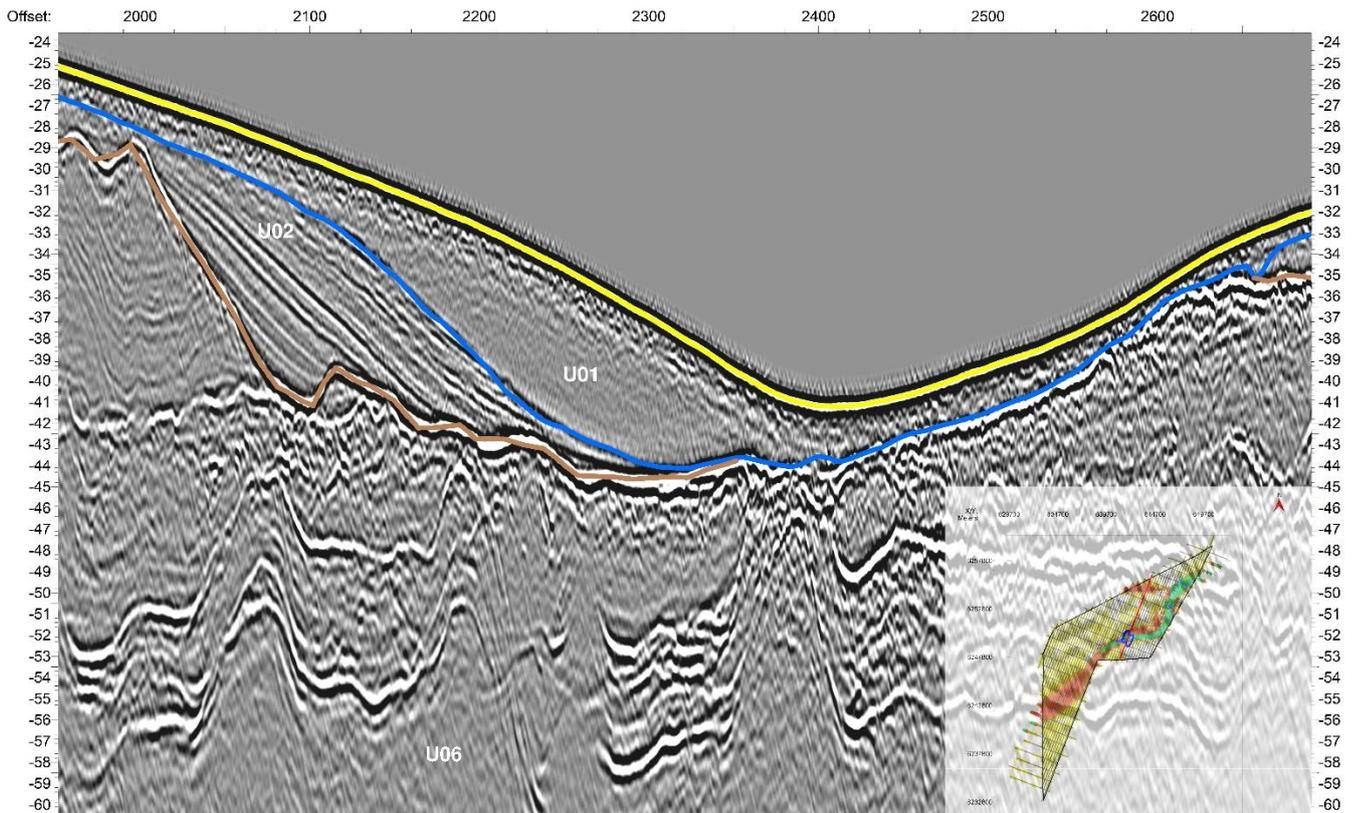
Figure 9-8 Seismic line A\_KG\_L031\_UHR\_T\_MIG\_STK. Example of U01, in this example seen bounded by B01 (Blue) at the base and the Seafloor (yellow) to the top. The seismic facies is mostly identified as being transparent with a disturbed upper part caused by seabed artefacts. The overview map in the lower right corner shows the position of the profile (red line), the displayed section (blue area), and the elevation of top of U01 (see also enclosure 3.01).
