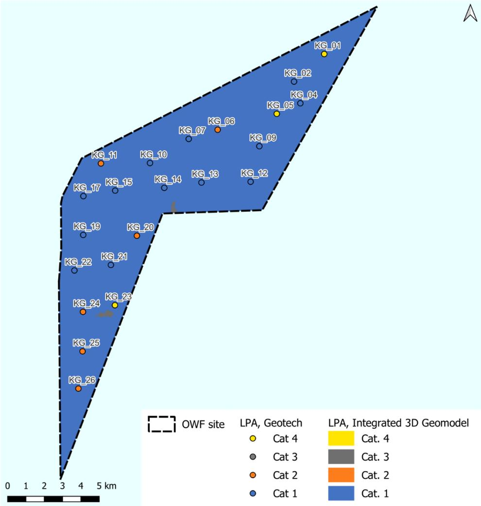
Figure 11-2 Results from leg penetration analysis for Generic Installation Vessel.
