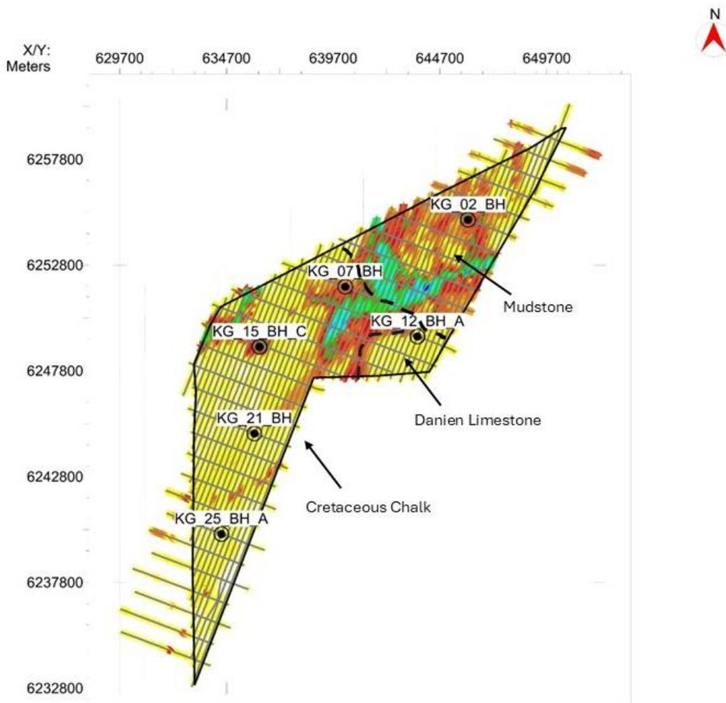
*Figure 9-18 Map of the top of the bedrock with the boreholes of Kattegat OWF marked. The black stippled lines mark the estimated boundaries between Danien Limestone, Chalk, and Mudstone. These lines are estimated based on the descriptions from the boreholes, seismic lines and GEUS Pre-Quaternary map.*
