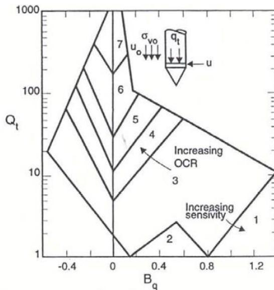
Figure 7-2 Robertson  $Q_t - B_q$  classification chart for soil behaviour type, cf. Ref. /2/. As recommended in Ref. /2/ the normalised cone resistance ( $Q_{tn}$ ) is considered instead of  $Q_t$  when evaluating the soil behaviour type.
