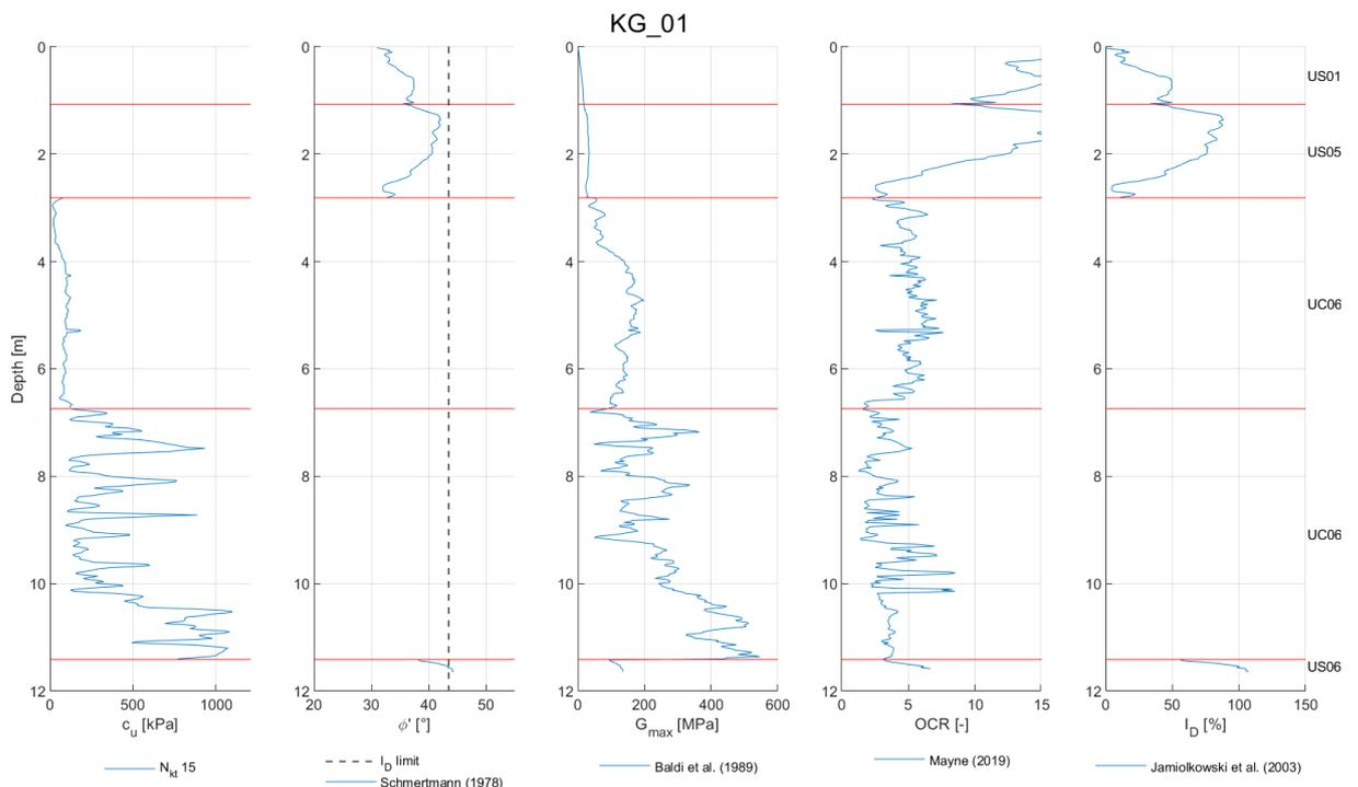
Figure C-1 Example of interpreted properties for KG\_01.
