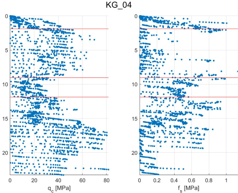
Figure 10-7  $q_c$  and  $f_s$  from CPT measurements for KG\_04 found as representative for zone I. More information about the location can be found in Appendix A.
