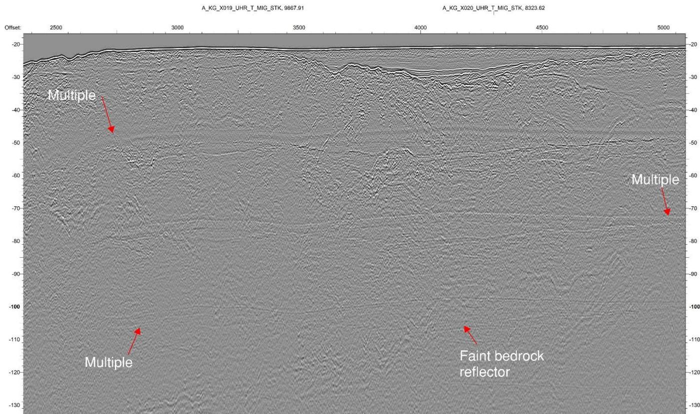
*Figure 9-1 Seismic line A\_KG\_L026A\_UHR\_T\_MIG\_STK. Example of the seismic quality showing 3 seabed multiples. Notice the low amplitude of the deeper reflectors which has lost energy due to attenuation.*
