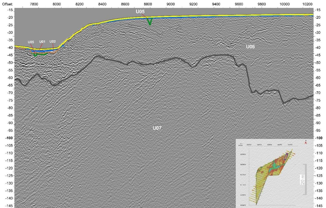
Figure 9-16 Seismic line A\_KG\_L043\_UHR\_T\_MIG\_STK. Example of U07 seen bounded to the top by B06 (Black horizon). The unit has in this example parallel inclined reflectors but is also found with parallel horizontal reflectors and with a chaotic facies. The overview map in the lower right corner shows the position of the profile (red line), the displayed section (blue area), and elevation of top of U07 (see also enclosure 3.07).
