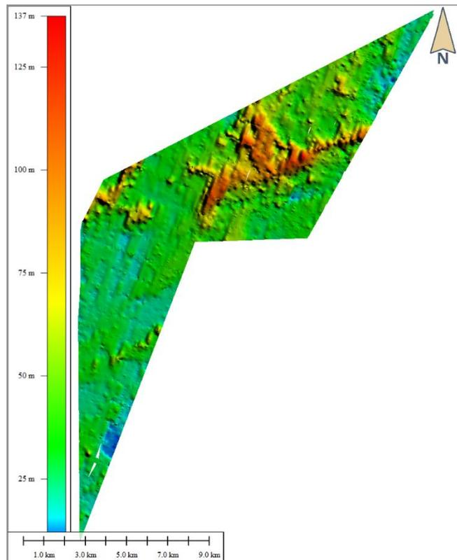
Figure 10-4 Depth below seabed to top of pre-Quaternary layers and deeper units defined as top of unit U07.
