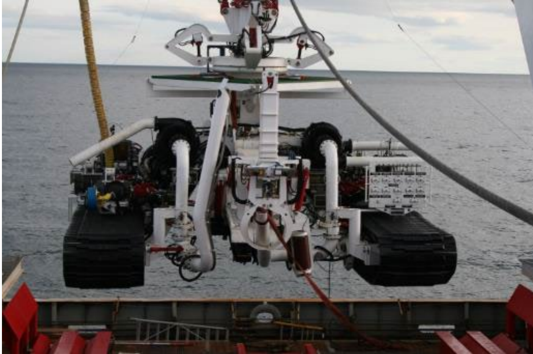
Helix Robotics I-trencher
