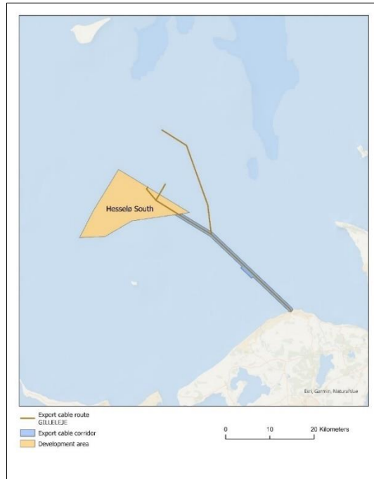
Figure 4-5. Hesselø OWF area and export cable corridor. The export cable corridor was previously investigated during the planning of the first Hesselø OWF area. Source: Energinet.
