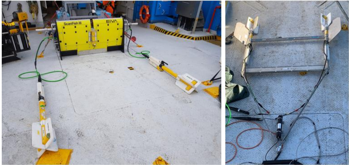
Figure 5-1: Magnetometer setup with two magnetometers on the Scanfish III from EIVA (left) and TVG frame (right) - the examples are from Mintaka I
