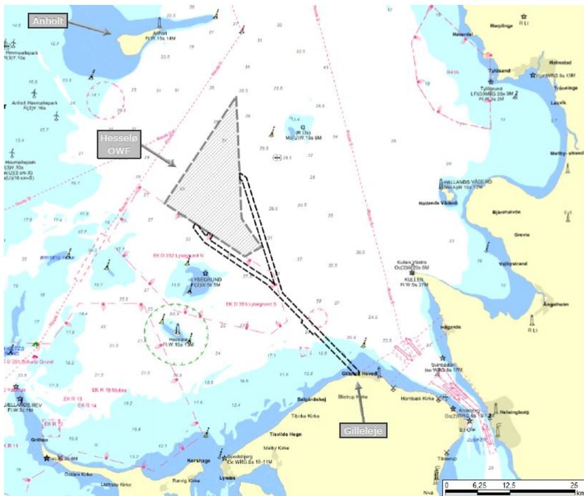
**Figure 6-8** Navigational chart for the southern part of Kattegat showing main ship routes, sea markings and bathymetry. The area of Hesselø OWF (the grey shaded area) is overlaid on the chart together with the position for the cable corridors and cable alignment (the dashed black lines). Source of the navigational chart: <https://kartor.eniro.se/?l=nautical>
