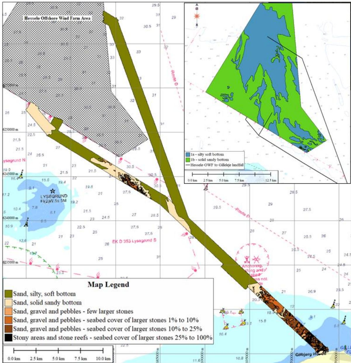
Figure 5-14 Overview of the interpreted seabed substrate types alongside the ECR corridor from Gilbjerg Hoved in the south to the OWF area in the north.
