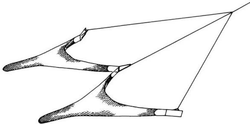
**Figure 6-5 Principal features of a twin trawl, source FAO.**
