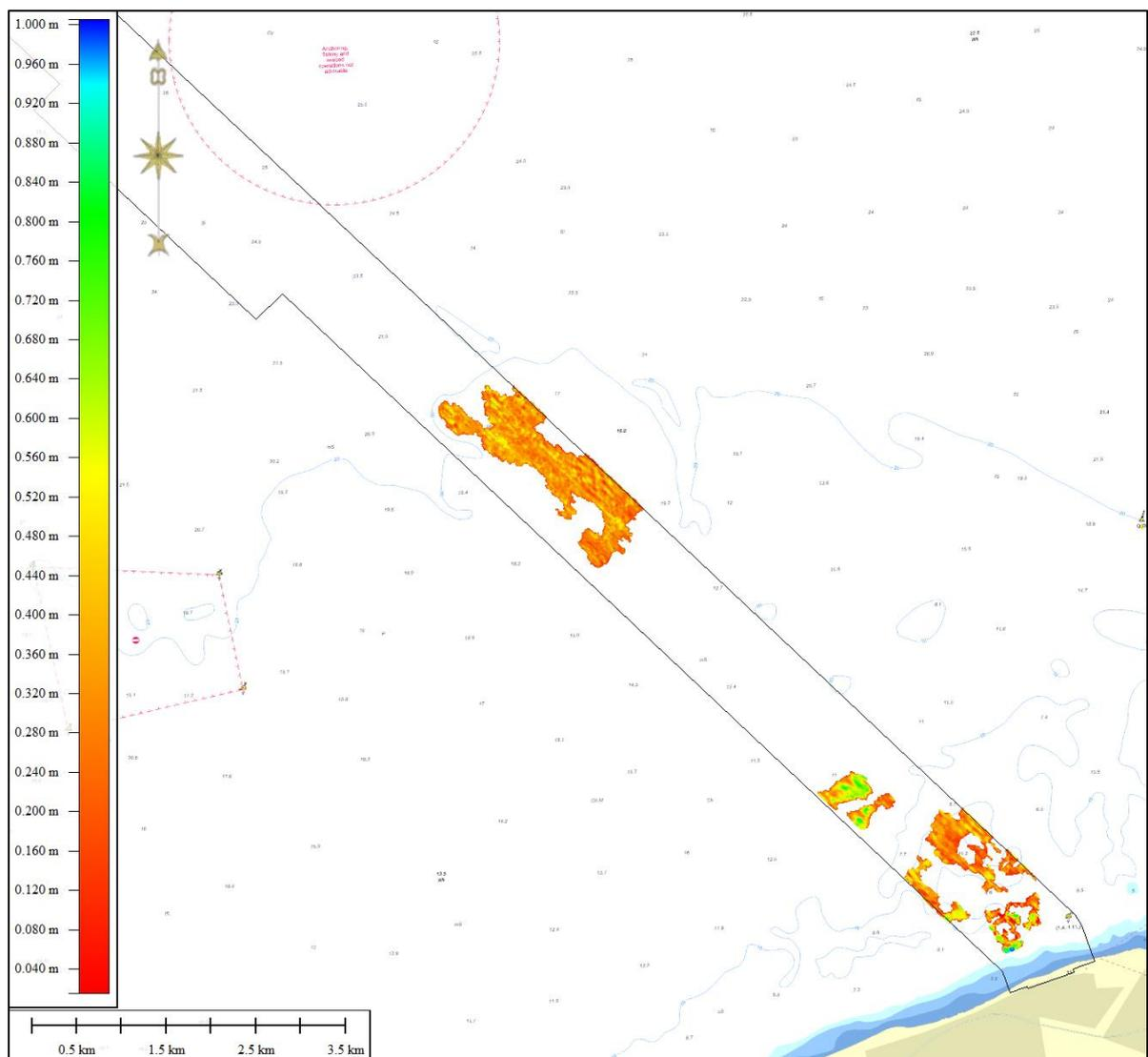
**Figure 5-3 Thickness map of the Holocene unit PG IV composed of coarse-grained sediments, sand and gravel. Typical thickness of the unit: 0.2-0.5m.**
