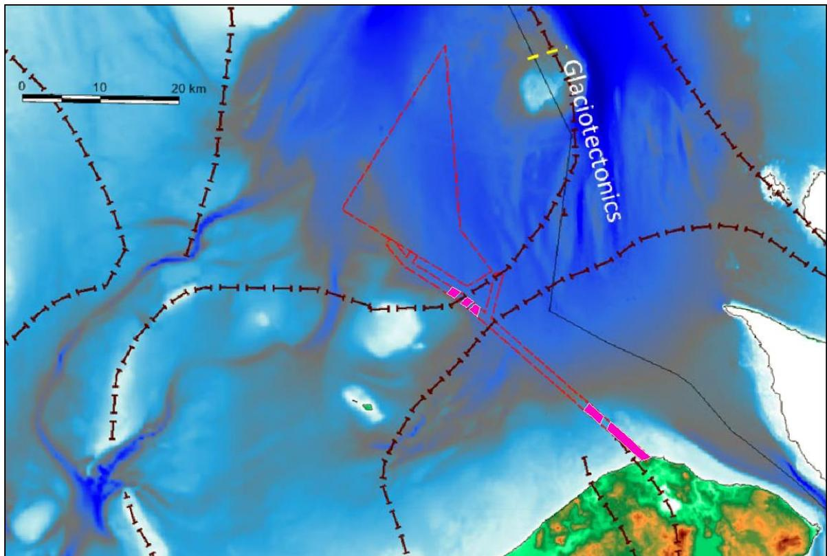
**Figure 5-12 Distribution of the glacial deposits (GL) along the cable corridor. The areas where glacial sediments have been identified close to the seabed are marked with pink. Ice marginal ridges interpreted in the previous studies in the southern Kattegat region are marked with black**
