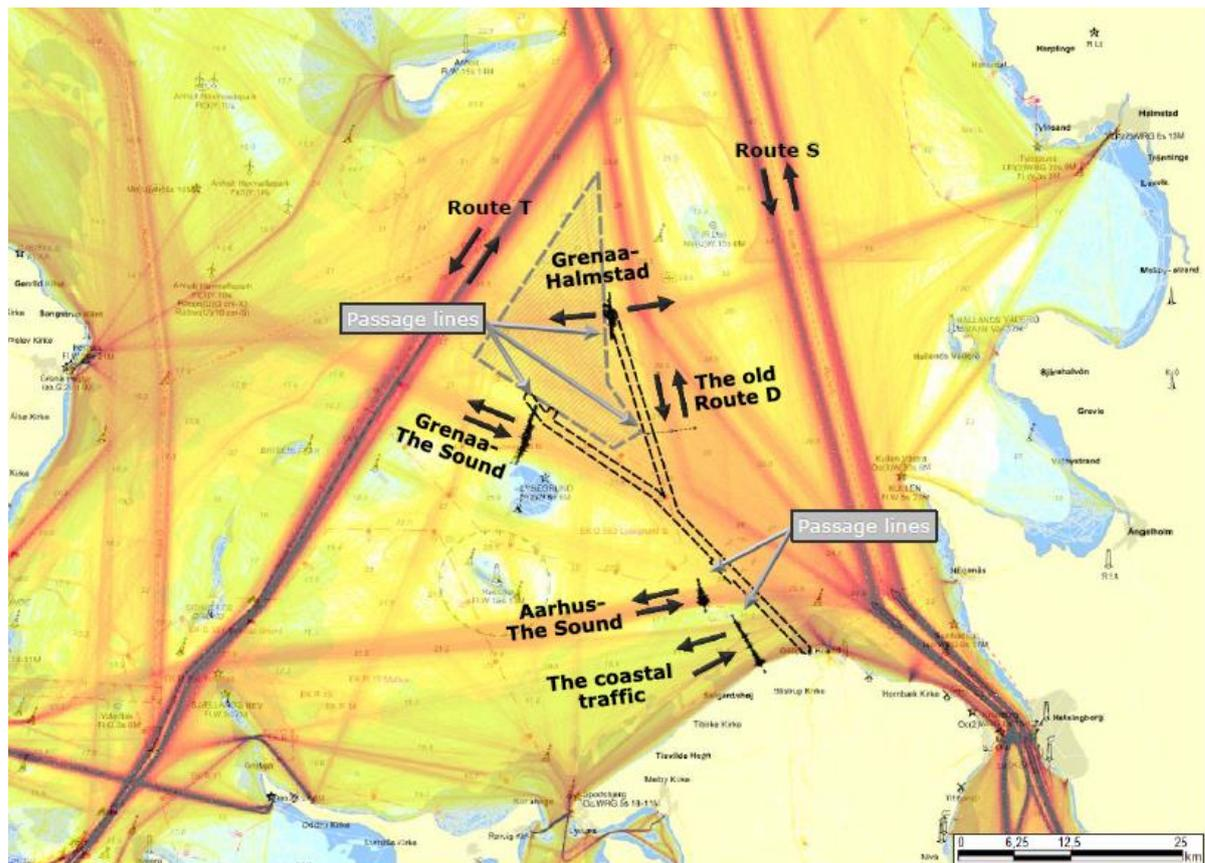
**Figure 6-9 Ship traffic intensity covering from 1st of July 2020 until 1st of May 2021 in the area around the OWF and its cables corridors. The identified routes crossing the cable corridor and location of the passage lines are marked.**
