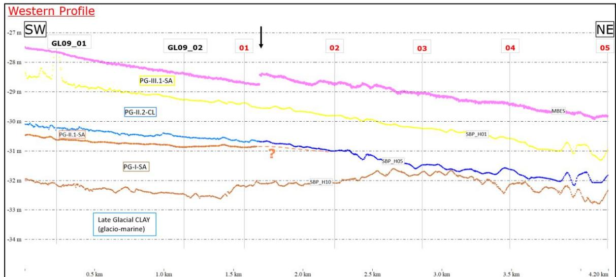
**Figure 5-22 Geological sections along the Western profile. The black arrow marks merging point between Hesselø ECR and OWF site areas. Geotechnical sampling points (CPTs and VCs carried out by Mewo) as well as synthetic borehole positions are included.**
