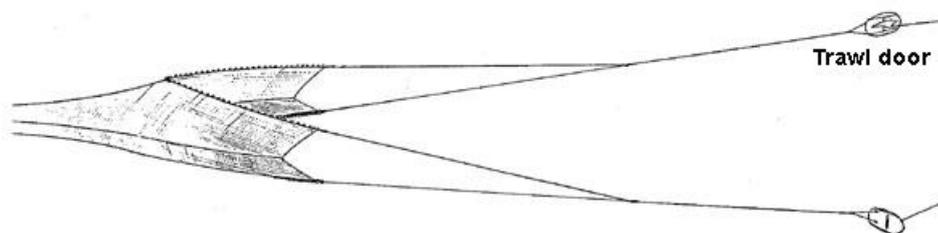
**Figure 6-4 Principal features of an otter (bottom) trawl, source FAO**
