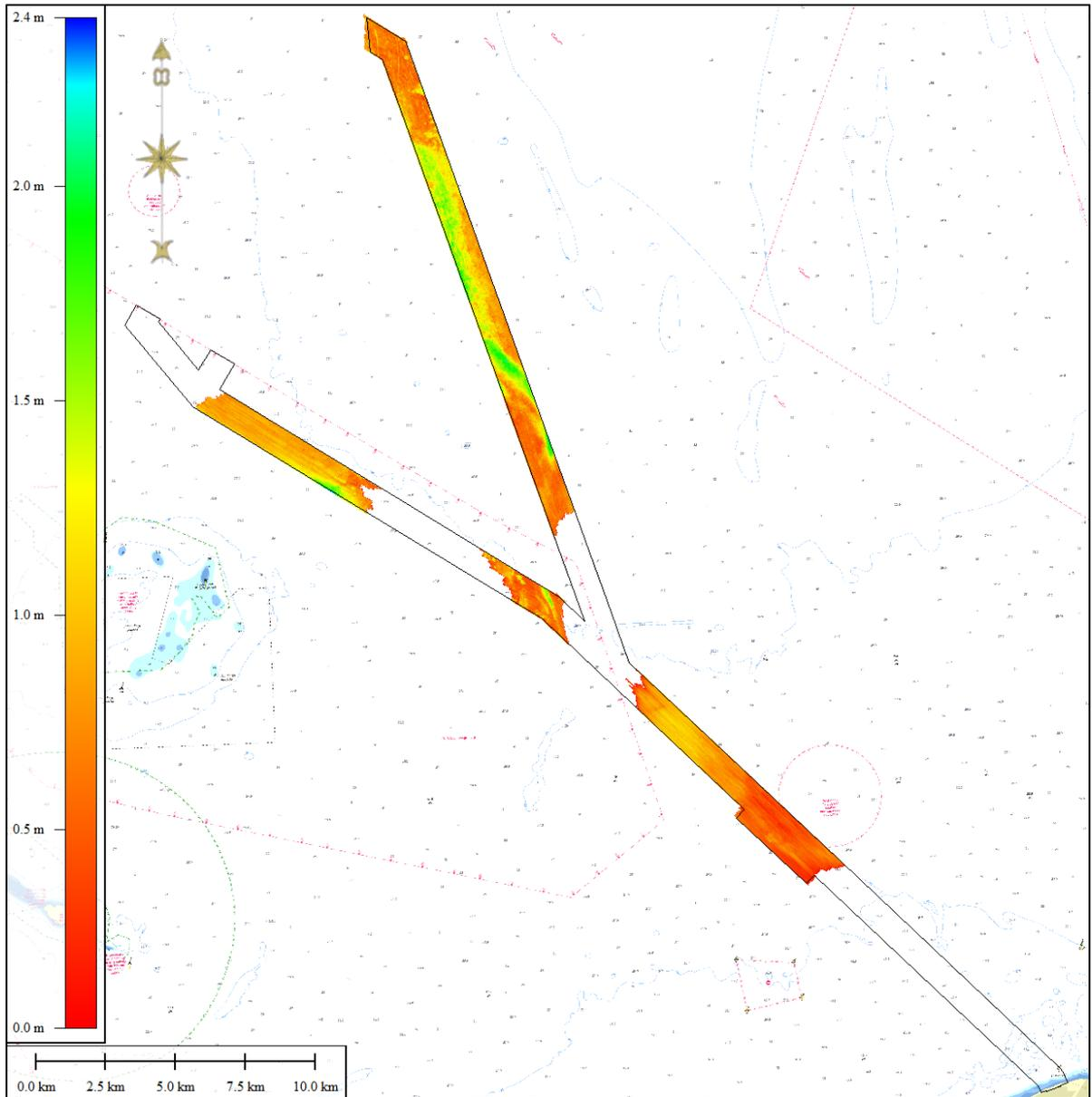
**Figure 5-5 Thickness map of the Holocene clay unit PG III.2 CL, typical thickness of the unit: 0.5-2.0m.**
