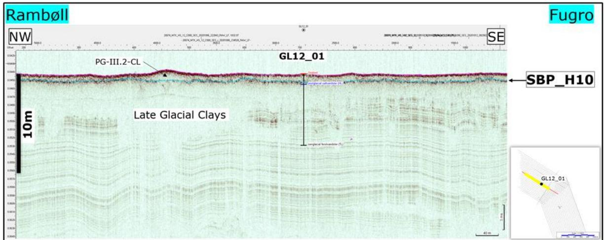
Figure 5-17 Eastern arm, cross section showing correlation between seismic horizons interpreted for Hesselø ECR and OWF site area
