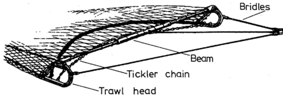
**Figure 6-3 Principal features of a beam trawl, source FAO.**
