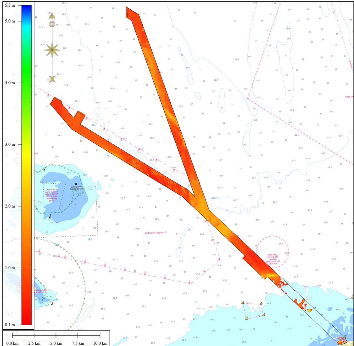
**Figure 5-6 Total thickness map of the youngest Holocene deposits- unit PG III.1 SA and PG III.2 CL.**
