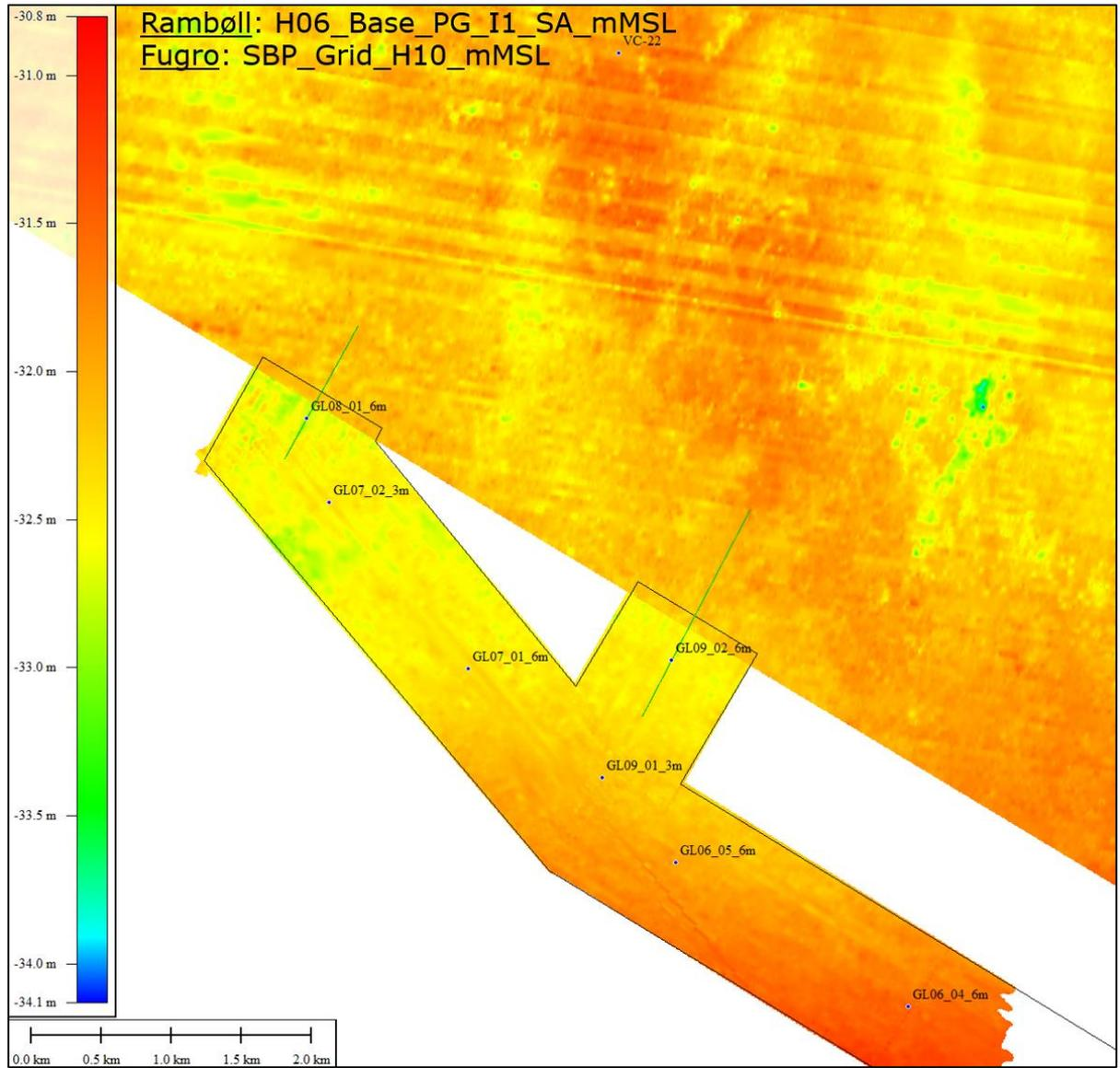
Figure 5-20 Western arm, Base PG I (Sand). Difference between models approx. 30-45 cm
