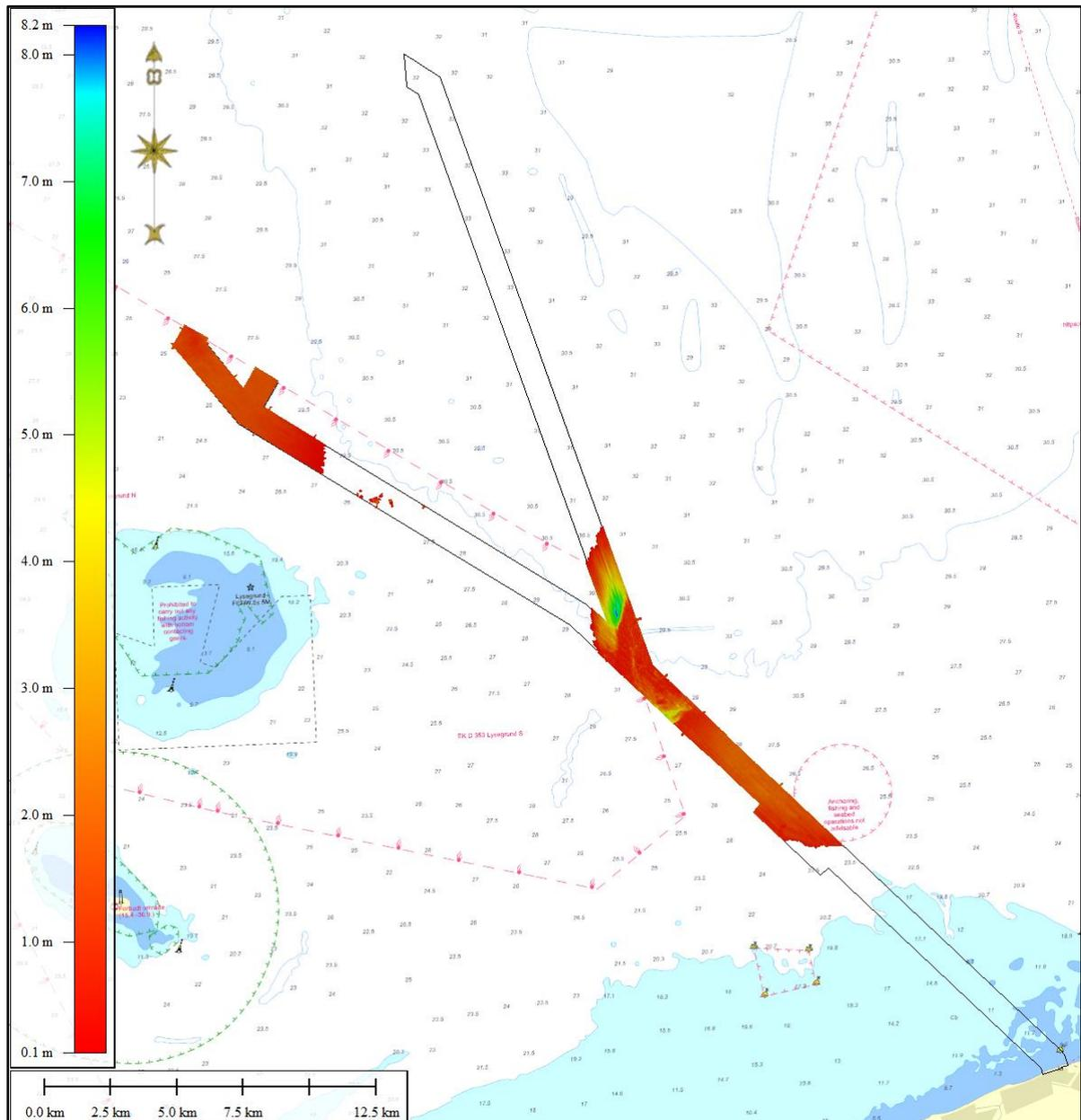
Figure 5-10 Thickness map of the Early Holocene sand unit PG I.
