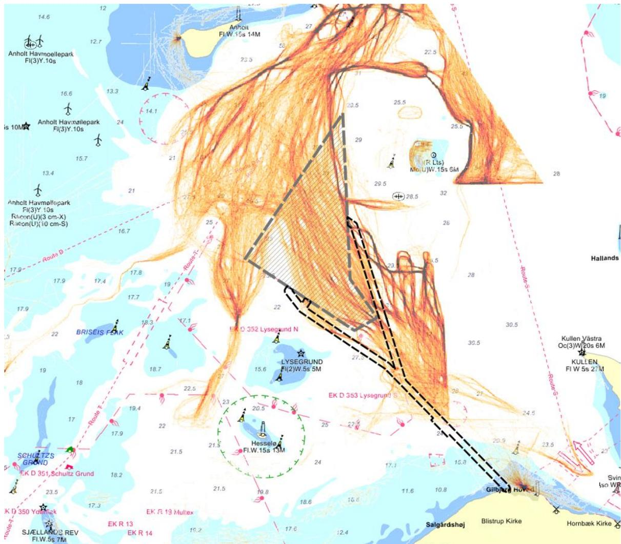
Figure 6-2 Ship traffic intensity covering only fishing ships sailing 2-4 knots corresponding to trawling speeds, from 1st of January 2019 until 31st of December 2019 in the area around the OWF and its cables corridors. The data does not cover the north-eastern corner, which is why a straight line is seen.
