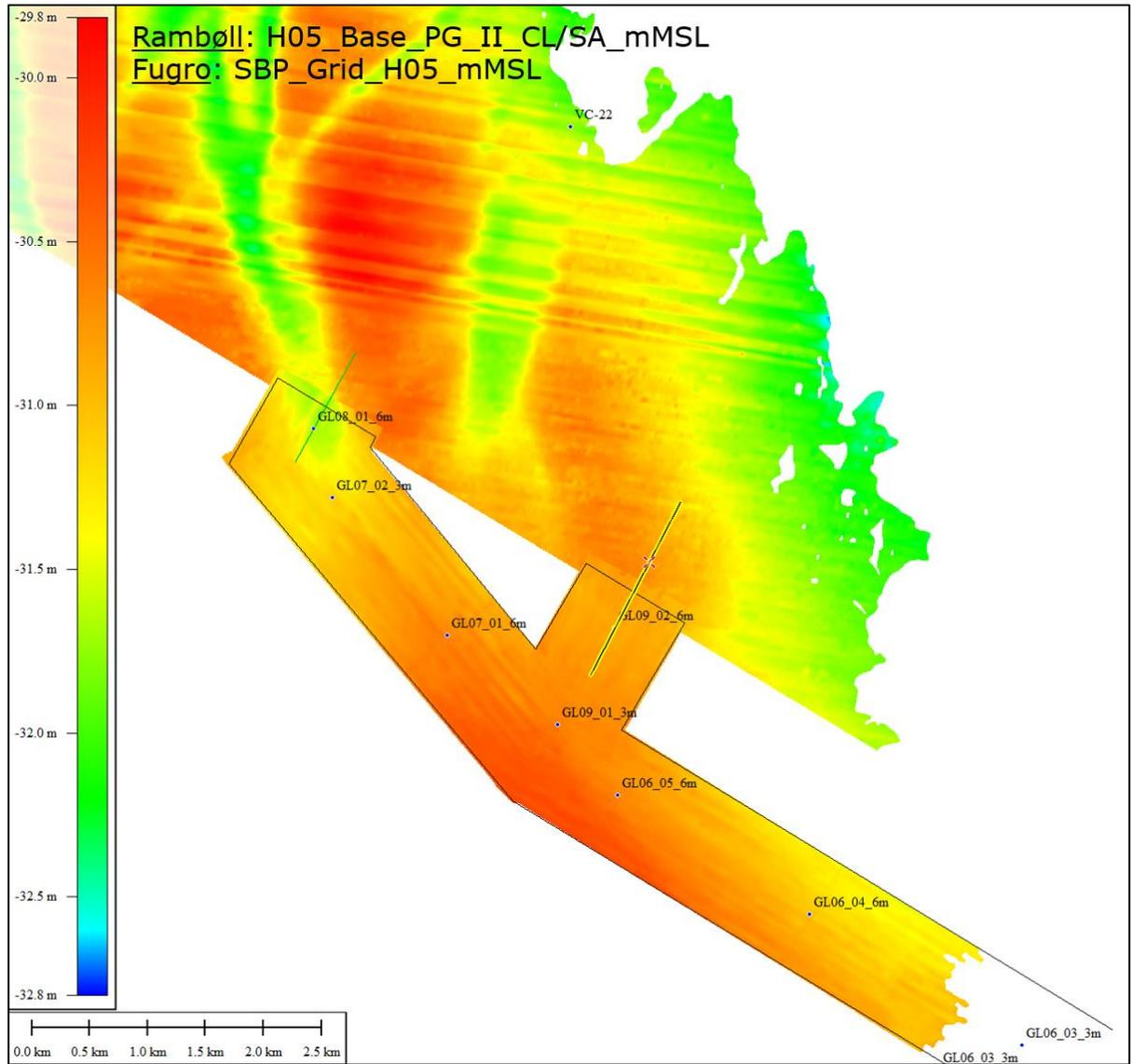
Figure 5-19 Western arm, Base PG II (Sand). Difference between models approx. 15-20 cm
