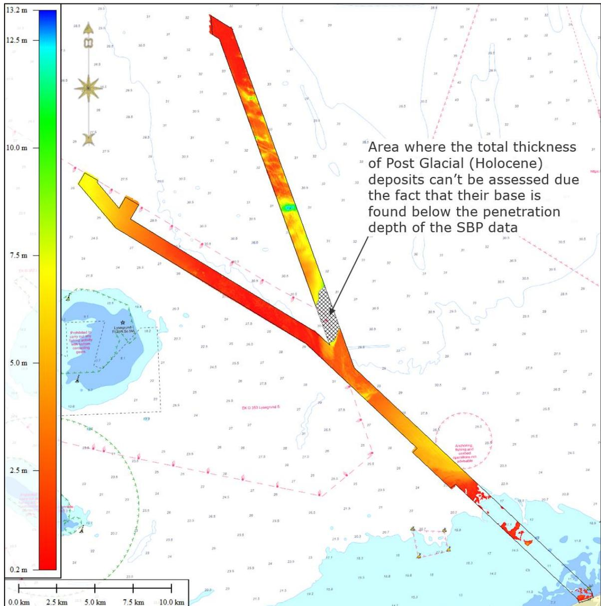
**Figure 5-9 Total thickness of the Post Glacial sediments, typically: 0.5-6.0m.**
