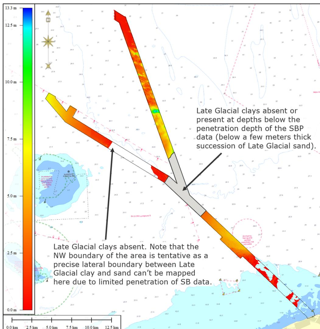
**Figure 5-11 Depth in meters below seabed to the top of the Late Glacial succession (LG CL).**
