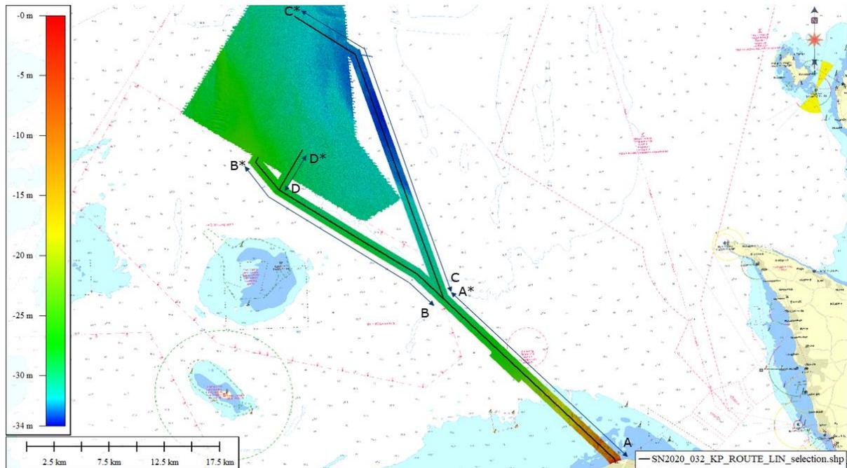
Figure 7-4: Water depth for the cable route
