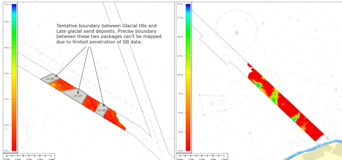
**Figure 5-13 Depth in meters below seabed to the top of the Glacial succession (GL).**
