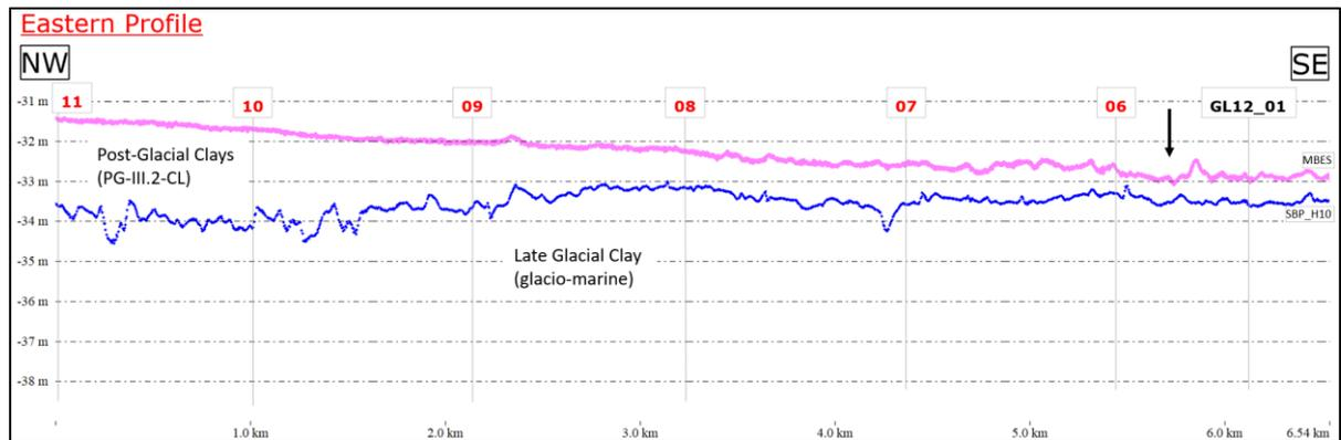
**Figure 5-23 Geological sections along the Eastern profile. The black arrow marks merging point between Hesselø ECR and OWF site areas. Geotechnical sampling points (CPTs and VCs carried out by Mewo) as well as synthetic borehole positions are included.**
