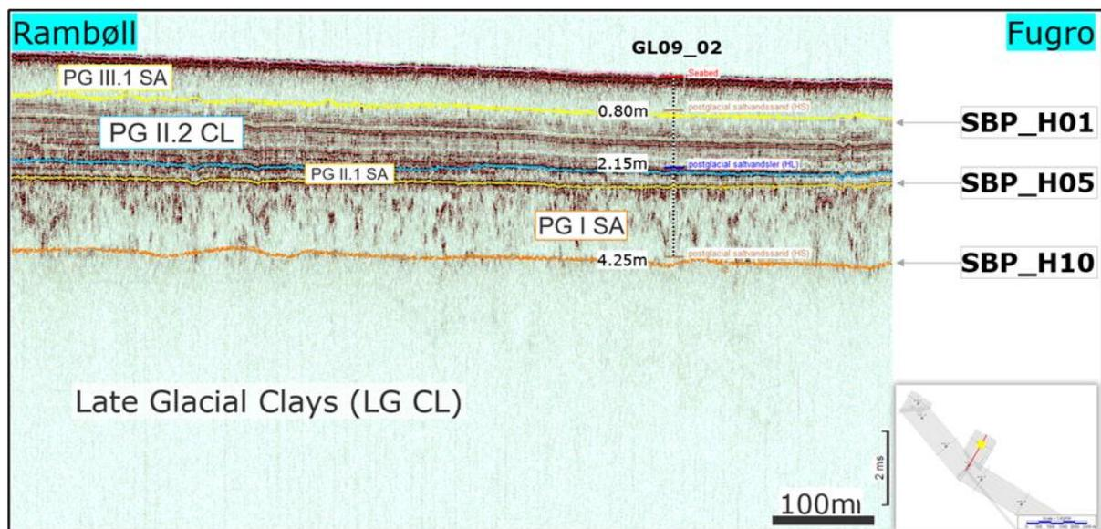
**Figure 5-16 Western arm, cross section showing correlation between seismic horizons interpreted for Hesselø ECR and OWF site areas**
