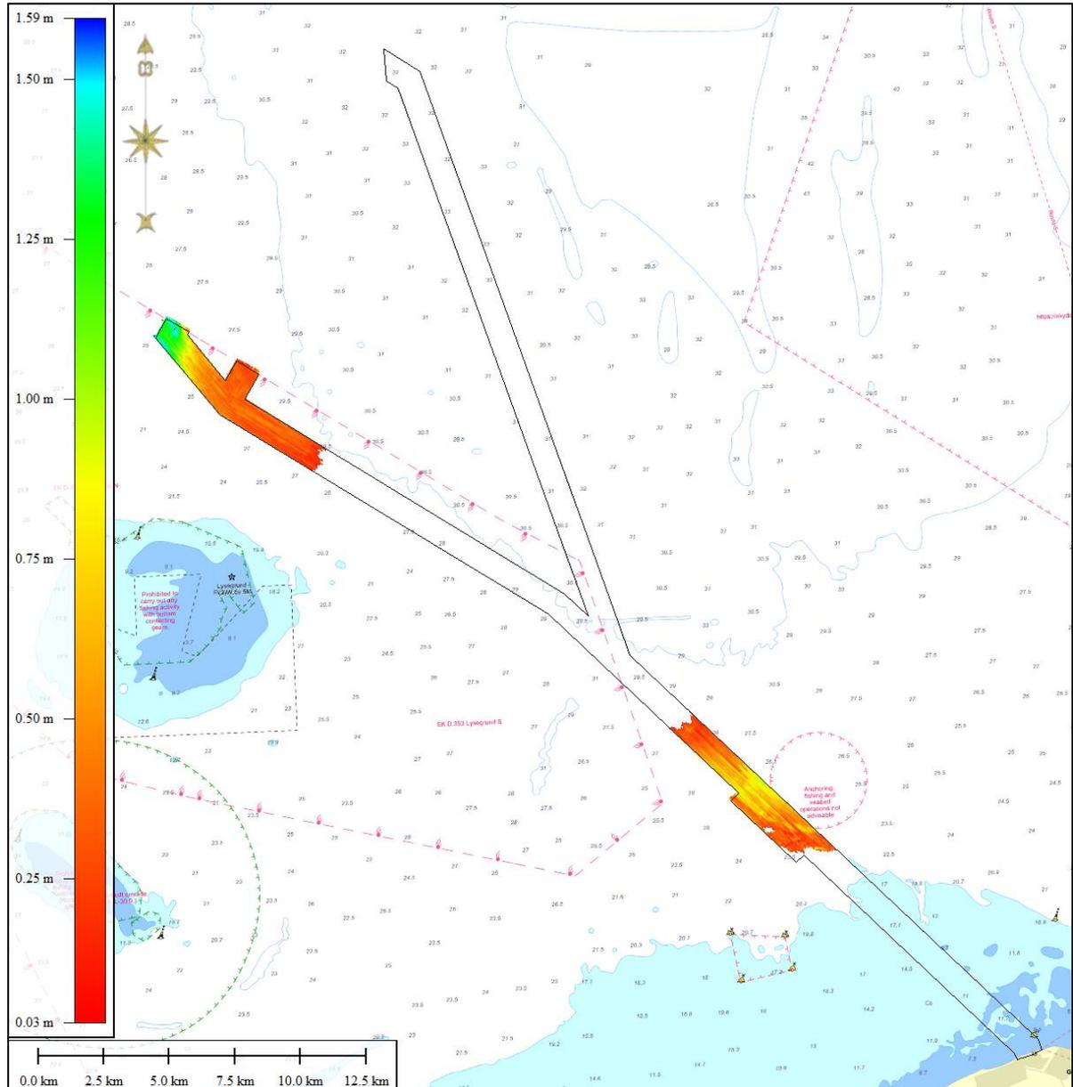
**Figure 5-7 Thickness map of the Holocene sand unit PG II.1 SA.**
