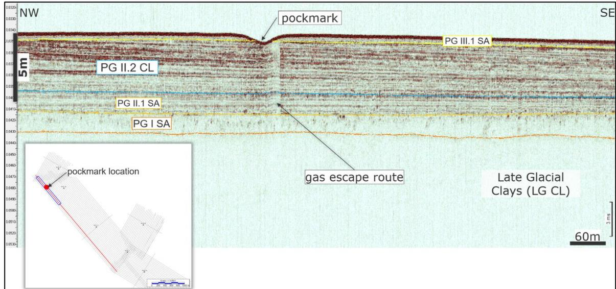
**Figure 7-2 Location of the pockmark identified on the acquired SBP data, line 20085\_MTK\_GL\_07\_L405\_SES\_20201107\_200440\_RAW\_LF**
