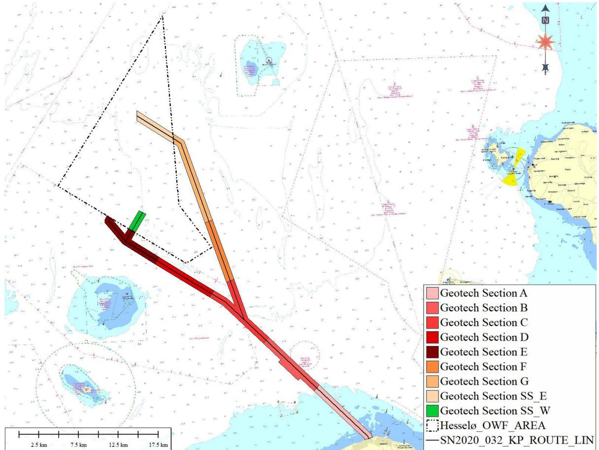
Figure 7-7 Subdivision of the ECR into geotechnical sections
