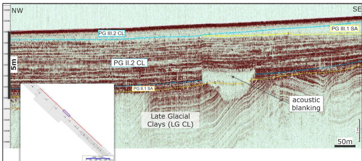
**Figure 7-1 Example of a shallow gas accumulation**
