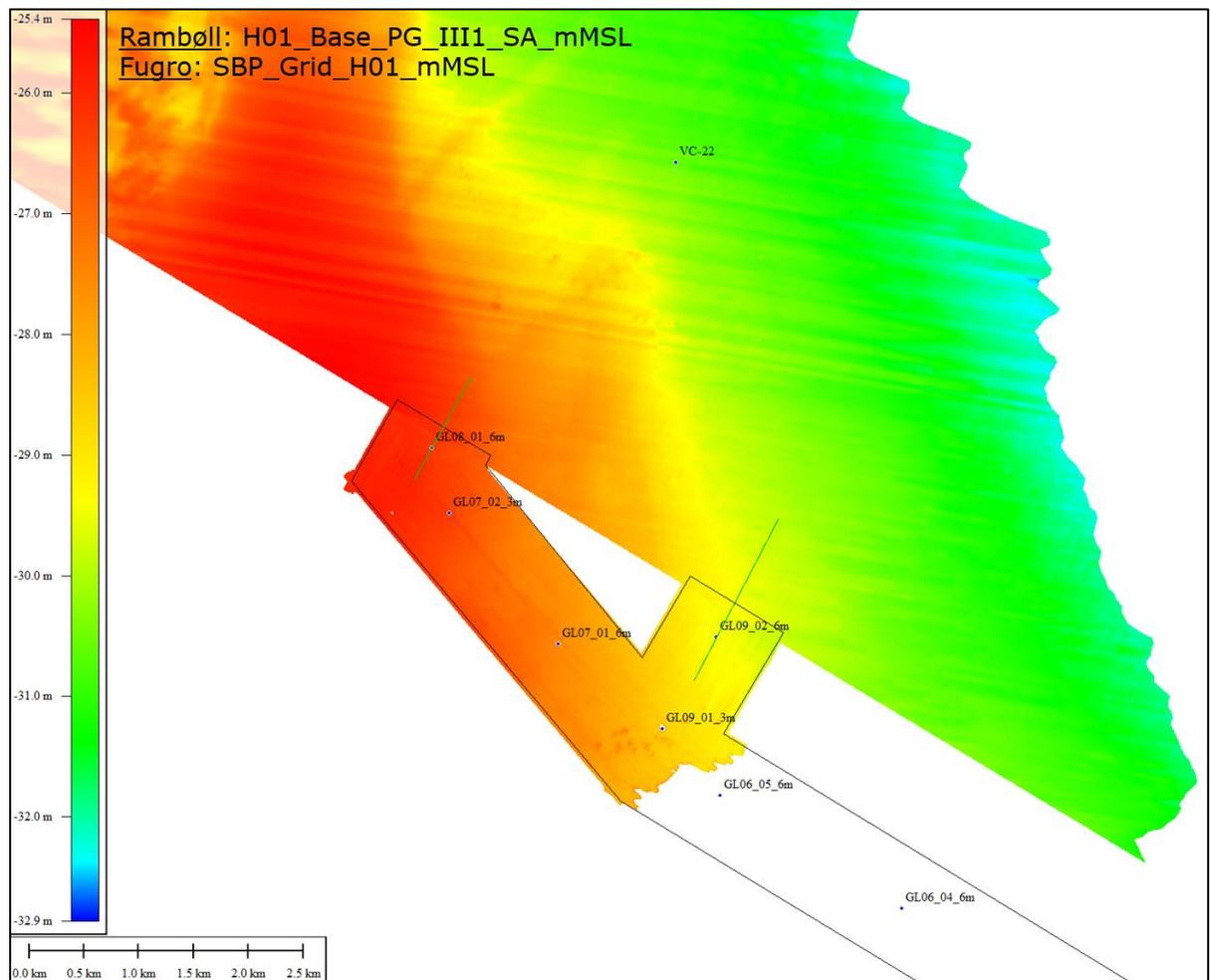
Figure 5-18 Western arm, Base PG III (Sand). Difference between models approx. 5 cm
