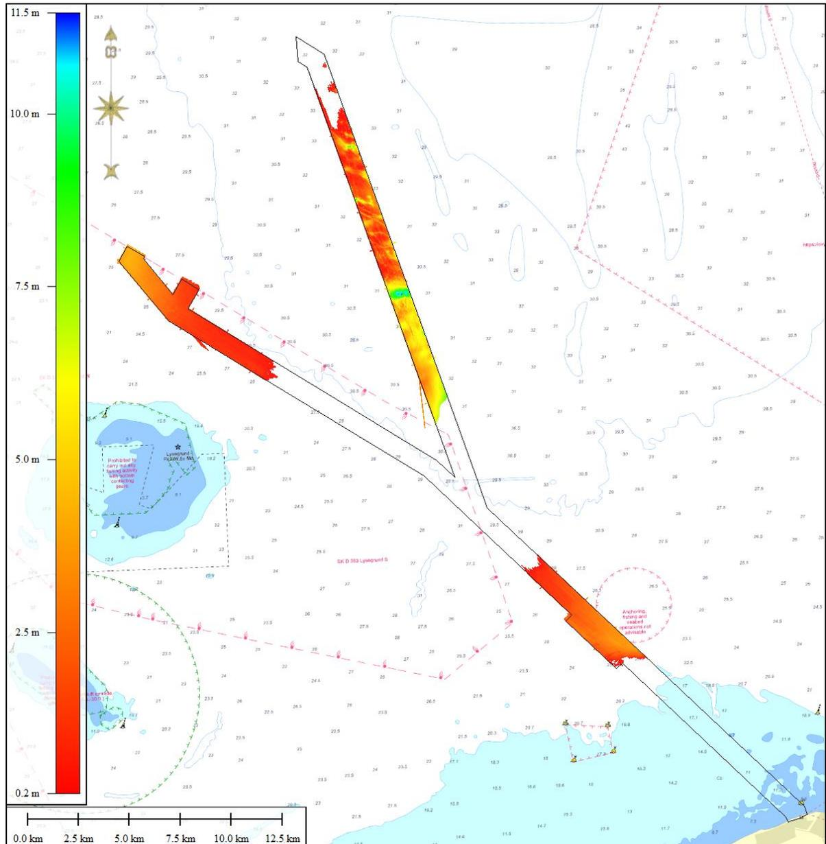
**Figure 5-8 Thickness map of the Holocene clay unit PG II.2 CL.**
