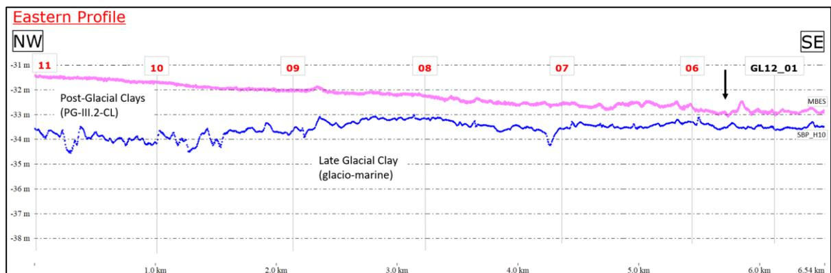
Figure 7-19 Geological section and synthetic boreholes along the Eastern arm.
