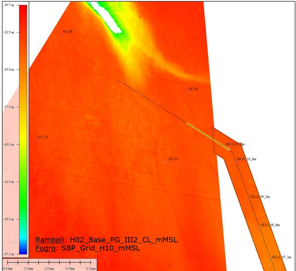
**Figure 5-21 Eastern arm, Base PG III (Clay). Difference between models approx. 0-5 cm**
