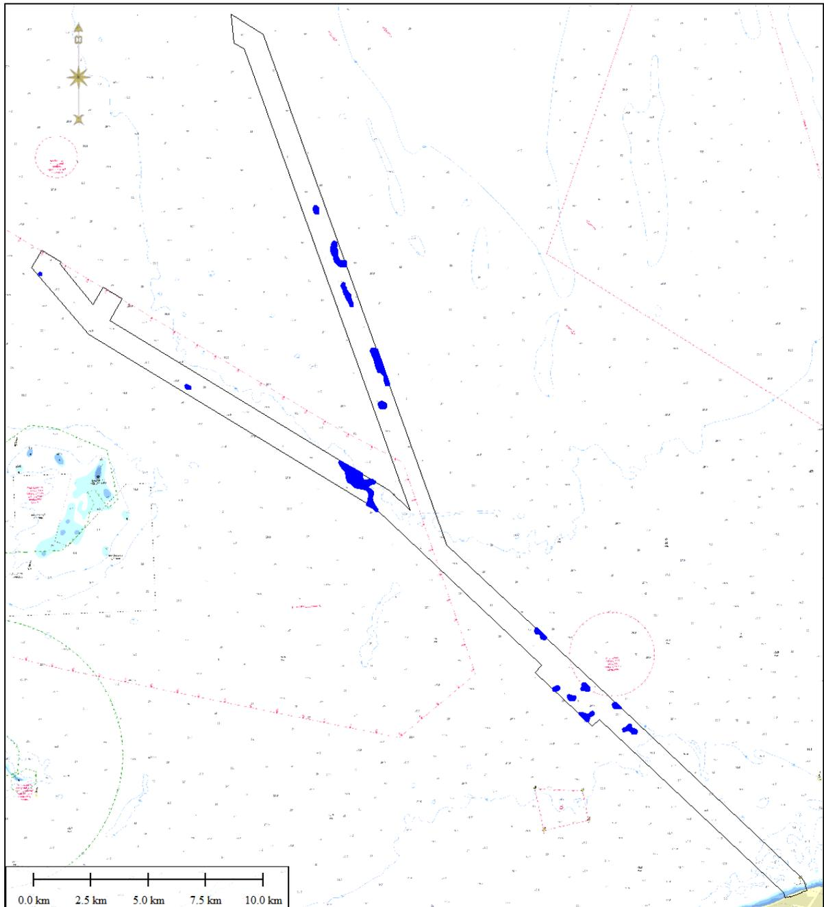
**Figure 7-3 Overview of locations showing the most pronounced presence of gas-filled sediments (marked with blue) within the Hesselø cable corridor.**
