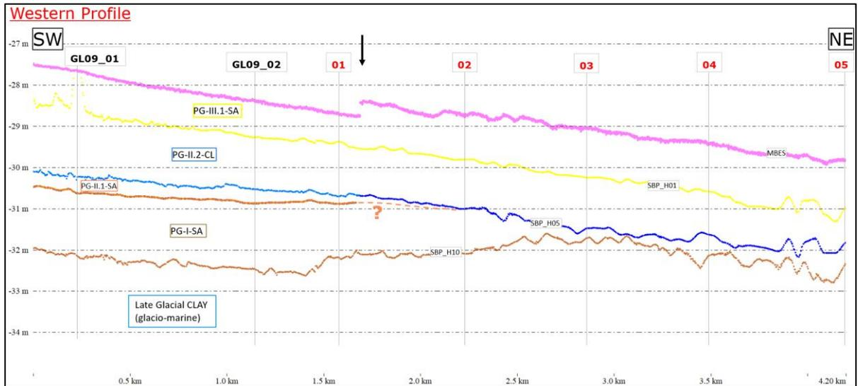
Figure 7-17 Geological section and synthetic boreholes along the Western arm.
