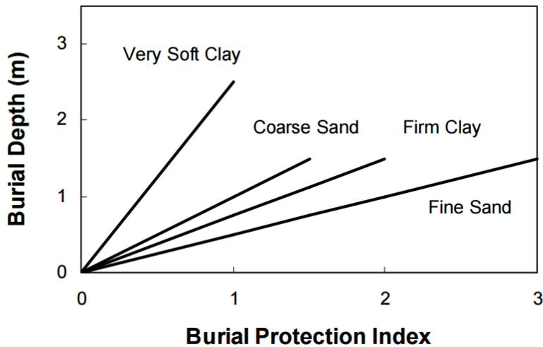
Figure 6-10 Relationship between BPI and burial depth in different soils /Ref 4/
