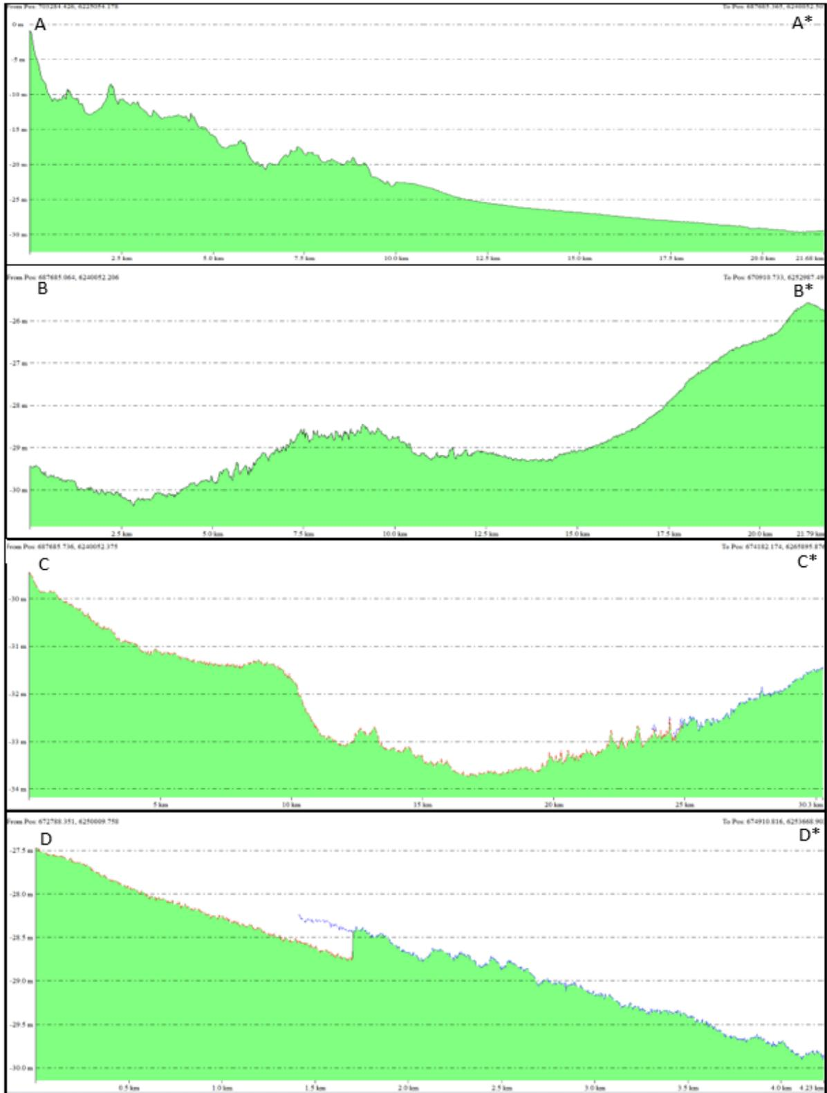
Figure 7-5: Cross-sections of the bathymetry along the cable route
