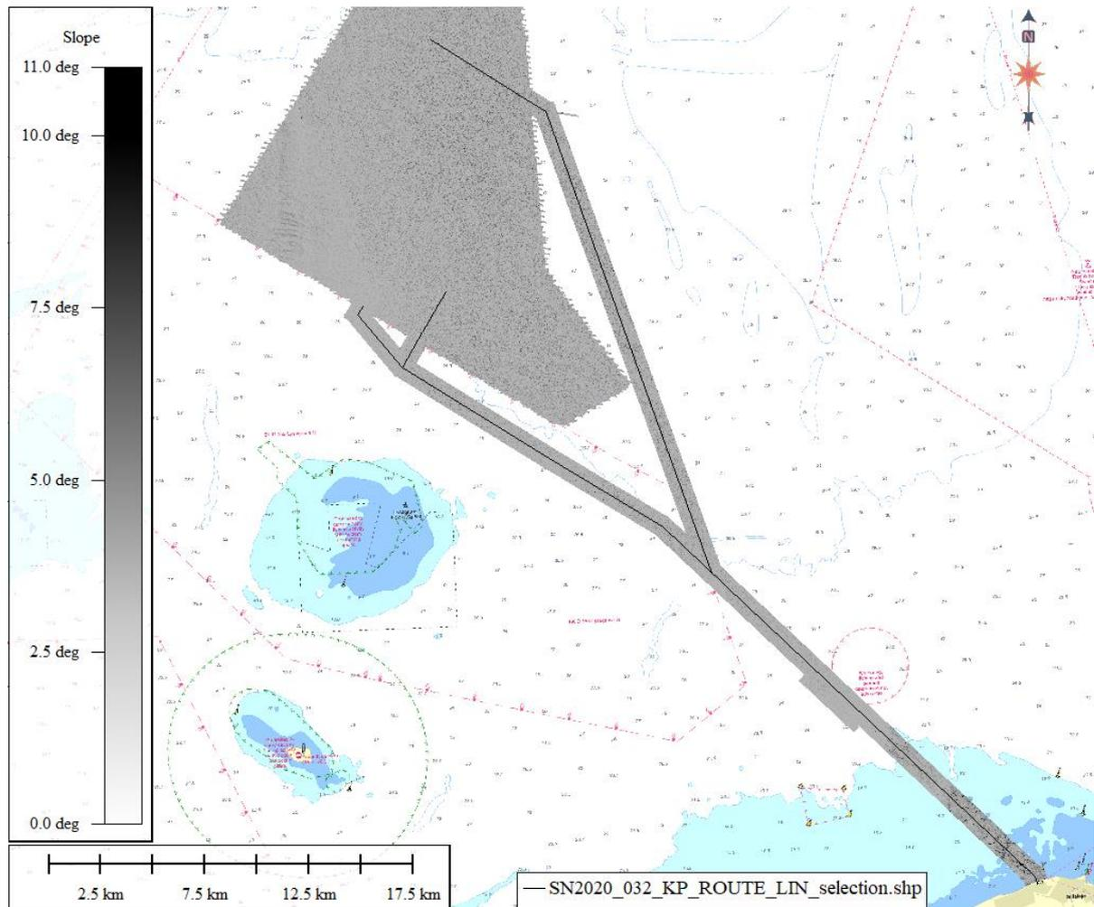
Figure 7-6: Slope in degrees along the cable route
