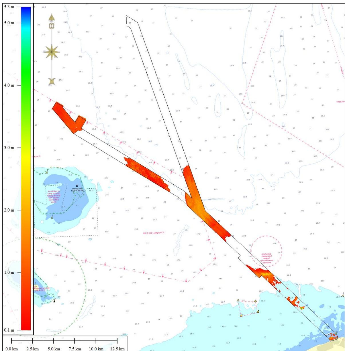
Figure 5-4 Thickness map of the Holocene sand unit PG III.1 SA, typical thickness of the unit: 0.5-2.5m.
