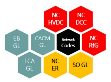
The connection codes (red) specify the minimum technical requirements that any kind of power-generating facility must comply with to be connected to the grid system.
